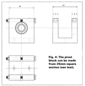
the block as shown in Fig. 4, and nip the bearing with a small screw.
