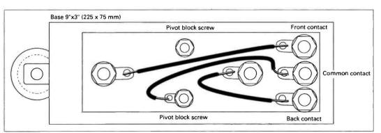
Fig. 9: An ideal position for the terminals is at the back edge of the key base, centrally positioned.
