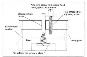
Fig. 7: The final method of tension adjustment described by G0MSZ, uses a tension spring, tensioning pin and an adjusting screw with a specially shaped head (see text).
