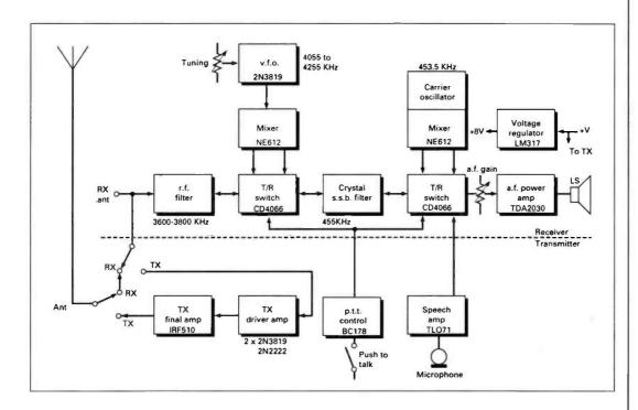
The 'Tiny Tim' is a 3.5MHz single sideband 'phone Transceiver In Miniature (hence Tiny TIM!). My aim was to design a rig which is complete, simple yet effective, low cost, suitable for home construction and with an output of about 10 to 20W p.e.p.
