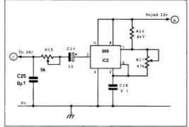
Fig. 2: The transceiver sidetone circuit.
