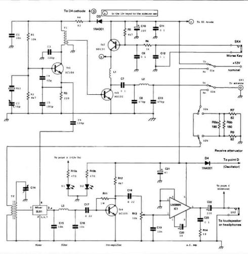
Next to be fitted was the p.a. and switching transistors. I didn't get nearly as much power out with the BD131 as Steve. So I exchanged it for a BFY51 and got about 1W out.
