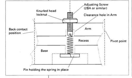
Standard taper pins are available such as 7/32 in diameter with a standard taper of 1/4 in in 12in, etc. Both the arm and block should be reamered together with shimming washers to provide the desired gap.
