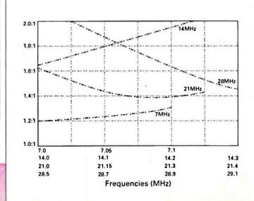
Fig. 5: Plotted s.w.r. curves of full-wave (on 7MHz) delta loop.
