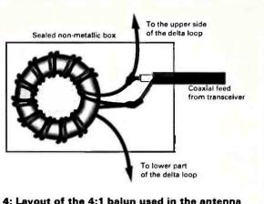
Fig. 4: Layout of the 4:1 balun used in the antenna system.
