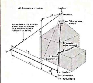
Fig. 3: House and asymmetrical loop antenna.
