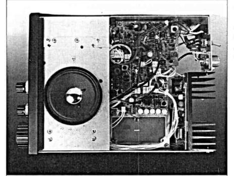
Fig. 2: An internal view of the Model 555 transceiver, showing the heatsinking for the p.a. stage (right).
