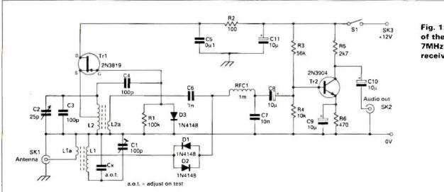
Fig. 1: Circuit of the basic 7MHz d.c. receiver.
