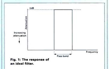
specifications are quoted it's necessary to look at the characteristics of the filters which are used. In an ideal world a filter characteristic would look like that shown in Fig. 1.
