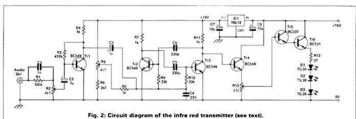
The resistor R13 serves as a current limiter. It can be used to monitor the diode drive which is set by R12 and must be set such that the l.e.d. (s) are not over-driven.
