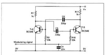
Fig. 1: A simple square wave generator, capable of being frequency modulated, forms the basis of the G6KSN infra red communications project (see text).
