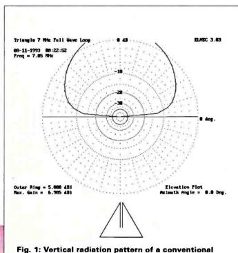
Fig. 2: Vertical radiation pattern of a conventional delta loop fed at bottom corner.
