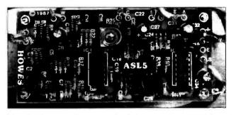
Fig. 1: Close-up photograph of the completed ASL5 dual bandwidth audio filter, as built by Tex Swann G1TEX.
