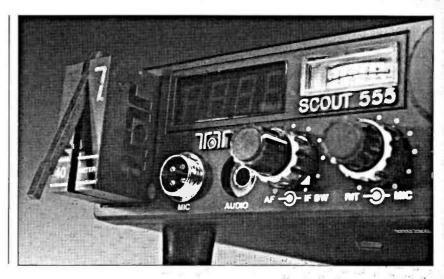
Fig. 1: Changing the band module on the Ten-Tec Scout 555.
