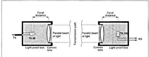
Fig. 4: To extend the range of the infra red communications system, a suitable lens is required for each installation. For practical operation, G6KSN recommends mounting the optical assembly on photographic tripods (see text).
