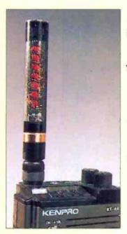
Once again PW has found an interesting item for Subscribers' Club Members and this time it's in the form of a novel plugin power checker. The Revex Power Checker PC 705 is ideal for hand-held transceivers and has a built-in BNC plug so that it can connect straight into the antenna socket of your rig. Capable of indicating power output levels of up to 5W, the Revex Power Checker's
