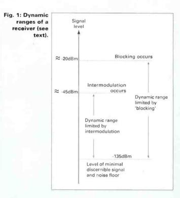
that might mask out the weak wanted ones. In this case the level of the intermodulation products must not be any greater than the m.d.s., i.e. no greater than the noise floor of the set. But again care should be taken to inspect exactly how the measurements are taken.
