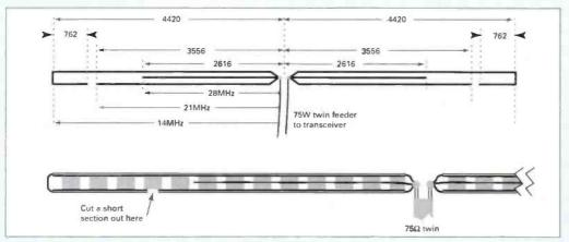
Fig. 3: Dave's dipole. Dave Raynor G4XNP uses a simple, but effective, three band dipole with this layout. The 28MHz elements are threaded through the holes of the slotted  $300\Omega$  feeder.
