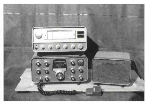
Fig. 2: The Heathkit SB-101 h.f. transceiver, with matching speaker/p.s.u., on the bottom with the KW 201 h.f. receiver on top.
