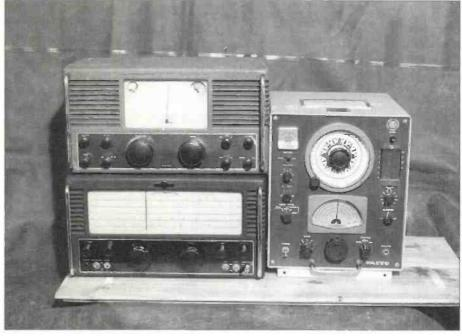
Fig. 4: The two Eddystone receivers on the left (top to bottom) are the \$504 and the \$750. Pictured on the right is a marine a.d.f. receiver, which will (if supplied with the correct antenna), provide a directional bearing on the signal being received.
