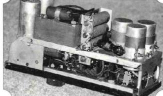
Fig. 9: Power supply chassis. The horizontally mounted metal rectifiers (with cooling fins) can be seen on the top centre (see text).
