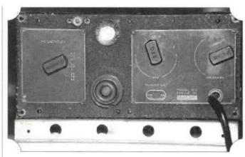
Fig. 3: Receiver section of the B2, showing magnifying lens mounted above tuning scale and slow motion tuning knob (see text).
