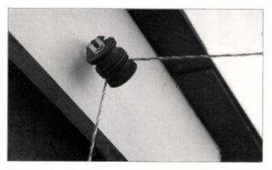
Fig. 1: An insulated 'pulley' for the washing line antenna. The electric fence (rope), forming the new washing line, has metal strands running through it.
