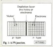
flows. The reason for this is that the holes are attracted towards the negative potential which is applied to the P type region.
