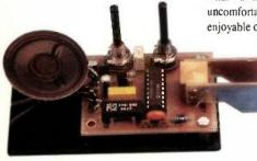
The double 'touch' paddle electronic keyer - available in ready made form only - from R A Kent (Engineers) proved to be a possible solution for G3XFD (see text).
