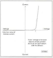
Fig. 3: Characteristics of a diode.
