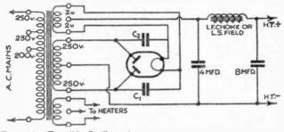
FIG. 146.—Two "buffer" condensers may be joined to the anodes of a full-wave rectifying valve to remove modulation hum.
