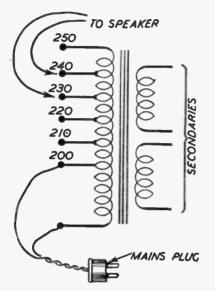
FIG. 190.—A " buzz " test for speakers using a mains transformer.
