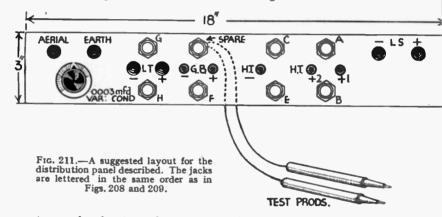
two ends of a tapped output transformer are connected to the two speaker terminals on the panel, the speaker itself being connected to any one of the other terminals by means of a flexible lead with spade terminal, and also to one terminal of a 4-mfd. condenser, the other terminal of which is joined to the earth terminal on the panel.
