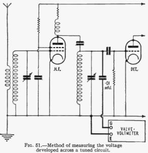
between 0 and 5 volts applied to the input terminals, and to obtain these readings the required voltage is selected by adjustment of the 250-ohm potentiometer with the 10-volt range of the universal meter connected across leads G and E and then noting the deflection given by the milliammeter when this voltage is applied to the valve-voltmeter. Some readers may care to plot a graph of these readings, and so be able to measure intermediate values directly, but the valve-voltmeter
