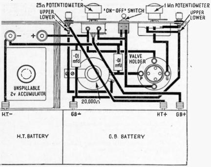
FIG. 48.-The full wiring plan for the valve-voltmeter.
