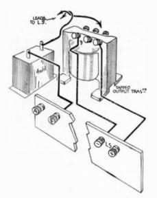
FIG. 210.—This shows how the refinement of a choke-capacity output filter can be added to the distribution panel.
