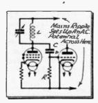
Fig. 151.—The coupling condenser is in series with the choke and leak across H.T.
