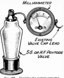
FIG. 163.-Checking the current consumption of an S.G. valve.
