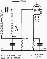
operated set the detector grid of the frequency-changer should be connected so as to receive the normal bias, as shown, when using the modified connections shown in Fig. 67.
