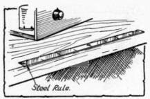
FIG. 194.—A steel rule screwed to the bench is handy for measuring wire, etc.
