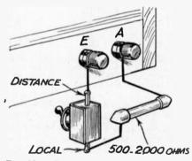
FIG. 96a.—Showing the simplest system of local-distance switching.
