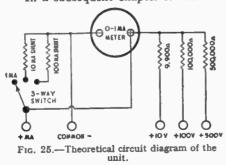
may be adapted for use as a direct-reading ohmmeter, giving accurate measurement of resistance for 500 to 50,000 ohms, by the insertion of the battery variable resistance and which have already been calibrate the used to various ranges. Space for this addition has been provided in the box, and
