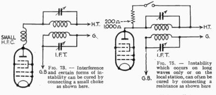
of one or both of the transformers. In most cases it will be sufficient to join a 500-ohm resistance in parallel with the primary of the first I.F., as shown in Fig. 75.
