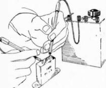
FIG. 29.—Showing the resistance calibrated readings added to the scale of a milliammeter.
