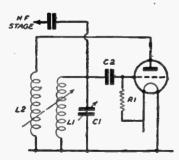
FIG. 83.—Theoretical diagram of a standard reaction circuit.
