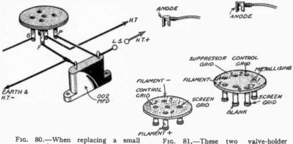
power valve by a pentode, a 5-pin holder must be used, a lead being taken from the centre socket to H.T. + as shown, and a fixed condenser joined between the anode socket and earth. FIG. 81.—These two valve-holder illustrations clearly show the altered connections required when replacing a 4-pin H.F. valve by a 7-pin H.F. pentode.
