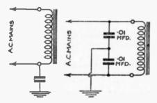
FIG. 144.—A condenser between earth and one side of the primary will prove very useful as a hum remover.
