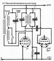
FIG. 70.--When a double-diode-triode type of valve is used as second detector the I.F. transformer which feeds it should be replaced by a double-wound tuner and .0005 mfd. variable condenser as shown here.
