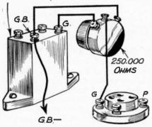
FIG. 100.—Overloading of the L.F. stage can be avoided by fitting a volume-control potentiometer, as shown here. justified. If it is not found necessary to apply a very high anode voltage to the detector valve, a resistancefed transformer is to be preferred, for this will provide greater amplification and better quality than an ordinary cheap transformer. On the other hand, a really highgrade transformer is hard to beat.
