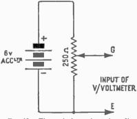
FIG. 49.—Theoretical circuit of the calibration apparatus.
