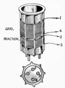
FIG. 92.—Details of an easily-made type of four-pin coil. Winding data is given in the text.
