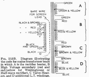
230 volts, and black and brown 250 volts. The screen someinterposed times between primary and secondary is generally a bare wire.For the secondaries red is employed for the high voltage, the centre tap being red and yellow. The rectifier heater is green, with green and yellow centre-tap, and for the heaters brown, with a brown and yellow centre-tap is
