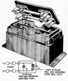
FIG. 104.—The Belling-Lee type 1171 interference suppressor and circuit.
