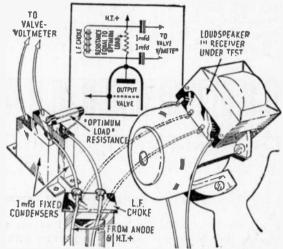
FIG. 59.—Disconnect the speaker from the set and substitute a resistance equal to the optimum load of the output valve in parallel with an L.F. choke,
