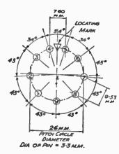
FIG. 219 .---- Valve-leg spacing for 9-pin valves.
