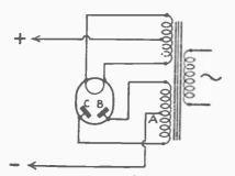
FIG. 147.—Any disconnection or poor contact between A and B or A and C will produce hum as the mains unit will be working as a halfwave rectifier. Test voltages between A and B and A and C with an A.C. voltmeter. Readings should be the same. identical. It should also be noted that abnormal hum may be due to the absence of an earth connection to the core of the transformer or of the smoothing choke, or to this connection making poor contact.
