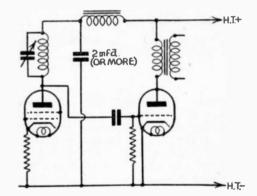
Fig. 154.—How the smoothing may be increased by including an L.F. choke.
