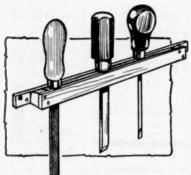
Fig. 199.—A handy rack for files, screwdrivers and chisels.
