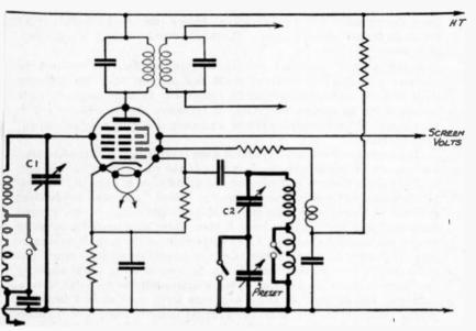
FIG. 181.—This skeleton diagram shows a superhet frequency-changer stage, with C1 and C2, the two-gang tuning condenser.
