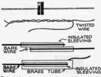
Fig. 118.—As a substitute for a broken condenser, one of the schemes shown above may be employed.
