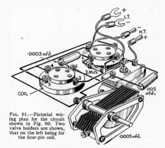
oscillator tuning condenser until a high-pitched whistle is heard in the speaker. This is obtained only when the set and oscillator are tuned to the same frequency, and consequently the four-pin coil must be of such a size that it is appropriate to the wavelength to which the set is tuned.
