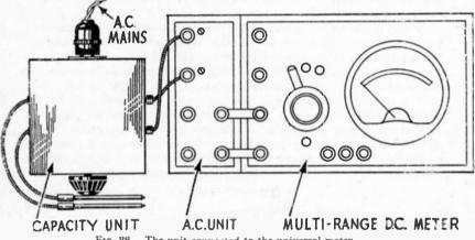
FIG. 38.-The unit connected to the universal meter.
