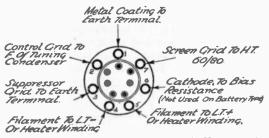
FIG. 85.-Standard connections for a 7-pin H.F. pentode.
