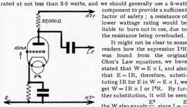
FIG. 214.-In order to determine the wattage rating of an anode resistance, it is necessary to know its resistance rating, and the current passing through it.
