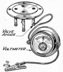
Fig. 162 .--- Showing a method of checking anode voltage.
