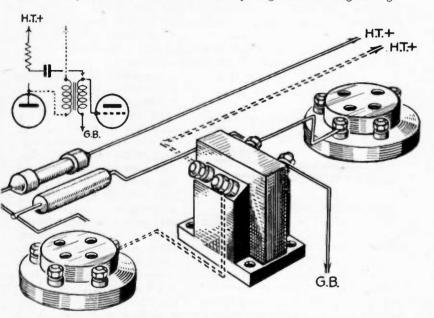
FIG. 117.—An L.F. transformer primary winding may break down. It may be replaced by a resistance and condenser coupling as shown.
