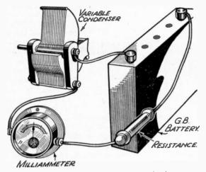
FIG. 157.-Testing a condenser for short circuits.
