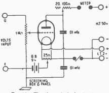
FIG. 46.—The theoretical circuit of the valve-voltmeter.
