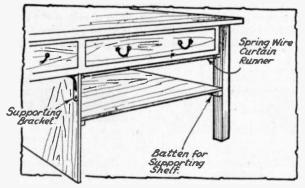
Fig. 200 .--- The " power-station " or battery compartment.
