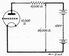
Fig. 212. A simple circuit which shows the relationship between current voltage and resistance.
