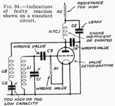
care should be taken not to reduce its value too much, as this will cause the amplification of the stage to be lowered. In such a case, the resistance should never be lowered in value to less than twice the impedance of the value.
