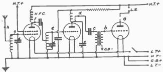
FIG. 20.—A simple three-valve battery circuit in its essentials. Touching the lettered points (beginning at *a*) in the order shown should result in "plops" being heard in the speaker if the circuit is in order.
