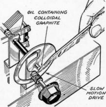
FIG. 187.—Using a feather for applying a little lubricant to the condenser bearing.
