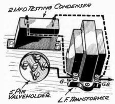
FIG. 167.-Localising hum by grid short-circuit method.
