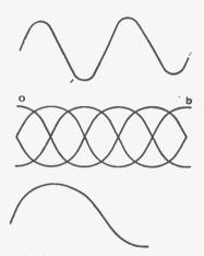
FIGS. 129, 130, and 131.—Screen traces of an alternating voltage waveform for different ratios of A.C. frequency to the time base "sweep" frequency. The traces are appropriate to ratios of 2/1, 5/4 and 1/1 respectively.
