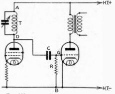
FIG. 153.-A standard tuned-anode circuit.
