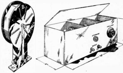
FIG. 54.—The type B coil and holder.
