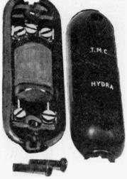
FIG. 110.—A flex lead suppressor (together with the circuit which is employed) from the Belling-Lee range.
