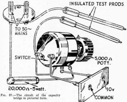
that is the measurement of capacity. For this purpose it is necessary that a source of A.C. is available and A.C. mains will usually be accessible to those readers who have constructed the rectifier unit. In this connection it is assumed that the mains to be used are 200-250 volts, 50 cycles, but any other voltage or periodicity can equally well be accommodated, by suitable modifications to the meter. Electrolytic condensers cannot be measured with this type of instrument, as it operates on A.C.
