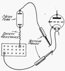
FIG. 76.—A general method for testing interelectrode insulation. types—4 and 5-pin, 7-pin, 9-pin, and side contact—with the neon lamp fitted behind a neat escutcheon, and a switching device to permit the various pairs of electrodes to be selected for testing.
