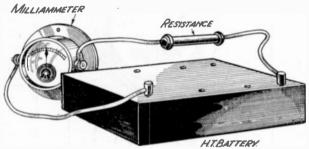
FIG. 159.-Checking the value of a fixed resistance.
