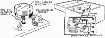
FIG. 26.—Fixing the 5,000 ohms variable resistance in position.
