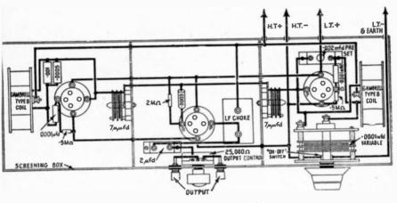
FIG. 56.—The wiring diagram of the L.F. oscillator.
