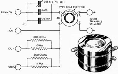
FIG. 32.—The theoretical circuit diagram of the A.C. unit.
