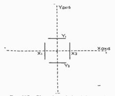
FIG. 125.—Plan view of the deflector plate arrangement to give horizontal, vertical, or resultant-deflection.
