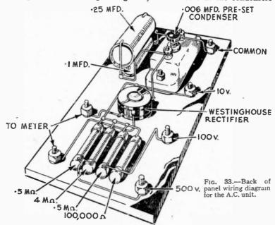
used are one of 0.25 mfd., one of 0.1 mfd., and a pre-set condenser with a maximum capacity of 0.006 mfd., this latter being included to enable a final adjustment to be made if it is possible to compare our meter with a meter of known accuracy. Should this not be possible, it will be found that this condenser should be screwed right home and then slacked off about one-quarter of a turn.
