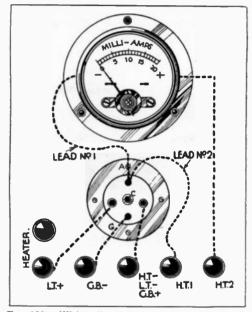
FIG. 160.-Wiring diagram of a simple valve tester.
