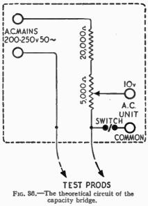
some instances a reduction of this resistance to a value of 3 or 2.5 megohms has been found to be necessary, though the reason for this is not readily apparent. Of course, care must be taken to disconnect the mains from the instrument while adjustments are made.
