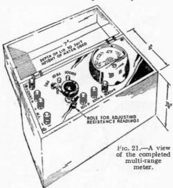
from clips the for adjustment. The procedure is as follows: connect the resistance we have just made to the clips, then decrease the variable resistance until the meter indicates 1 mA., open the switch and remove this resistance from the clips and replace it with 2 yards of No. 20 S.W.G. " Eureka " wire, switch on and the reading of the meter should be just about 0.1 mA. Now switch off and shorten the wire, testing inch by inch, taking care to switch off every time
