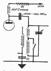
FIG. 174.—A modification of Fig. 64. It may be advisable to retain the resistance R1, and the condenser C1 to act as decoupling components.
