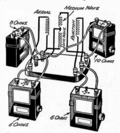
FIG. 169.—A combined theoretical and practical diagram showing the points between which a dual-range tuner with loose-coupled aerial winding should be tested with an ohm-meter, and the (very approximate) reading to be expected.
