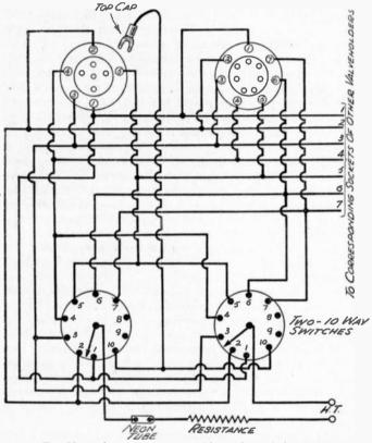
FIG. 77.-A layout tor a tester of inter-electrode insulation,
