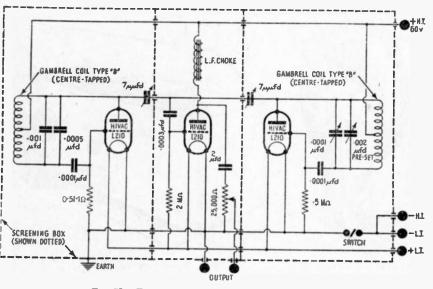
FIG. 53.-Theoretical diagram of the L.F. oscillator.
