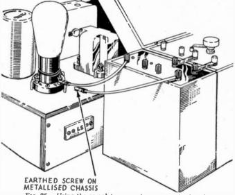
FIG. 35.-Using the complete apparatus as an output meter.
