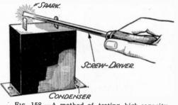
FIG. 158.—A method of testing high-capacity condensers.
