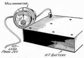
FIG. 161.—Checking total current consumption.
