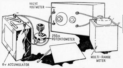
FIG. 50.—Adjusting the zero reading.
