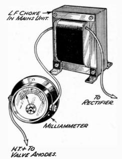
FIG. 165.—Measuring the total H.T. current consumption.
