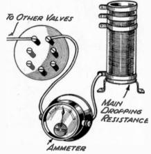
FIG. 164.-Measuring the heater current in A.C./D.C. receiver.
