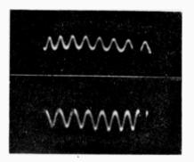
FIG. 139 (top).—The signal at the grid of a double-diode-triode. FIG. 140 (bottom).— The signal at the detector diode anode. The decrease of amplitude of Fig. 140, with respect to Fig. 139, is due to loss in the resistance-capacity network between diode and grid.
