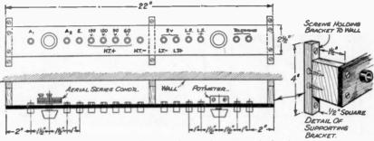
FIG. 201.-The lay-out of the universal terminal strip.
