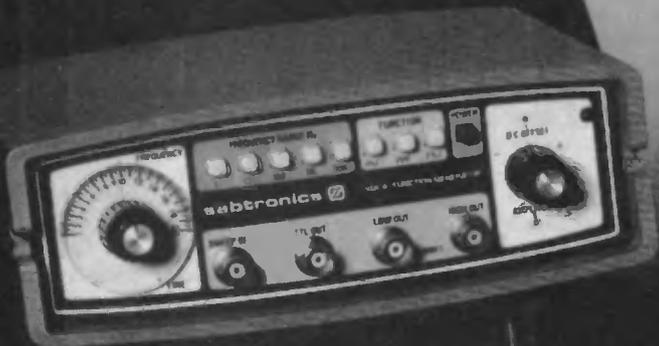
5020A 1Hz to 200kHz function generator
