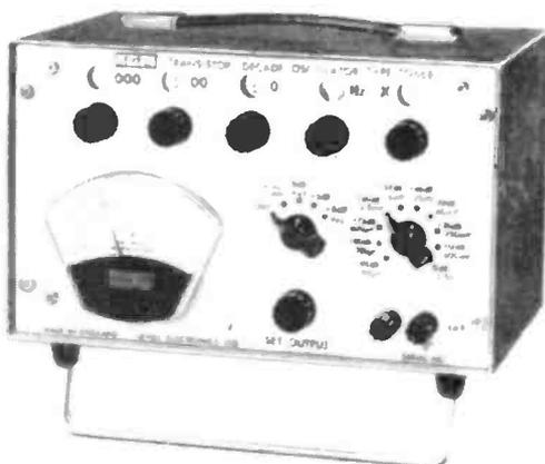
**FREQUENCY** 0.2Hz to 1.22MHz on four decade controls.
