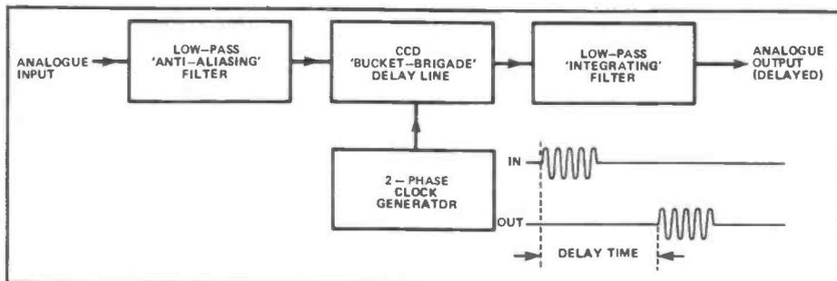
Figure 3: Block diagram of a basic analogue delay line system.
