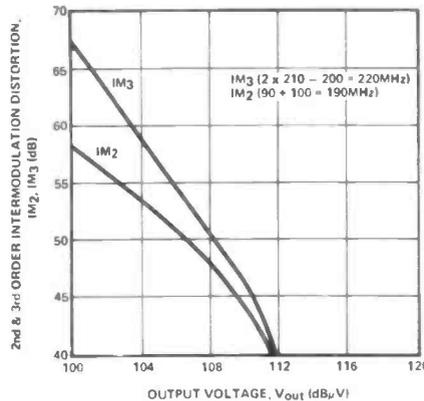
Typical 2nd & 3rd order intermodulation distortion at V<sub>CC</sub> = +17V. masthead pre-amp).
