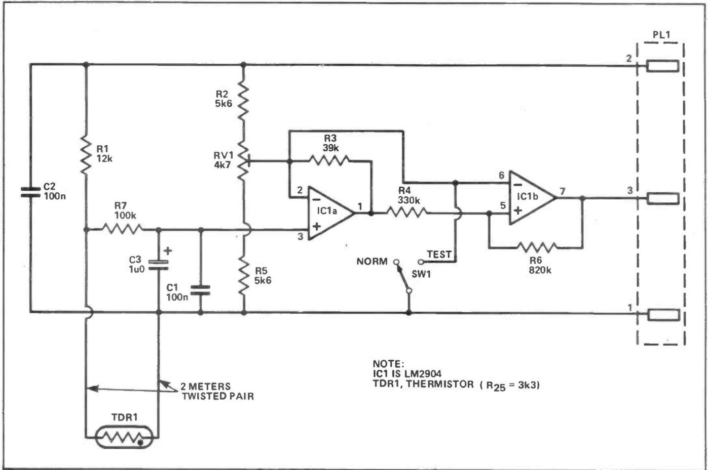
Figure 6: The Circuit Diagram of the Remote Ice Warning System.
