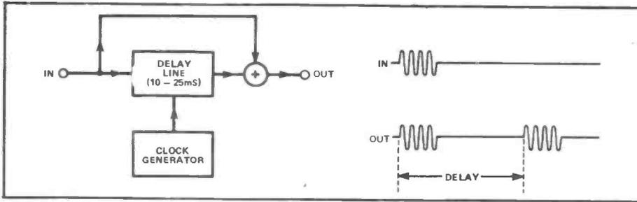
Figure 5: Double-tracking circuit.
