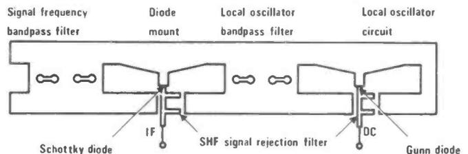
Figure 2: Details of a 12GHz converter with planar circuit.
