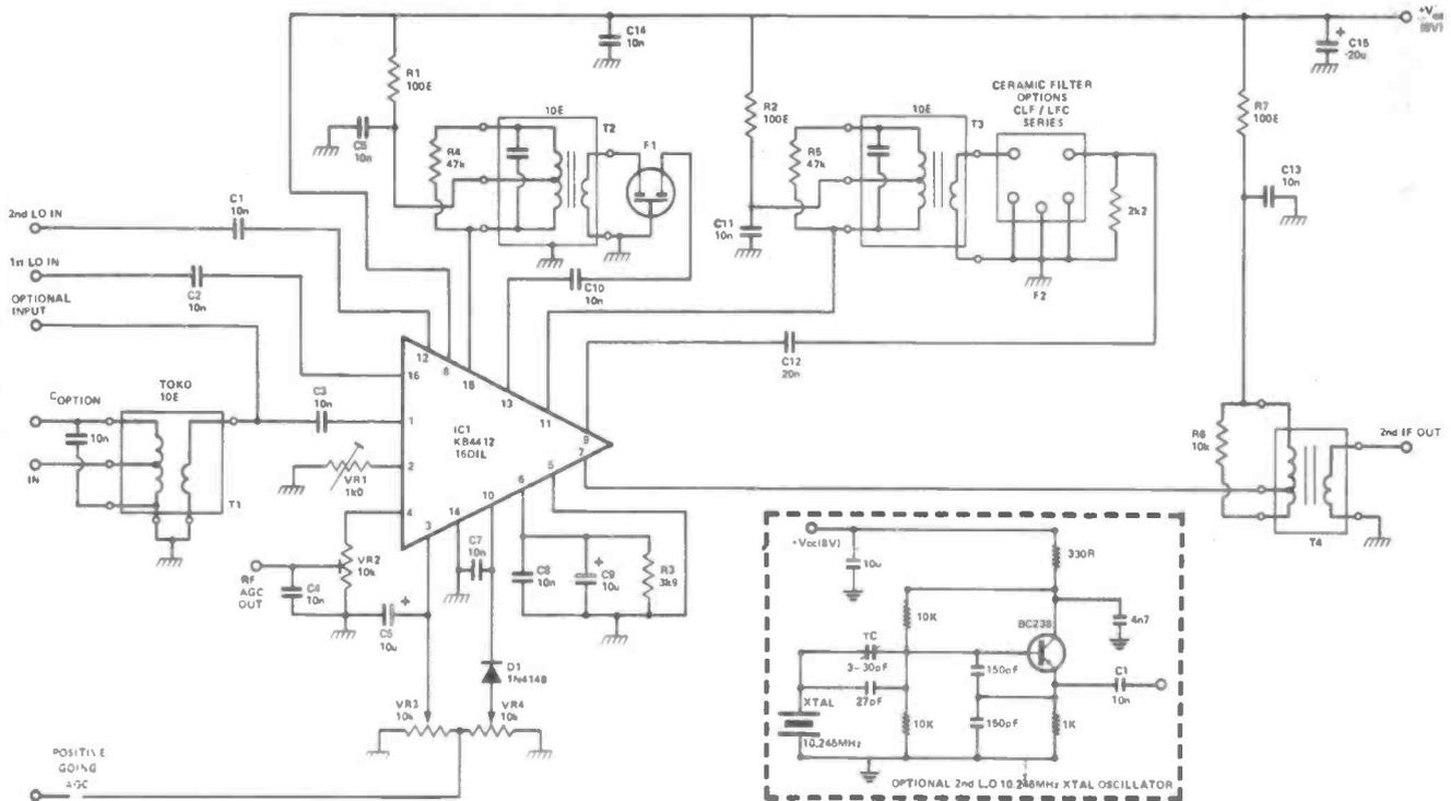
Application with dual conversion - inputs up to 40MHz can be used. Use the KB4412 detector system (see last month's databrief) for a complete AM/SSB system for LF/HF
