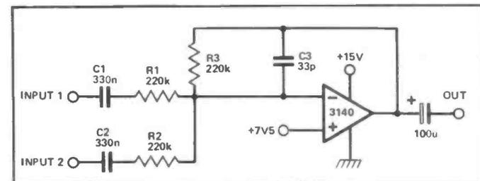
Figure 24: Combined 2-input mixer/1st-order low-pass filter.
