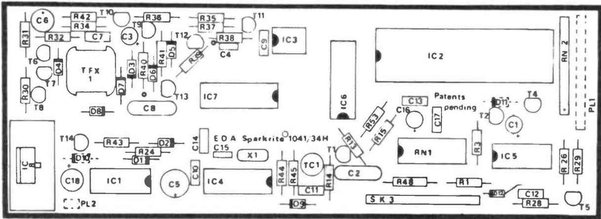
Figure 3: (Above) Shows the main board's component overlay.
