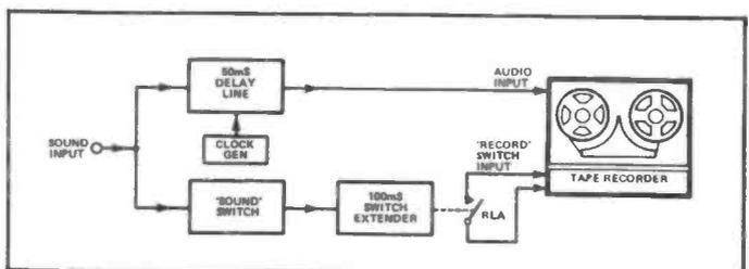
Figure 14: Automatic Tape Recorder with 'predictive' switching.
