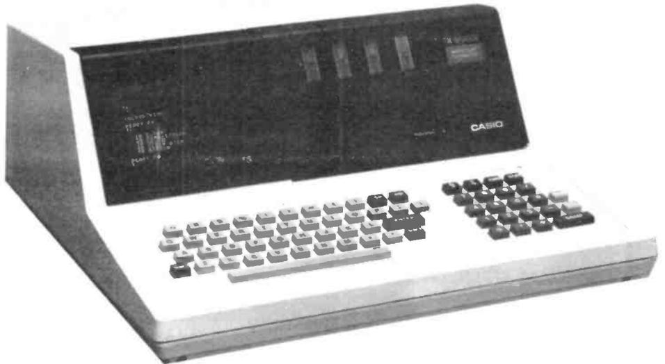
A separate keyboard is used for numeric entries and has associated with it special function keys such as COMP - to allow direct calculations without the need for PRINT statements — and STAT — to facilitate the use of the FX-9000P's repertoire of statistical routines.
