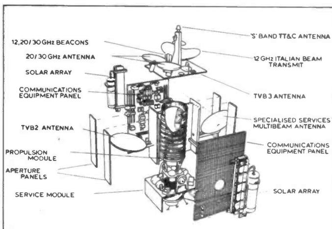
Figure 5: L-SAT 1 configuration.
