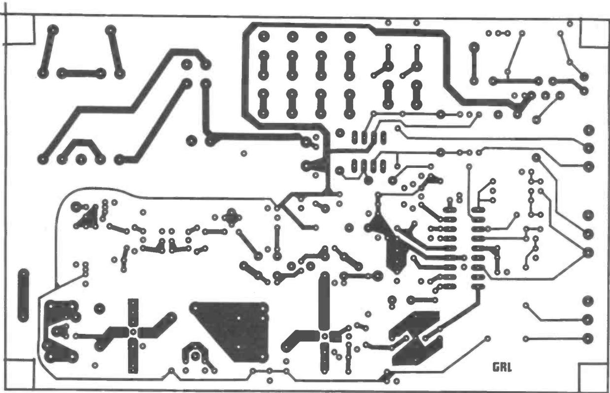
Figure 3: PCB Foil Pattern, Track Side.
