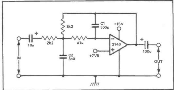
Figure 22: 25 kHz 2nd-order maximally-flat low-pass filter.
