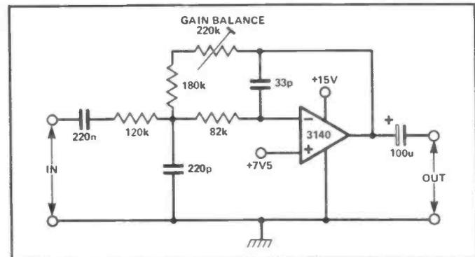
Figure 23: Adjustable-gain 2nd-order low-pass output filter.
