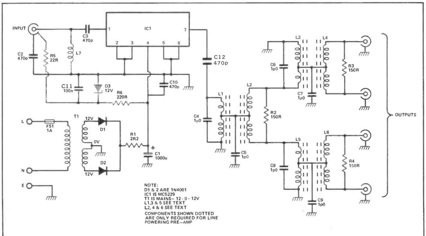
Figure 1: The complete circuit diagram, components shown dotted are only required if the unit is used in conjunction with the R&EW Masthead Amp.
