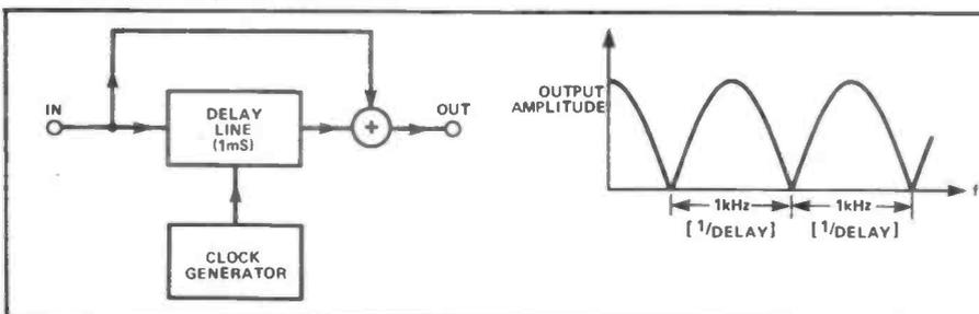
Figure 8: CCD comb filter. Notches are about 20-30 dB deep, 1 kHz apart.
