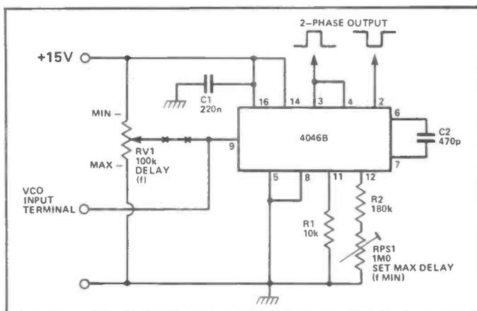
Figure 20: High-performance voltage-controlled 2-phase CMOS clock generator.
