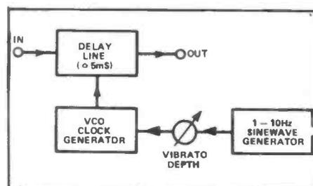
Figure 4: True vibrato circuit, which applies slow frequency modulation to all input signals.
