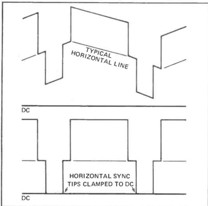
Figure 7a: (TOP) Video demodulator output showing video riding on energy dispersal wave;
