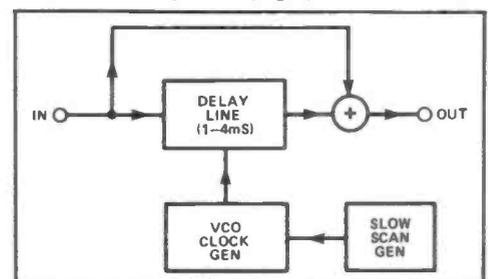
Figure 9: A Phaser is a variable comb filter, in which the notches are slowly swept up and down the audio band.
