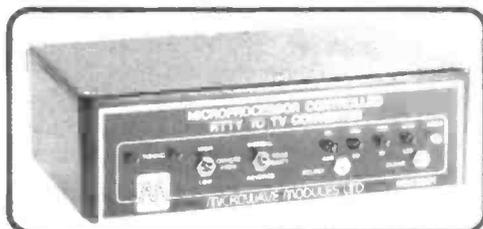
This converter, MM2001, contains a terminal unit, and a microprocessor controlled TV interface, and requires only an audio input from a receiver and a 12 Volt DC supply to enable a live display of "off-air" RTTY and ASCII on a standard domestic UHF TV set. The display format is 16 lines of text, each 64 characters wide.
