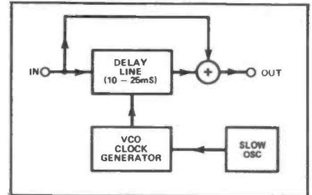
Figure 6: Auto-Double-Tracking (ADT) or mini-chorus circuit.
