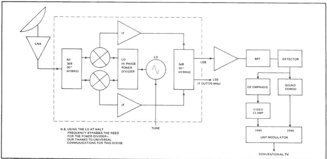
Figure 4: Use of an image rejection mixer for single conversion techniques.
