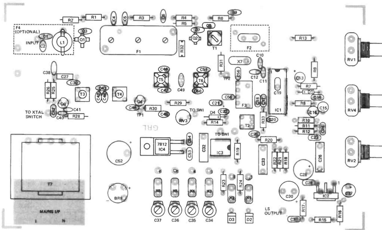
Figure 5: Component Overlay.
