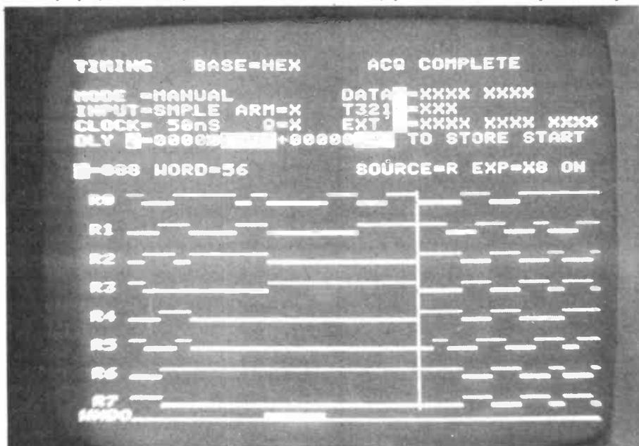
Photo 2: The window section of photo 1 expanded 8 times. Note the on-screen cursor, the display of the cursor location, and the its location value.
