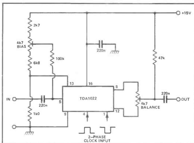
Figure 17: Delay line using the TDA1022.
