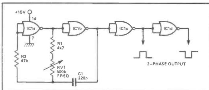
Figure 19: Variable-frequency general-purpose 2-phase CMOS clock generator.
