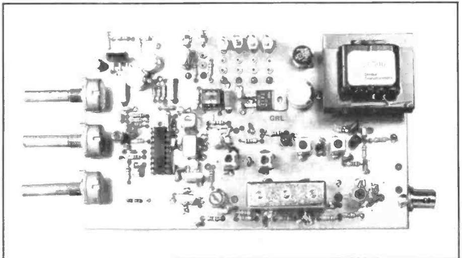
Figure 1: Prototype UOSAT Receiver PCB.
