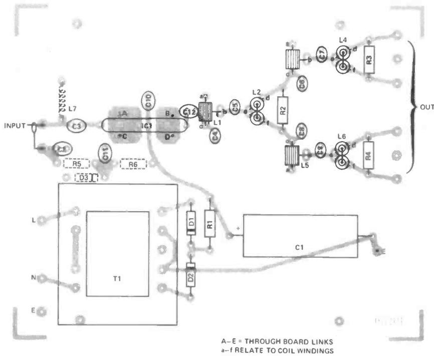
Figure 2: Component overlay of the distribution amplifier.
