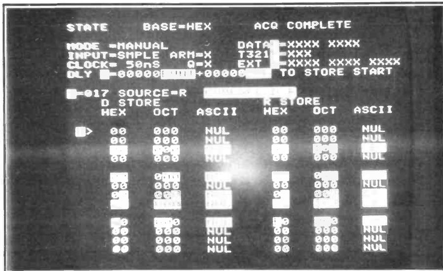
Photo 5: The compare mode, showing inequalities between the reference and data memory in inverse video.
