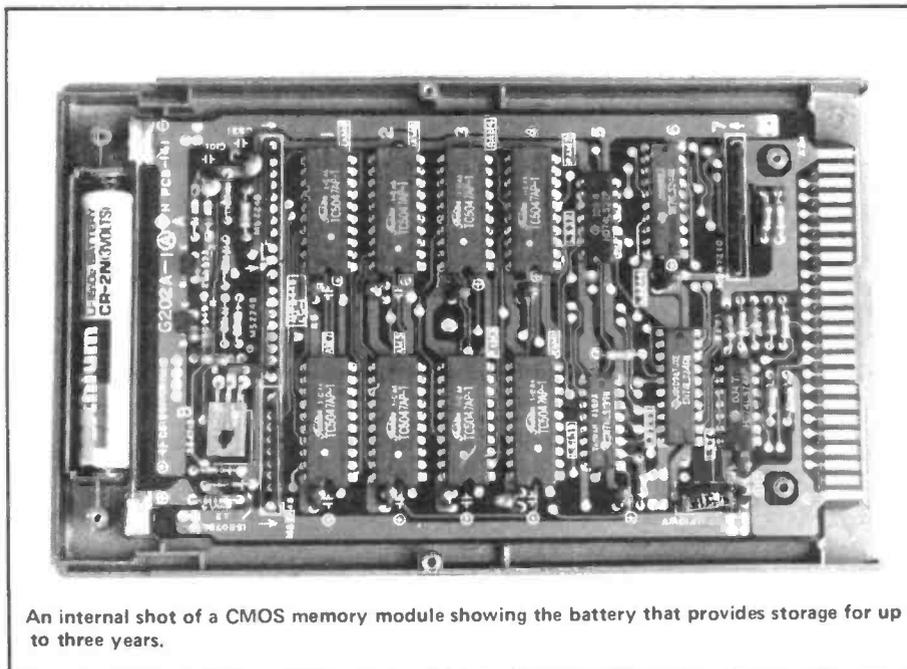
An internal shot of a CMOS memory module showing the battery that provides storage for up to three years.
