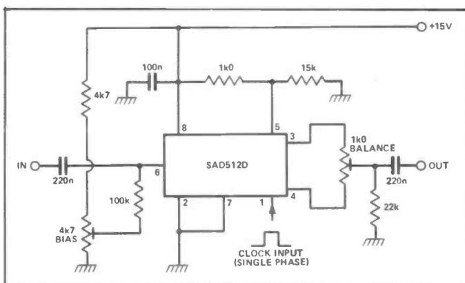
Figure 18: Delay line using the SAD512D
