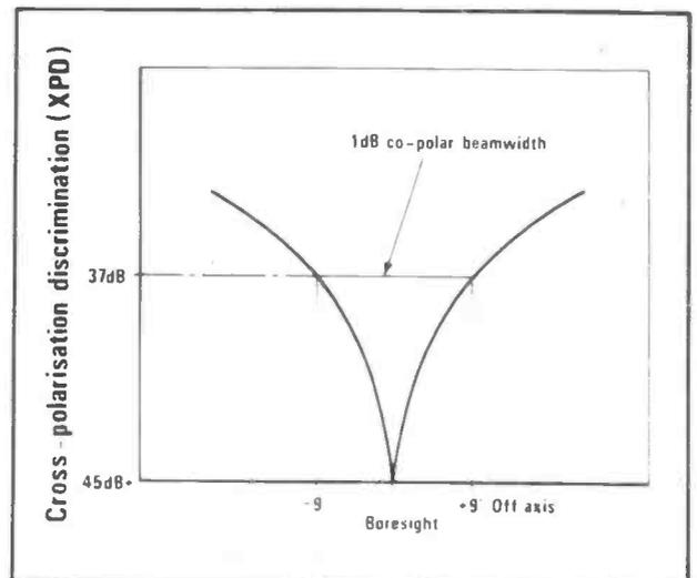
Figure 6: The polarisation discrimination of a satellite receiving aerial decreases rapidly away from its centre boresight direction.
