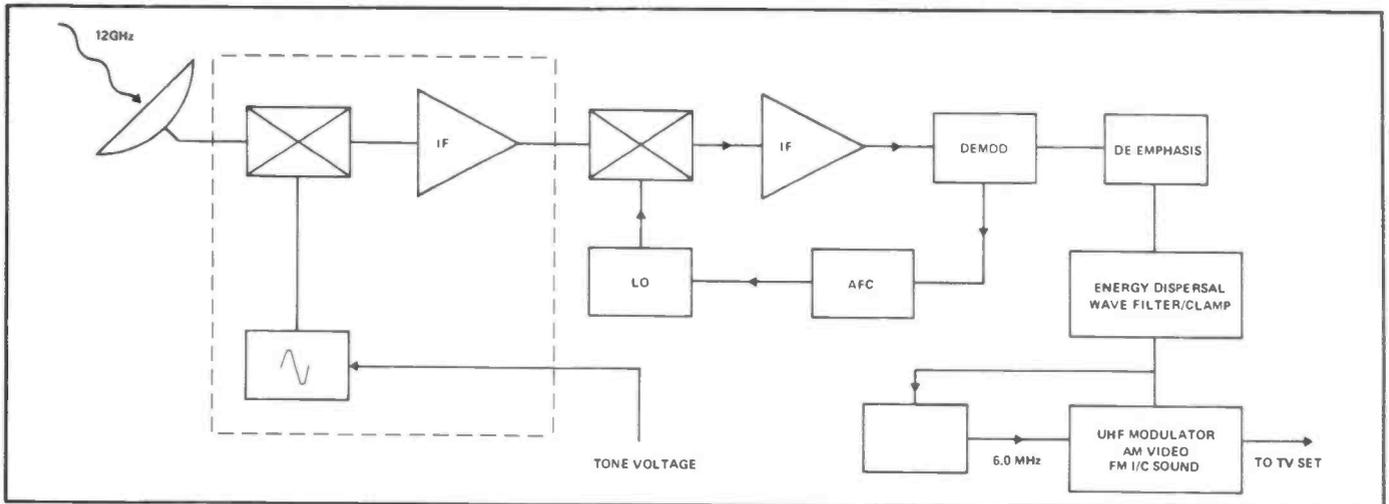
Figure 3: Block diagram of a conventional satellite receiver.
