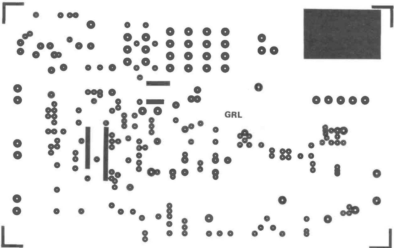
Figure 4: PCB Foil Pattern, Component Side.
