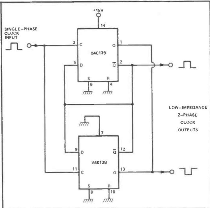
Figure 21: Single-phase to 2-phase converter, with low impedance output.
