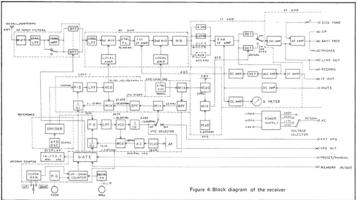
Figure 4: Block diagram of the receiver
