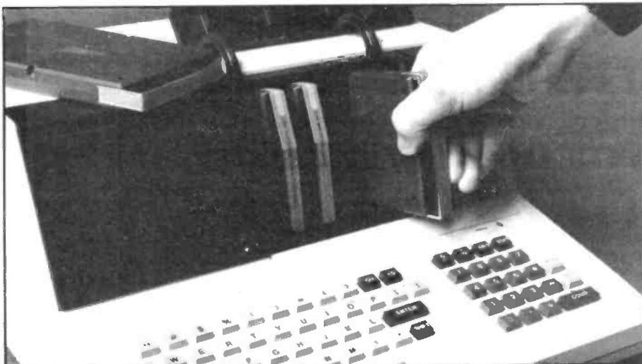
The hinged flap of the FX9000 is raised to allow access to the expansion modules.
