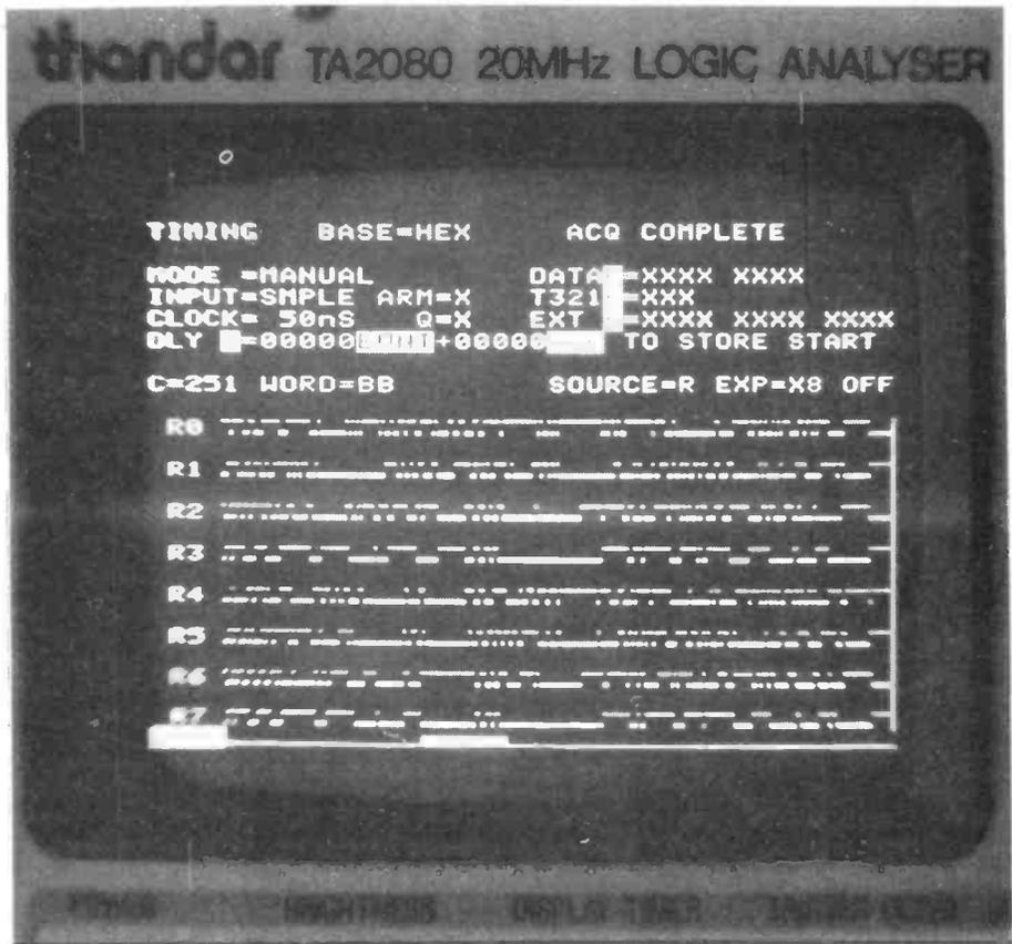
Photo 1: The analyser in the timing mode
