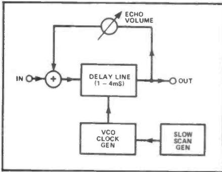
Figure 10: A flanger is a phaser with accentuated and variable notch depth.
