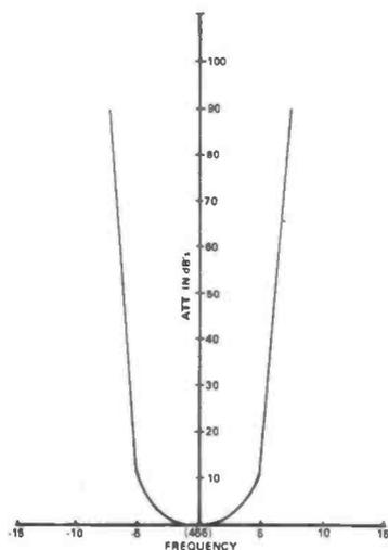
Figure 5 : Response of a |445KHZ ceramic ladder filter
