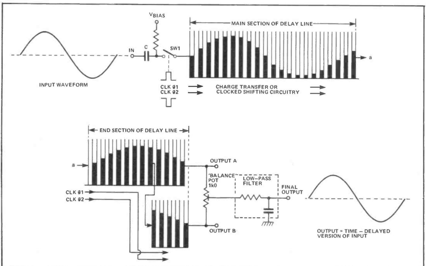
Figure 1: Basic operating principle of the 'Bucket Brigade' delay line. See text for explanation.
