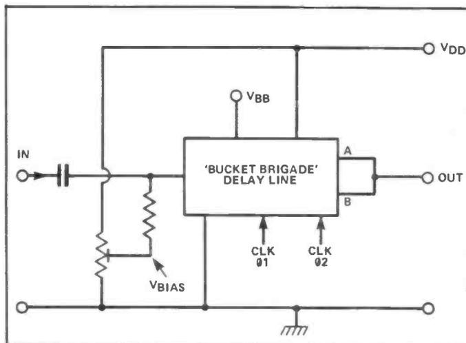
Figure 2: Essential 'usage' elements of an analogue delay line chip.
