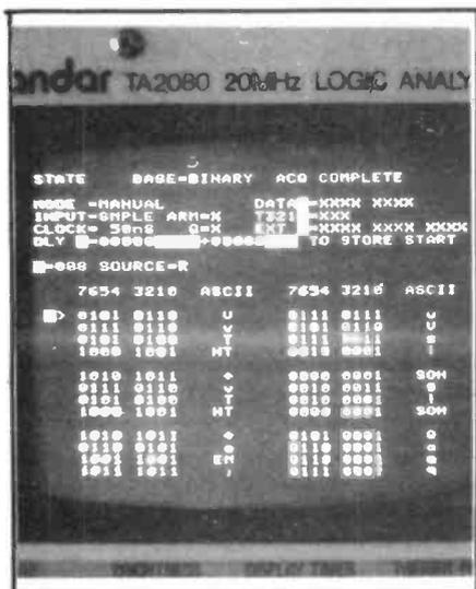
Photo 3: The analyser in the state mode - binary base.
