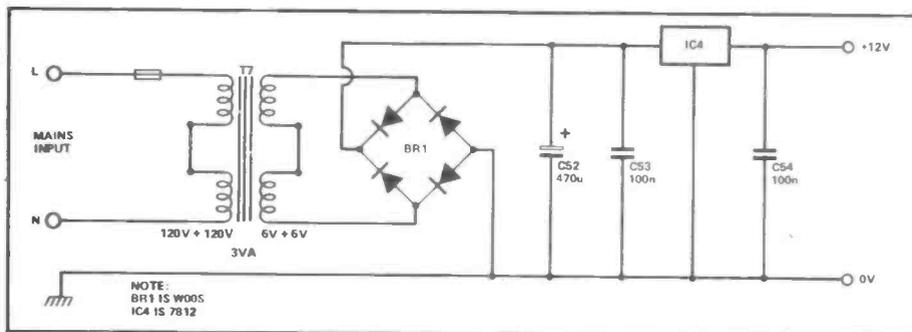
Figure 6: Power Supply Circuit Diagram.
