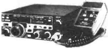
10W RF output on SSB, CW and FM. Standard and non-standard repeater shifts. 5 memories and priority channel shifts. Memory scan and band scan, controlled at front panel or microphone. Two VFO's LED S-meter 25KHz and 1KHz on FM. 1KHz and 100KHz tuning steps on SSB. Instant listen input for repeaters.
