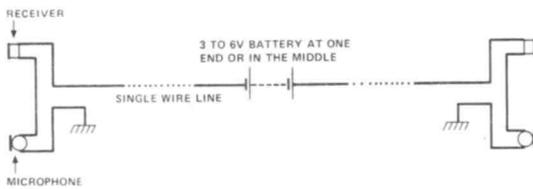
Figure 1(a): Simple series circuit. This is the simplest speech transmission arrangement. The transmission line is unbalanced and therefore prone to interference, crosstalk, 50Hz hum pick-up and earth potential differences.
