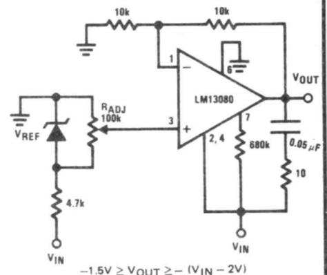
Figure 8: Negative Variable Voltage Regulator.
