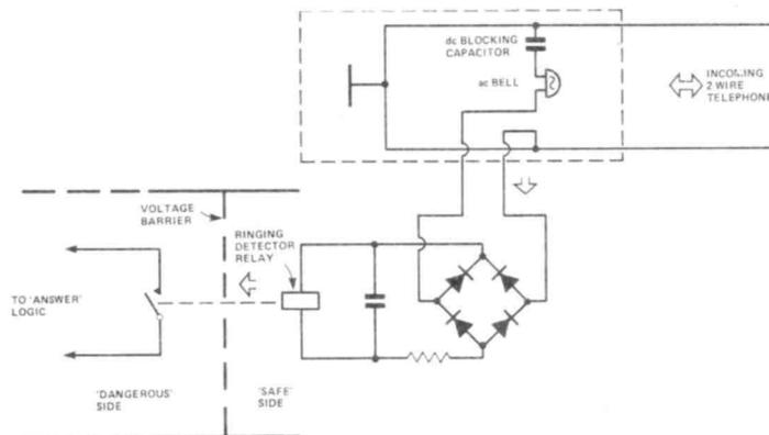
**Figure 7(a):** Ringing detector circuit. The relay operates to the rectified ringing current. The relay contact can then be used to initiate the automatic all answering sequence.
