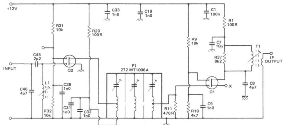
**Figure 3: Circuit for the RF and mixer stages.**
