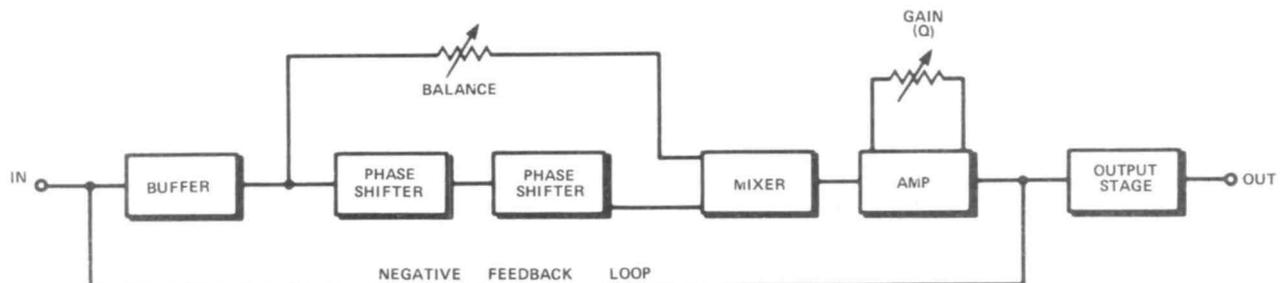
Figure 3: Block diagram of a typical notch filter.
