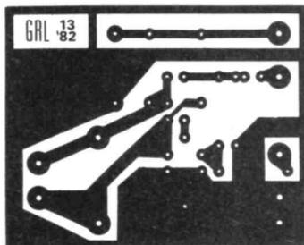
Figure 2: PCB foil pattern
