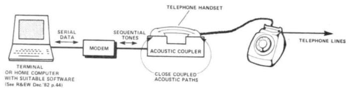
**Figure 3(b): When an acoustic coupler is employed the call is set up under 'user control'. There is then no need for the line controlling interface section, with relay control lines. A good reliable acoustic link is essential to reduce the problems of extraneous room noise and spontaneous variations in the overall channel attenuation.**
