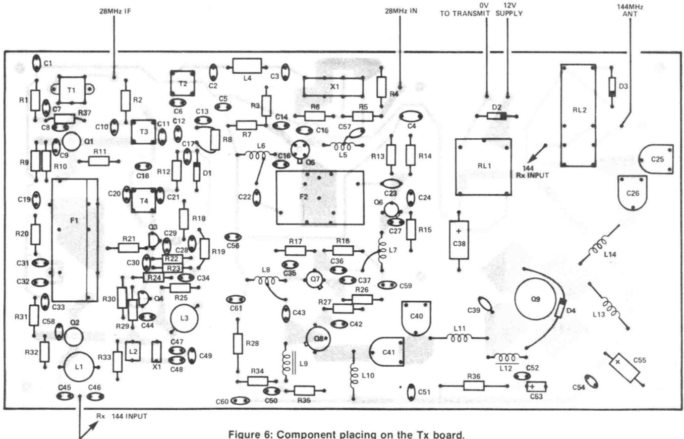
Figure 6: Component placing on the Tx board.
