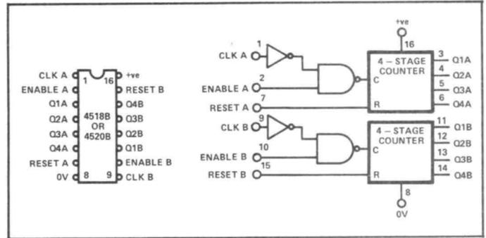
**Figure 14:** Outline and functional diagrams of the 4518B (decade) and 4520B (binary) dual counters.
