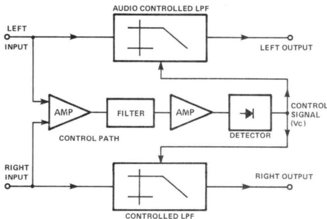
Figure 3: Block diagram of essential components in the DNR system.
