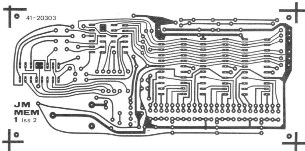
Figure 4: PCB track side.
