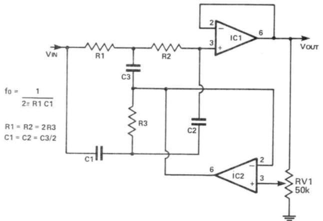
Figure 2: Practical circuit of a notch filter with adjustable Q.
