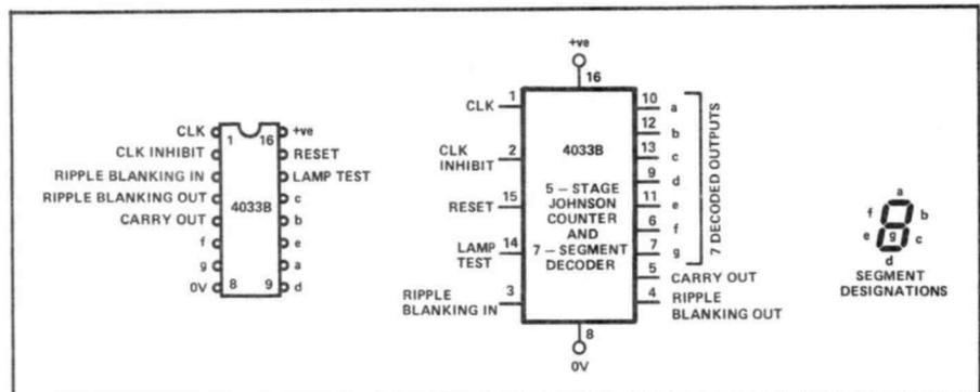
Figure 11: Outline and functional diagram of the 4033B decade counter with 7-segment display driver and RIPPLE BLANKING facility.
