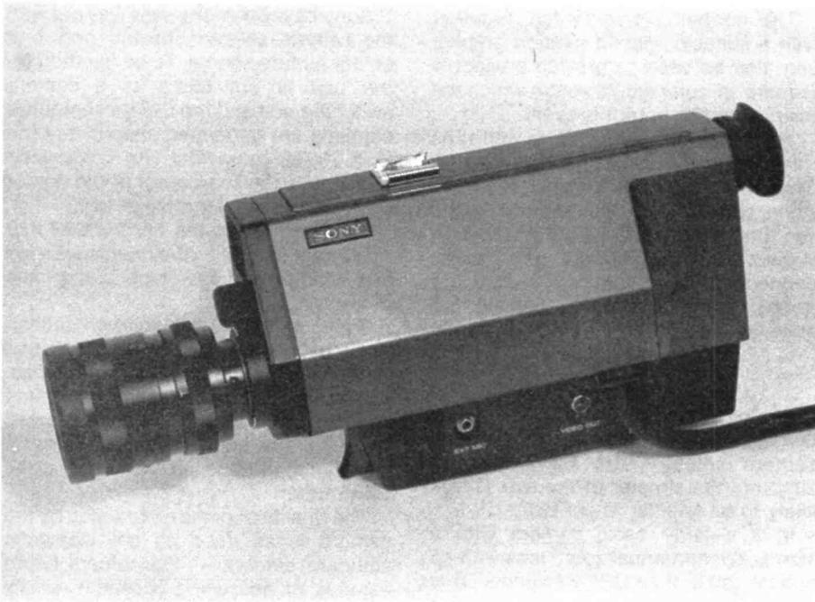
**Figure 2:**The HVM — 100CE is a B&W camera that is capable of being locked to an external sync. source.
