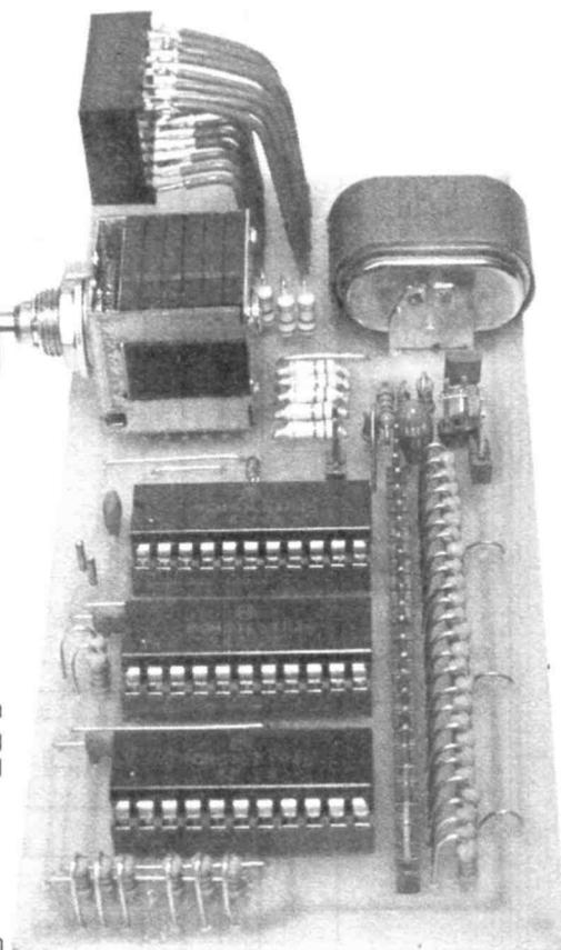
cell selection is achieved via a low-cost 40-way switch, originally destined for use in CB rigs. The switch also provides decoding for driving two 7-segment displays to indicate channels 1-40. Thus, with address lines A6 and A7 at low(0v), 40 locations are available and by selecting a combination of A6 and A7 high (6V), this is increased to 160. Locations 41-160 can be coded using two additional LED's to indicate when A6 and A7 are active.
