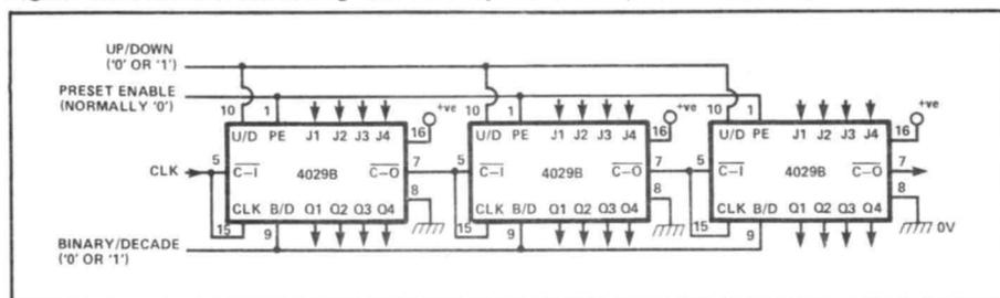
**Figure 20:** Method of cascading 4029Bs for asynchronous 'ripple' clocking.
