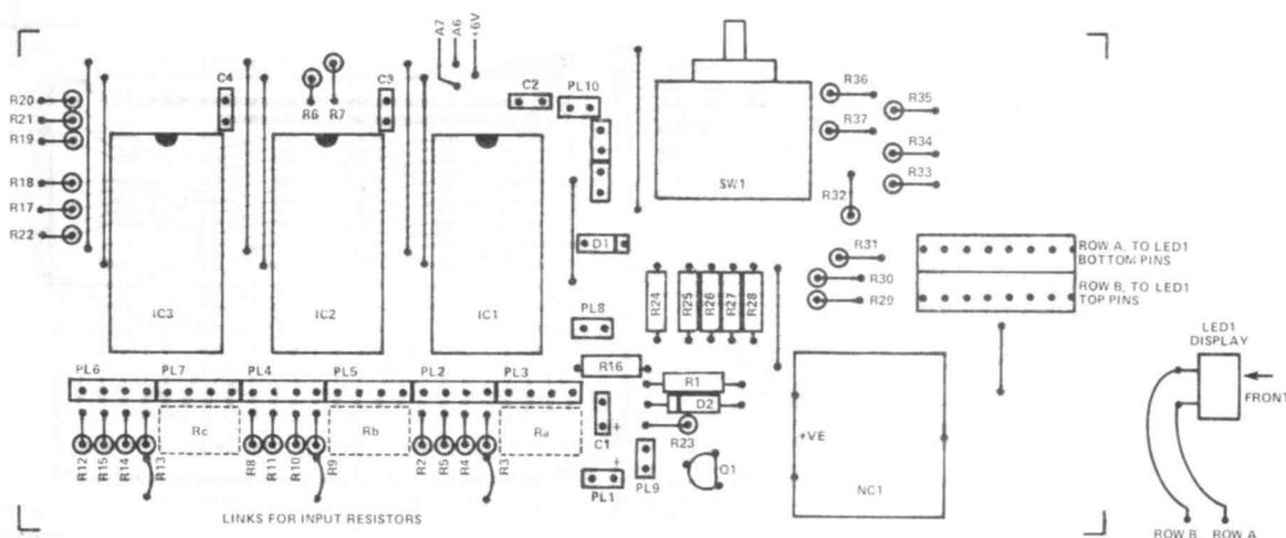
Figure 5: PCB component overlay.
