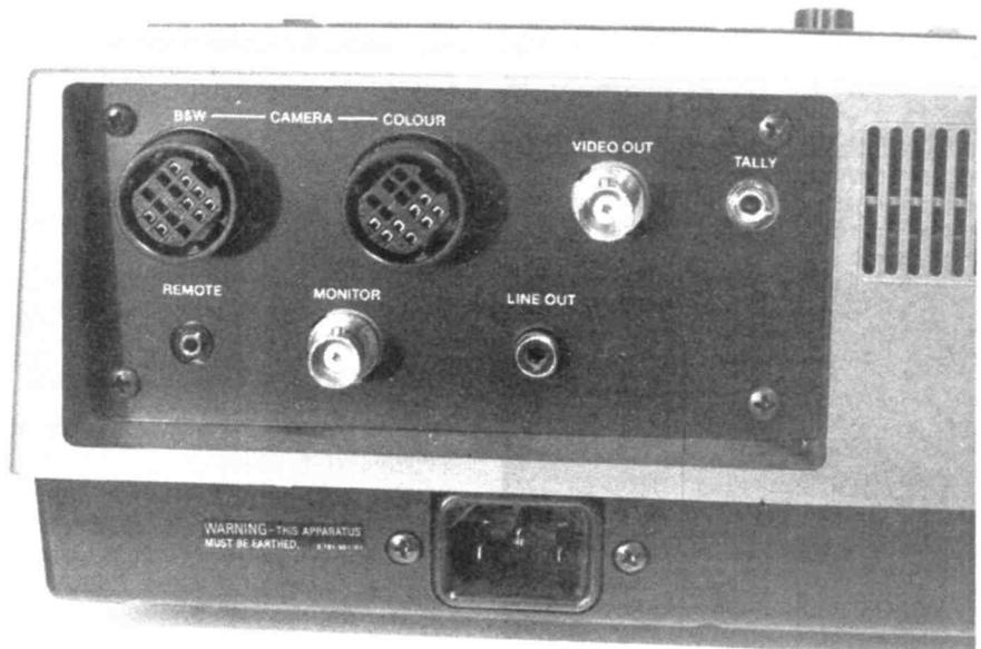
**Figure 3:**The rear panel of the camera selector provides all the video and audio in/out connectors. The Sony K type camera selectors provide all camera connections in one handy plug.
