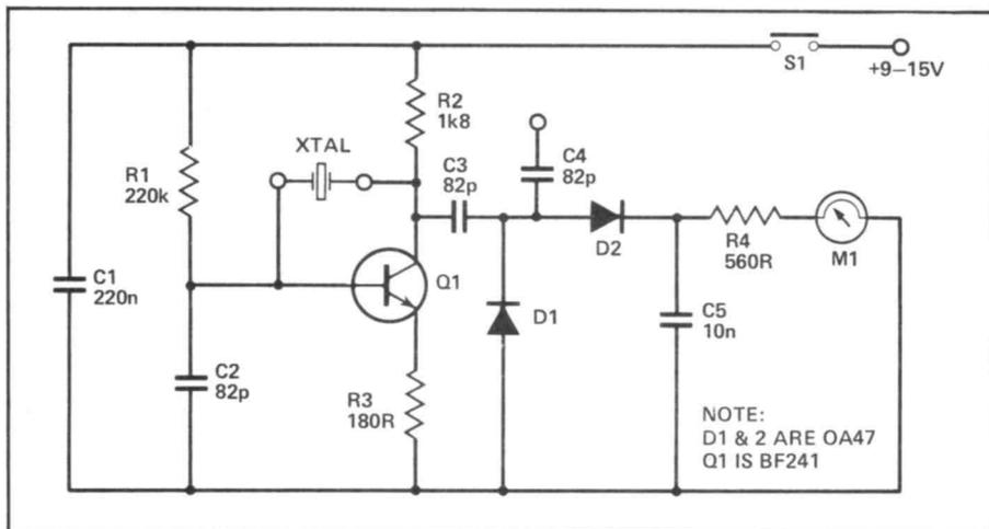
Figure 1: Circuit of the crystal tester.
