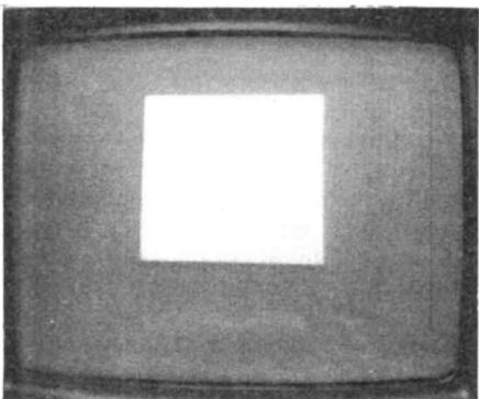
Figure 6: The B&W camera is focused on the caption graphic — in this case a white rectangle on a black background.
