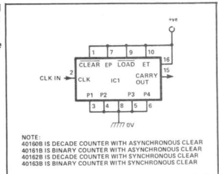
**Figure 17:** Method of connecting the 40160B to 40163B range of ICs for 'normal' counter operation.
