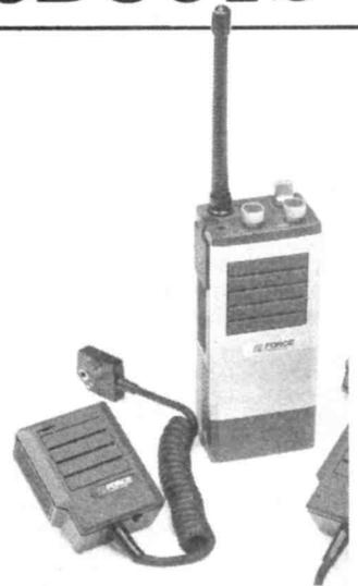
and a vehicle conversion charger which enables the portable to be used as a mobile unit. The vehicle charger is supplied complete with a mobile microphone, external speaker, mounting hardware and antenna connector.
