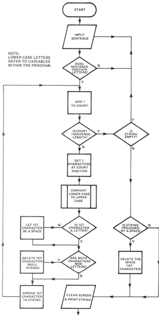
Figure 3: Flowchart for the sentence processing routine.
