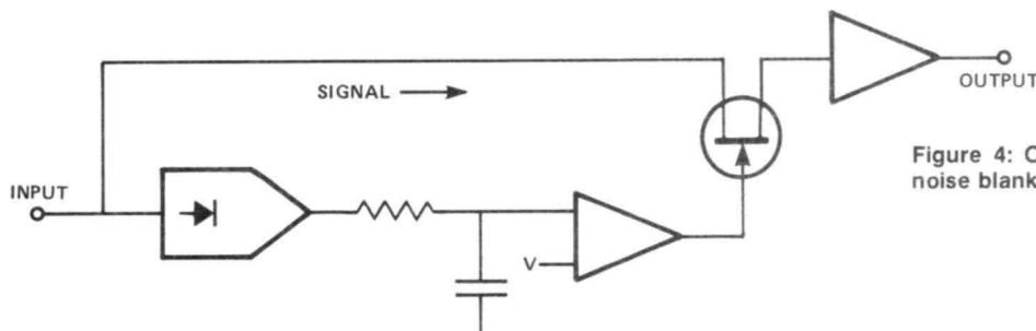
Figure 4: Operating principle of a noise blanking circuit.
