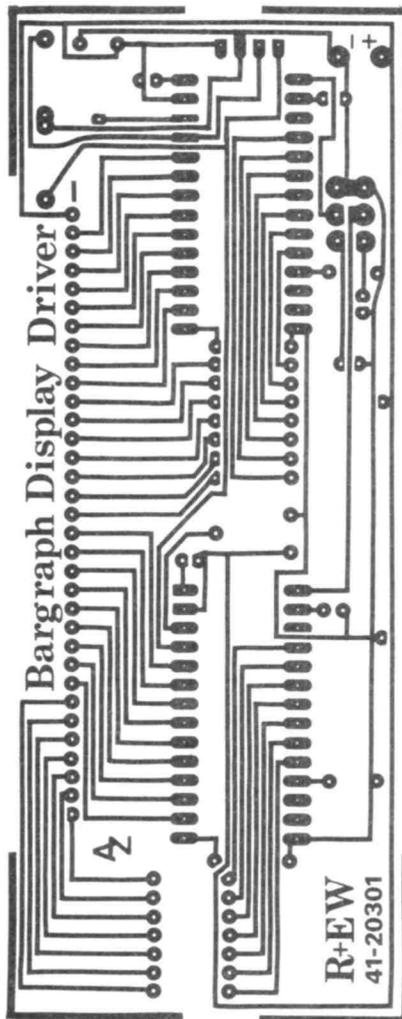
PCB foil pattern for Bargraph Display Board
