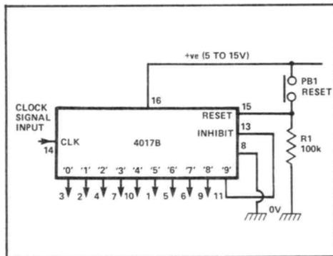
**Figure 7:** Method of connecting the 4017B for sequence-and-stop action.
