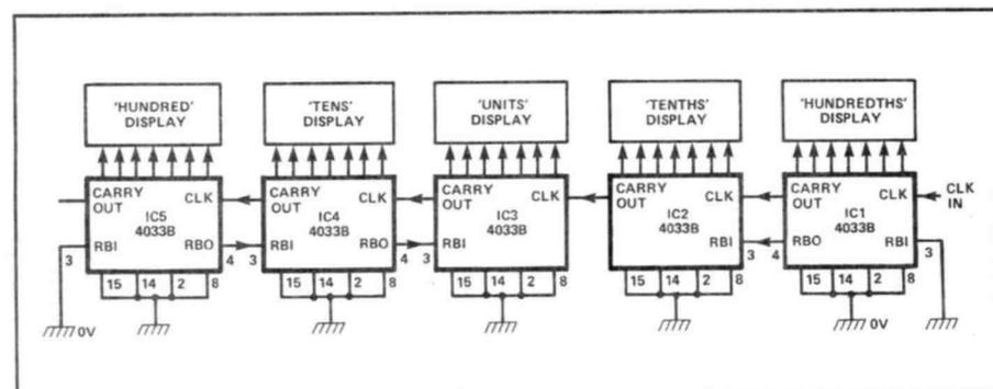
Figure 13: Method of connecting the RBI (RIPPLE BLANKING IN) and RBO (RIPPLE BLANKING OUT) of the 4033B to give leading and trailing zero suppression in a multi-decade display so that, for example, the count '009-90' is displayed as '9-9'.
