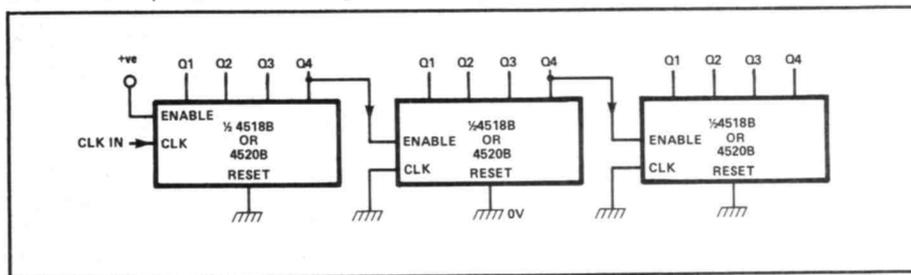
**Figure 15:** Methods of cascading 4518B or 4520B counters for ripple operation.
