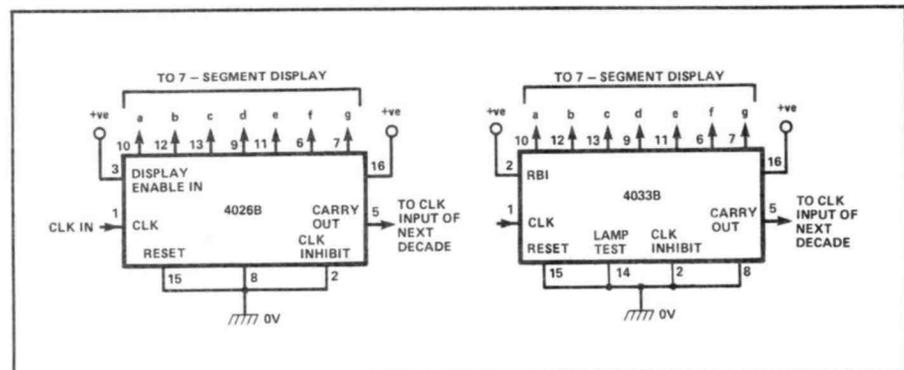
Figure 12: Methods of connecting the 4026B and 4033B for normal decade dividing/display operation. In the case of the 4033B, the RBI connection does not give suppression of display zeros.
