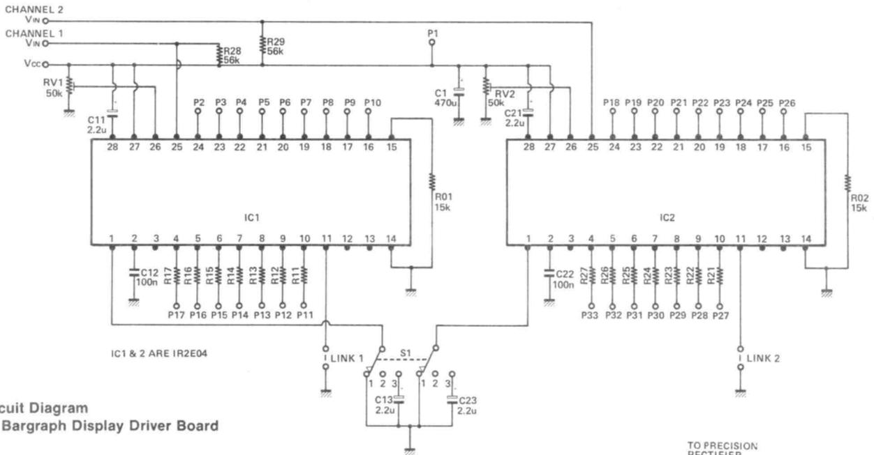
Circuit Diagram for Bargraph Display Driver Board
