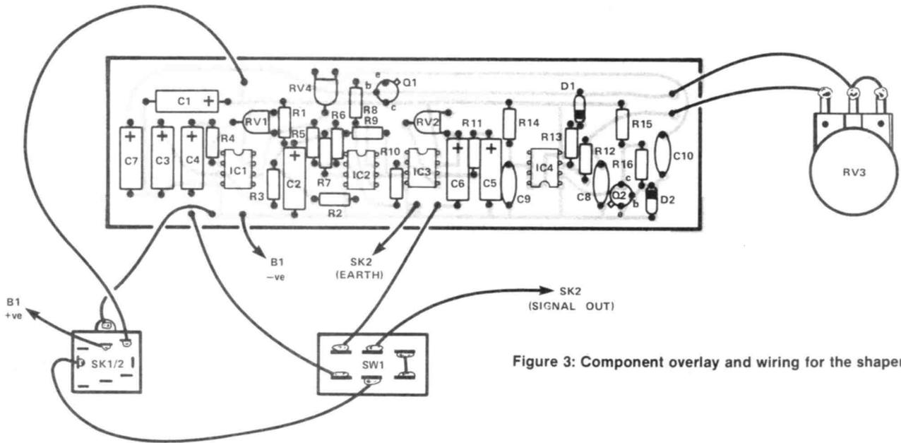
Figure 3: Component overlay and wiring for the shaper.
