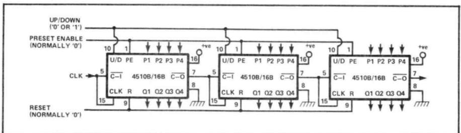
**Figure 24: Method of cascading 4510B or 4516B ICs for asynchronous 'ripple' clocking.**
