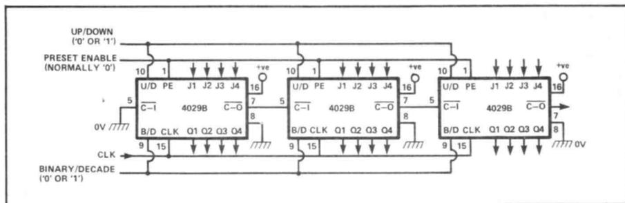
**Figure 19:** Method of cascading 4029Bs for synchronous 'parallel' clocking.
