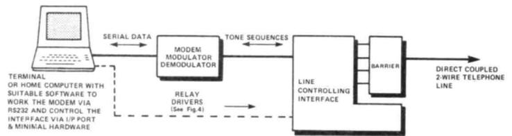
**Figure 3(a): Disposition of the Modem, Interface and Barrier. The Barrier section is essential for direct ('hard-wired') connections.**
