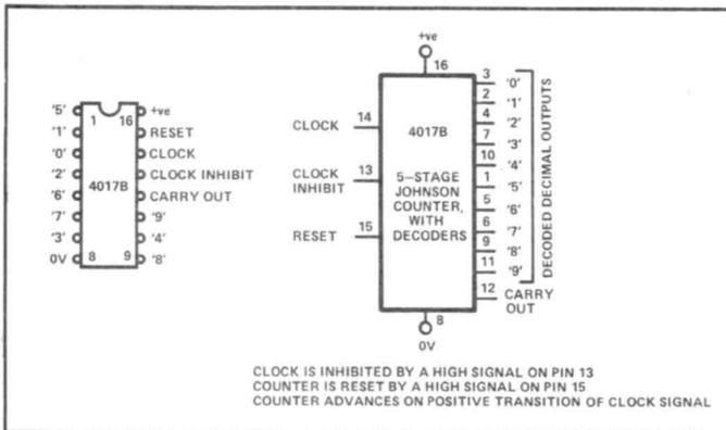
Figure 1: Outline and functional diagram of the 4017B Decade counter.
