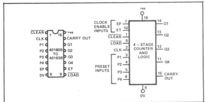
**Figure 16:** Outline and functional diagrams of the 40160B to 40163B range of programmable 4-bit counters.
