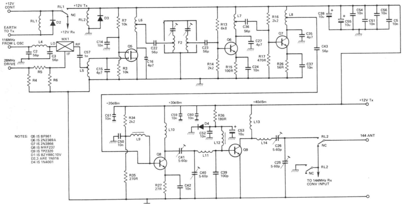
Figure 1: Circuit of the Tx mixer and output stages.
