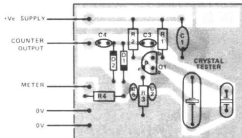
Figure 3: Component placing and wiring for the tester.
