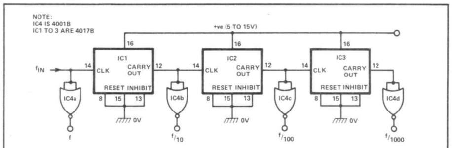
Figure 4: Any number of 4017B's can be cascaded to make a multi-decade divider. If the outputs are externally loaded, they should be buffered, as shown here.
