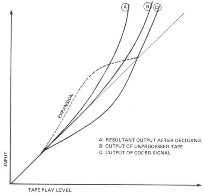
Figure 8: Non-ideal record/playback characteristics.
