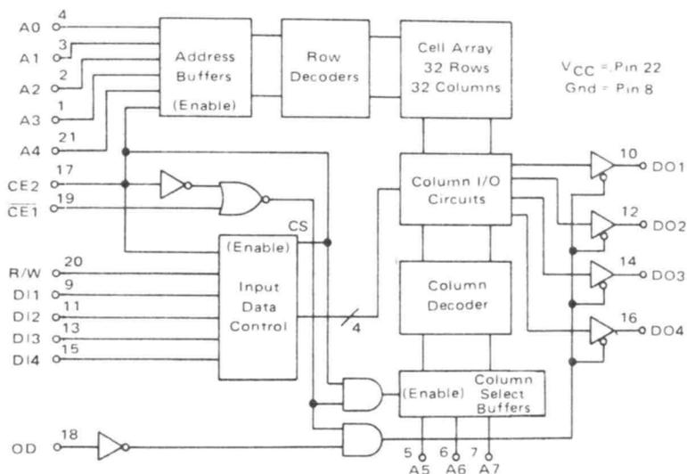
Figure 1: Block Diagram of 51L01
