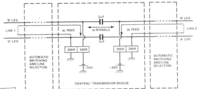
Figure 1(c): The standard form of the transmission 'bridge' uses relays for the inductors. Each relay has two windings so as to maintain AC balance and the two telephone lines are separated by capacitors so that the relays can monitor each line separately.
