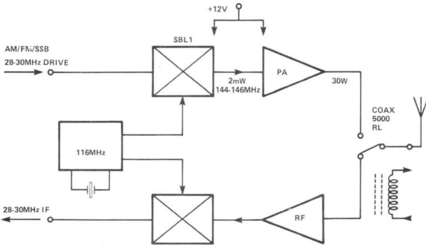
**Figure 2: Block diagram of the Transverter.**
