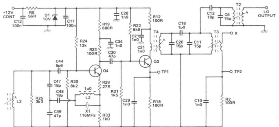
**Figure 4: Oscillator and Buffer circuit.**
