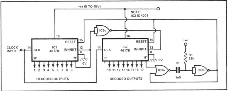
**Figure 8:** A 10- to 17-stage counter/decoder, set for divide-by-17 operation.
