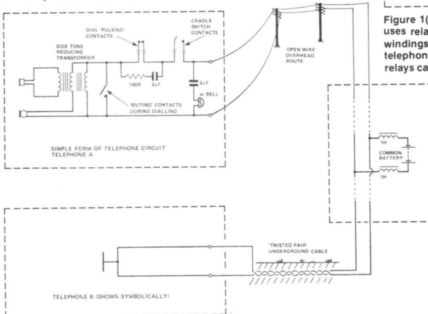
Figure 1(b): A more practical arrangement for energising the lines from the central telephone exchange.
