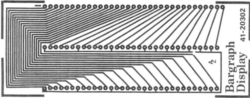
PCB foil pattern for Bargraph Display Driver Board
