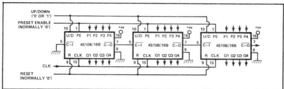
**Figure 23: Method of cascading 4510B or 4516B ICs for synchronous 'parallel' clocking.**
