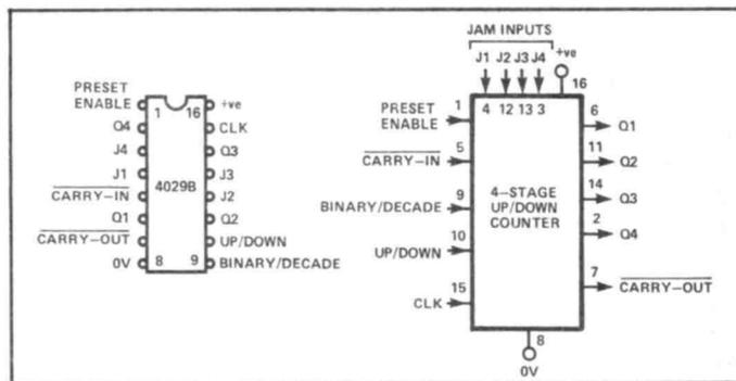
**Figure 18:** Outline and functional diagram of the 4029B presettable UP/DOWN counter.
