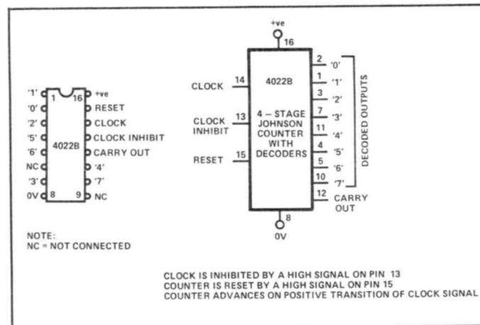
**Figure 9:** Outline and functional diagram of the 4022B Octal counter.
