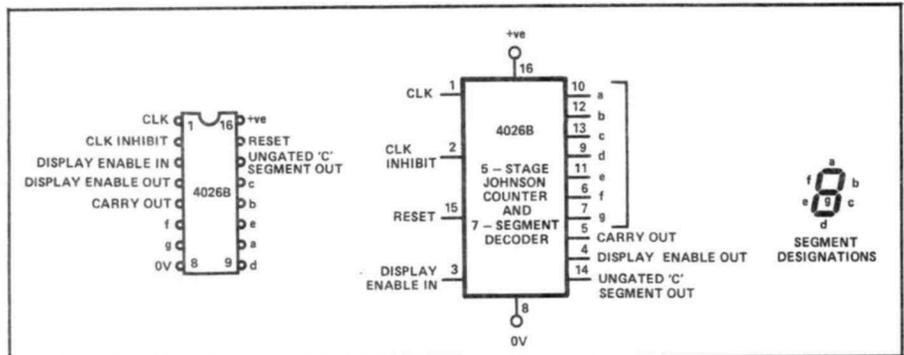
Figure 10: Outline and functional diagram of the 4026B decade counter with 7-segment display driver and DISPLAY ENABLE control.
