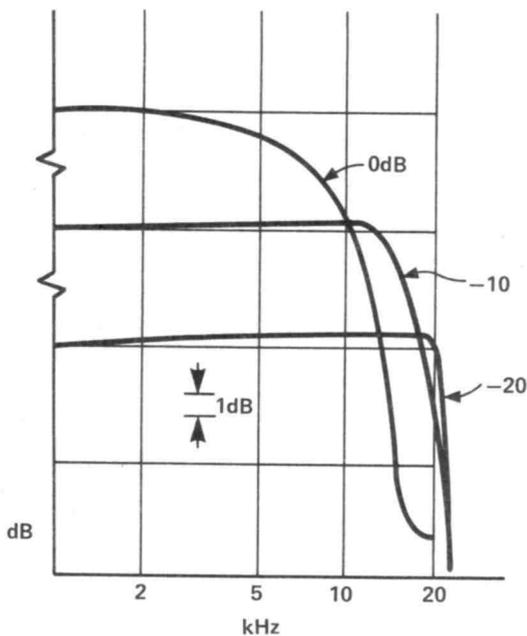
Figure 7: High frequency response of a typical cassette recorder.
