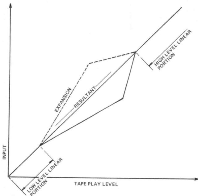
Figure 6: Ideal curves for record/playback processing.
