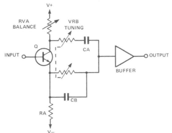
Figure 2: Circuit of an improved filter design.
