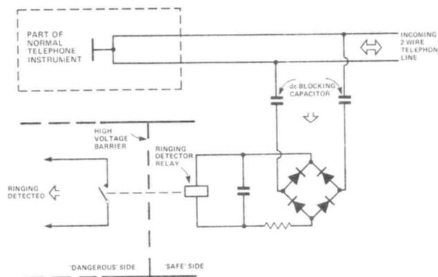
**Figure 7(b):** If a ringing detector circuit is used, it must not 'bridge' the safety barrier.
