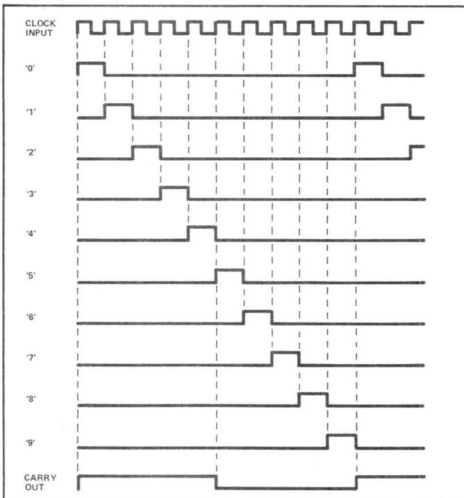
Figure 2: Waveform timing diagram of the 4017B, with its RESET and CLOCK INHIBIT terminals grounded.
