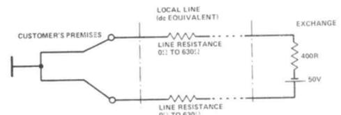
Figure 1(e): For DC the same line looks like a 50 volt DC source having an internal resistance of between 400 ohms and 1660 ohms depending on the length of the line.
