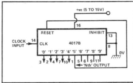
**Figure 5:** Simple method of connecting the 4017B as a divide-by- $N$  ( $N = 2$  to 9) counter with ' $N$ ' decoded outputs. The circuit is shown set for divide-by-5 operation.
