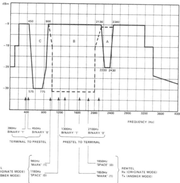
**Figure 2: Maximum one-minute-mean power levels of individual spectral components of the output signal from apparatus connected to the PSTN. Signals are permitted in Area A only if accompanied by signals in Area B at a power level not lower than 12dB below the power level of the signal in Area A. Signals are permitted in Area C provided that there is no false operation of trunk signalling equipment.**
