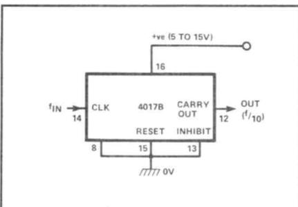
Figure 3: 4017B connected as a decade counter/divider.
