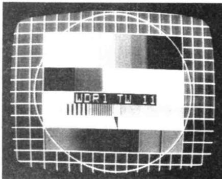
Figure 1: Westdeutscher Rundfunk FuBK test card from the Teutoburger Wald transmitter on channel E11.
