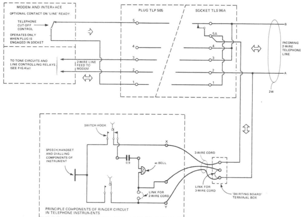
**Figure 5: Circuit diagram of the ringer in a typical telephone instrument.**
