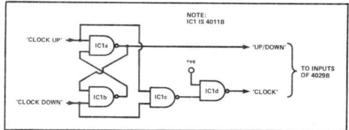
**Figure 21: Simple circuit for converting the 4029B to a 'dual clock' UP/DOWN counter.**
