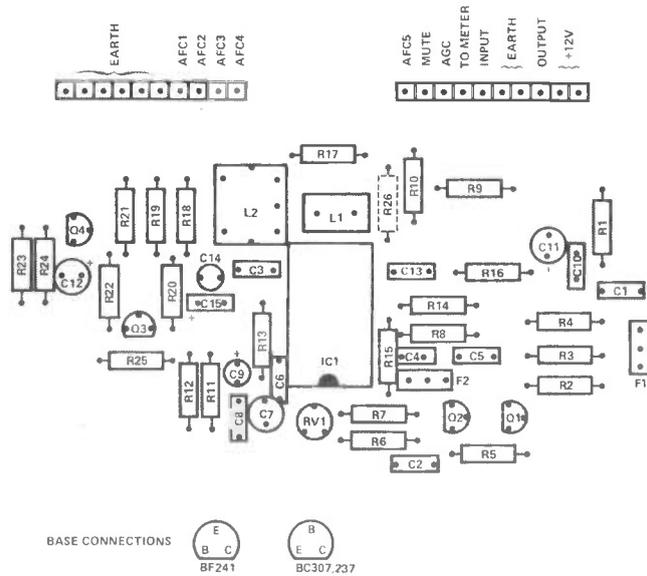
Figure 3: Component overlay for the Wideband FM-IF strip.
