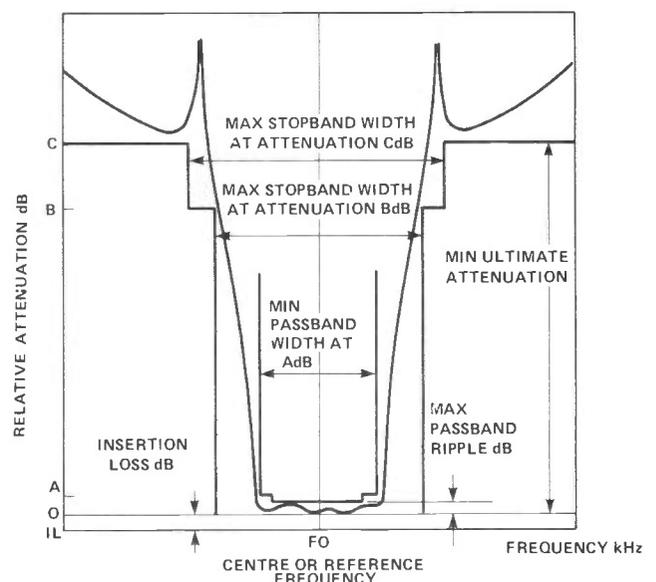
**Figure 1: Explanation of the filter specification.**
