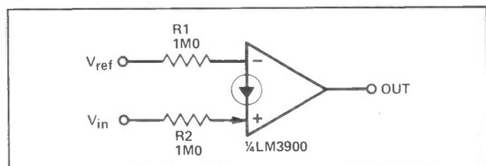
Figure 13: Non-inverting voltage comparator.
