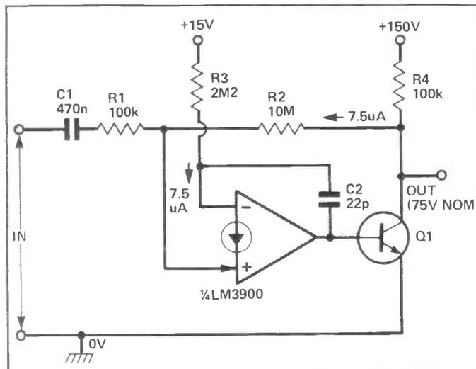
Figure 10: High-voltage amplifier with  $\frac{1}{15}$  100 gain.
