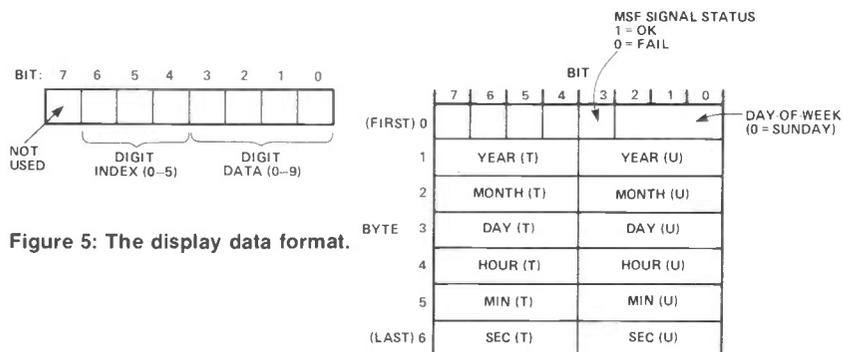
Figure 5: The display data format.
