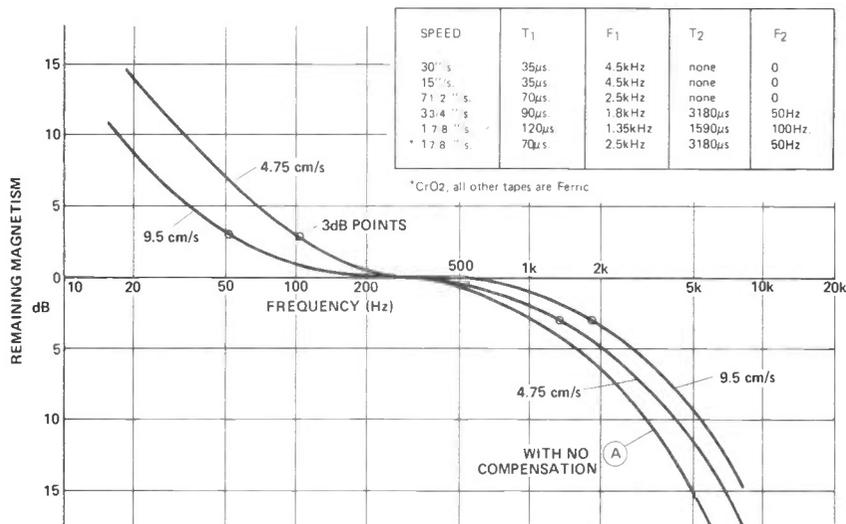
**Figure 6: Equalisation standards for tape recording at different tape speeds.**
