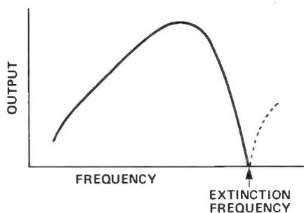
**Figure 5: Typical tape head replay characteristics.**
