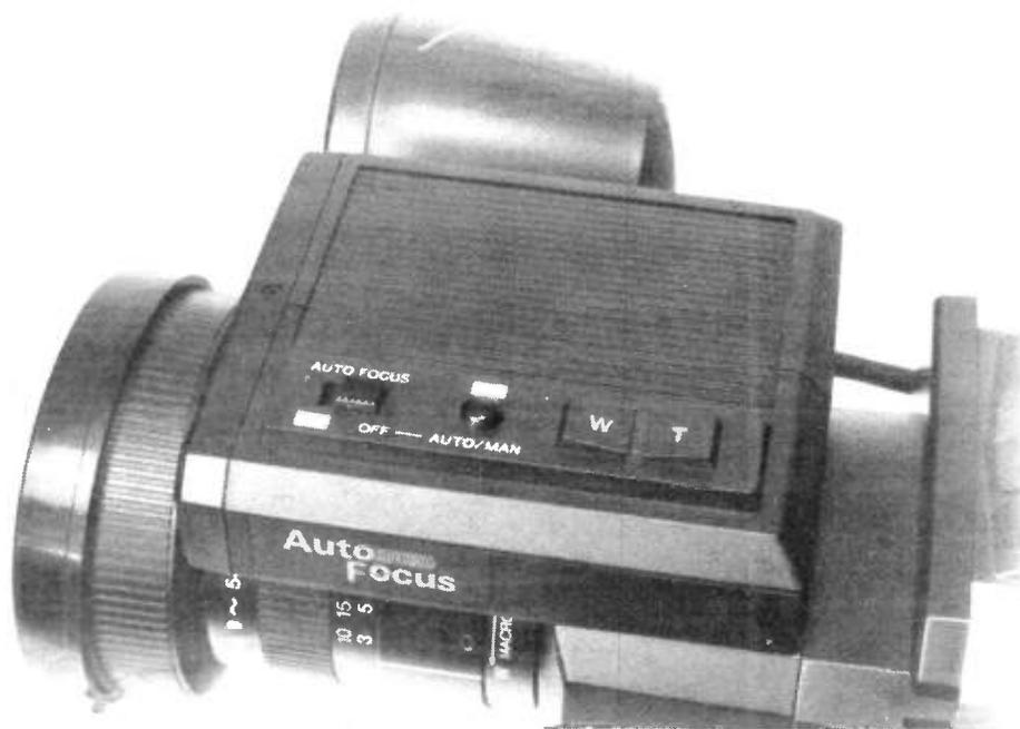
Detail of the auto focus control's and the power zoom rocker switch.
