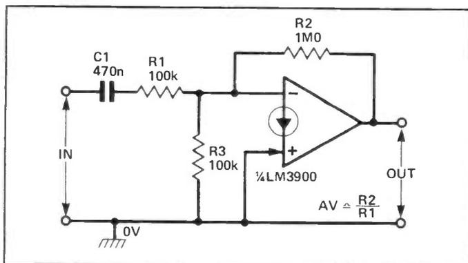
Figure 7: Inverting ac amplifier with  $N/15$   $V_{be}$  biasing.
