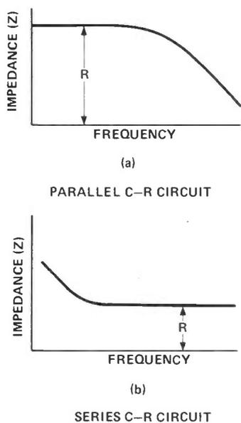
**Figure 7: Parallel (above) and series (below) CR circuit curve.**
