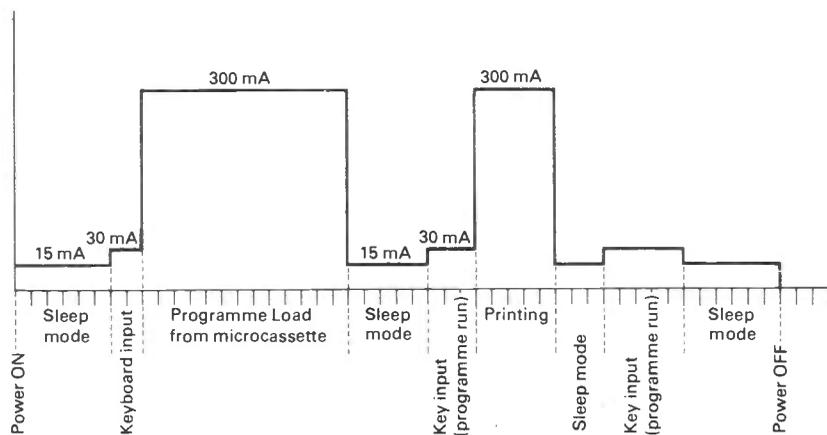
Figure 4: Current consumption over a typical minute
