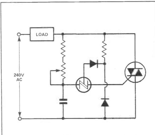
Figure 1: Typical lamp dimmer circuit using discrete circuitry.
