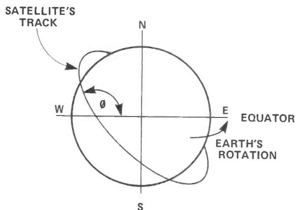
**Figure 1:** The track of satellite's orbit around the earth.  $\theta$  = angle of inclination. Remember the earth rotates from west to east, whereas the track of the satellite stays the same in space.
