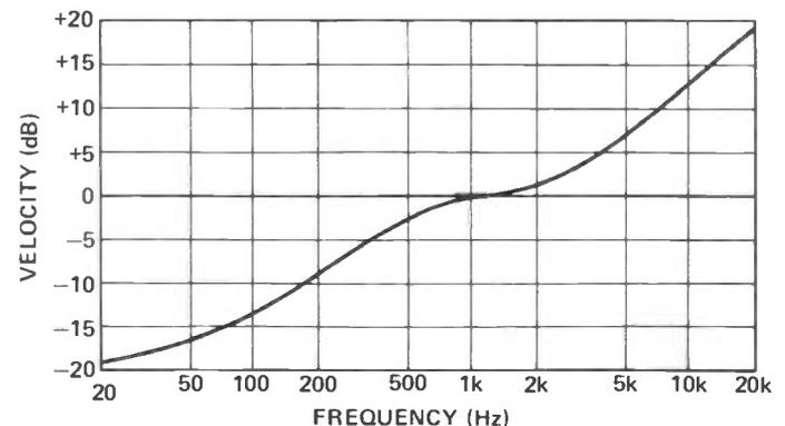
Figure 2: The RIAA characteristic for 'recording' equalisation.
