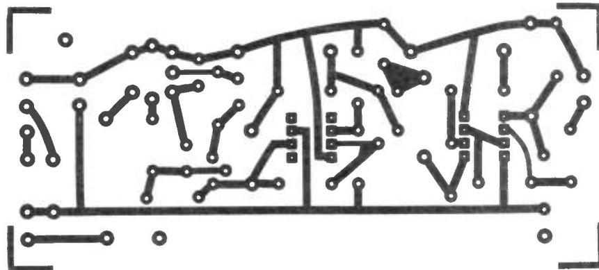
Figure 5: PCB foil pattern for the transmitter.
