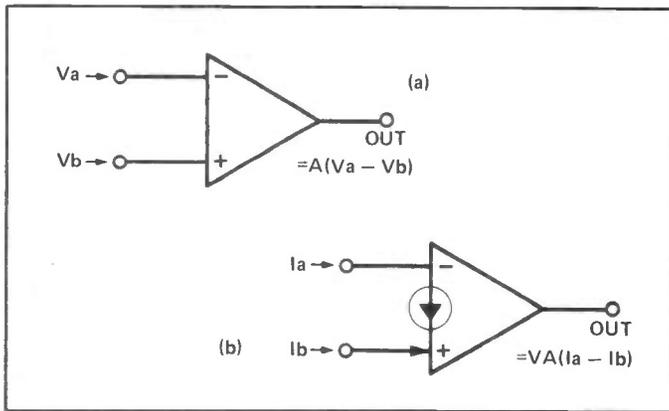
Figure 1: A conventional op-amp (a) is a voltage-differencing amplifier, but a Norton op-amp (b) is a current-differencing device.
