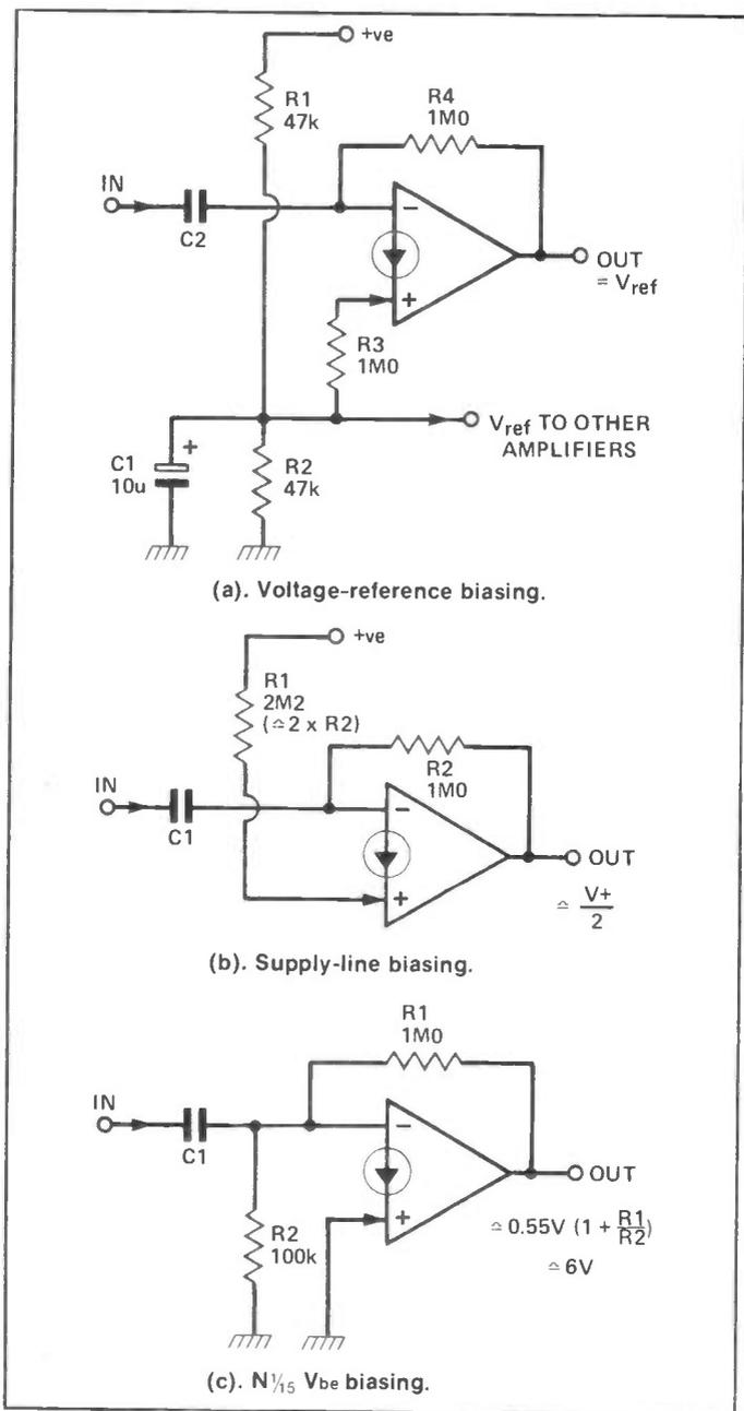
Figure 5: Methods of biasing LM3900 op-amps for linear operation.
