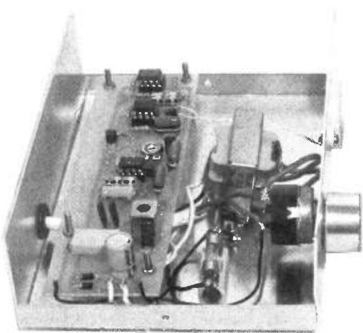
Internal view of the completed receiver. The flat disc in the top right is a piezo transducer.
