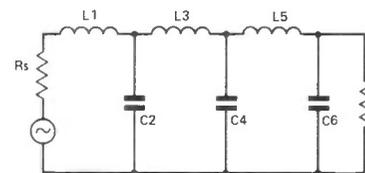
2. Transform all reactive elements to put all six reactances into the series arms of the ladder using five Impedance Invertors (Nanton Transformation). Because of the impedance inverter all six series reactances will be inductive.
