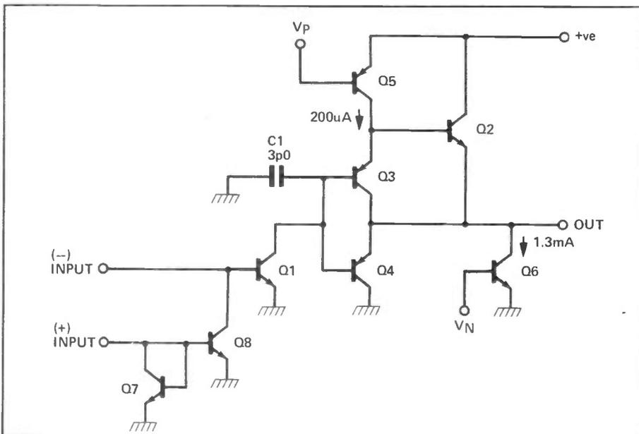
Figure 3: Circuit of each of the four identical op-amp stages of the LM3900.
