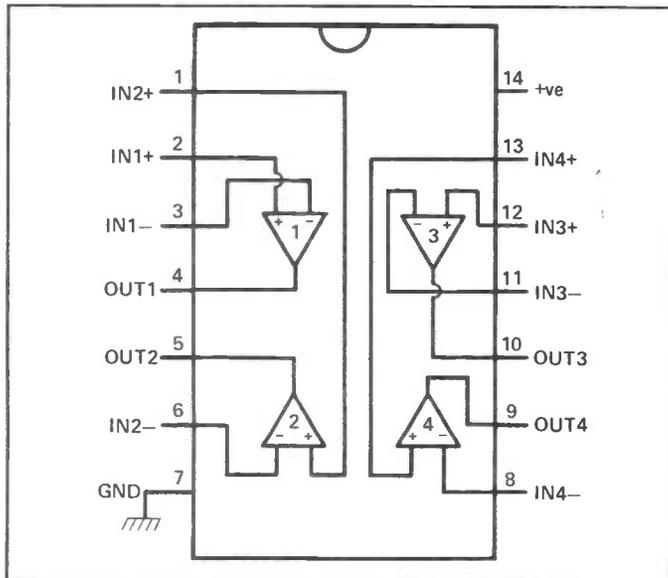
Figure 2: Connections of the LM3900 quad Norton op-amp.
