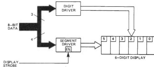
Figure 4: The general form of a multiplexed display suitable for the Rewbichron design.
