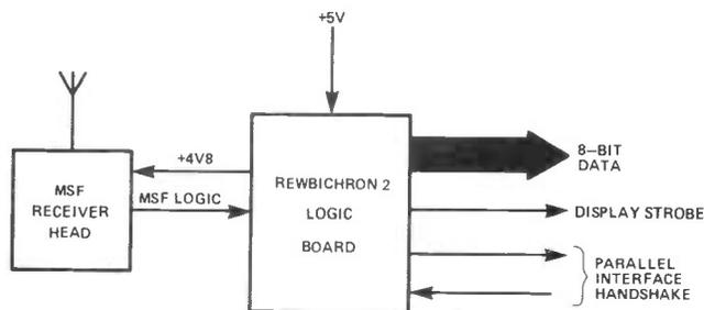
Figure 3: Block diagram of the main logic board.
