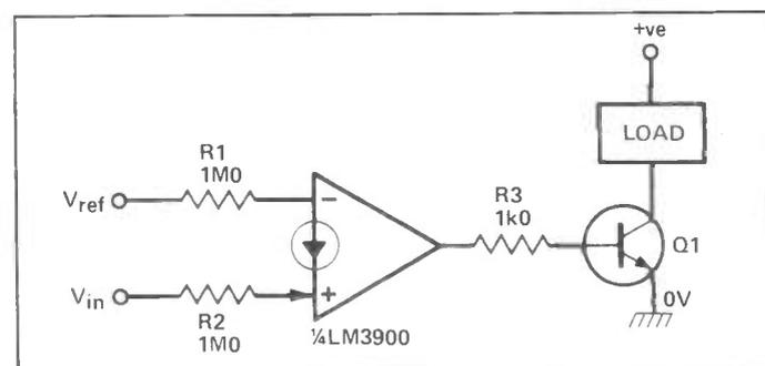
Figure 14: Non-inverting power comparator.
