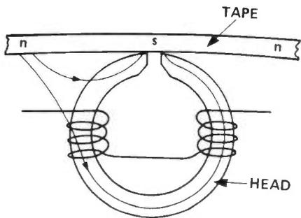
**Figure 4: Effect on tape magnetisation when wavelength is long compared to head dimensions.**
