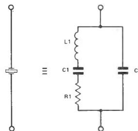
**Figure 3: Equivalent circuit of a crystal.**
