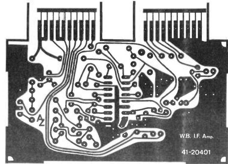
Figure 4: PCB foil pattern for the FM-IF strip. Note that the six elongated pads in the top right hand corner are connected to earth.
