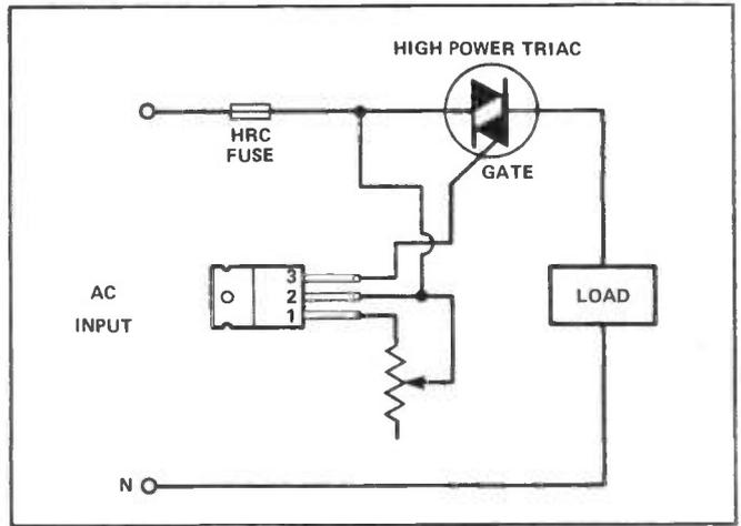
Figure 4: Drive circuit for high power triacs.
