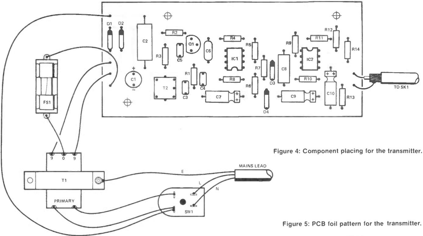
Figure 4: Component placing for the transmitter.
