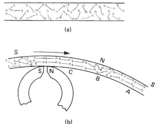
Figure 3: Organisation of 'bar magnets' on a tape (a) before and (b) after contact with the recording head (long wavelengths).
