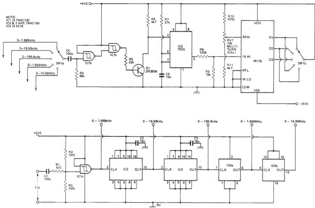
This circuit is of a practical DVM-based Digital Frequency Meter that reads up to 19.99MHz full-scale in five decade ranges. The circuit accepts input signals in the range 200mV to 5V0 RMS, and operates as follows.
