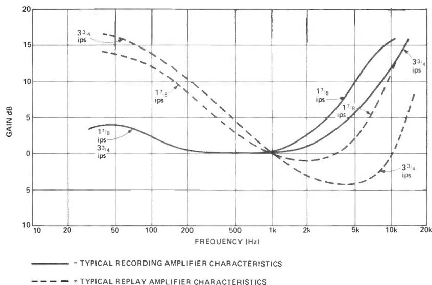
**Figure 8: Tape replay equalisation on a typical amplifier (with speed adjustment).**
