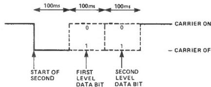
Figure 1: Certain 'seconds' pulses are modified to carry two bits.
