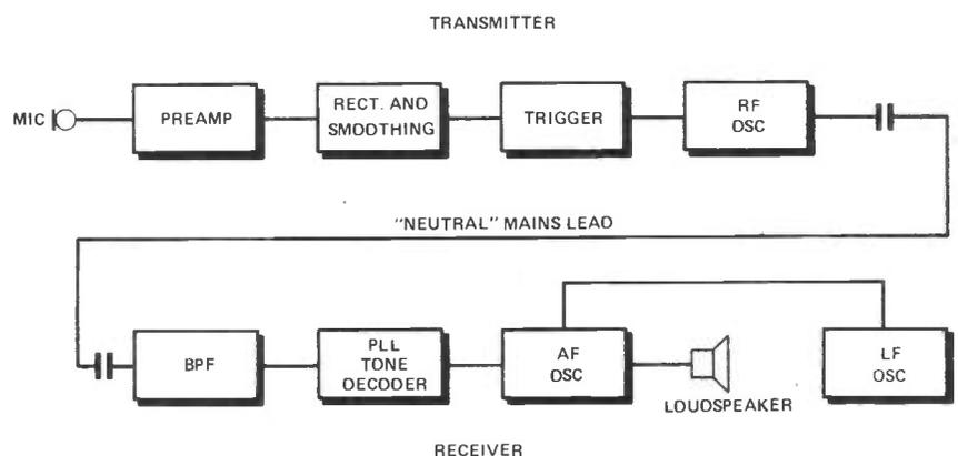
Figure 1: Block diagram of the complete signalling system.
