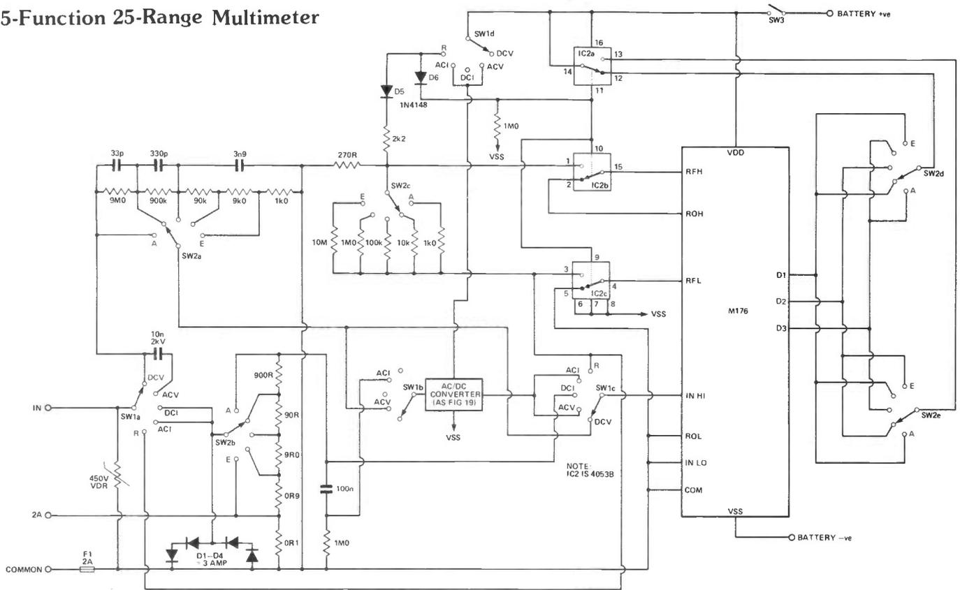
The reader should have little difficulty in following the circuit. Functions are selected by SW1, ranges by SW2. SW1a connects the inputs to the voltage, current or resistance measuring networks, and SW1d activates the
