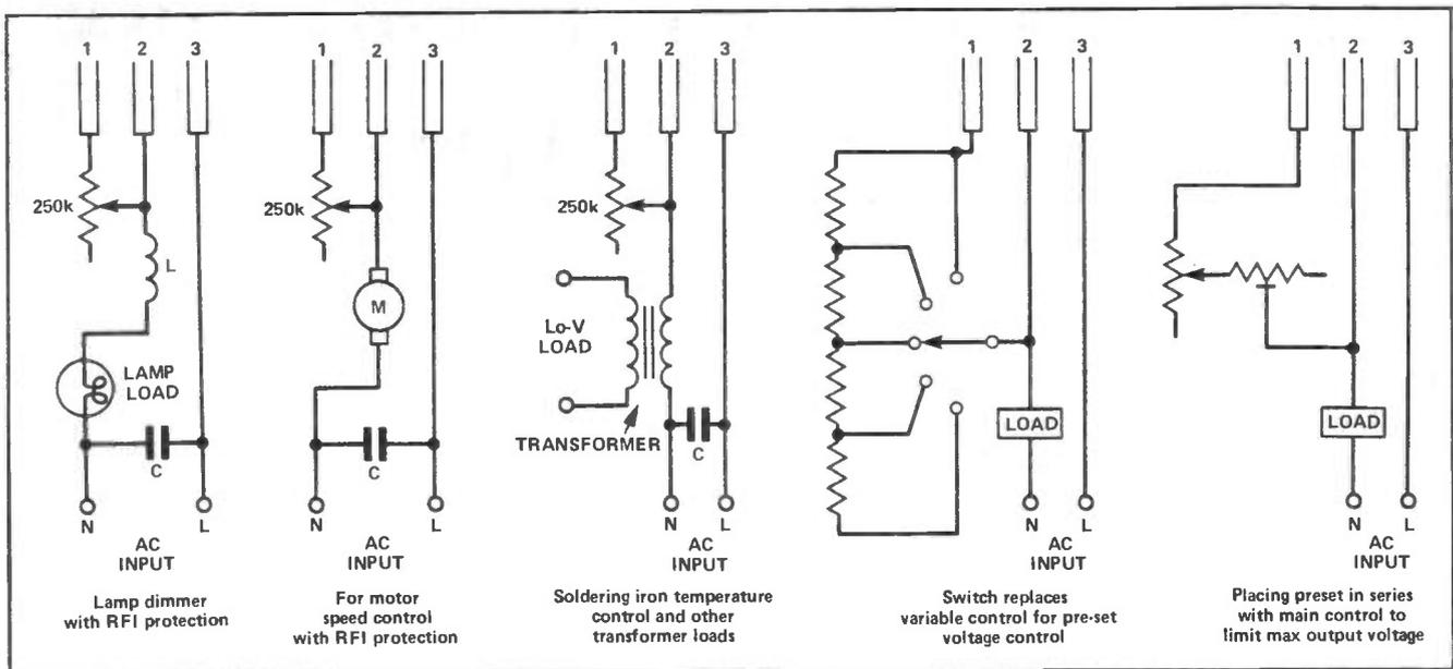
Figure 3: Typical applications for controller.
