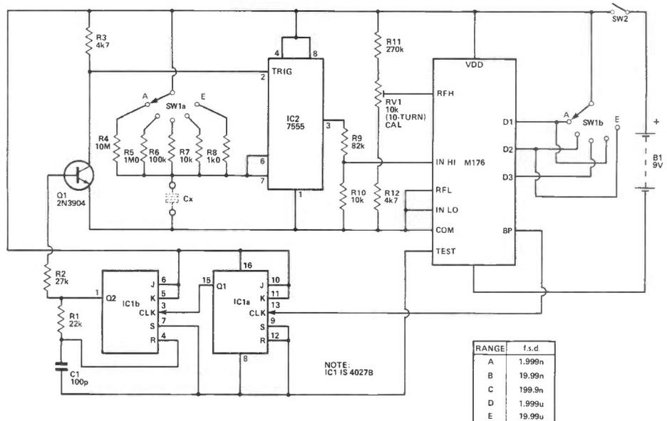
resulting signal is fed to the module's IN HI terminal, where it is integrated by the internal  $10\text{M} - 10\text{n}$  filter. Divider R11-RV1-R12 feeds 100mV nominal to the RFH terminal of the module, and RV1 is used to adjust the precise calibration of the Capacitance Meter.
