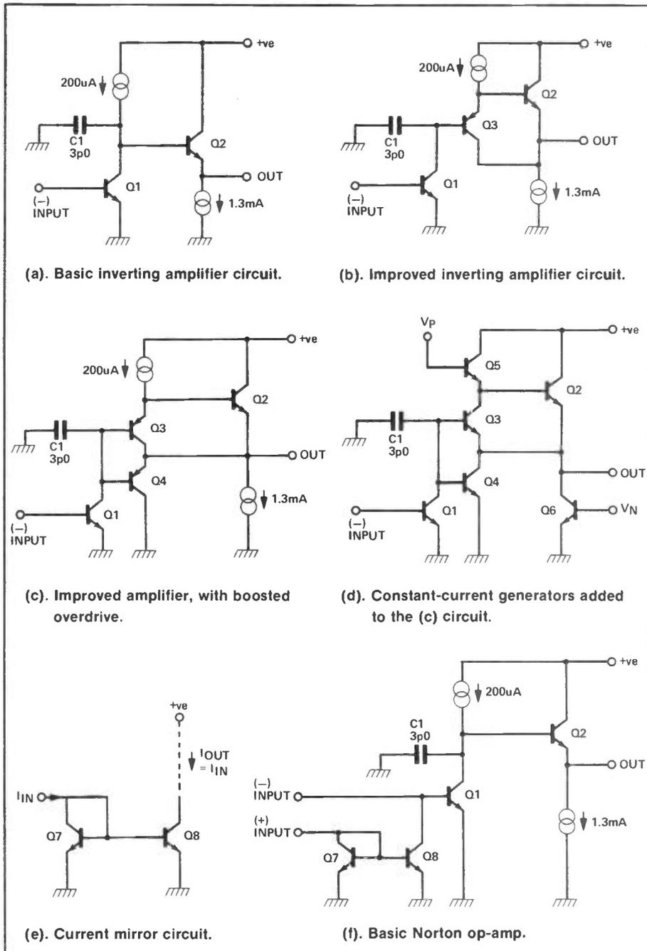
Figure 4: Stages in the development of the Fig. 3 circuit.
