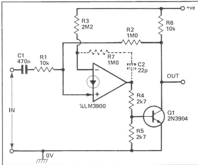
Figure 9: Wideband (200 kHz) high-gain (x100) amplifier.
