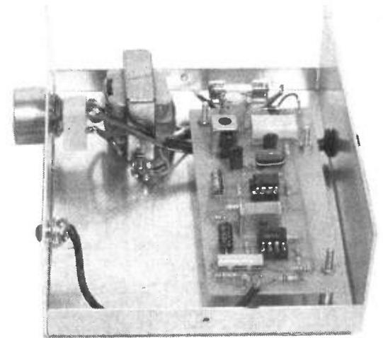
The prototype transmitter, with mic socket and mains on/off switch (the high surge current type is not essential).
