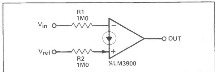
Figure 12: Inverting voltage comparator.
