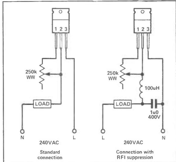
Figure 2: Basic controller connections.
