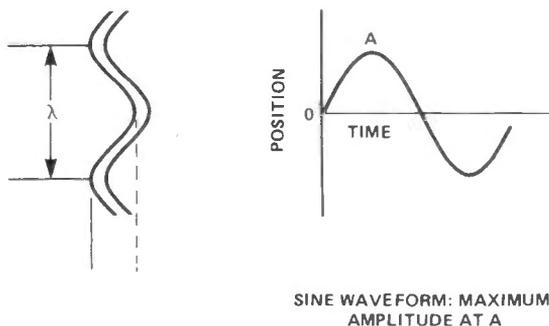
Figure 1: Sinewave represented in the form of a groove on a record.
