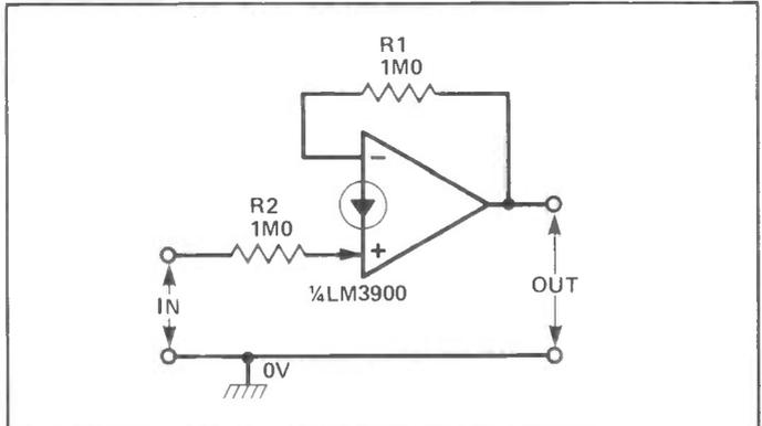
Figure 11: DC voltage-following buffer.
