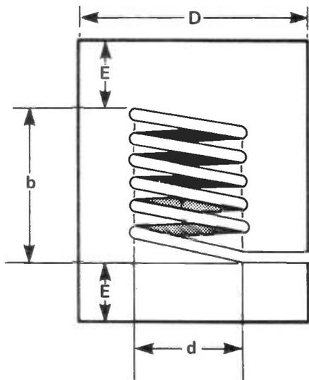
Figure 6: The basic design of a circular cavity filter.
