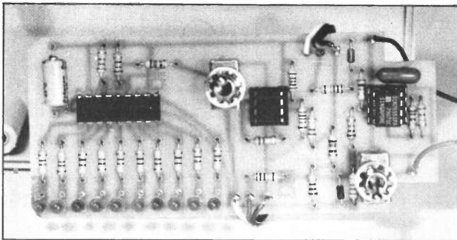
Internal view of the transistor tester.
