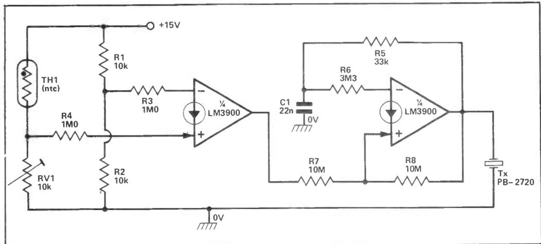
Figure 33: Audible-output over-temperature alarm.
