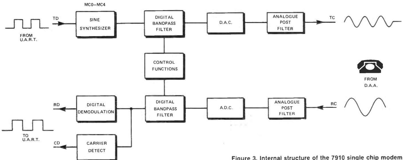
Figure 3. Internal structure of the 7910 single chip modem.
