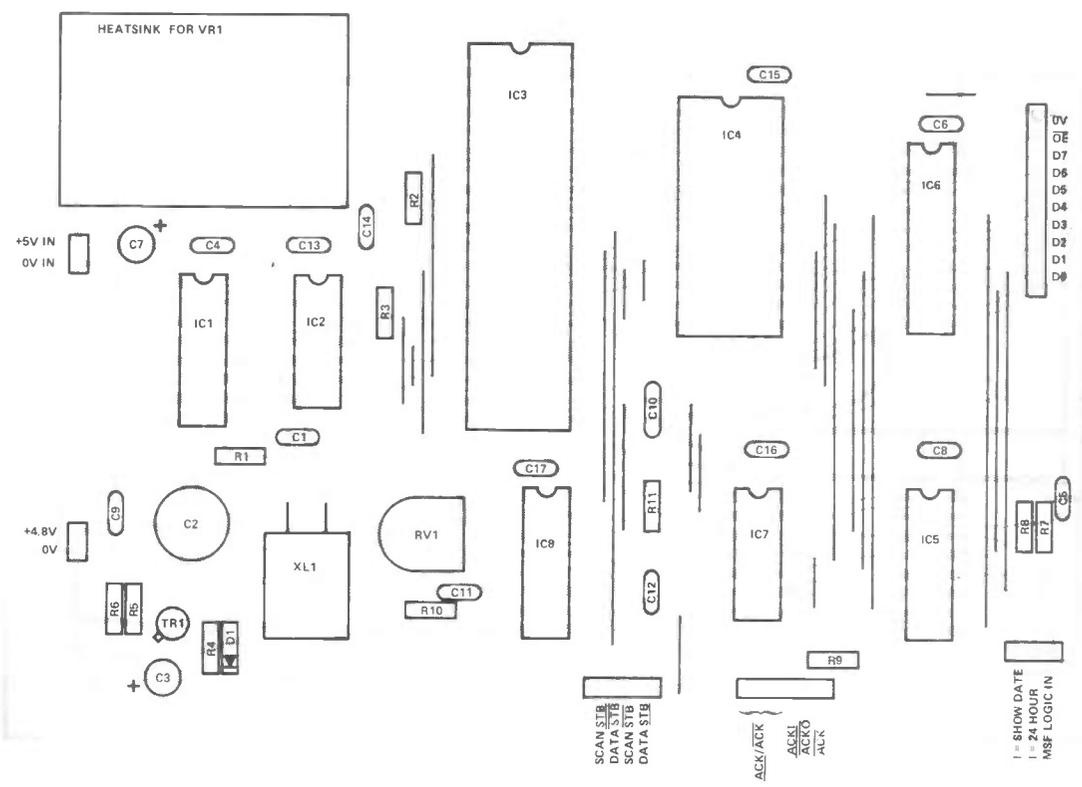
Figure 10. Overlay of the Rewbichron's logic board.
