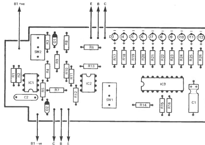
Figure 3. Component placing on the tester PCB.
