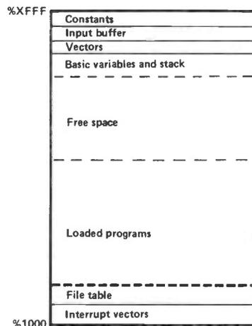
Figure 3. The Z8 Exec RAM memory map. A standard file format is used to enable easy location when loading files.
