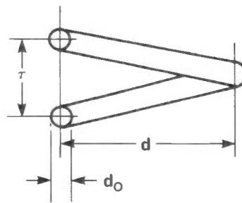
Figure 7: Winding measurements are taken from the mean of the wire diameter.
