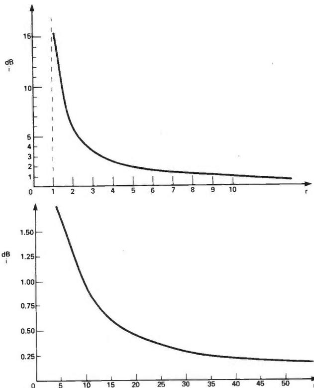
Figure 2: Insertion loss of a filter plotted against r the ratio of the unloaded to loaded Q of the filter.
