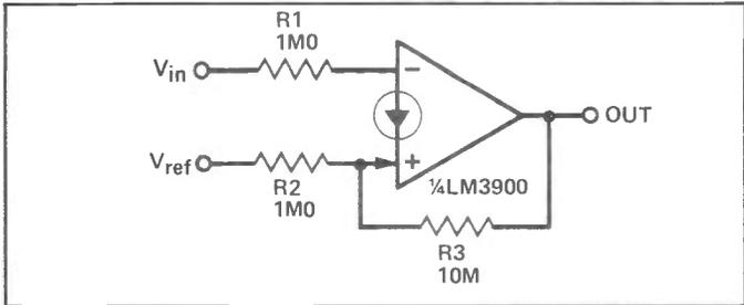
Figure 15: Inverting Schmitt trigger.
