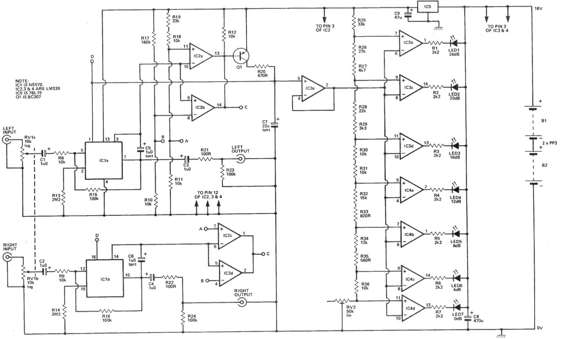
Figure 1. Full circuit of the Audio Limiter
