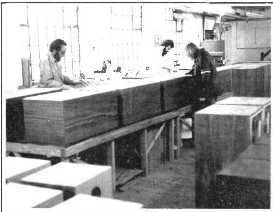
Fitting the contoured foam to the sides of the tapered transmission line. A special adhesive is used to make sure the foam is fitted securely. Each cabinet is then thoroughly checked before passing onto the next stage.
