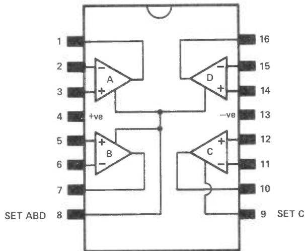
Figure 1: Pin configuration of the LM346N. The layout is identical for the LM124 and LM148.
