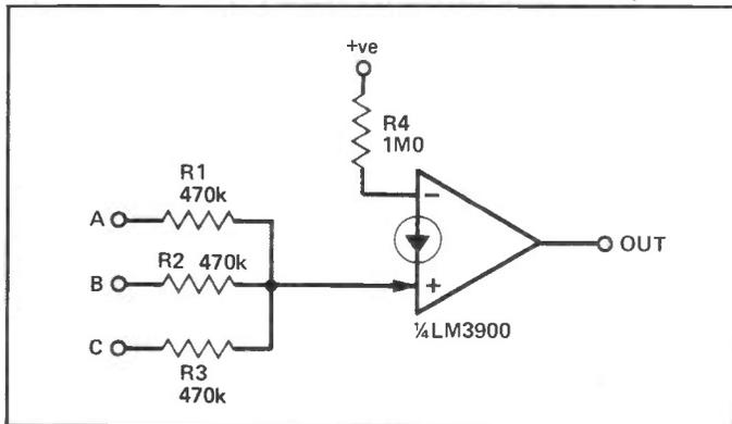
Figure 20: 3-input OR gate (can be converted to a NOR gate by transposing the op-amp inputs).
