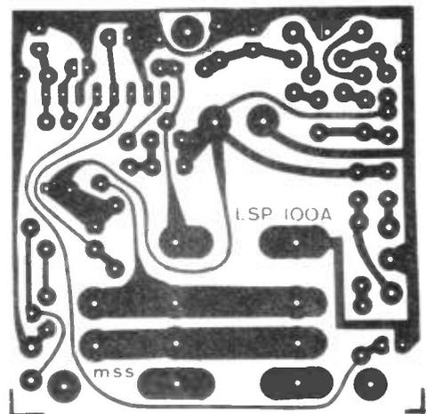
Foil pattern for loudspeaker protection board.
