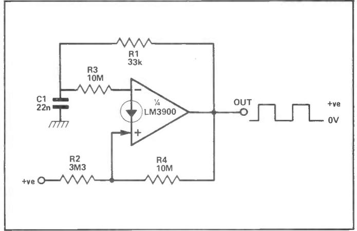
Figure 31: 1 kHz square-wave generator.
