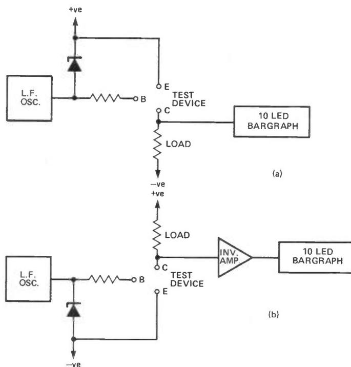
Figure 1. The two basic circuit configurations for testing NPN and PNP transistors.
