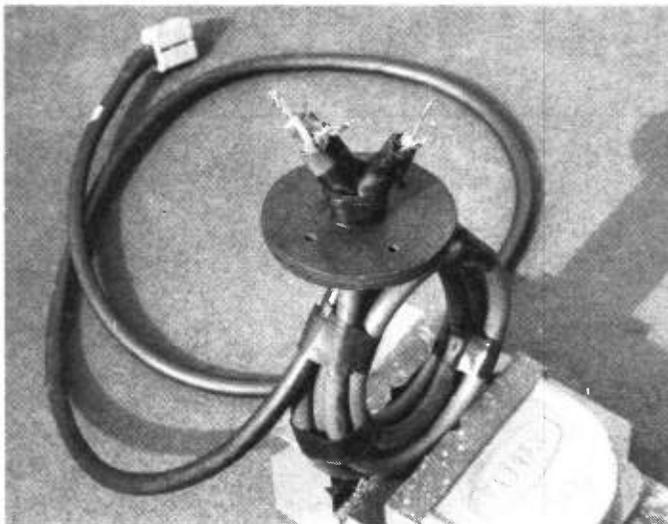
Figure 2. Arrangement of stub and matching sections of coaxial cable and insulating disc for ends of dipoles for the 10 metre crossed dipole antenna .
