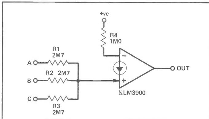
Figure 21: 3-input AND gate (can be converted to a NAND gate by transposing the op-amp inputs).
