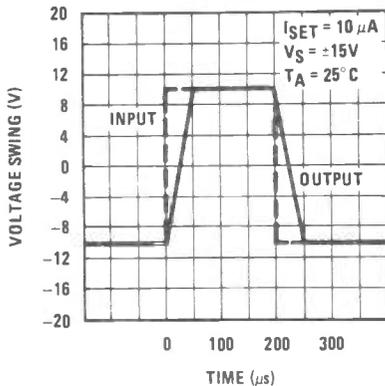
Figure 3: Pulse response against voltage swing.
