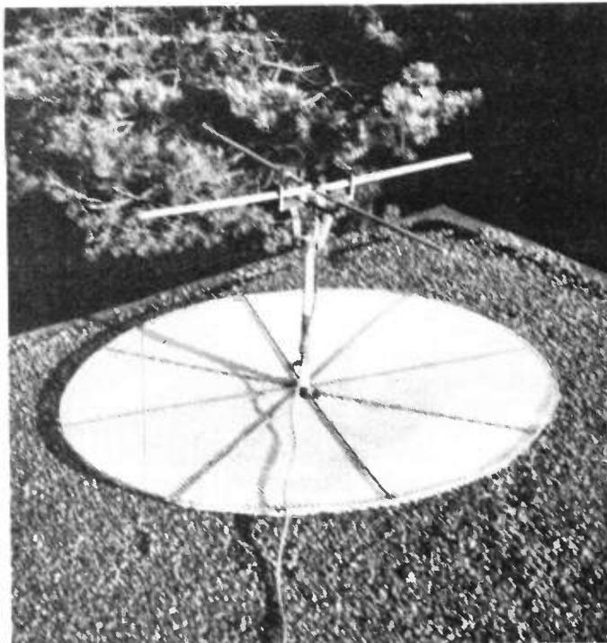
Figure 3. General arrangement of the 2 metre crossed dipole and earth mat to give good vertical radiation.
