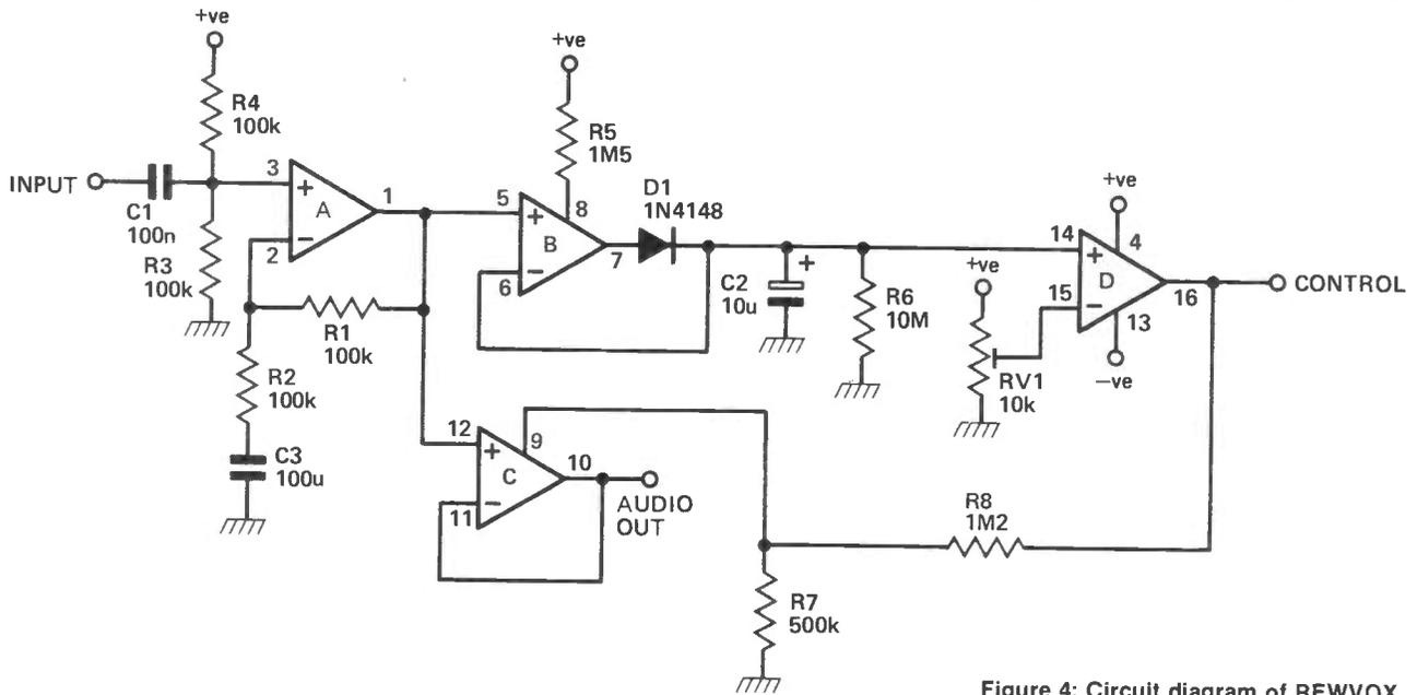
Figure 4: Circuit diagram of REWVOX.
