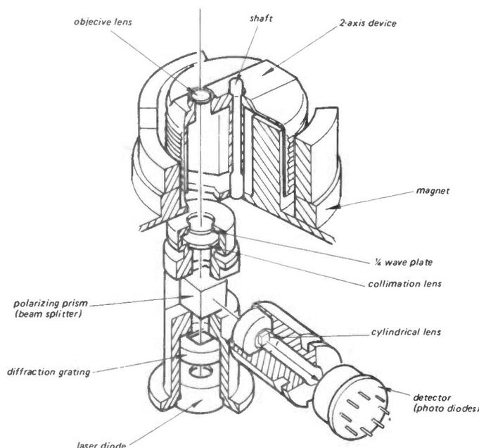
Figure 7: A schematic view of the Sony players optics.
