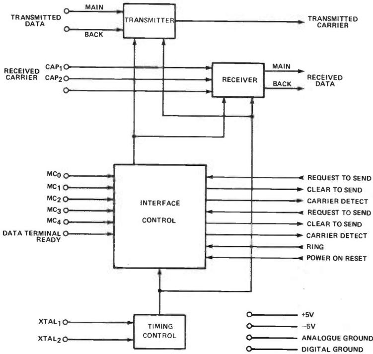
Figure 4. Control circuitry involved in modem design.
