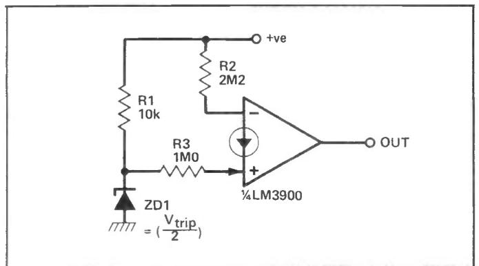
Figure 19: Supply under-voltage detector.
