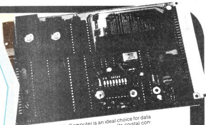
The Essex Tiny Basic Computer is an ideal choice for data acquisition and process control systems. Its crystal controlled timer and interrupts provide accurate timing and fast response to critical events, while the watchdog timer ensures reliable operation. Programs can be entered and tested from an RS232 terminal, and then be copied into EPROM. Alternatively, Instant ROM modules may be used both during development and for program storage.
