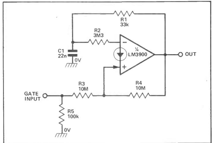
Figure 32: Gated 1 kHz astable.
