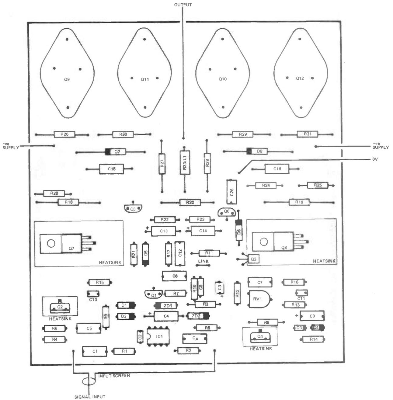
Component overlay for the 100W Power Amplifier.
