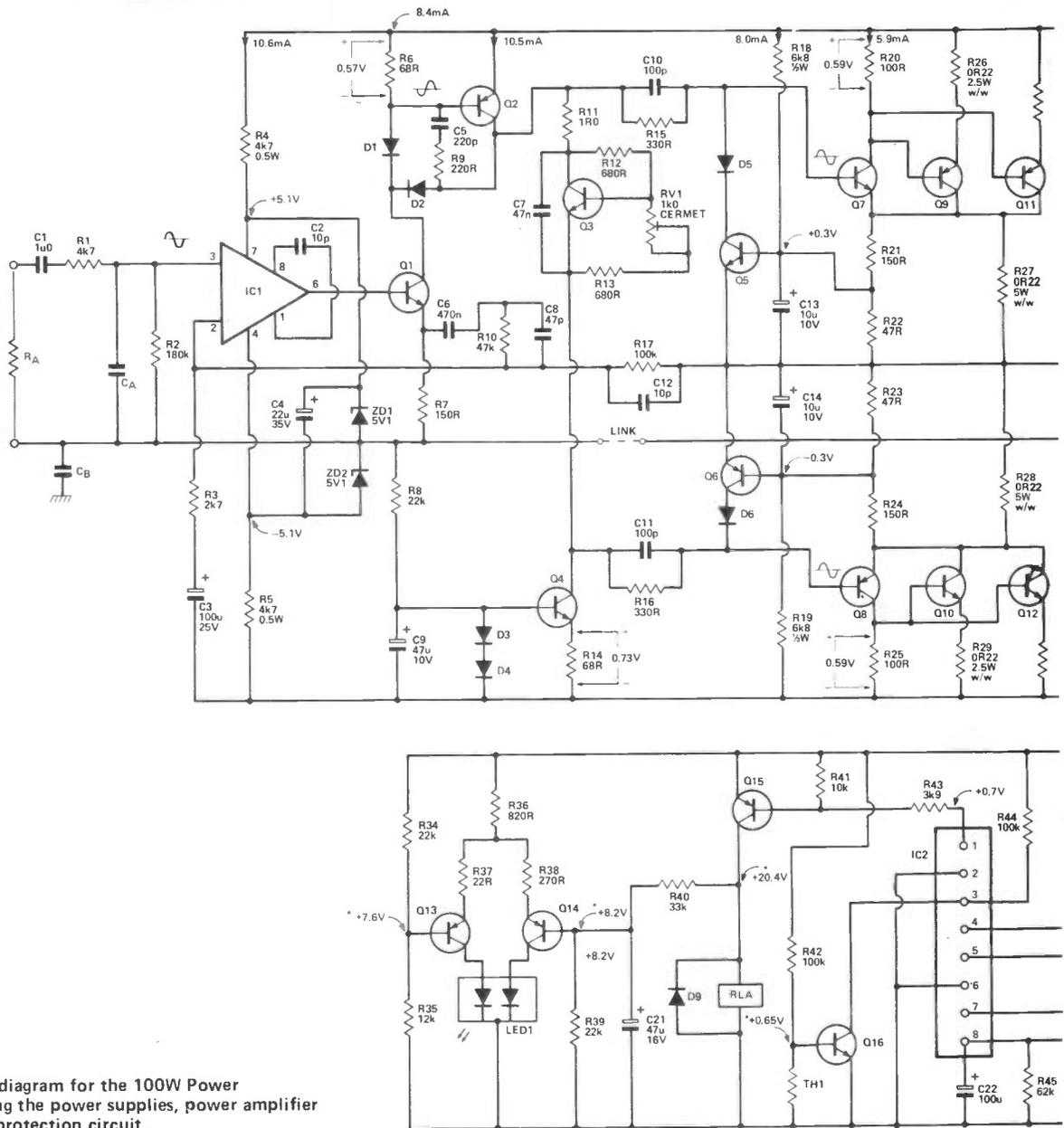
Complete circuit diagram for the 100W Power Amplifier, showing the power supplies, power amplifier and loudspeaker protection circuit.
