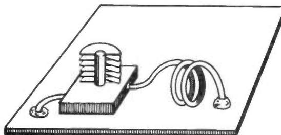
If the required attenuation cannot be achieved using one filter element then more can be used, say one before an amplifier and one after. This will produce the required attenuation but will also reduce the 3dB bandwidth which may be an undesired result.
