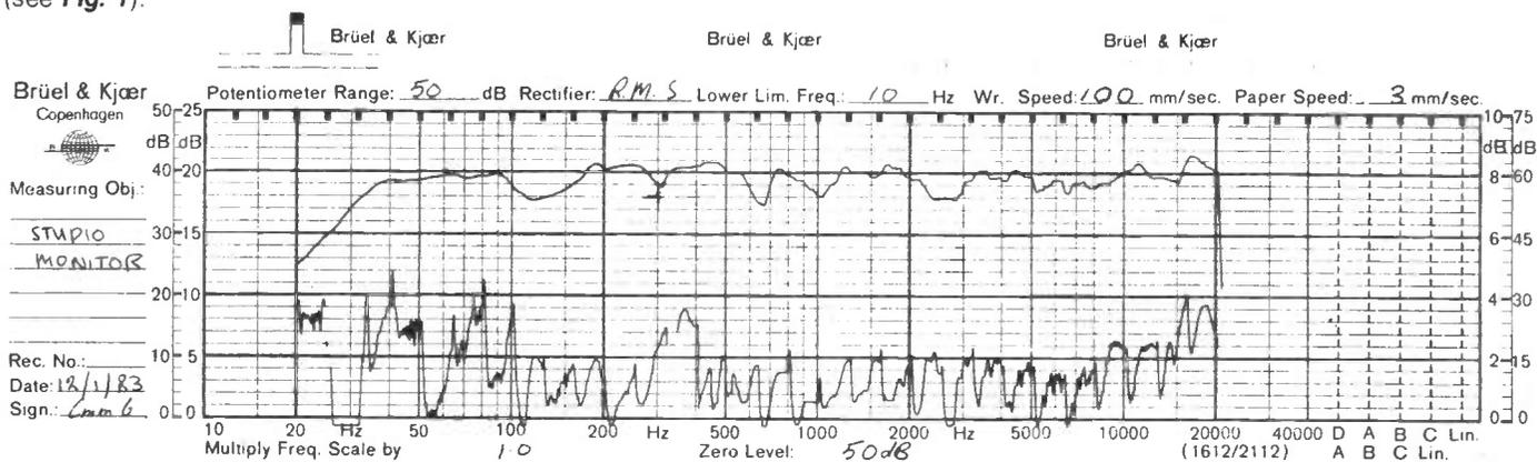
Upper Curve Frequency Response - 1 metre on Mid Axis 5 Volt Input.
