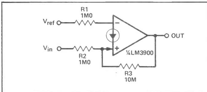
Figure 16: Non-inverting Schmitt trigger.
