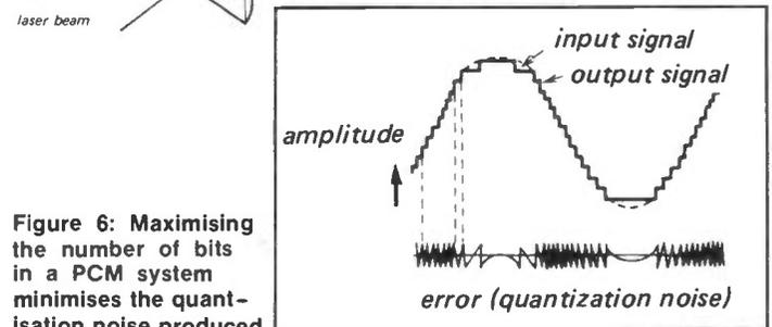
Figure 6: Maximising the number of bits in a PCM system minimises the quantisation noise produced.
