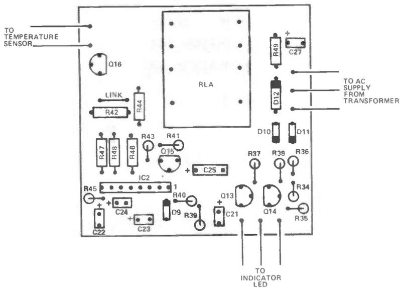
Component overlay for the loudspeaker protection board.
