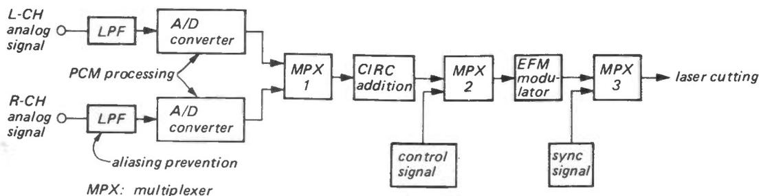
Figure 1: Block diagram of the A/D conversion system used in the production of CD discs.
