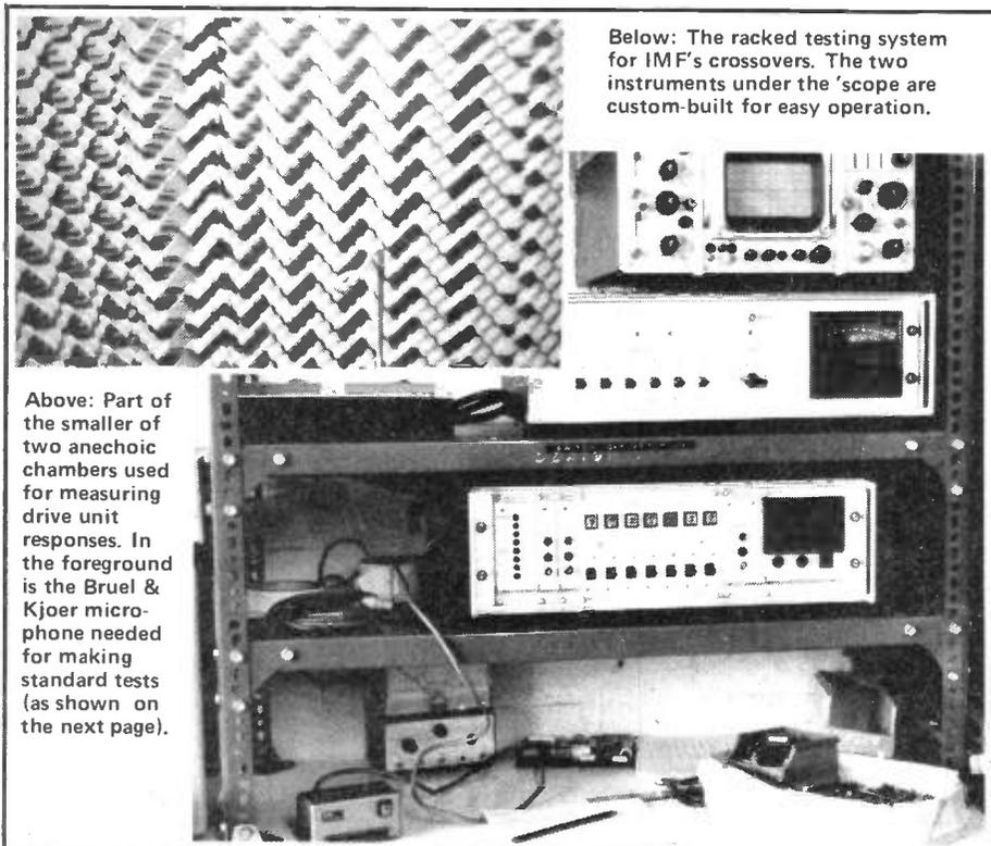
Below: The racked testing system for IMF's crossovers. The two instruments under the 'scope are custom-built for easy operation.
