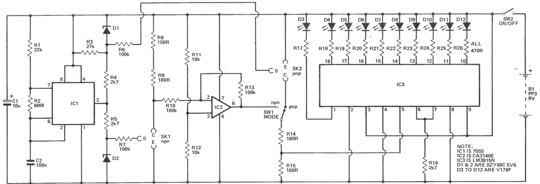
Figure 2. Complete circuit of the tester.
