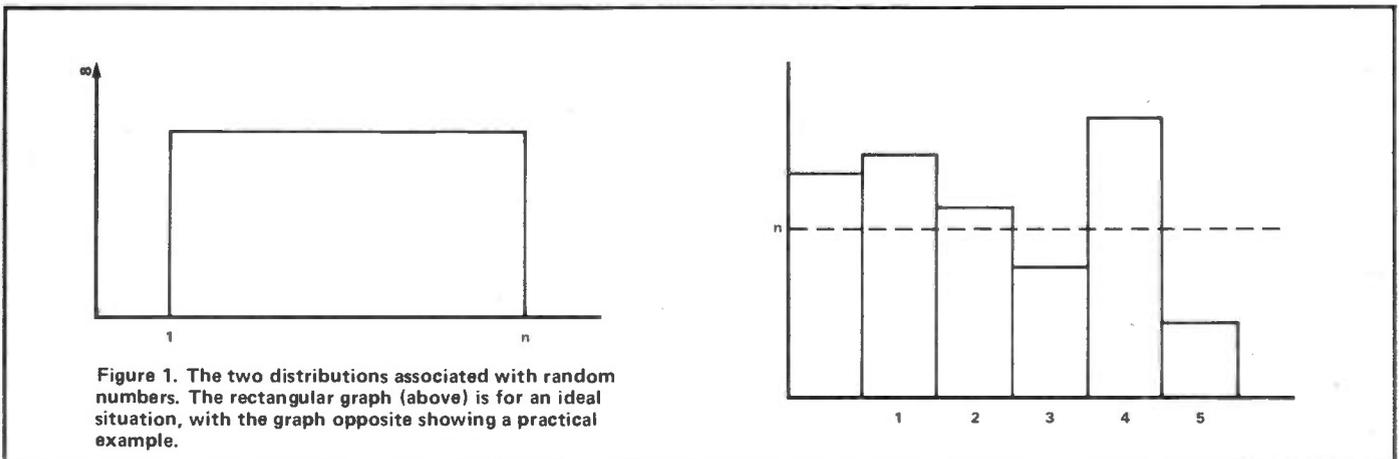
Figure 1. The two distributions associated with random numbers. The rectangular graph (above) is for an ideal situation, with the graph opposite showing a practical example.
