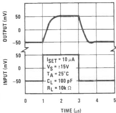
Figure 2: Transient response, showing input and output waveforms.
