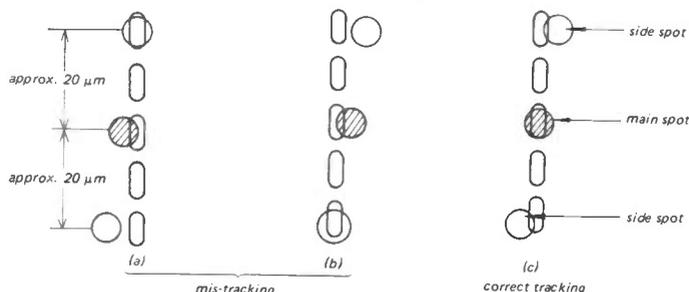
**Figure 8: The tracking control system operates by monitoring the amount of light reflected back from the main beam's side spots.**
