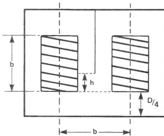
Figure 9: Coupling of filters is achieved by cutting a slot in the wall separating two resonators.
