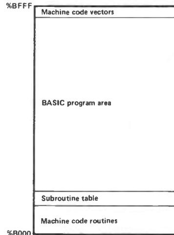
Figure 2. Memory map of Z8 Exec's Part 1 EPROM. This contains the command line interpreter.
