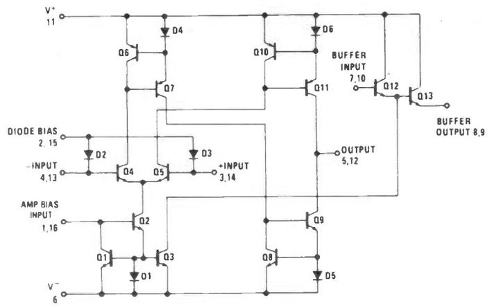
Figure 2: One operational transconductance amplifier.
