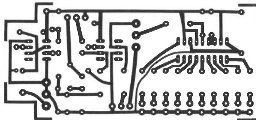
Figure 4. PCB foil pattern for the transistor tester.
