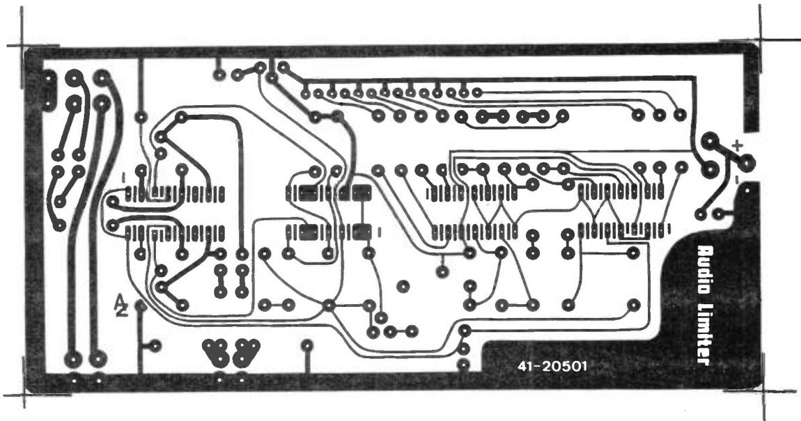
Figure 2. Foil pattern for the limiter board.
