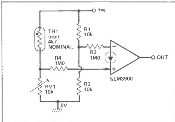
Figure 17: Over-temperature switch.
