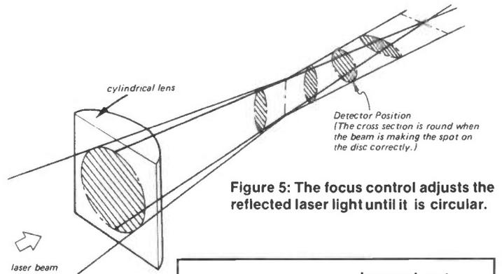
Figure 5: The focus control adjusts the reflected laser light until it is circular.
