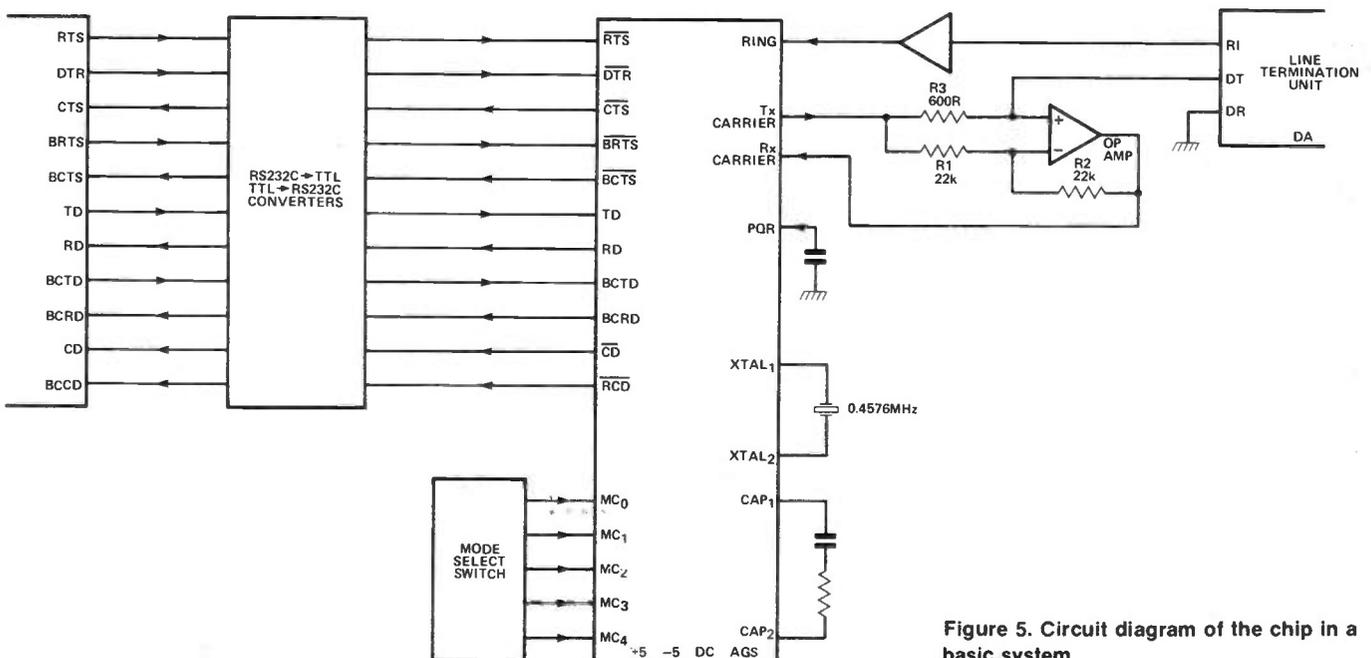
Figure 5. Circuit diagram of the chip in a basic system.
