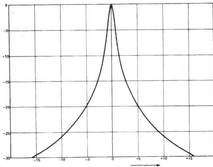
Figure 1: Amplitude vs frequency of a typical parallel tuned circuit.
