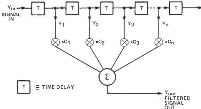
Figure 2. A similar filter without external feedback path.
