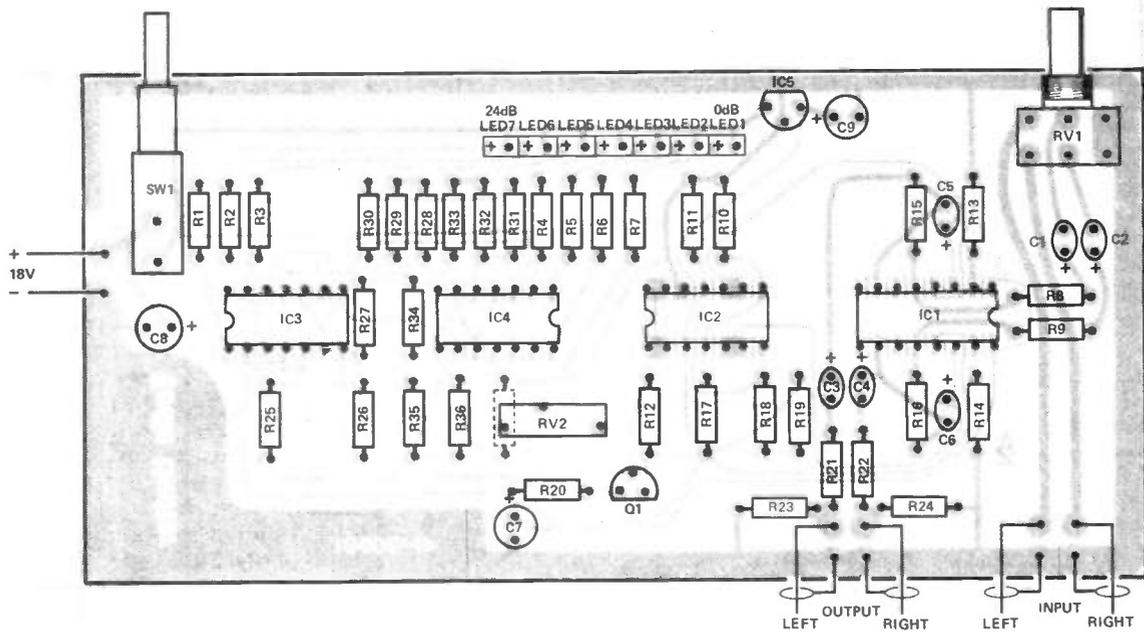
Figure 3. Component placing on the single PCB.
