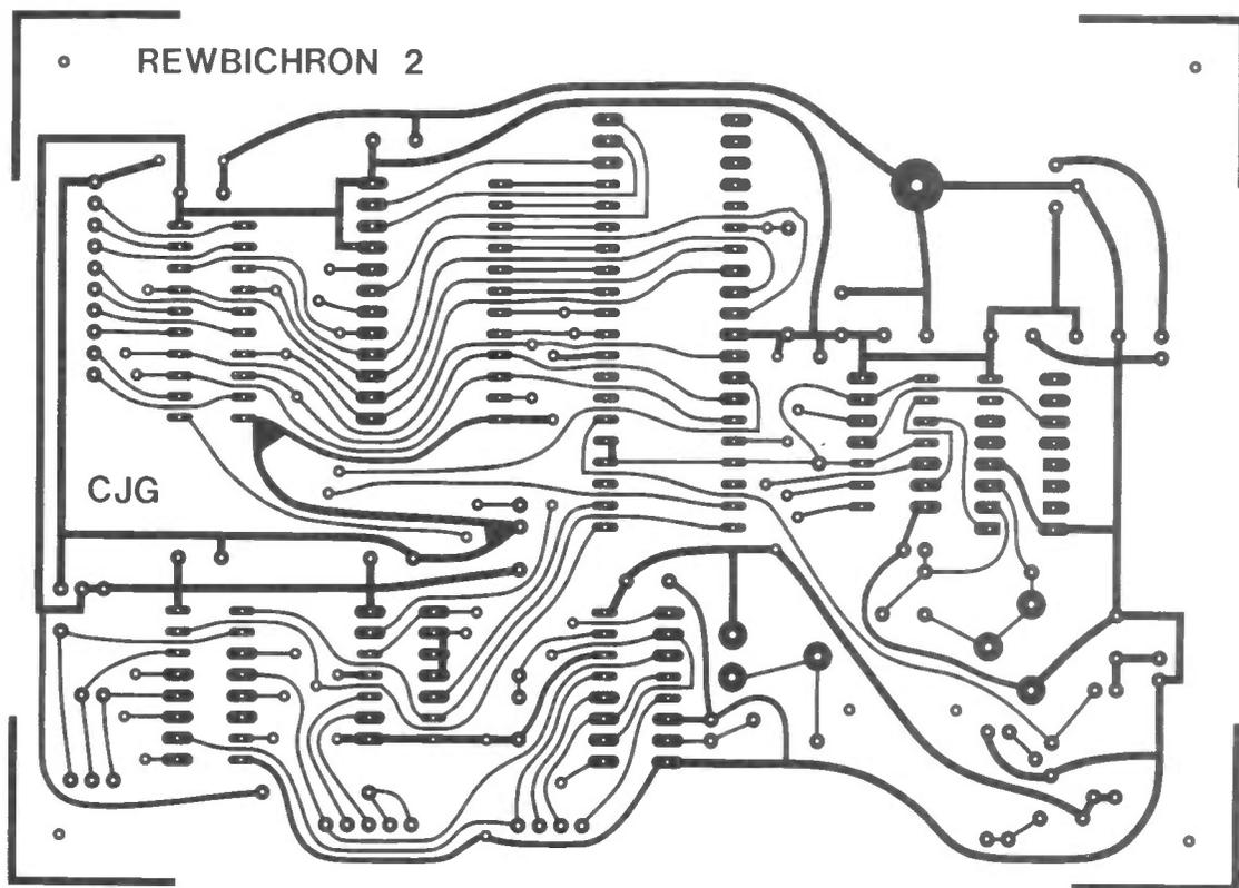
Figure 9. The logic board's foil pattern.
