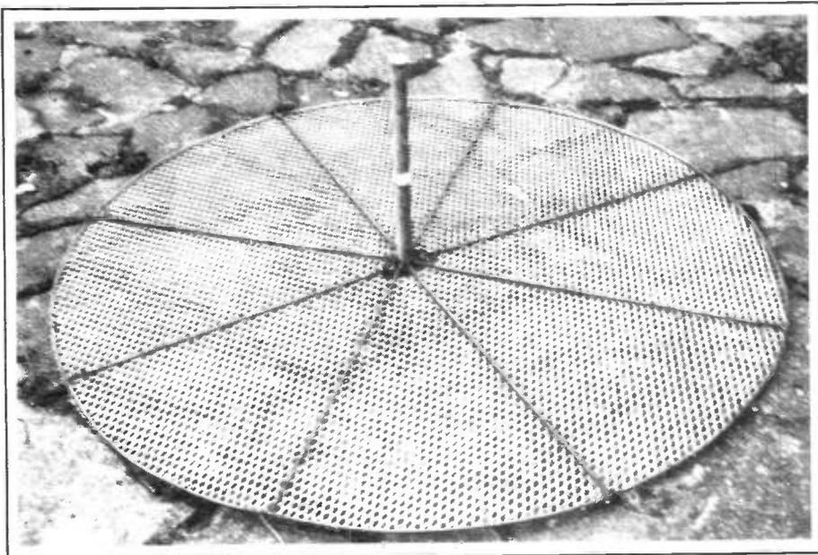
Figure 4. Detail of construction of earth mat and supporting 'mast' for the 2 metre crossed dipole.
