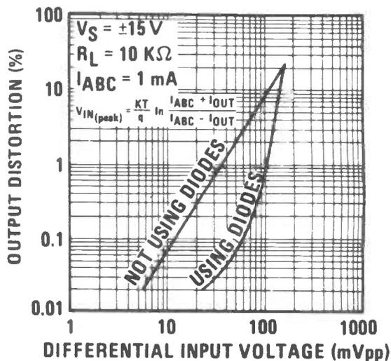
Graph of output distortion vs differential input voltage to show the effect of linearizing diodes.
