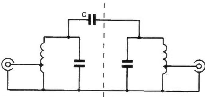
Figure 4: Coupled circuits result in better attenuation while maintaining a reasonable working bandwidth.
