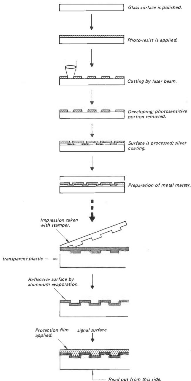
Figure 3: An illustration of the CD disc's manufacturing process.
