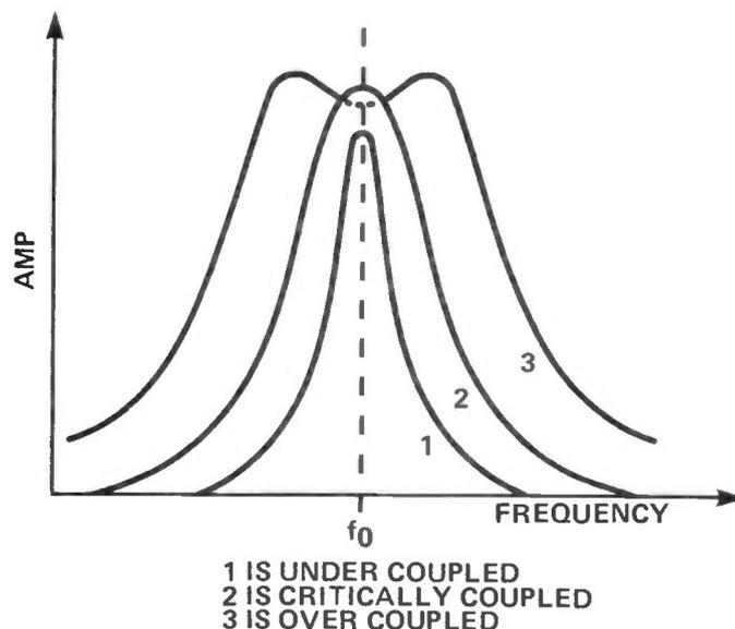
Figure 5: The result of varying the coupling between two filters.
