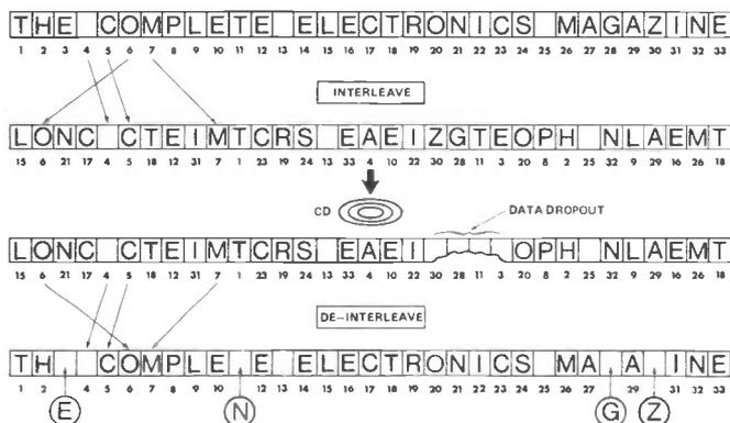
Figure 2: An illustration of the interleaving process which spreads individual data blocks over a larger area of the disc's surface. This minimises the effect of any drop-outs.
