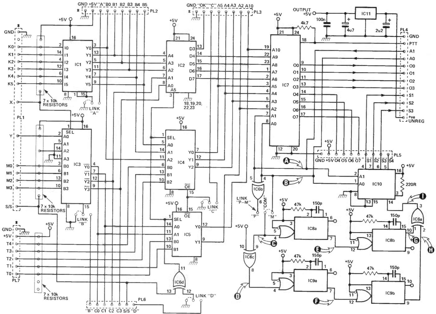
Figure 2: Synthesizer Control circuit diagram.
