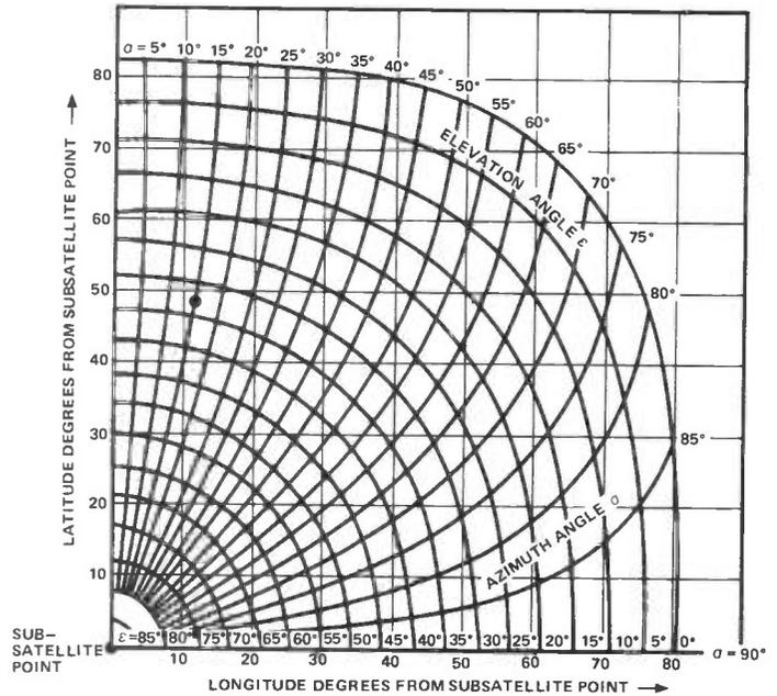
Figure 2: Azimuth and elevation angles can be taken from this diagram.
