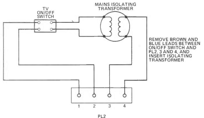
Figure 5. The TV on/off switch can be used to supply the isolating transformer.
