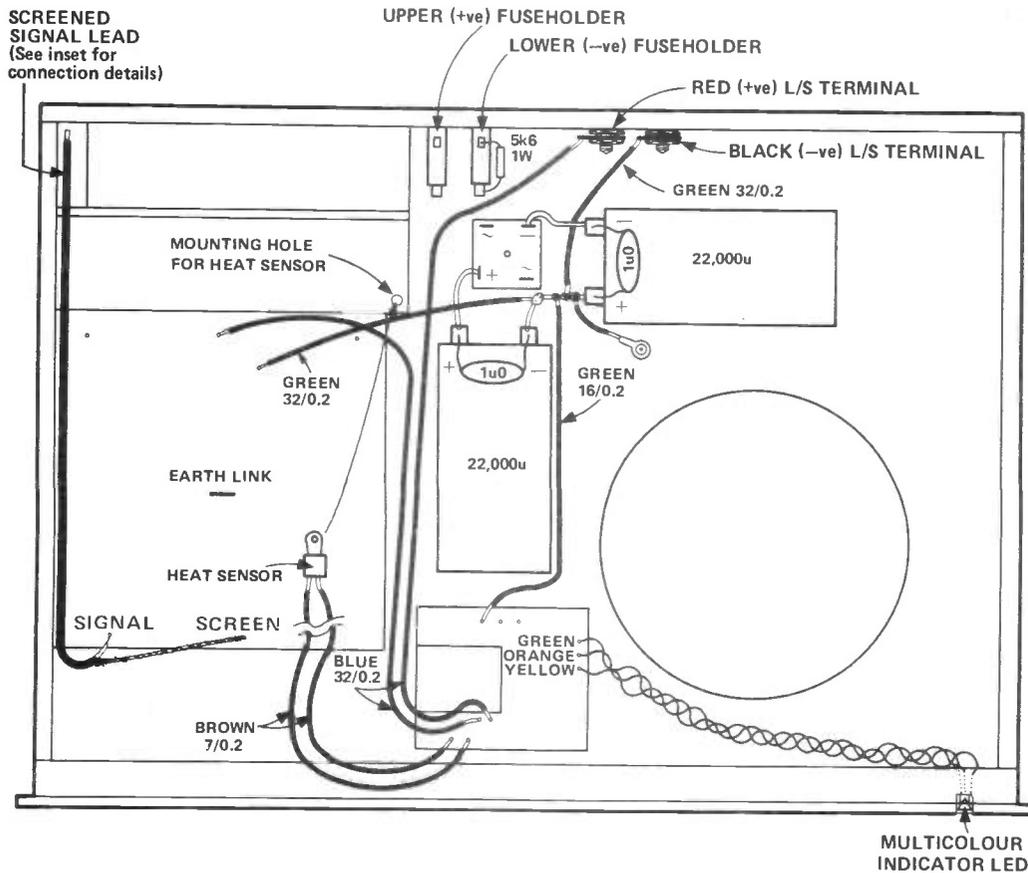
Figure 6: Main amplifier signal wiring. ▶
