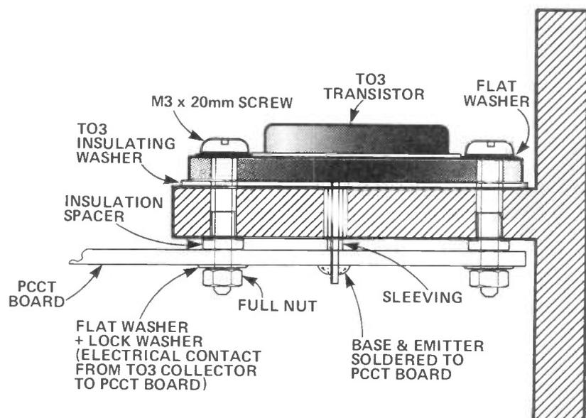
Figure 1: Heatsink bracket section showing power transistor mounting.
