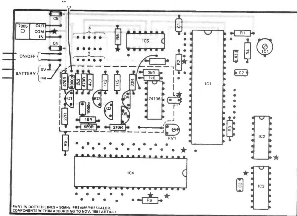
Figure 8a. Component placing on the double sided PCB.
