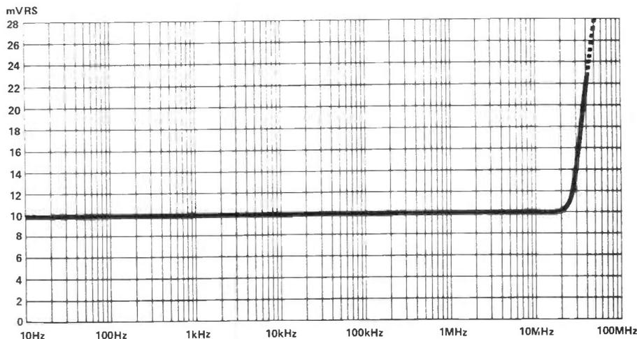
Figure 2: Sensitivity versus frequency—sinusoidal input.
