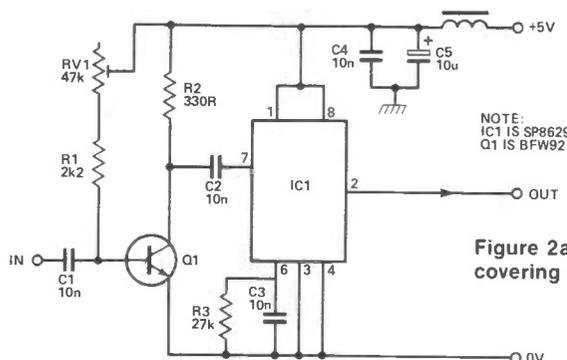
Figure 2a. One of the preamp/prescalers covering the 200MHz range.
