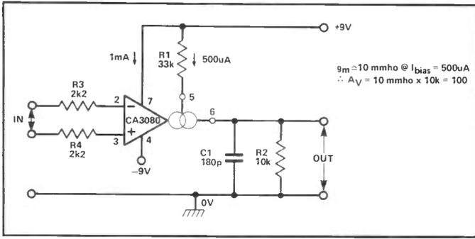
Figure 6. Differential amplifier with 40dB voltage gain.
