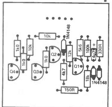
Foil pattern and component overlay for 500kHz pre-amplifier
