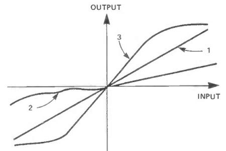
Figure 1. Curves representing the three different component types. Number 1 is for linear components (eg, resistors), number 2 for polarity sensitive components (eg, electrolytic capacitors) and number 3 represents non-linear devices such as op-amps.
