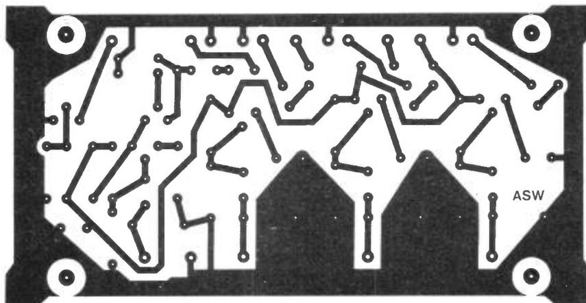
Figure 7b. Foilside of the above PCB overlay.
