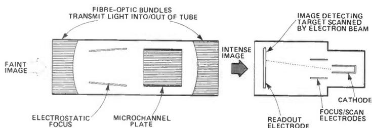
Figure 5. Microchannel plate and Vidicon for focussing and detecting images.
