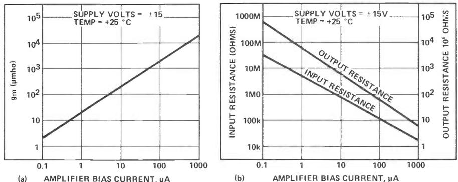
**Figure 5.** The transconductance (a) and the input and output resistances (b) of the CA3080 vary with the bias current value.
