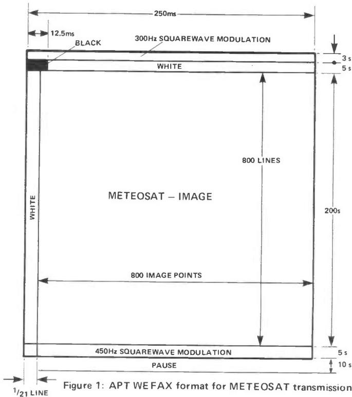
Figure 1: APT WEFAX format for METEOSAT transmissions.
