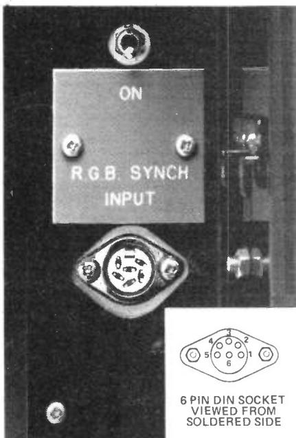
A small panel is fitted below the on/off switch. The inset gives pin designations for the DIN socket.
