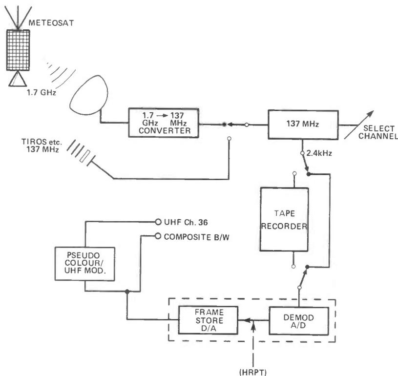
Figure 4: A complete METEOSAT ground station system.
