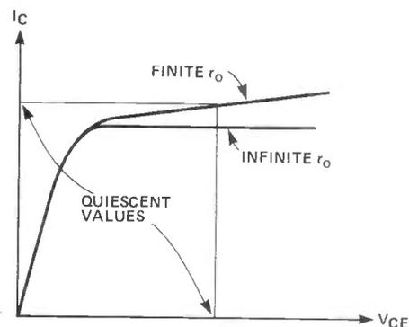
Figure 4. Graph showing the  $I_c/V_{CE}$  characteristics is modelled by  $R_o$ .
