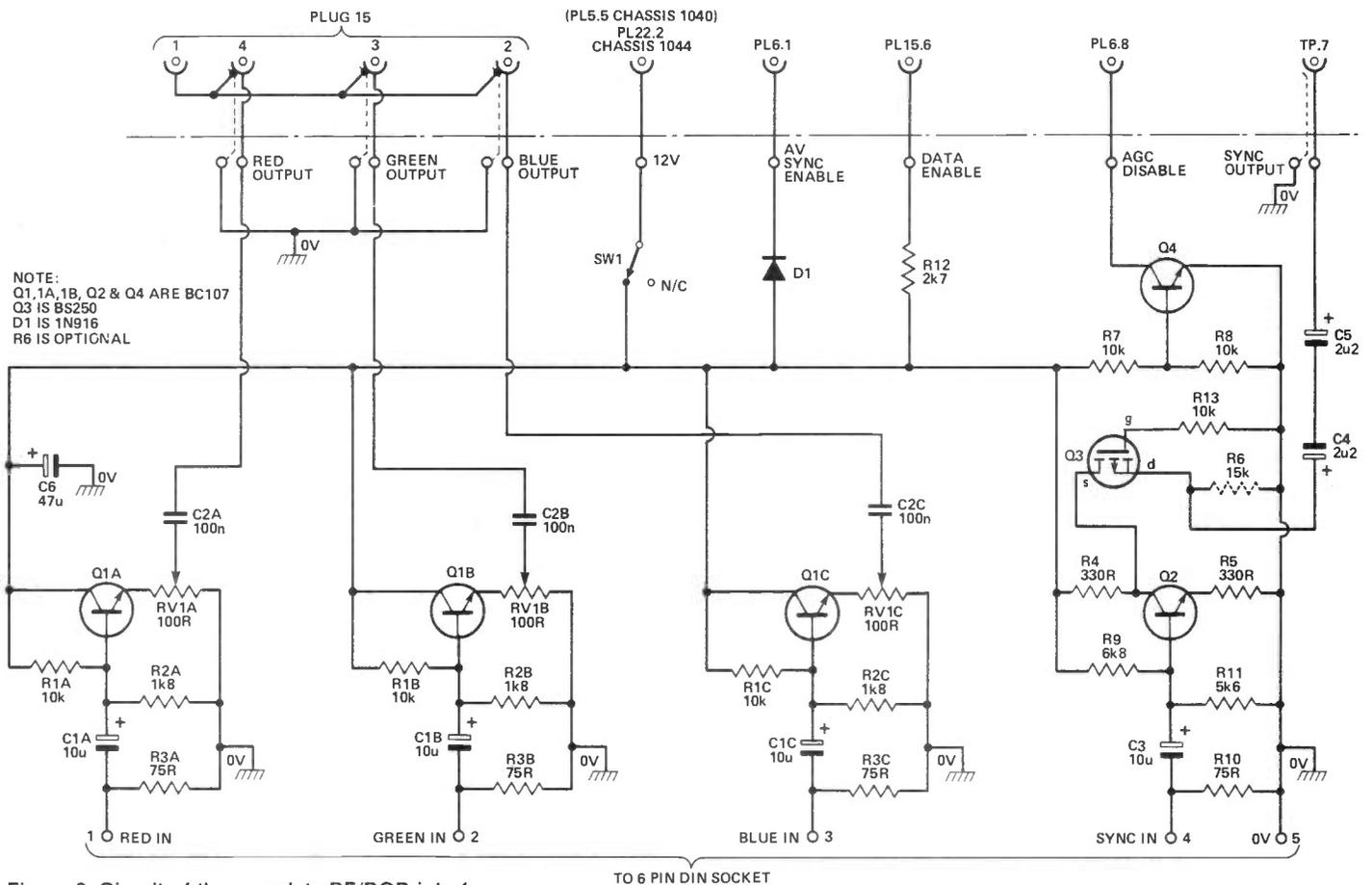
Figure 2. Circuit of the complete RF/RGB interface.
