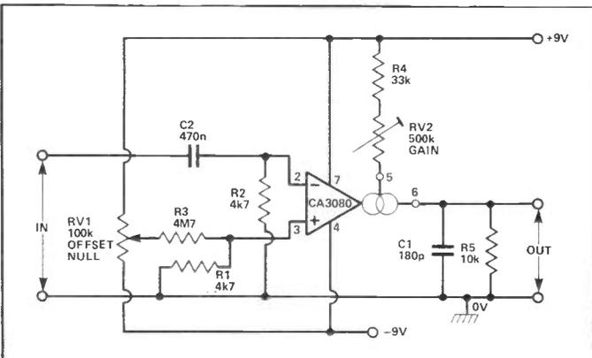
Figure 8. Variable-gain (x5 to x100) AC amplifier.
