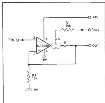
Figure 12. Programmable Schmitt trigger.
