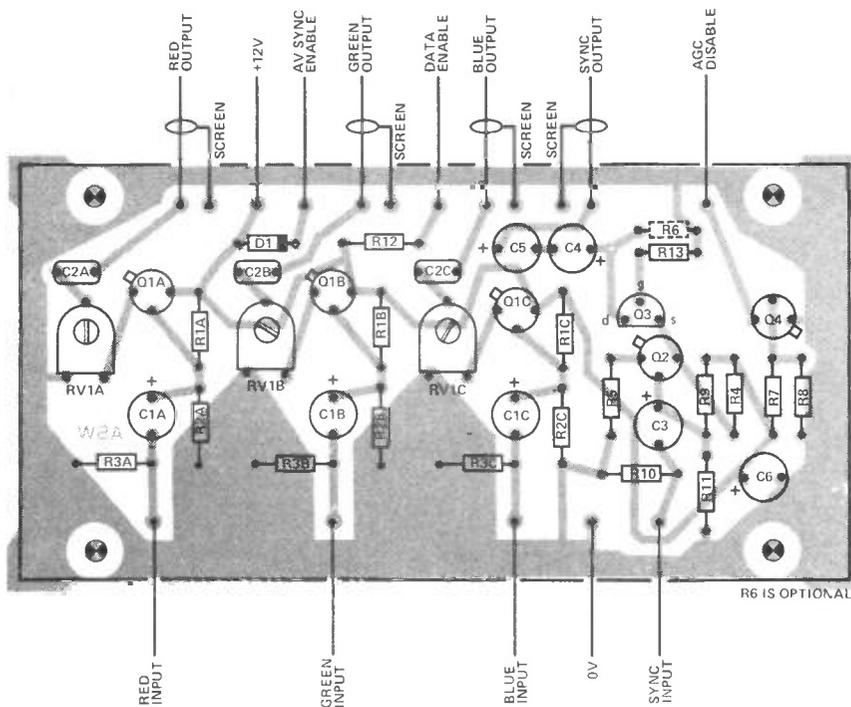
Figure 7a. Component overlay of the completed PCB.
