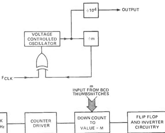
Figure 9. Basic frequency synthesiser and down-counter block.
