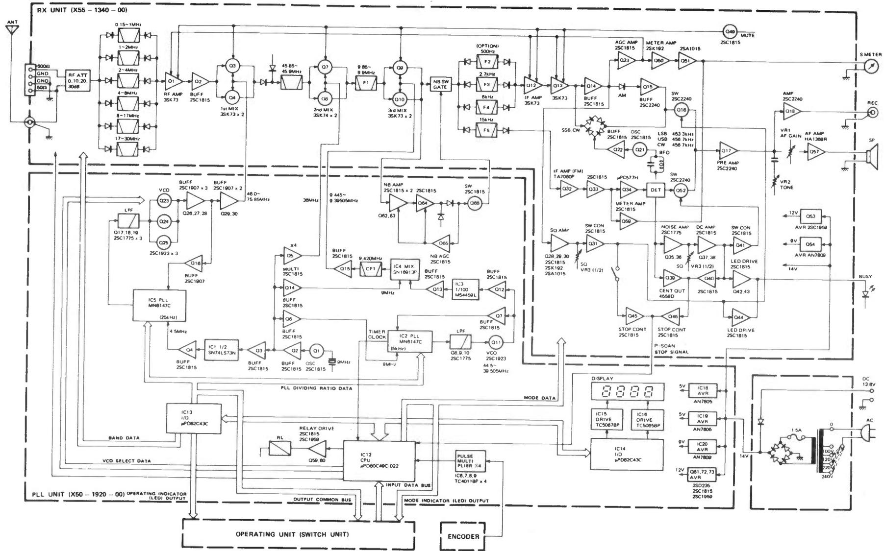
Figure 1: Block diagram of the R2000, showing both the HF and PLL sections.
