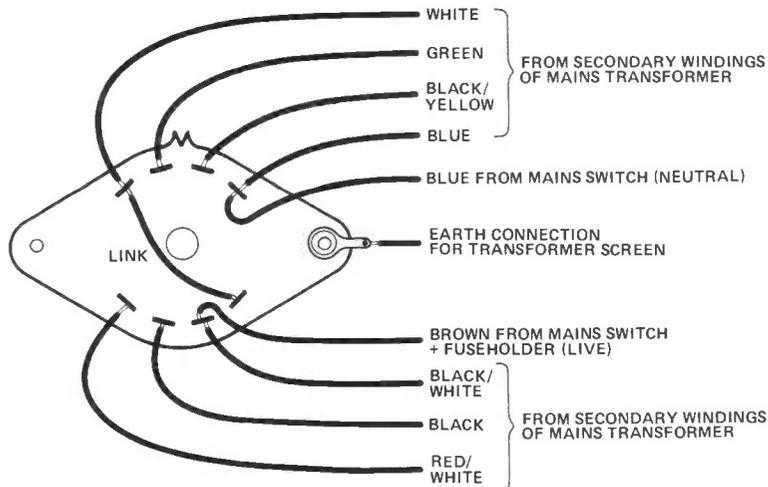
Figure 2: Rear view of voltage selector showing connections.
