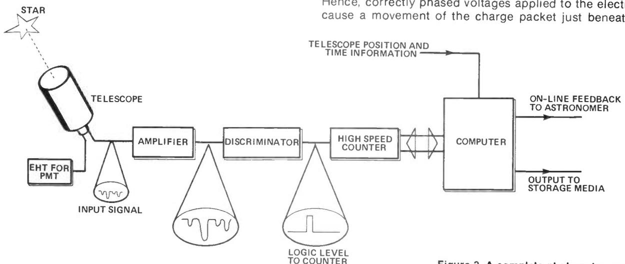
Figure 3. A complete photometry system.
