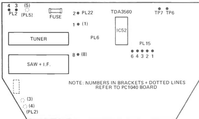
Figure 4. Connections on the TX9 printed boards.
