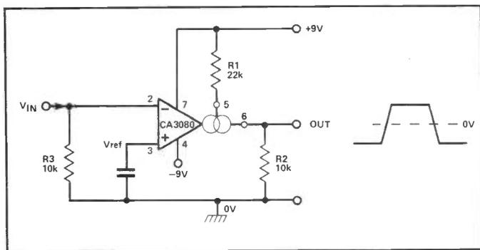
Figure 10. Fast inverting voltage comparator.
