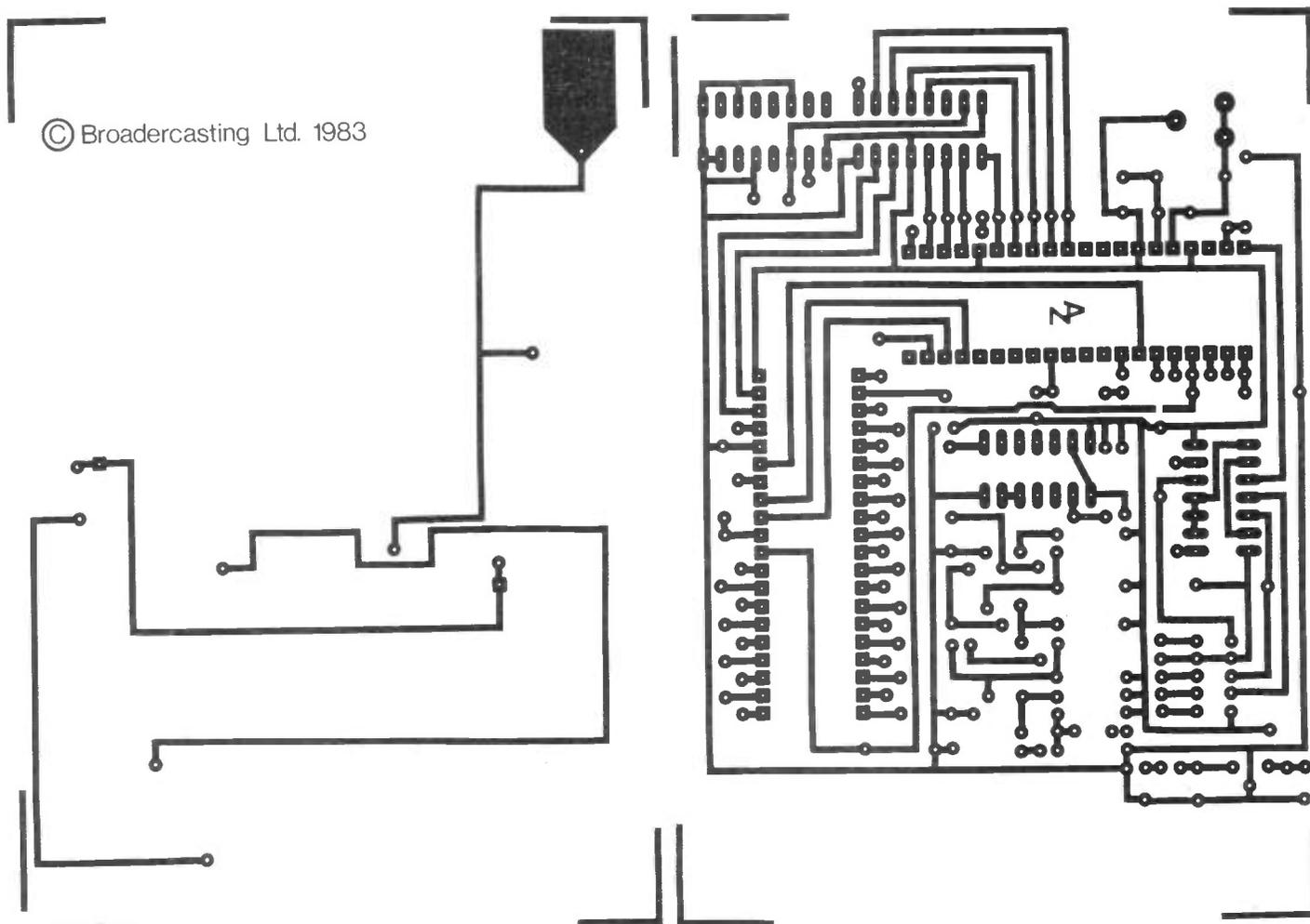
Figure 8b. The two sides of LCD-DFM board (includes pads for 50MHz prescaler).
