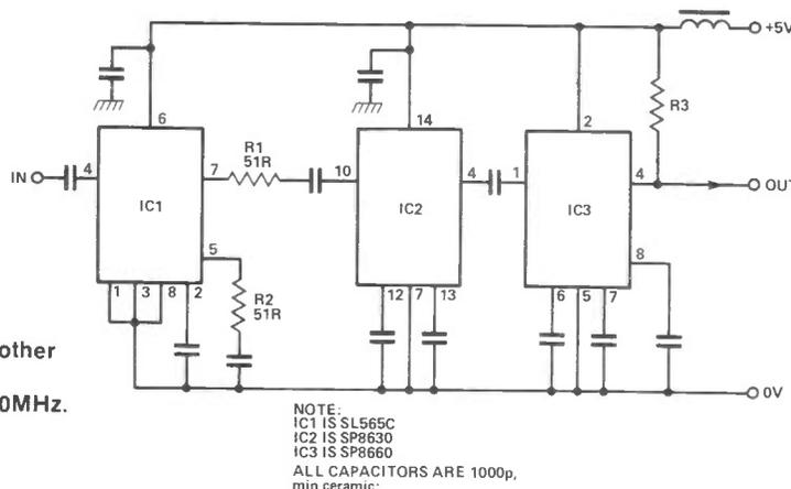
Figure 2b. The other prescaler, which operates up to 600MHz.
