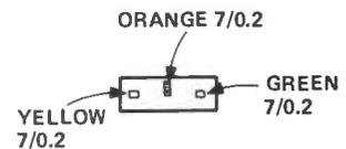
Figure 4: Rear view of indicator LED showing connections.
