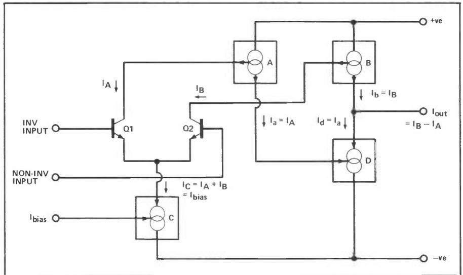
**Figure 4.** The CA3080 comprises one differential amplifier and four current mirrors.
