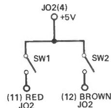
Figure 5: Switch wiring for 120 channel expansion.
