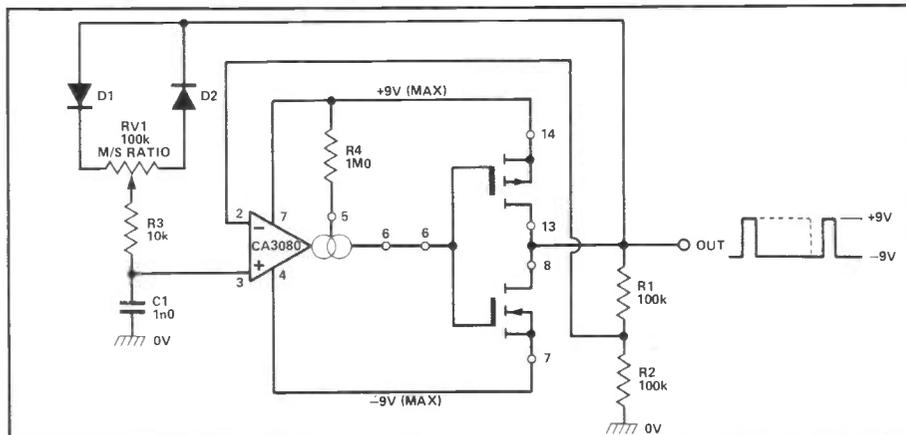
Figure 13. Variable mark-space ratio astable.
