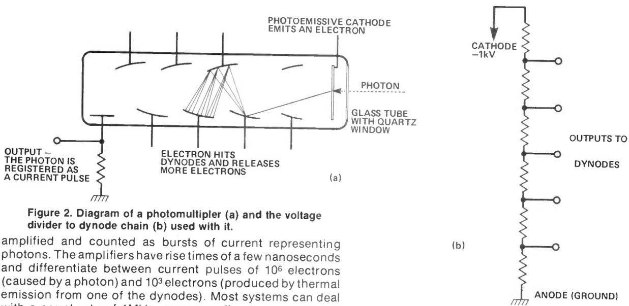
Figure 2. Diagram of a photomultiplier (a) and the voltage divider to dynode chain (b) used with it.
