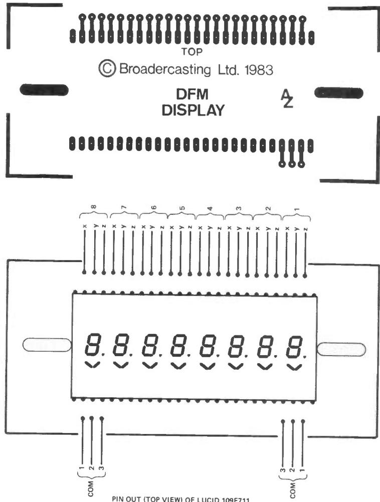
Figure 9. PCB foil pattern (above) and overlay (below) for the 8-digit display.
