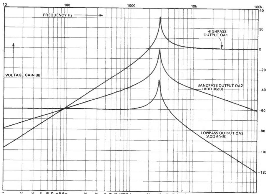
Figure 8. Plot of voltage gain against frequency for the figure 7 circuit.
