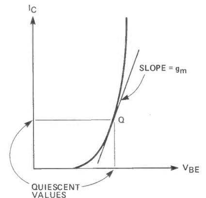
Figure 2. Finding the slope of the  $I_c$ - $V_{BE}$  characteristic at point Q.
