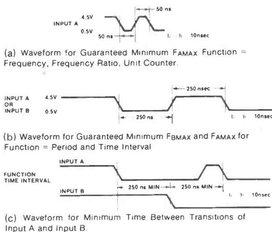
Figure 2. Waveforms for guaranteed minimum frequencies when used as a counter (a), tuner (b) and during AB transitions (c).
