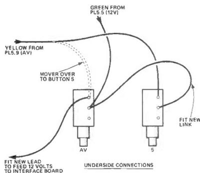
Figure 6. Alternative switching between RF and RGB using the AV button.
