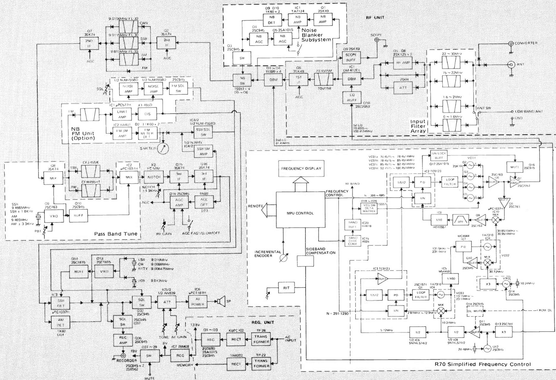
Figure 2: The Icom R70 block diagram, with the main areas highlighted.
