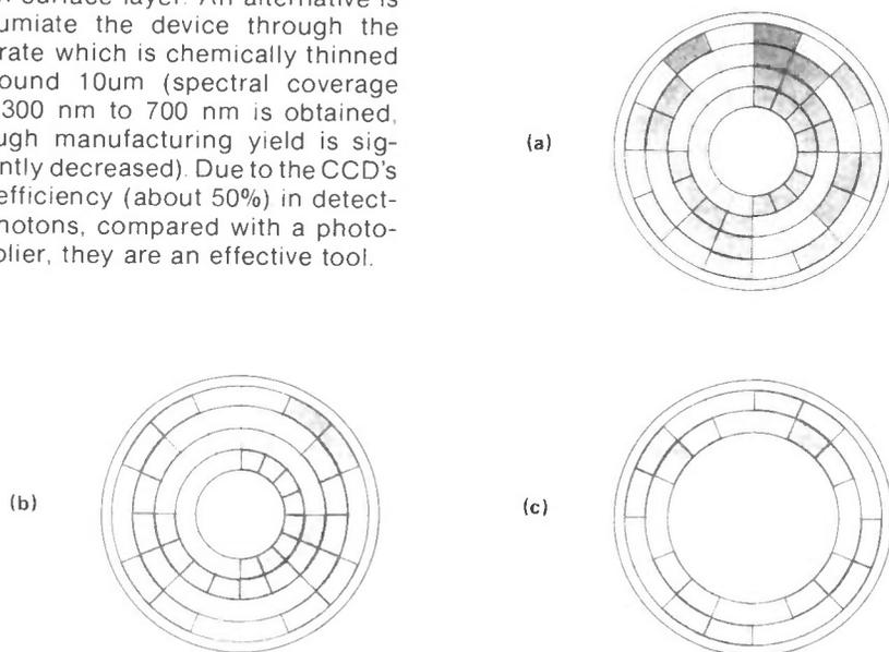
Figure 7. Digitising reference discs, absolute encoders for Binary (a) and Gray codes (b) and an incremental system (c) encoder disc.
