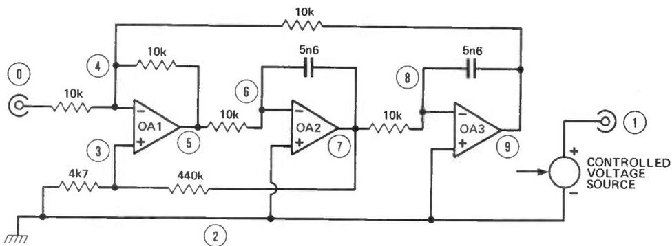
Figure 7. State variable bandpass filter circuit.
