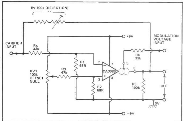
Figure 9. Ring modulator or 4-quadrant multiplier.
