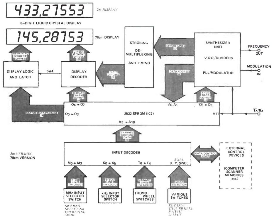
Figure 1: Synthesizer Control block diagram.
