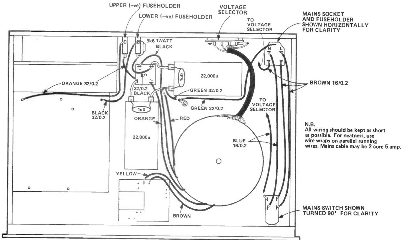
Figure 5: Main amplifier power supply wiring.
