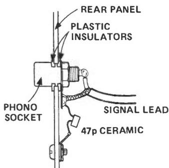
Figure 3: Rear panel section showing phono socket and plastic insulators.
