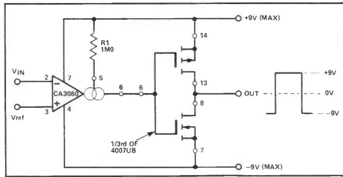
Figure 11. Non-inverting micro-power voltage comparator.
