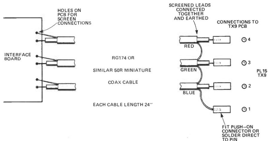
Figure 3. Wiring the interface to the TX9 PCB.
