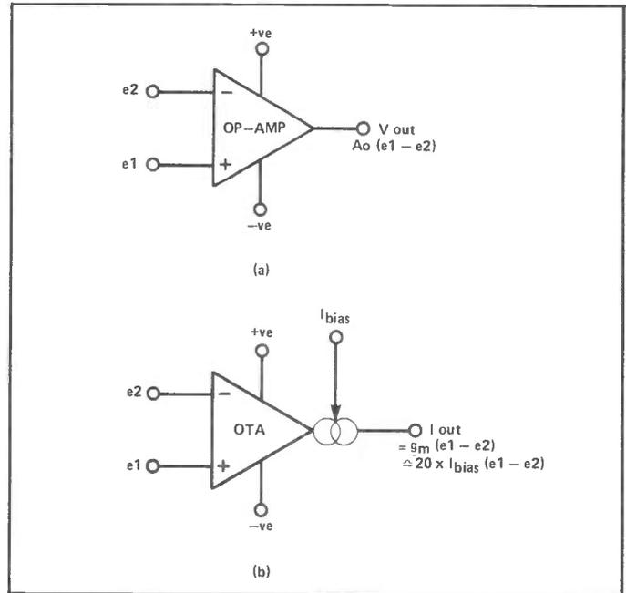
**Figure 1. A conventional op-amp (a) is a fixed-gain voltage-amplifying device. An OTA (b) is a variable-gain voltage-to-current amplifier.**
