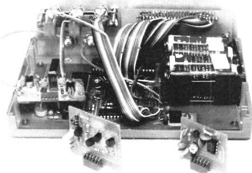
The completed Digital Frequency Meter, as viewed from behind the display. The two boards in the foreground are the 200MHz and 600MHz prescalers.
