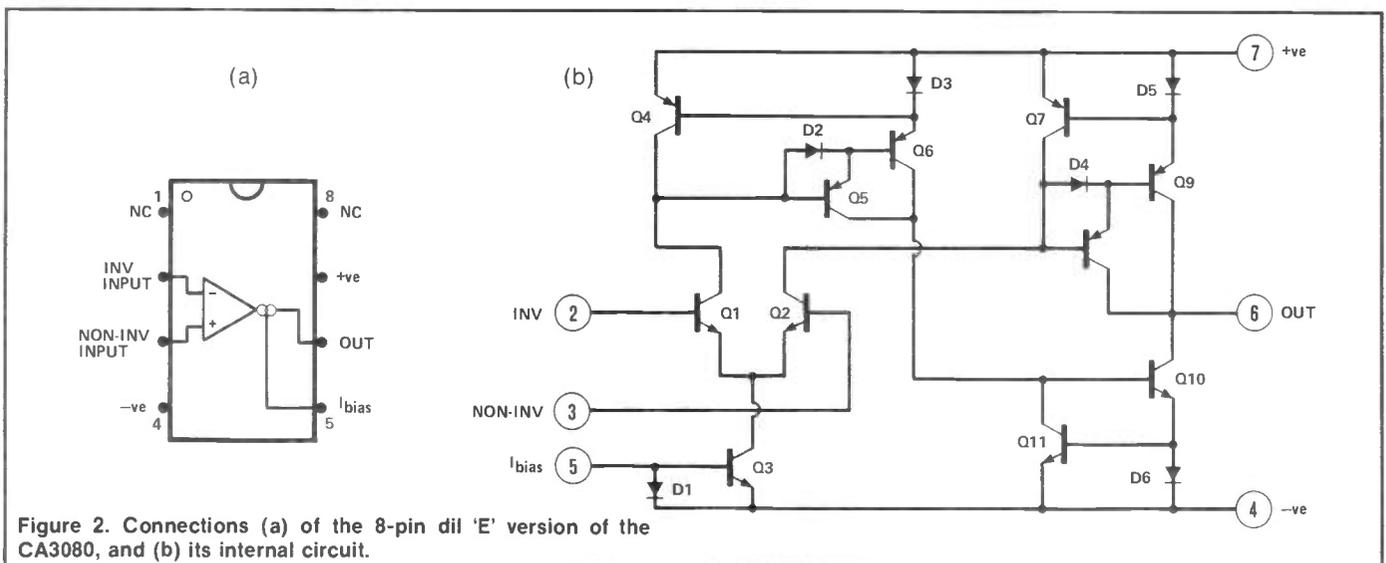
**Figure 2. Connections (a) of the 8-pin dil 'E' version of the CA3080, and (b) its internal circuit.**
