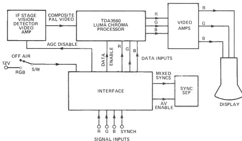
Figure 1. Block diagram showing connections for the interface.
