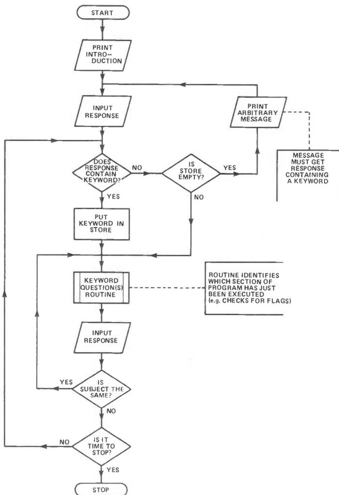
Figure 1. Flowchart reflecting the structural basis of programs which respond to questions using a key word searching routine.
