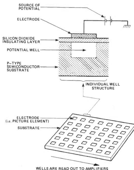
Figure 6. The CCD imaging array, with one cell enlarged to show electrode connections.
