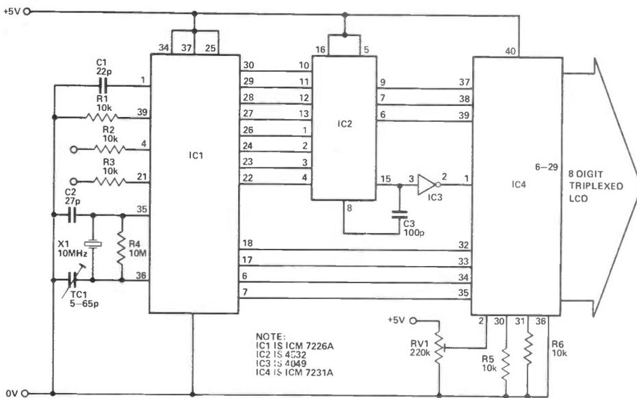
Figure 7a. Main circuit of the LCD-DFM.
