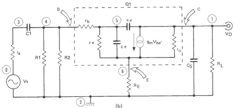
Figure 3. A single transistor amplifier (a) and the linear model (b) which represents it.
