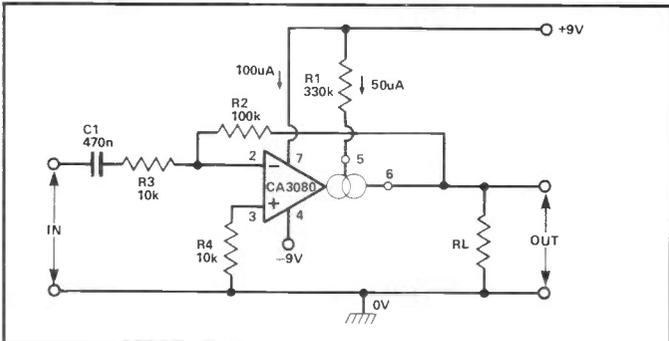
Figure 7. 20dB micro-power inverting amplifier.
