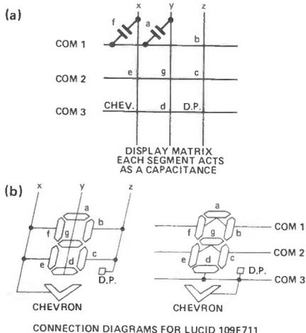
Figure 1. Display wiring as represented by a cross-matrix (a) and the actual segments (b).
