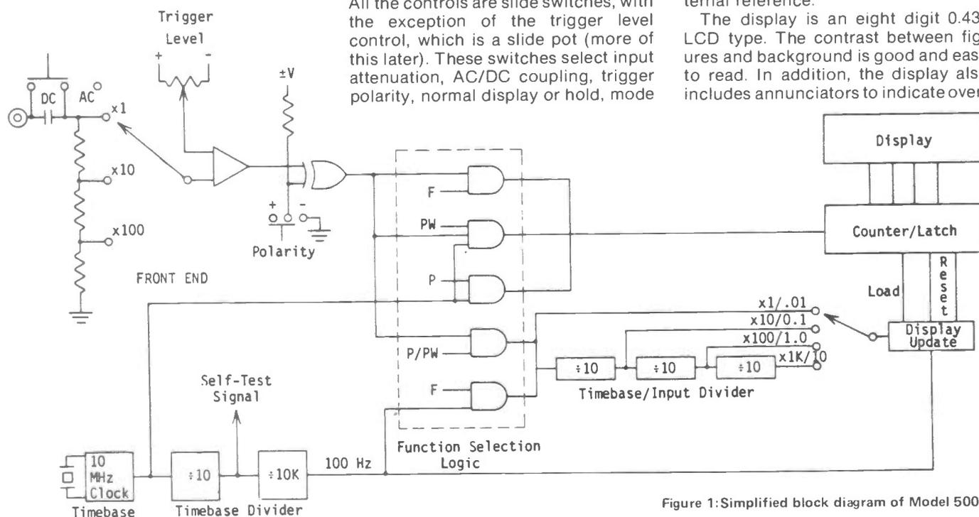
Figure 1: Simplified block diagram of Model 5000.
