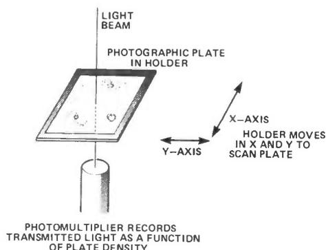
Figure 4. Representation of a scanning densitometer.
