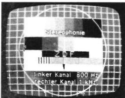
Figure 1: West German FuBK test card carrying a stereo TV sound test transmission.
