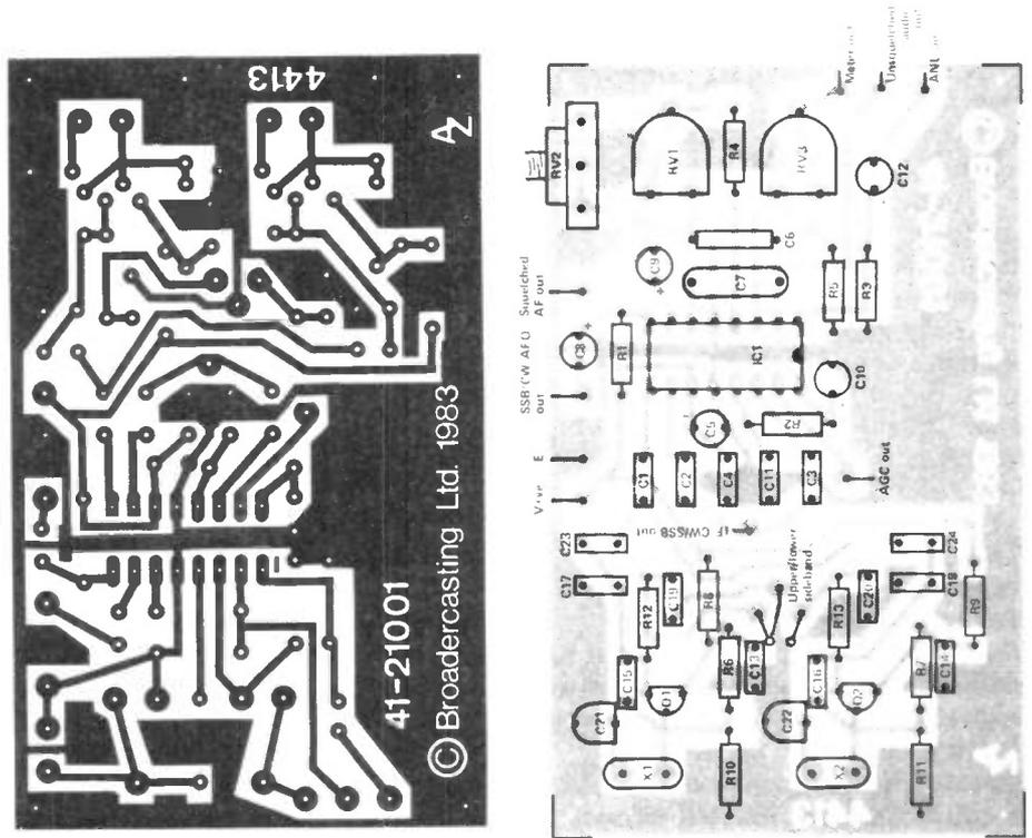
Figure 5: KB4413 Detector block PC foil and overlay
