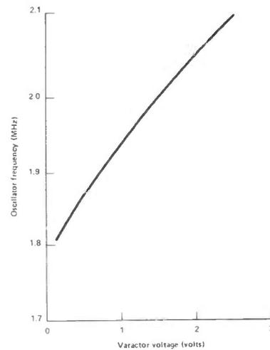
Figure 12: Voltage/frequency relation for a varactor controlled oscillator.
