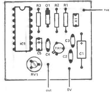
Figure 6: Component overlay for 4020-based toneburst.
