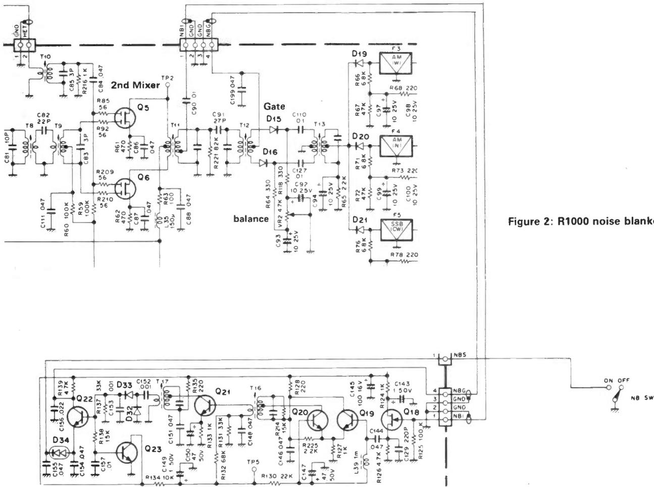
Figure 2: R1000 noise blanker circuitry.
