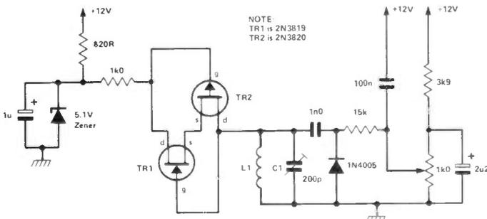
Figure 11: Varactor controlled oscillator incorporating a Lambda diode.
