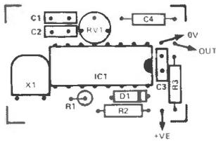
Figure 4: Component placing on the tone-burst board.
