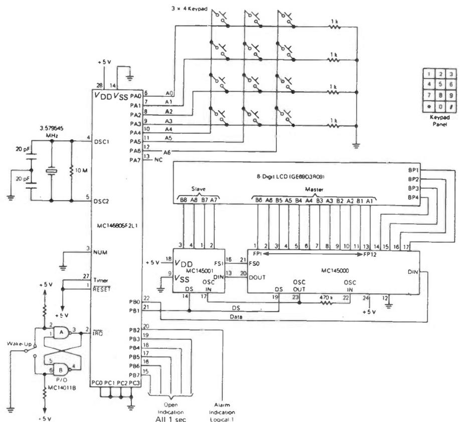
Figure 4: Digital lock system schematic diagram.
