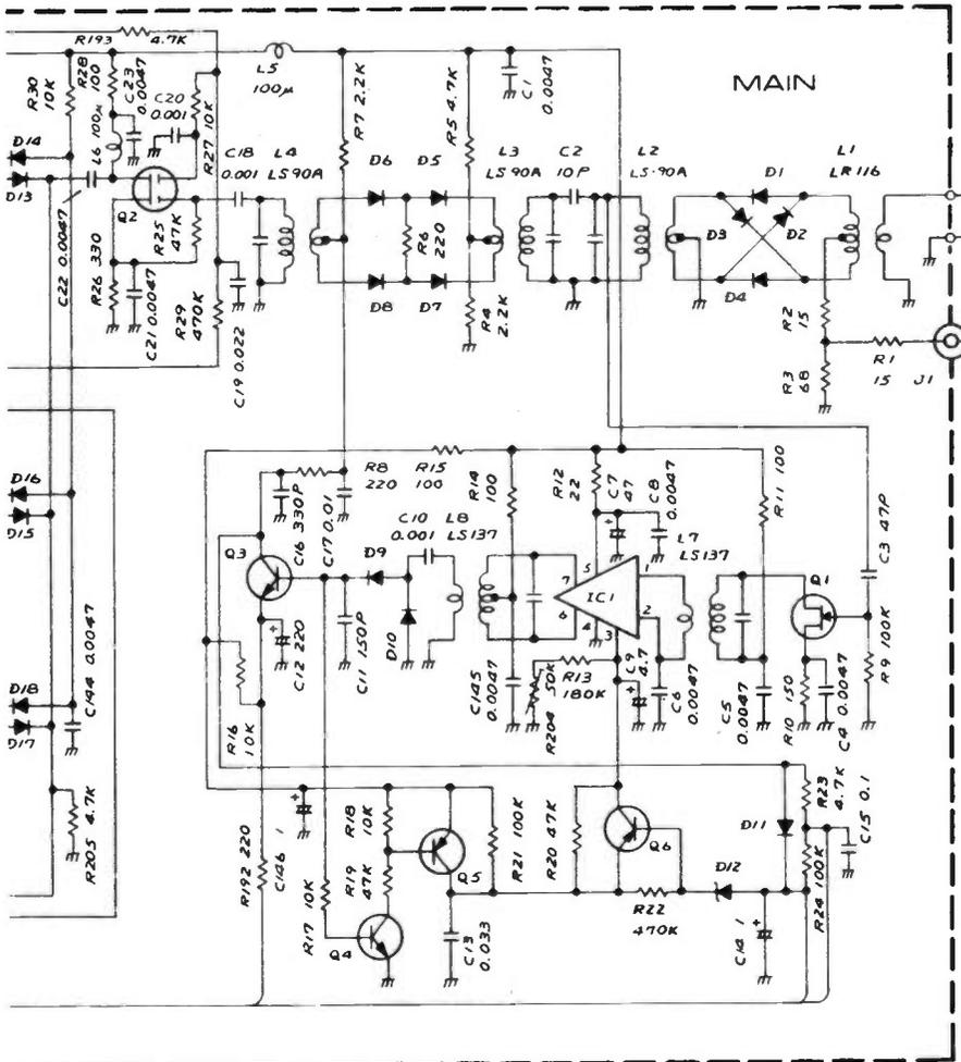
designer has discovered (like we all do) that an uncoupled noise blanker can actually introduce more noise than it removes. The emitter of Q3 is also heavily decoupled via C12, since this comparatively long lead would provide an excellent additional noise source if given the chance.
