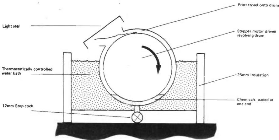
Figure 2: Side view of drum and trough.
