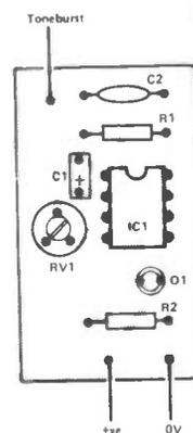
Figure 4: Component overlay for LM3909-based toneburst.
