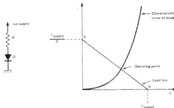
Figure 5: Determining the operating point of a resistor/diode circuit.
