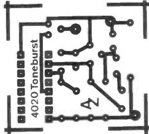
Figure 5: PCB for 4020-based toneburst.
