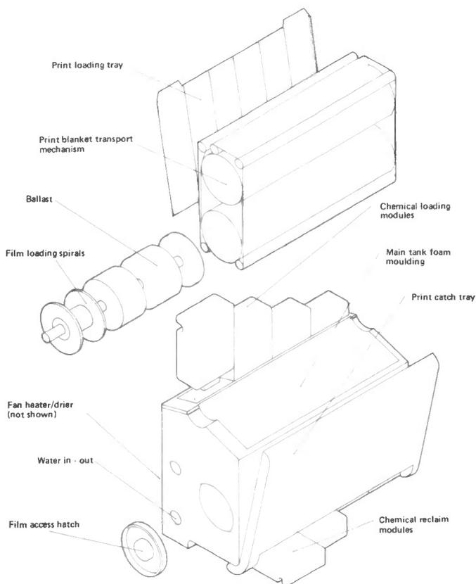
Figure 4: Component layout — exploded view.
