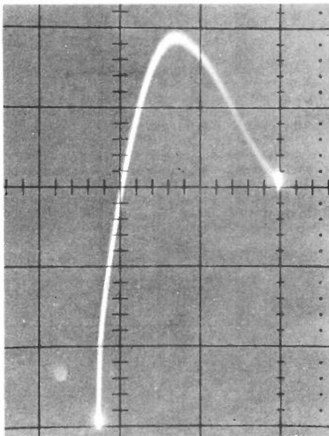
Photo 1: Oscillograph of Lambda Diode characteristic curve as obtained from a curve tracer. 1mA/division in  $\gamma$ ; 2V/division in  $x$
