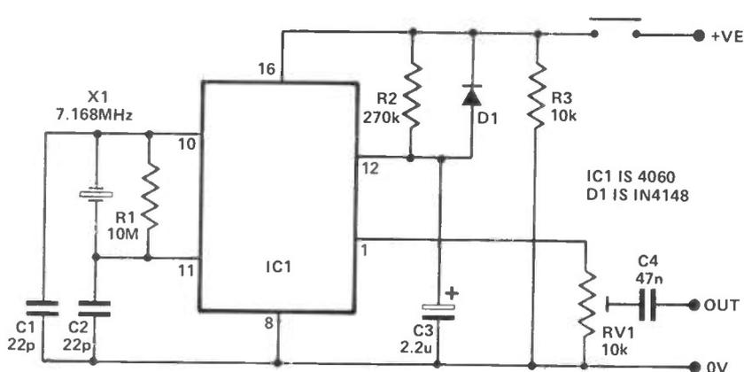
Figure 3: Circuit for the toneburst generator.
