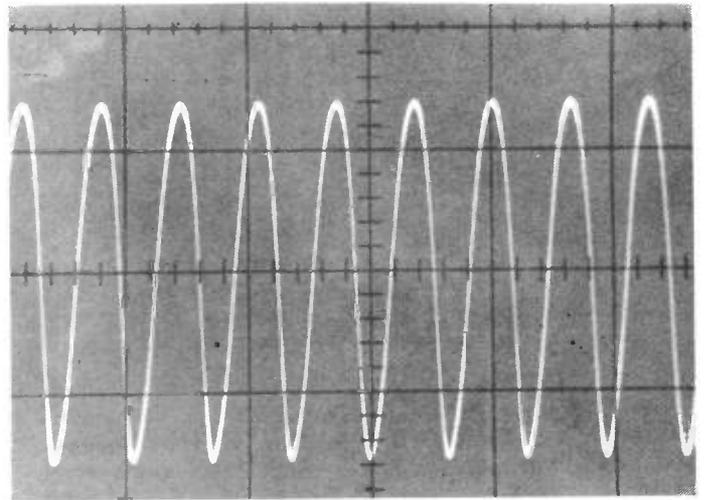
Photo 3: Oscillograph of VFO output. 100nsec/div in x; 0.2 volts/div in y.
