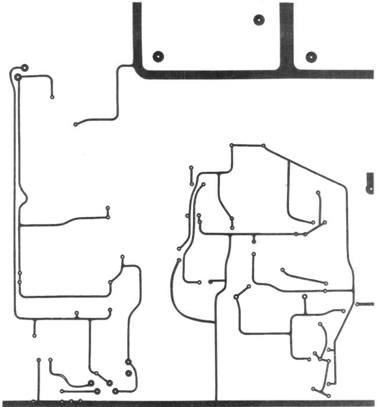
Figure 3b: PCB foil pattern for main motherboard. Top plane.
