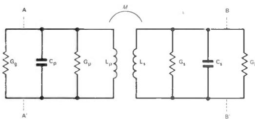
Figure 8: Equivalent circuit for a double-tuned band filter.
