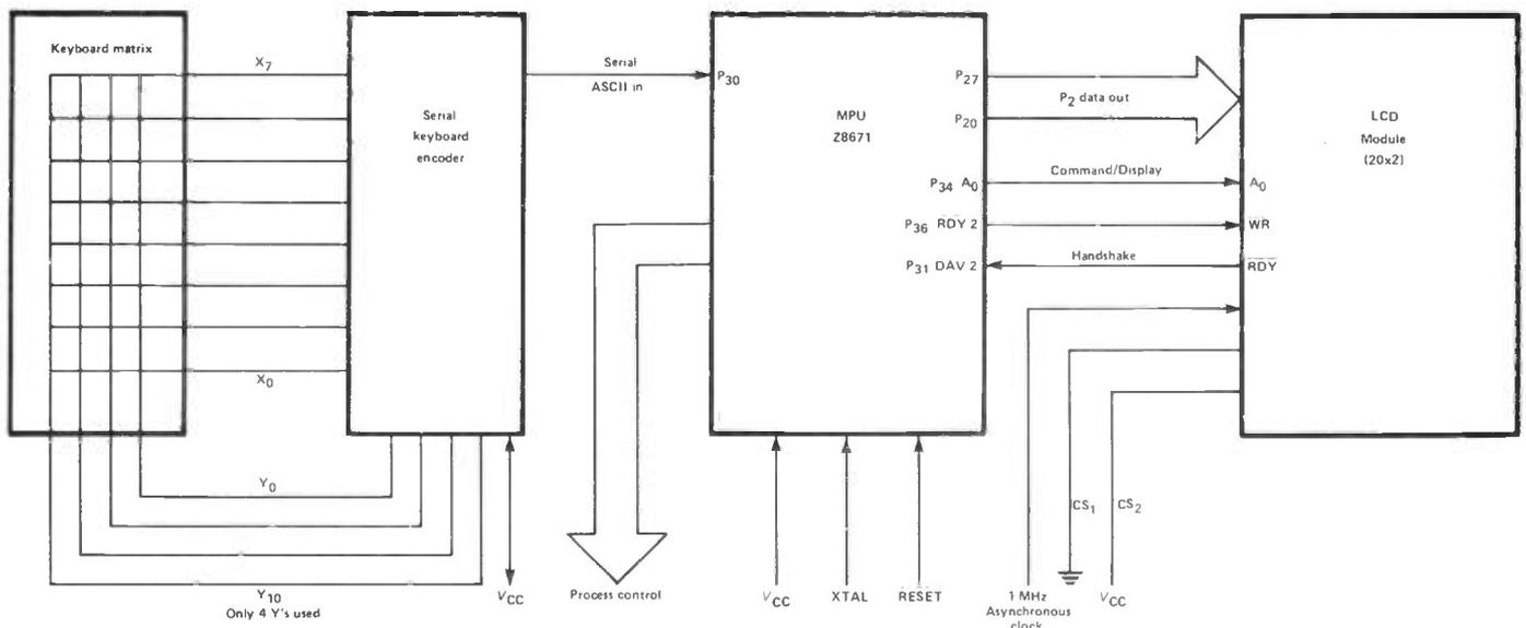
Figure 8: Block circuit diagram of keyboard, Z8 and LCD interface.
