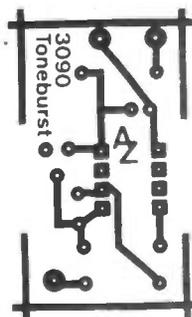
Figure 3: PCB for LM3909-based toneburst.
