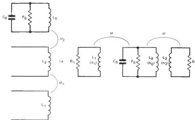
Figure 4: Equivalent circuit for a single-tuned band filter.
