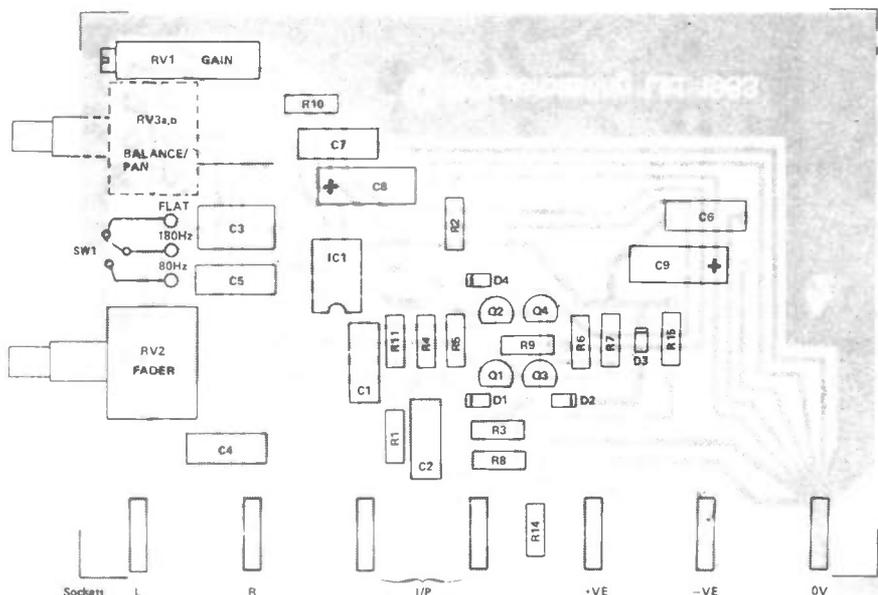
Figure 2: Component overlay for input amplifier.
