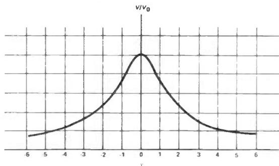
Figure 6: Amplitude-frequency characteristic for a single-tuned band filter.
