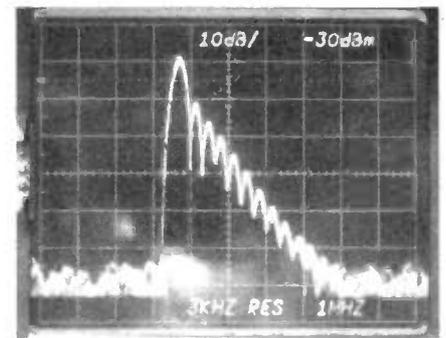
Photo 2: Spectrum analyser is used to demonstrate the effect of a filter being activated by a pulse with a rise time greater than the filter bandwidth can handle.
