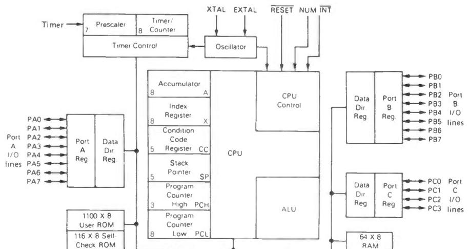
Figure 2: MC6805P2 HMOS microcomputer block diagram.
