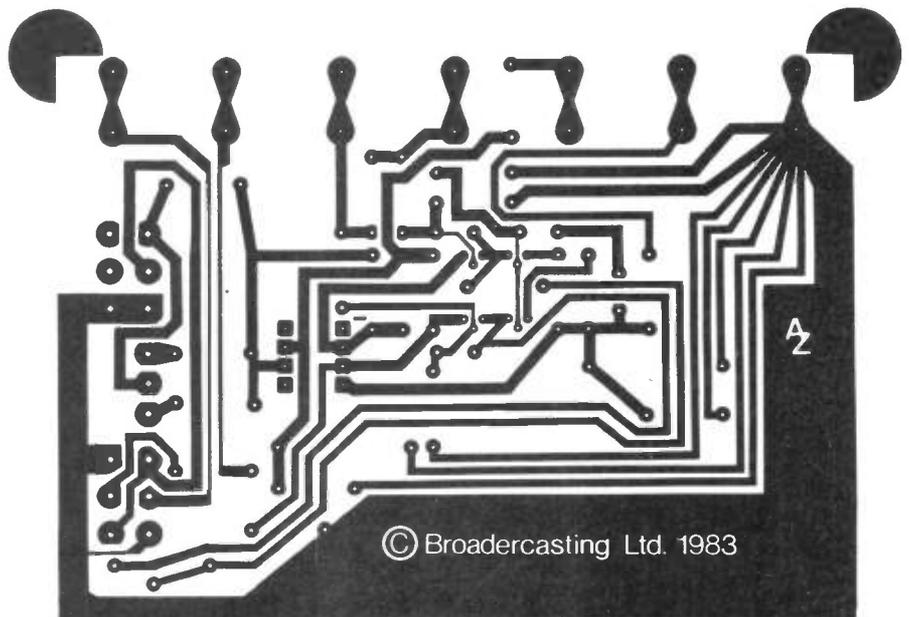
Figure 1: Foil pattern for input amplifier PCB.
