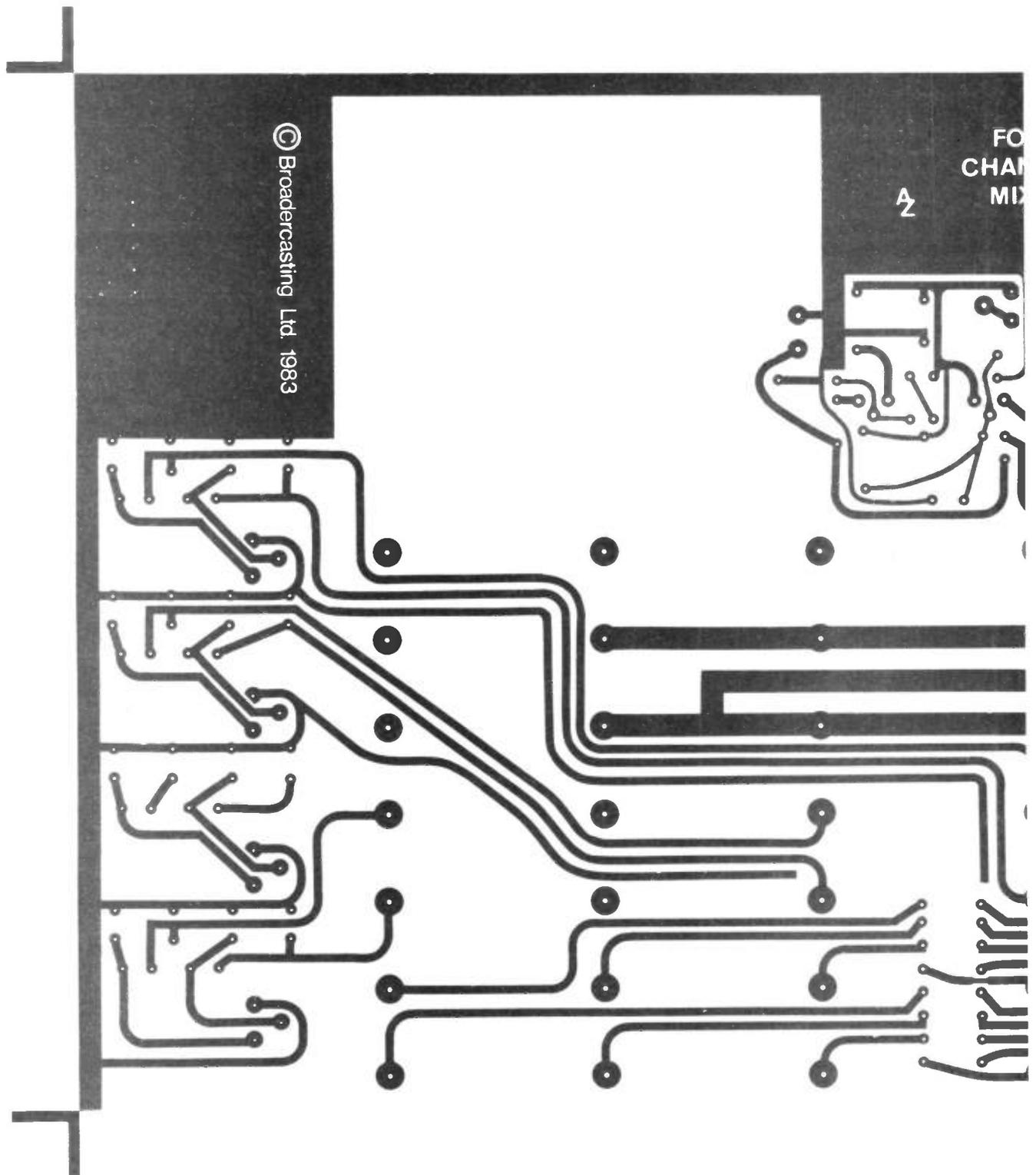
Figure 3a: PCB foil pattern for main motherboard. Bottom plane.
