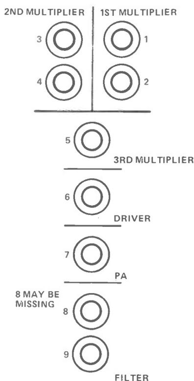
Figure 2: The transmitter tuning coils.
