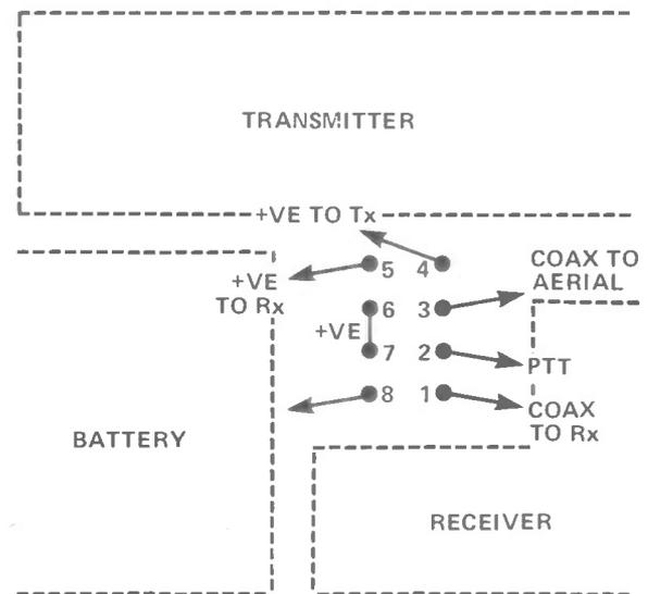
Figure 1: Connections from the relay (looking from PCB side).
