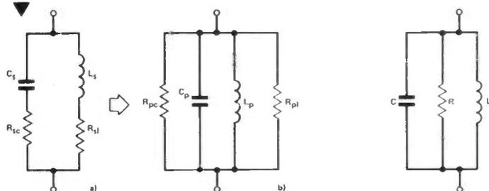
Figure 2: Equivalent circuit based on the coil constants. ▲
