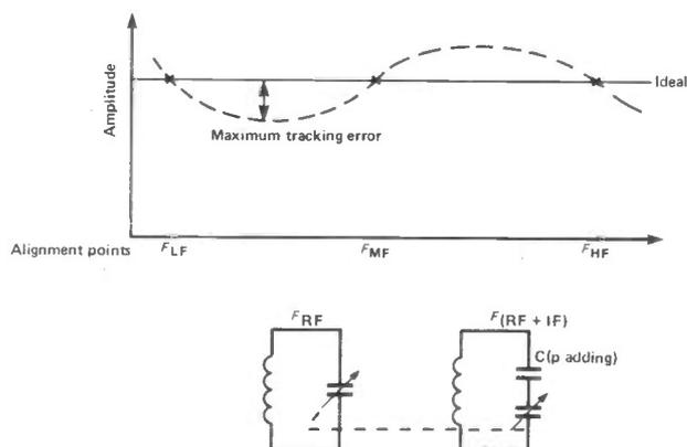
**Figure 1: The classic '3 point tracking' compromise for making the best of the inevitable difference between the resonant frequencies of an antenna and an oscillator coil.**
