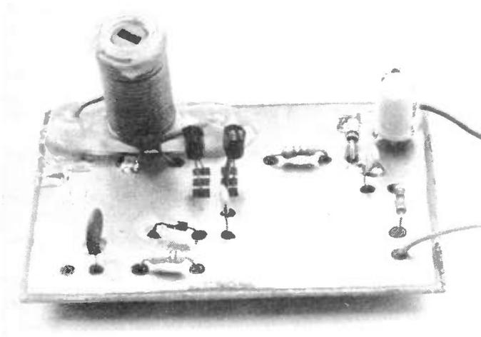
Photo 2: 15MHz variable frequency oscillator (VFO) incorporating a Lambda Diode
