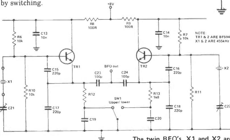
The twin BFO's. X1 and X2 are CRM455 resonators
