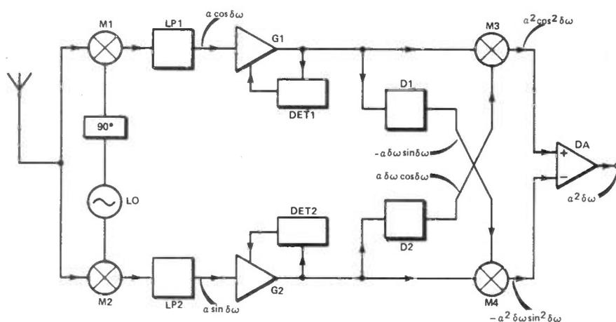
Figure 2: STC's suggested approach to coil-less FM radio.
