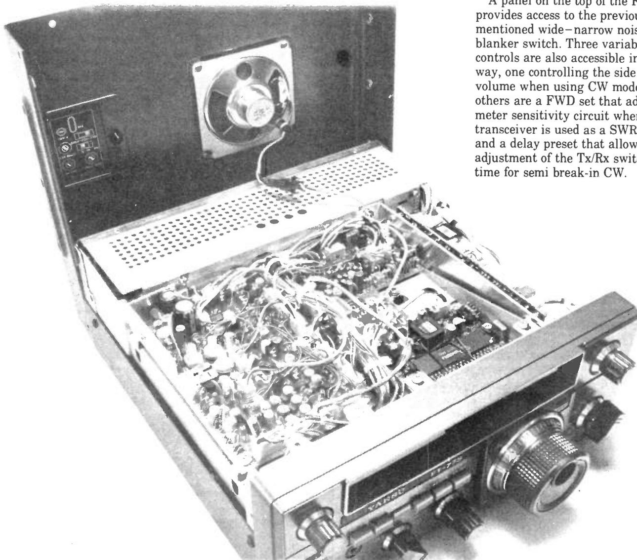
The fixed frequency crystal holder is also under the top access panel, and this is provided with a preset trimmer to allow accurate frequency selection. It should be noted that the fixed frequency crystal is selected within the VFO range of 5–5.5MHz and therefore provides a spot frequency in each band that is selected.
