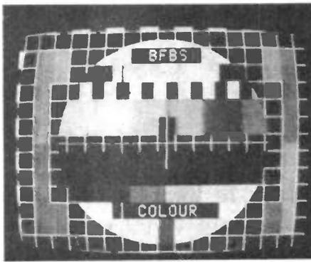
Figure 3: The standard PM5544 radiated by the BFBS in West Germany. Photo courtesy of Juergen Klassen (Berlin).
