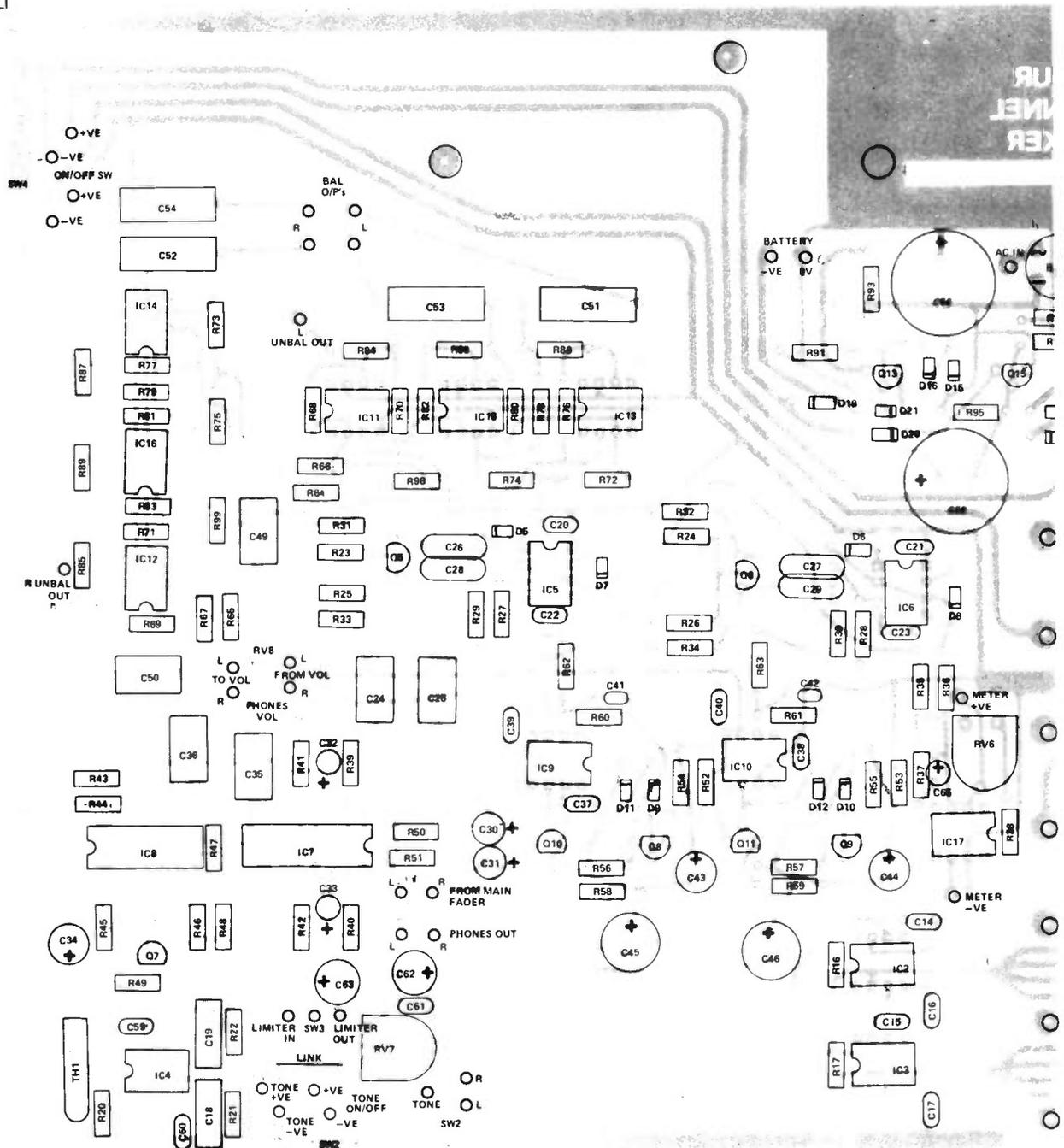
Figure 4: Mixer motherboard component overlay.
