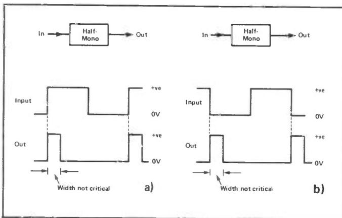
**Figure 1:** A 'half-mono' circuit may be used to detect a) the leading or b) the trailing edge of an input waveform.
