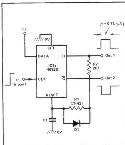
Figure 15: 'D'-type flip-flop used as a monostable.
