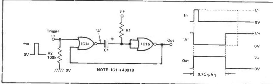
Figure 11: 2-gate NOR monostable is triggered by a positive-going signal and generates a positive-going output pulse.
