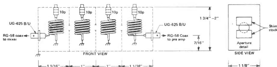
Figure 6: Bandpass filter. NB: Mount the BNC connectors near to the front.
