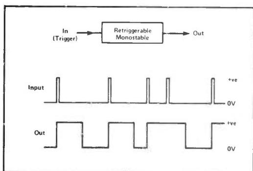
Figure 4: A retriggerable monostable starts a new timing cycle on the arrival of each new trigger signal.
