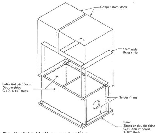
Figure 9: Details of shielded box construction.
