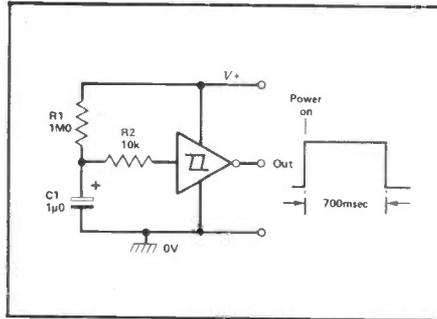
Figure 10: Power-on reset-pulse generator.
