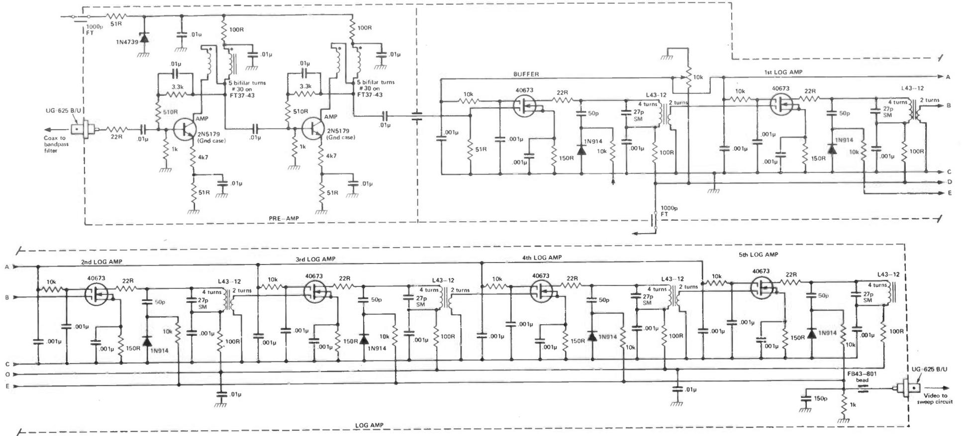
Figure 7: Circuitry of the pre-amp and the log amp.
