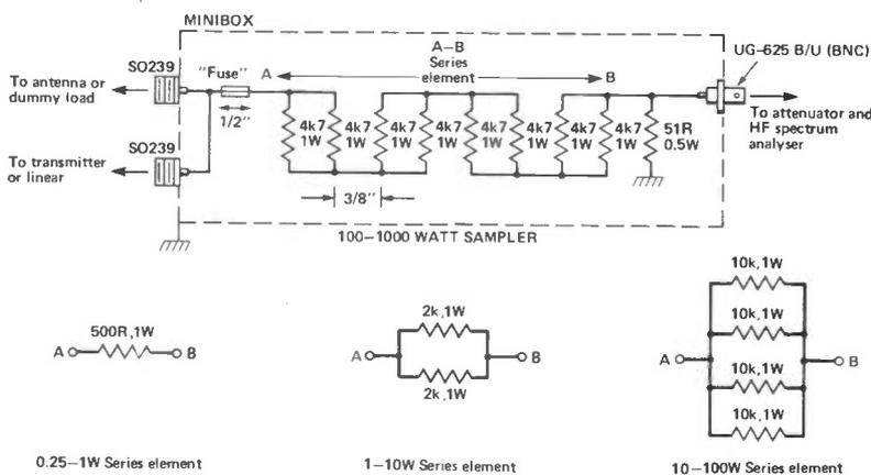
Figure 3: L-pad sampler. Always test run the sampler before connecting it to the attenuator.
