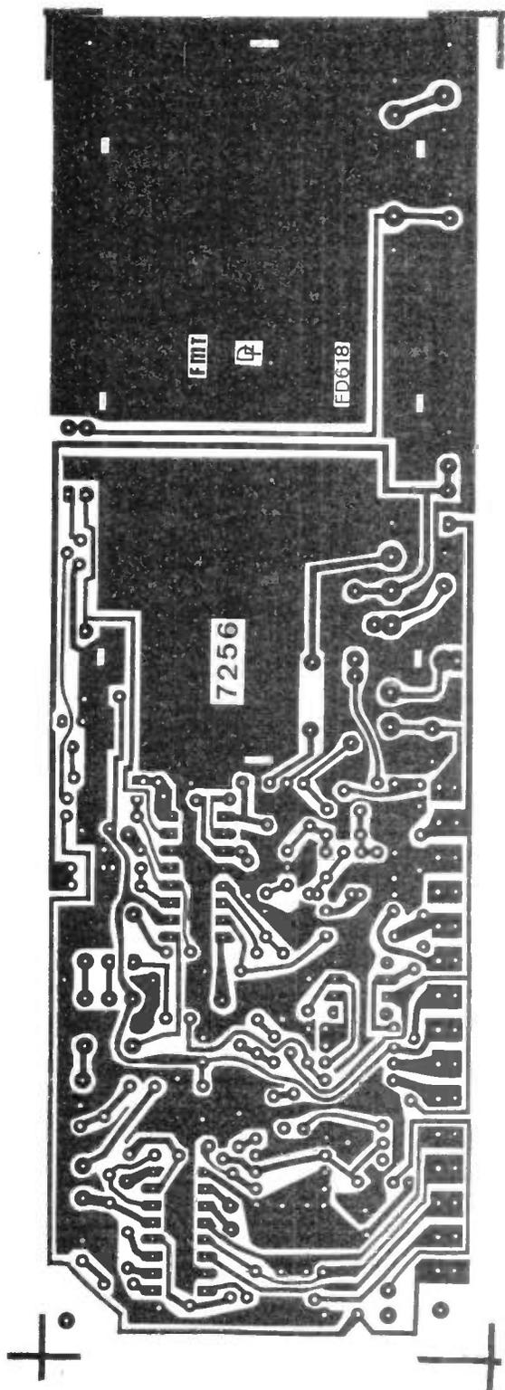
Figure 2b: PCB pattern for the underside.
