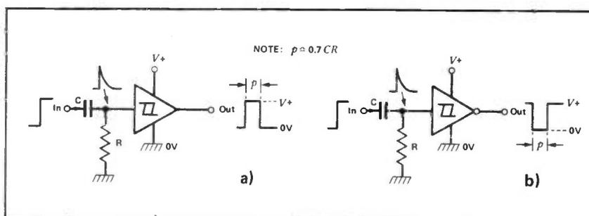
Figure 7: Leading-edge detector circuits giving a) positive and b) negative output pulses.
