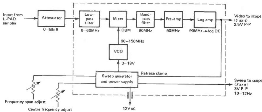
Figure 2: Block diagram.
