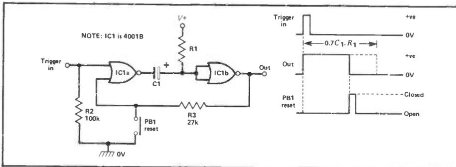
Figure 13: Resettable NOR-type monostable.
