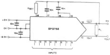
Figure 5: D/A set-up (negative output with respect to ground).
