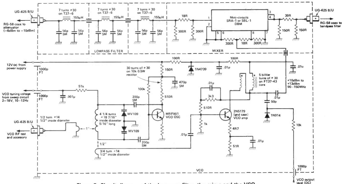
Figure 5: Circuit diagram of the low-pass filter, the mixer and the VCO.
