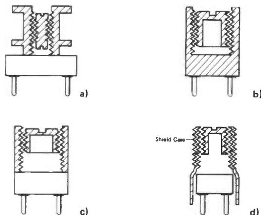
**Figure 2. Adjustable core structures.** a) Tapped bobbin for screw cores; b) Base with tapped section for cap core; c) Tapped section separate from base; d) Use of threaded shield case.
