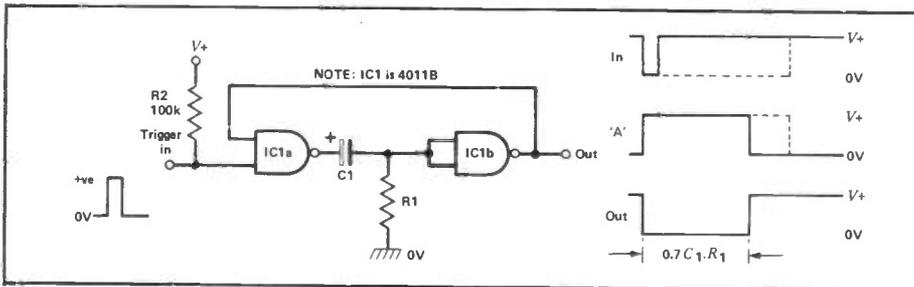
Figure 12: 2-gate NAND monostable is triggered by a negative-going signal and generates a negative-going output pulse.
