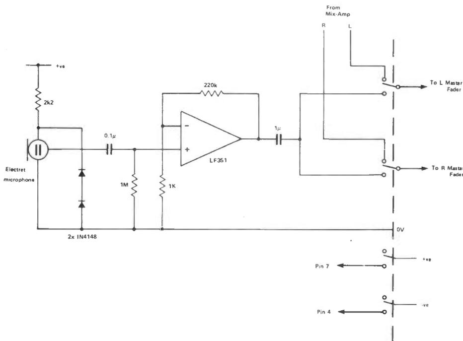
Figure 2: Slate microphone and amplifier.
