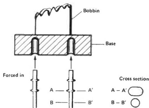
**Figure 3: Pin insertion.**
