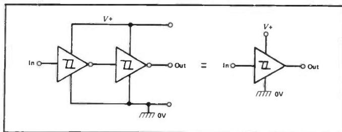
Figure 6: A non-inverting Schmitt can be made by wiring two inverting Schmitt elements in series.
