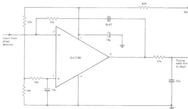
Figure 3: The CA3130 op-amp configured as an integrating filter.
