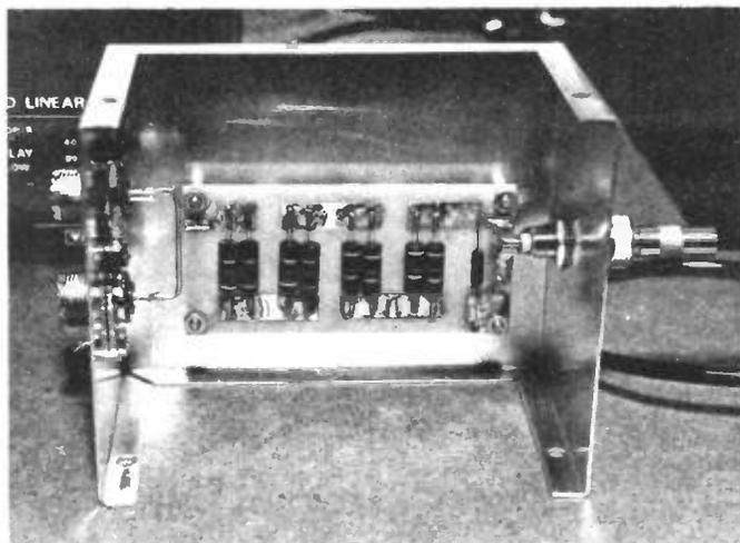
Photo 4: The L-pad sampler.
