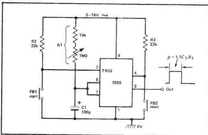
**Figure 19: Manually-triggered 1.1-100sec monostable with reset facility.**
