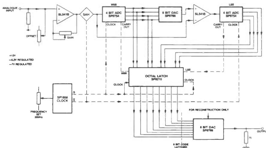
Figure 1: Block diagram for the SP9000 series-based A/D converter.
