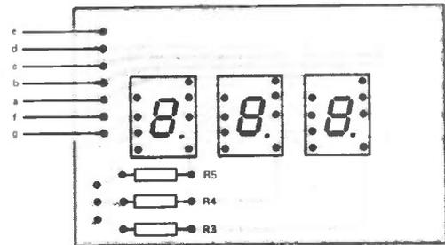
Figure 6: Component overlay for display unit.
