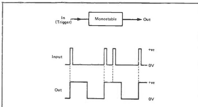
**Figure 2:** A standard monostable generates an accurate output pulse on the arrival of a suitable trigger signal.
