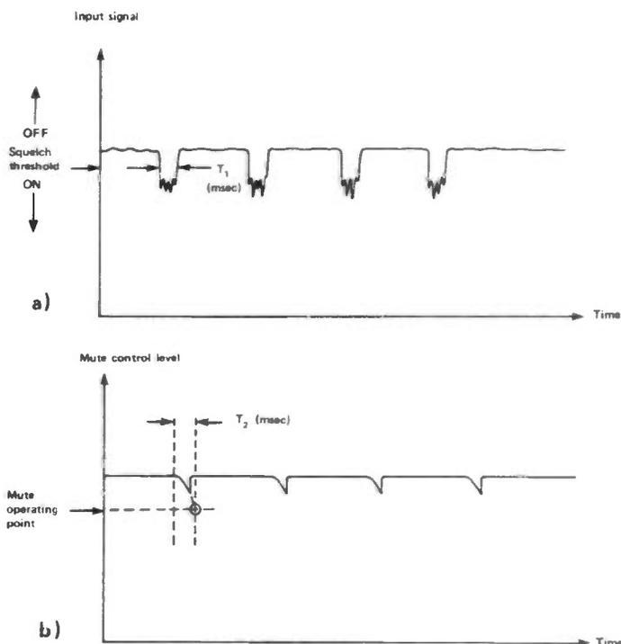
Figure 4: a) Signal flutter brought about by driving past a line of trees. b) Effect of mute. The flutter immunity will depend on the mute operating point with respect to the average incoming signal level. Mute is rarely 'absolute' — i.e. regardless of the incoming signal level.
