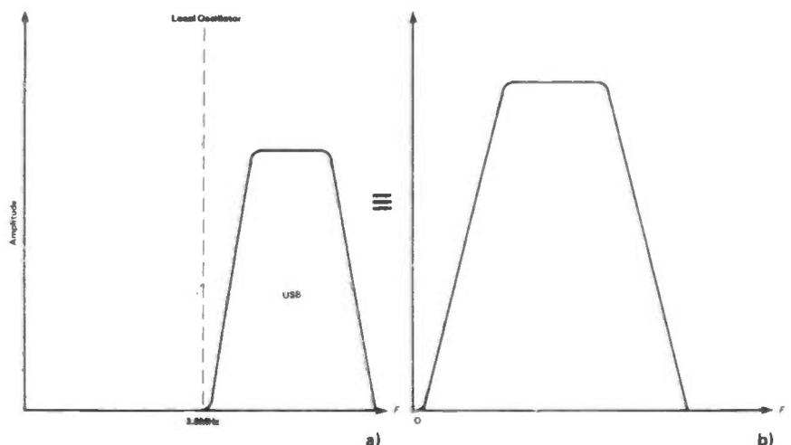
**Figure 1: Direct conversion basics a) USB signal with RF injected locally to set the datum point for the resultant audio spectrum. b) The resultant audio spectrum.**
