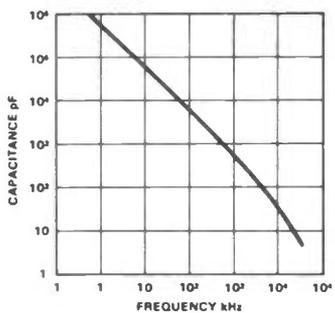
Figure 4: Typical NE564 performance characteristics.
