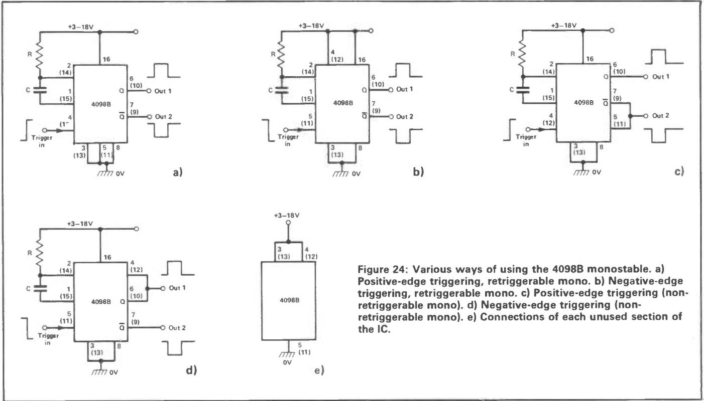
Figure 24: Various ways of using the 4098B monostable. a) Positive-edge triggering, retriggerable mono. b) Negative-edge triggering, retriggerable mono. c) Positive-edge triggering (non-retriggerable mono). d) Negative-edge triggering (non-retriggerable mono). e) Connections of each unused section of the IC.
