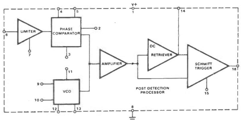
Figure 2: Block diagram of the NE564.
