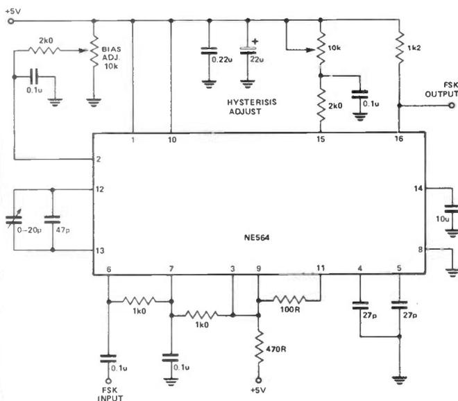
Figure 5: Circuit for an FSK decoder that incorporates an NE564.
