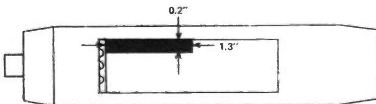
Figure 9: Cut-out details for case of Analogic Probe.
