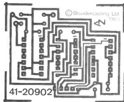
Figure 4: PCB foil pattern for Rotary Encoder Interface (Sept '83).
