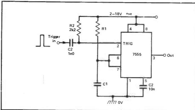
**Figure 20: Simple electronically-triggered 7555 monostable.**
