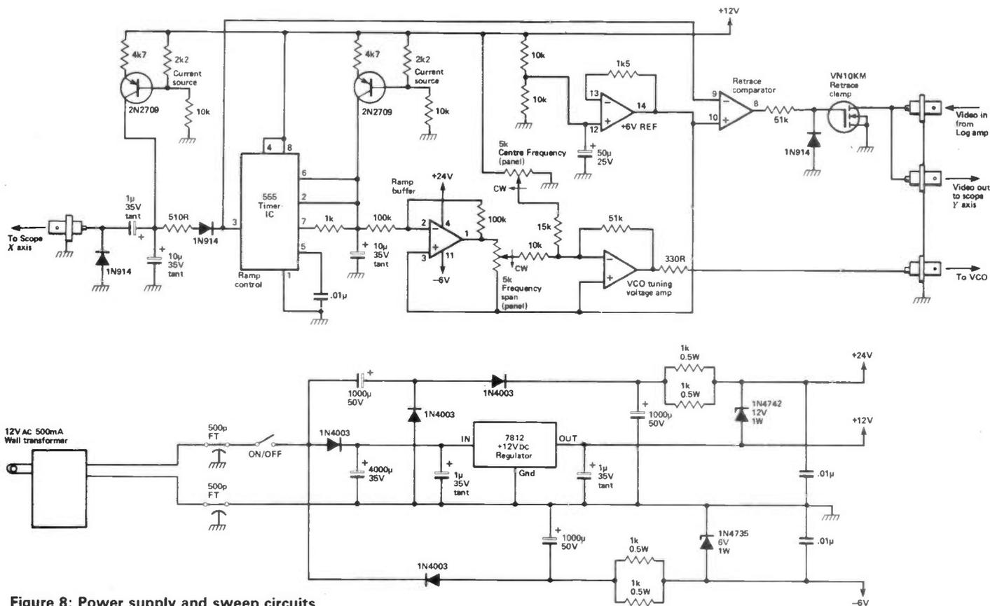
**Figure 8: Power supply and sweep circuits.**
