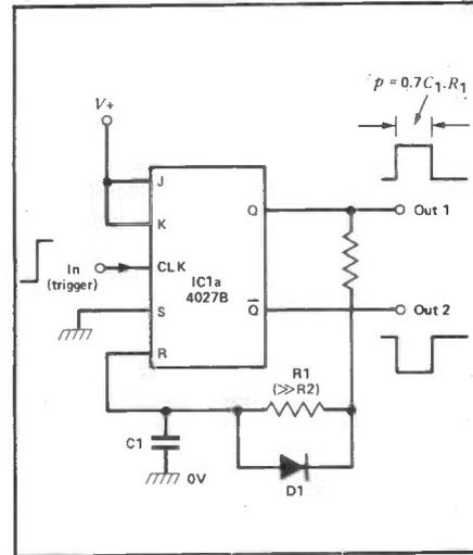
Figure 16: JK-type flip-flop used as a monostable.
