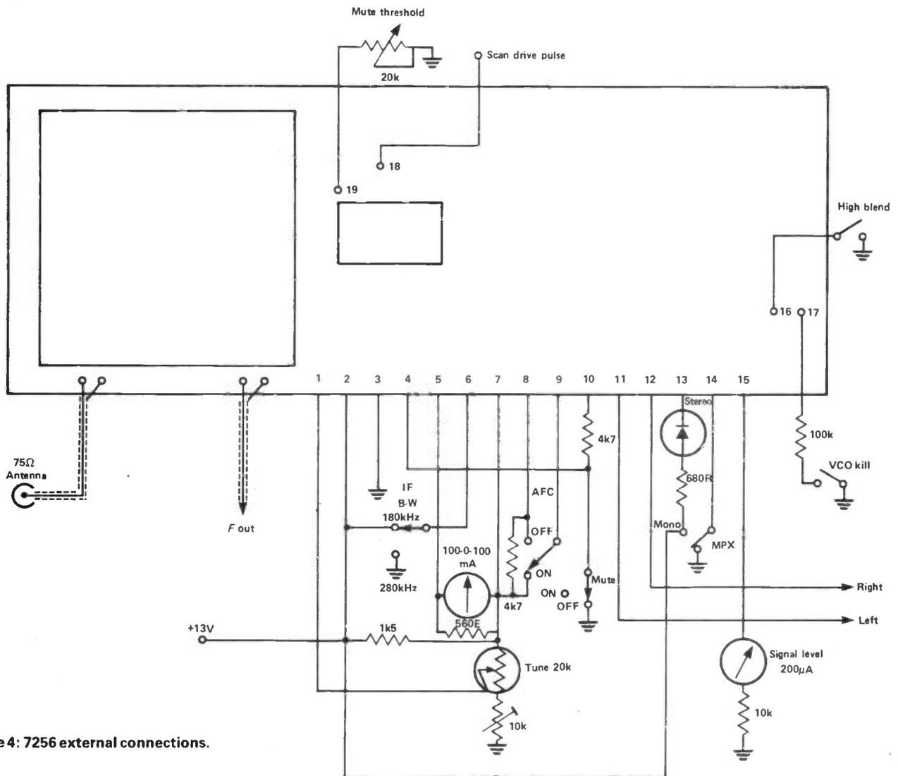
Figure 4: 7256 external connections.
