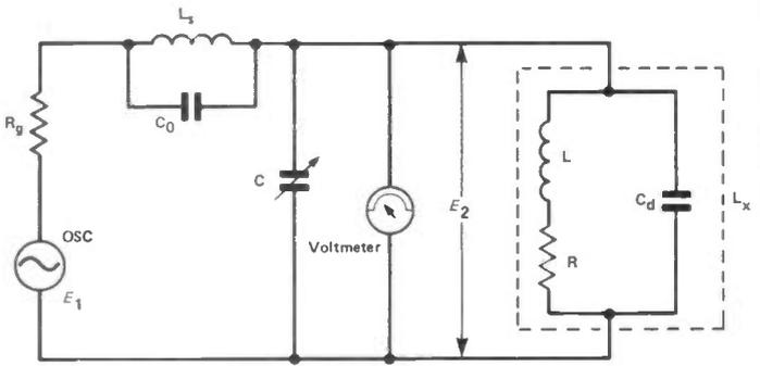
Figure 5: Single-frequency method of measuring  $C_d$ .  $L_s$  auxiliary coil;  $C_0$  distributed capacitance of  $L_s$ .
