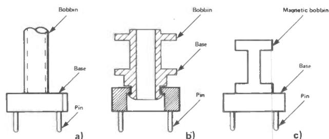
Figure 1: Bobbin — base structures. a) Bobbin and base in one unit; b) Separate bobbin and base — bobbin snapped into place; c) Bobbin bonded to the base.
