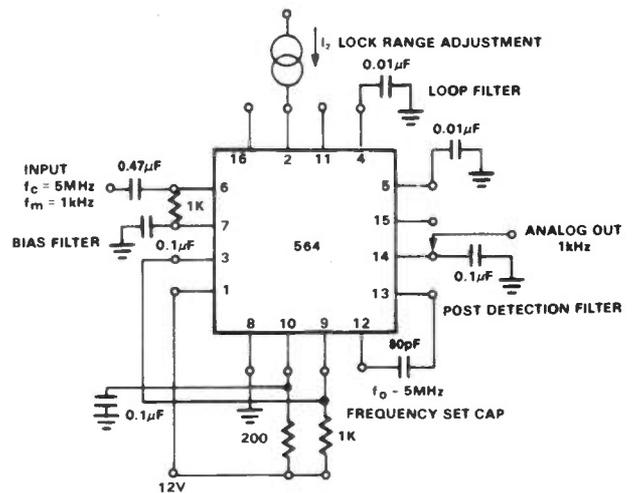
Figure 6: Circuit for an FM demodulator at 12V based on an NE564.
