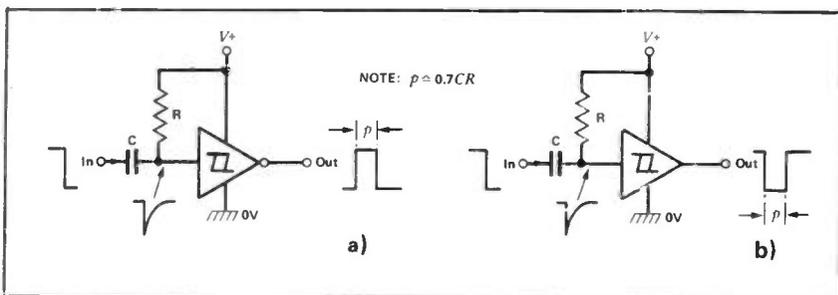
Figure 8: Trailing-edge detector circuits giving a) positive and b) negative output pulses.
