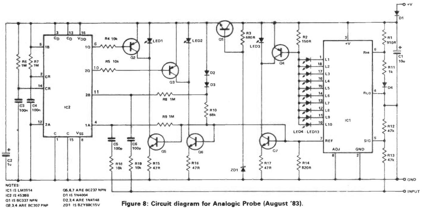
Figure 8: Circuit diagram for Analogic Probe (August '83).
