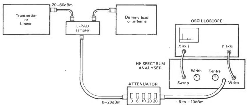
Figure 1: Typical HF spectrum analyser hookup. Always check that transmitter, linear, L-pad, attenuator, analyser and scope are grounded.
