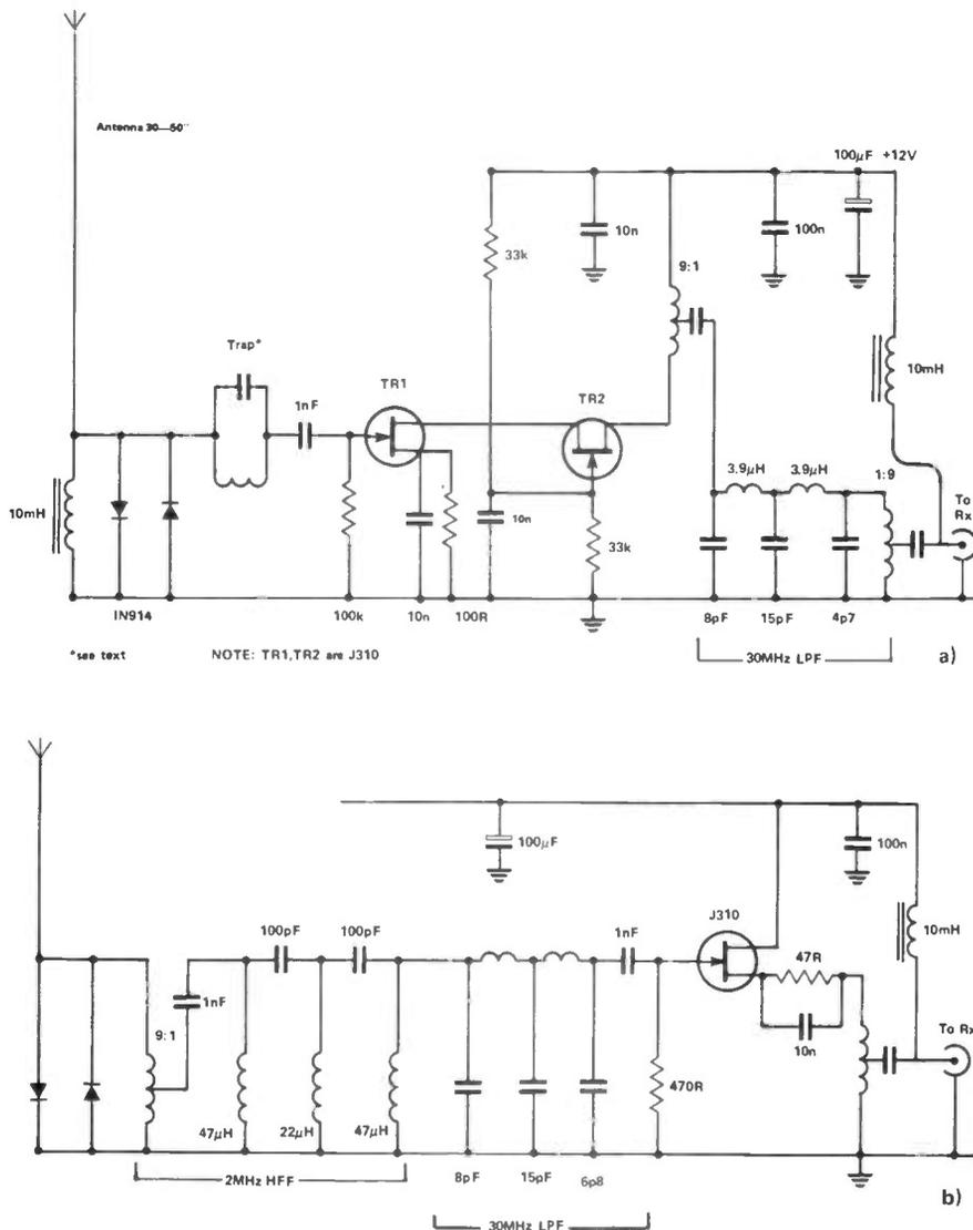
**Figure 3: a) An active antenna head amplifier with low pass filtering. b) An active antenna stage with bandpass filtering.**
