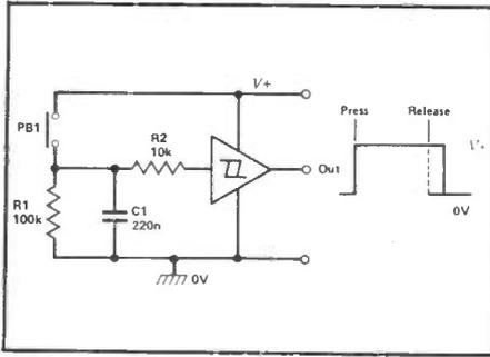
Figure 9: 'Noiseless' push-button switch.
