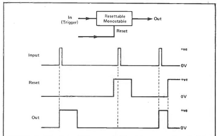
**Figure 3:** The output pulse of a resettable mono can be aborted by a suitable reset pulse.
