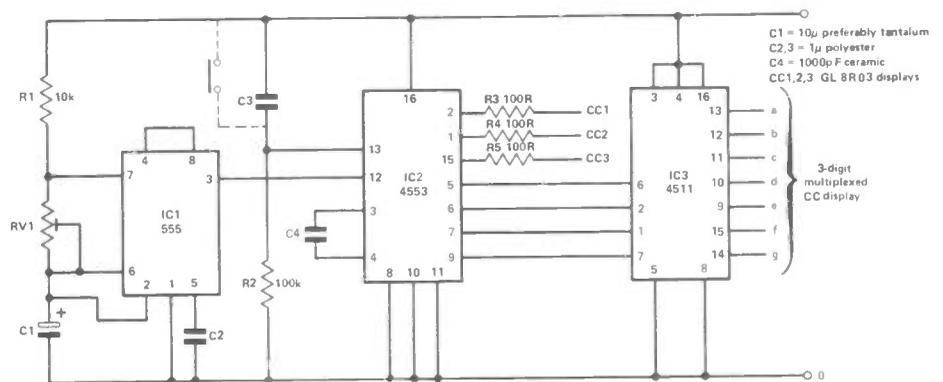
Figure 1: Circuit diagram of timer unit.
