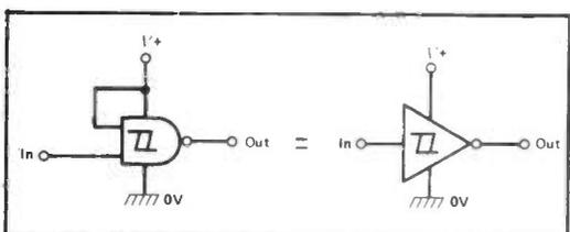
Figure 5: A 4093B 2-input NOR Schmitt can be used as a normal Schmitt inverter by wiring one input high.
