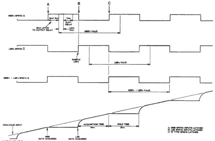
Figure 3: Timing diagram for the 20MHz clock.
