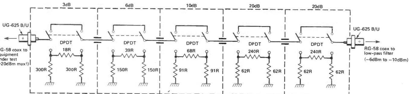
Figure 4: 0-59dB step attenuator.
