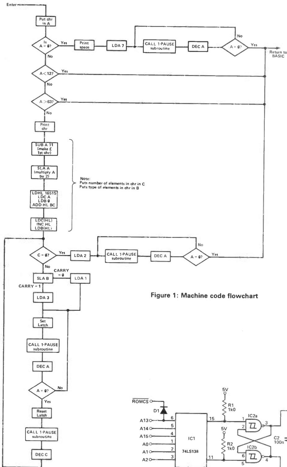
Figure 1: Machine code flowchart
