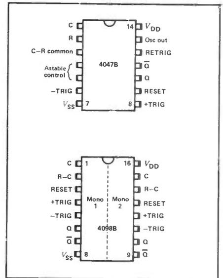
**Figure 22: Outlines and pin notations of the 4047B monostable/astable IC and the 4098B dual monostable.**
