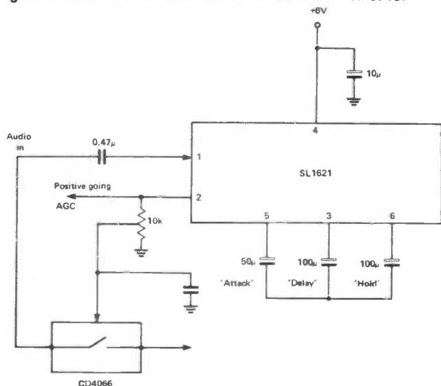
Figure 3: SL1621C AGC generator also controlling mute in an audio-derived application.
