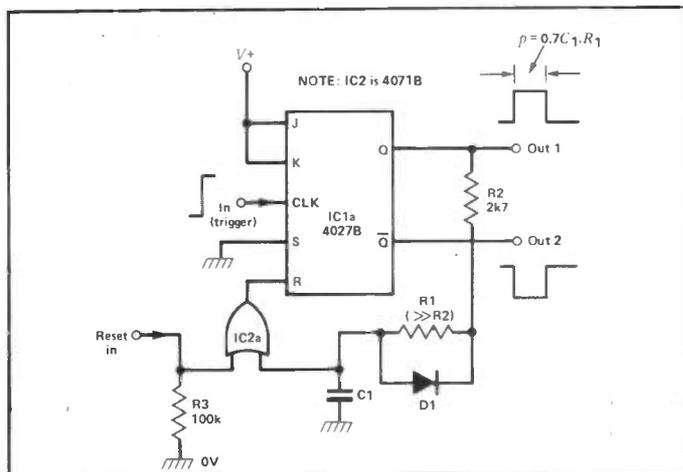
Figure 17: Resettable JK-type monostable.
