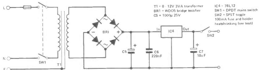
Figure 2: Circuit diagram of display unit.
