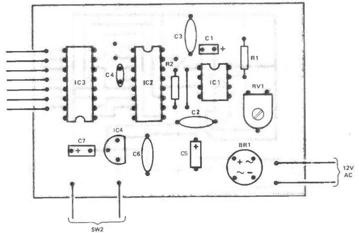
Figure 4: Component overlay for timer unit.
