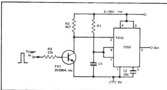
**Figure 21: Pulse-triggered 7555 monostable.**
