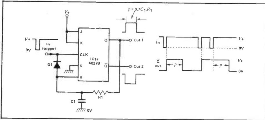
**Figure 18: Retriggerable JK-type monostable.**
