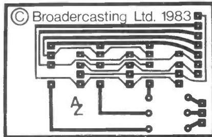
Figure 5: PCB for display unit.
