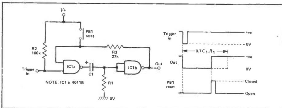
Figure 14: Resettable NAND-type monostable.
