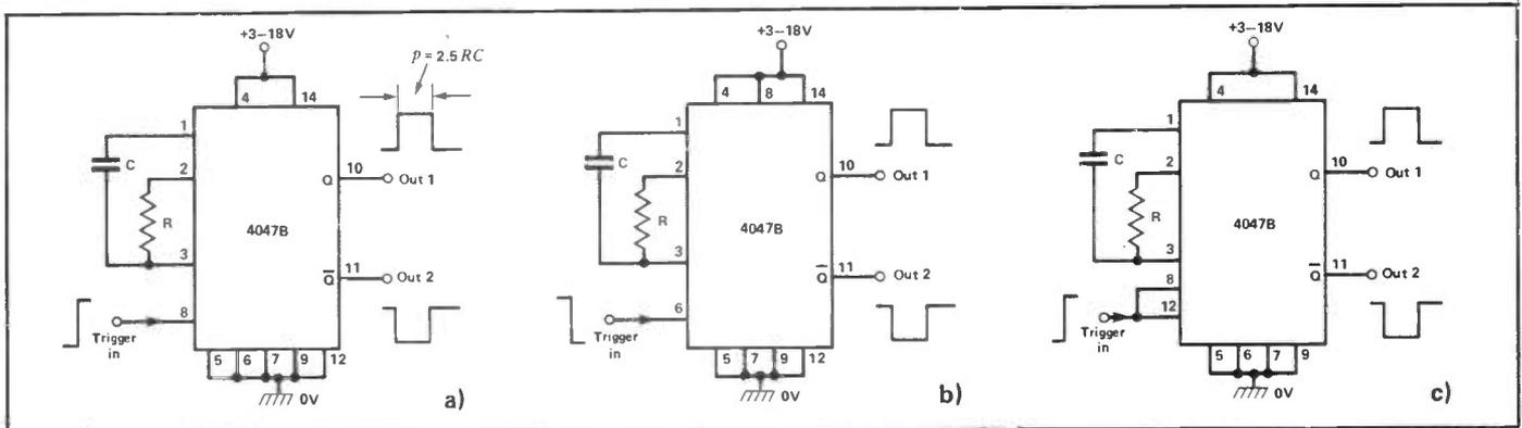
Figure 23: Various ways of using the 4047B as a monostable. a) Positive-edge triggered monostable. b) Negative-edge triggered monostable. c) Retriggerable monostable, positive-edge triggered.
