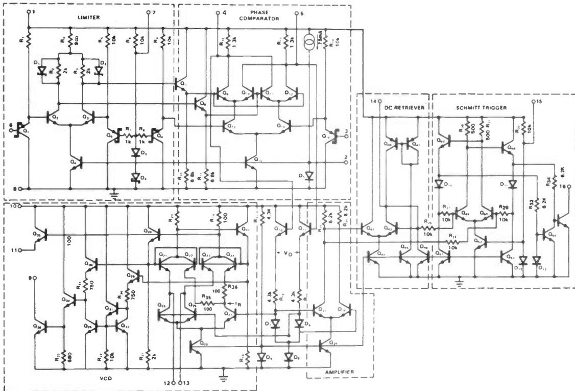
Figure 3: Circuit diagram for the NE564, with errors corrected (see text).
