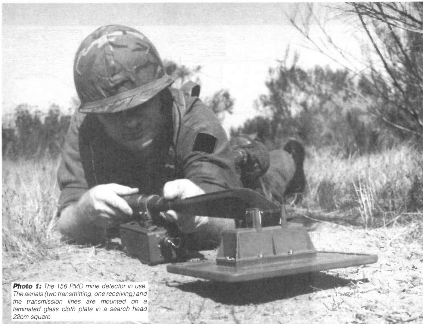
**Photo 1:** The 156 PMD mine detector in use. The aerials (two transmitting, one receiving) and the transmission lines are mounted on a laminated glass cloth plate in a search head 22cm square.
