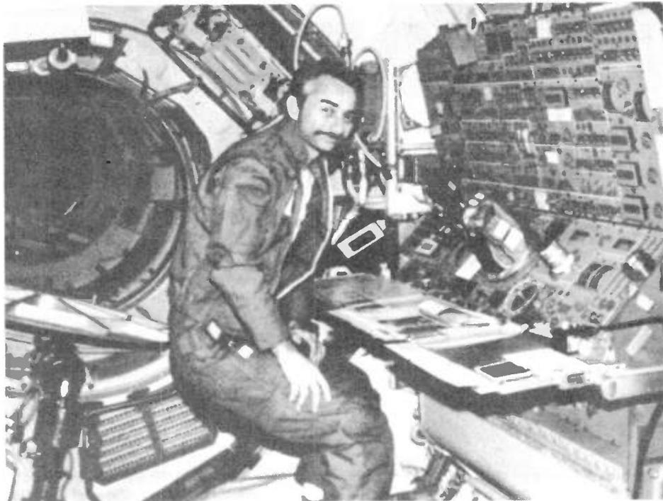
*Dr Owen Garriott, W5LFL, at the console of Skylab in a photograph taken in 1973. He is shown controlling a battery of telescopes pointed at the Sun. Notice that, while he appears to be sitting, zero-gravity means that he doesn't need a chair.*
