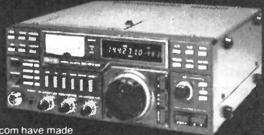
Icom have made improvements to the IC-251 and brought it up to date. Power can be adjusted up to 25W on all modes SSB, CW and FM. Squelch works on all modes and a listen-input facility has been added for Repeater work. RIT shift is shown on the display. 10 Hz tuning facility. Options include a switchable front end pre-amp. Speech synthesizer announcing displayed frequency. 22 Channel memory extension - with scan facilities. Internal chopper PSU, SM5 desk mic. Why not call us for further details?
