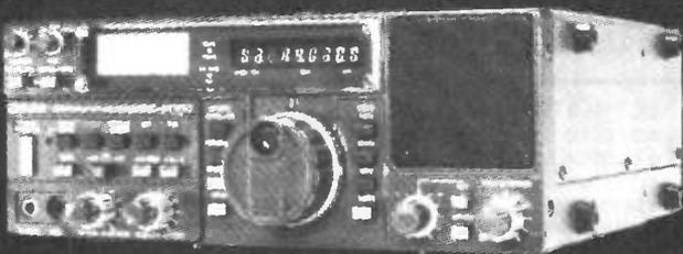
The R-70 covers all modes (when the FM option is included), and uses 2 CPU-driven VFO's for split frequency working, and has 3 IF frequencies: 70MHz, 9MHz and 455KHz, and a dynamic range of 100dB. It has a built-in mains supply.
