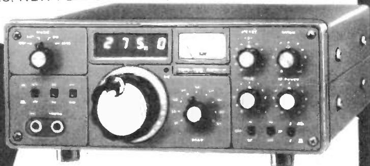
**KW + TEN-TEC ARGOSY II HF SSB/CW TRANSCEIVER**
