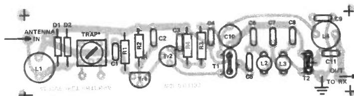
**Fig 6** Component overlay
