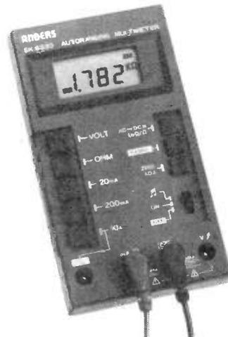
custom LSI circuit automatically selects the optimum range for any voltage or resistance reading, (a feature that can be manually overridden if so desired) whereupon that reading is displayed together with the captions relating to selected function and range. Additional captions can be used to indicate auto/manual mode, DC input polarity or low battery power.
