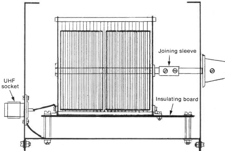
Fig 4 Mounting of capacitor C1
