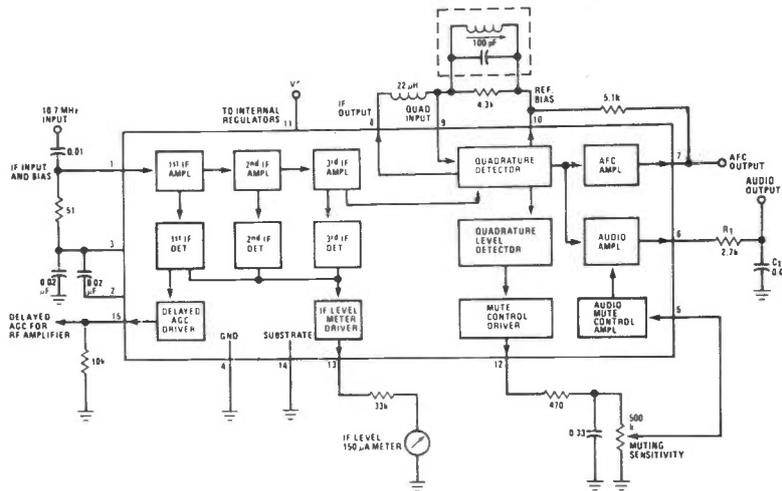
Fig 3 (a) Block diagram LM 3089
