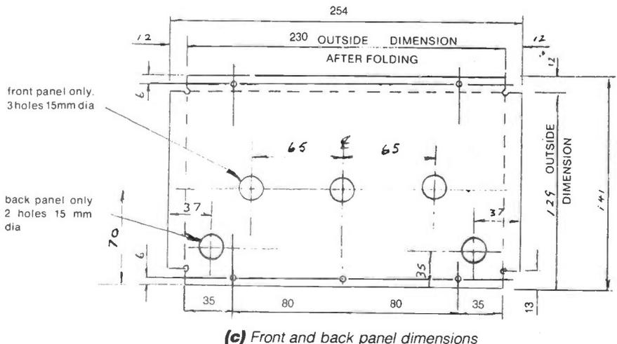
Fig 7 Dimensions of the metalwork
