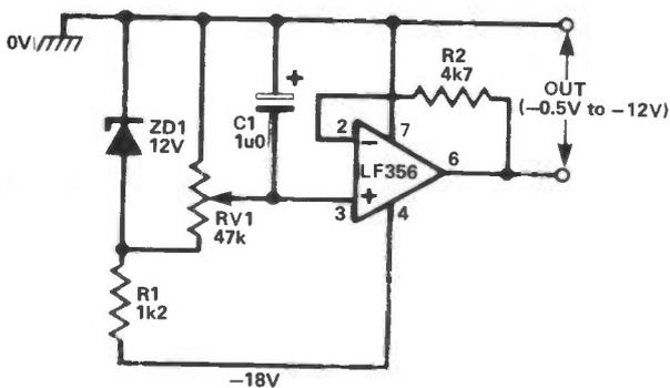
**Fig 18** Variable negative voltage reference
