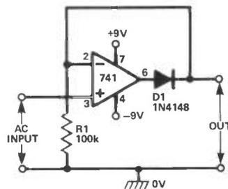
Fig 1 Simple half-wave rectifier circuit
