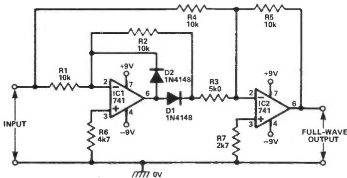
**Fig 6** Precision full-wave ac/dc converter
