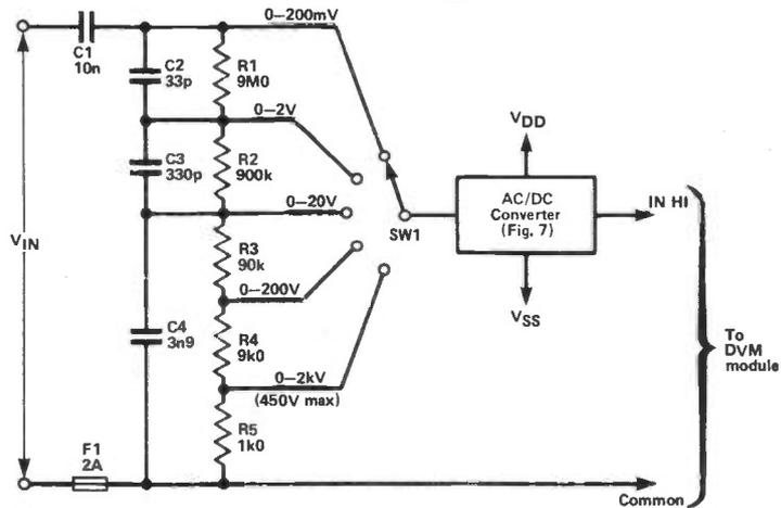
**Fig 8** 5-range ac volt-meter converter for use with DVM modules
