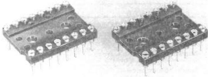
insertion-force collet sockets are used and are available with solder tail or 2- or 3-level wire wrap pins. Collet sockets with gold contacts and gold body or tin body are in a blue Valox low profile body with a notch for polarization or pin identification. 6- through 14-pin on 0.500 centres are also available (contact factory for details). For applications requiring a raised socket above the PCB, an elevator type is available (as special) to raise the socket as much as 1.250ins.
