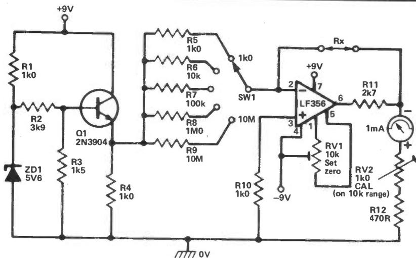
**Fig 16** 5-range linear-scale ohmmeter
