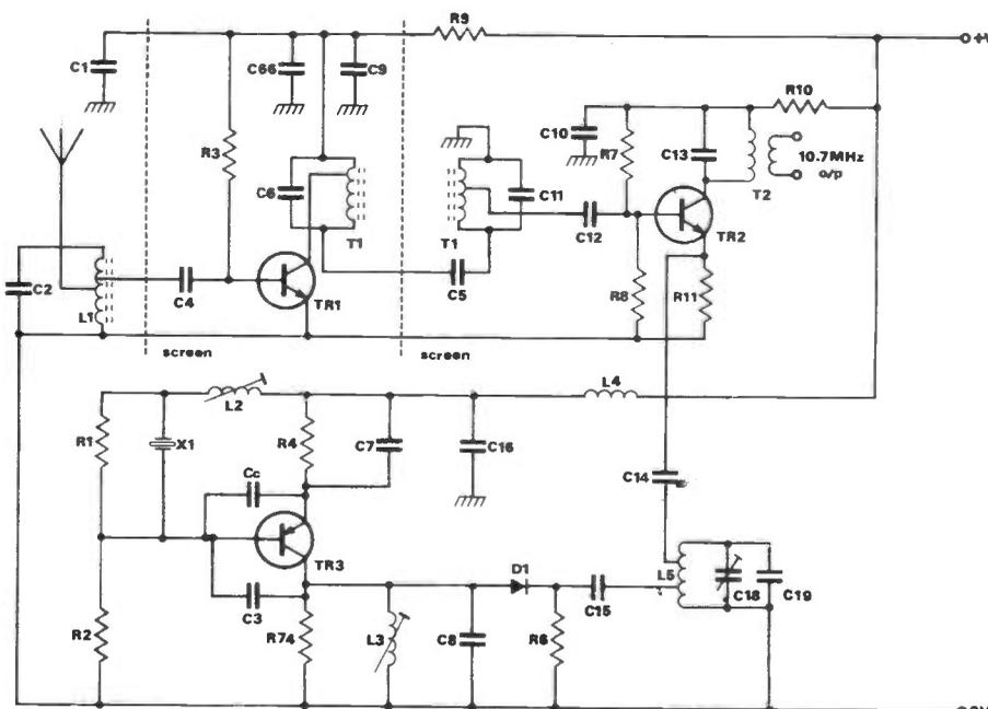
Fig 2 Circuit detail before modification but showing connections for Cc
