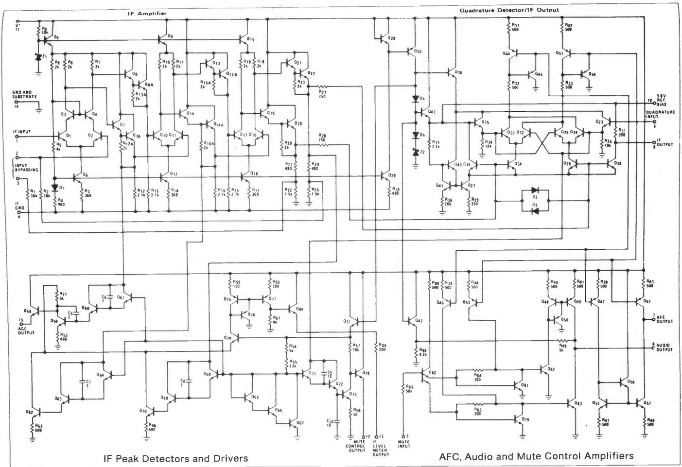
Fig 3 (b) Circuit diagram LM3089
