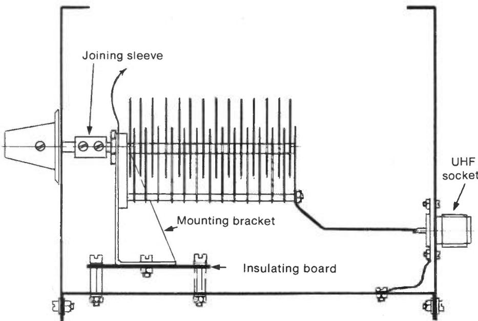
Fig 5 Mounting of capacitor C2
