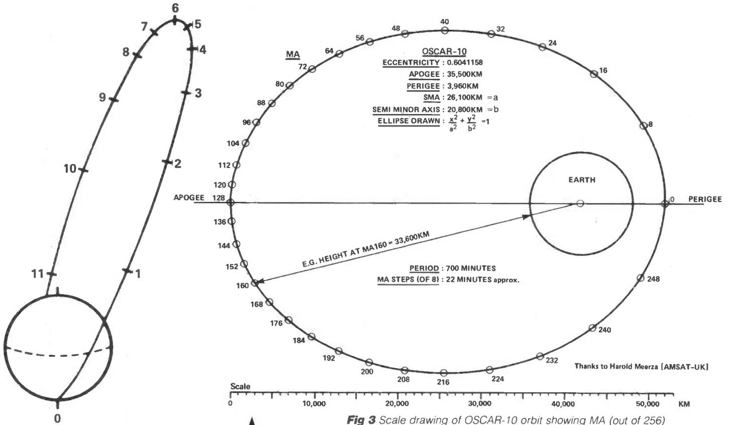
**Fig 2** The position of a Satellite with a 12-hour period at hourly intervals showing speed variations
