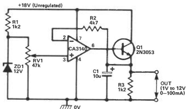
**Fig 19** Simple variable-voltage regulated power supply
