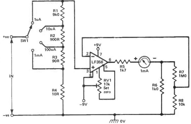
Fig 14 4-range dc microammeter
