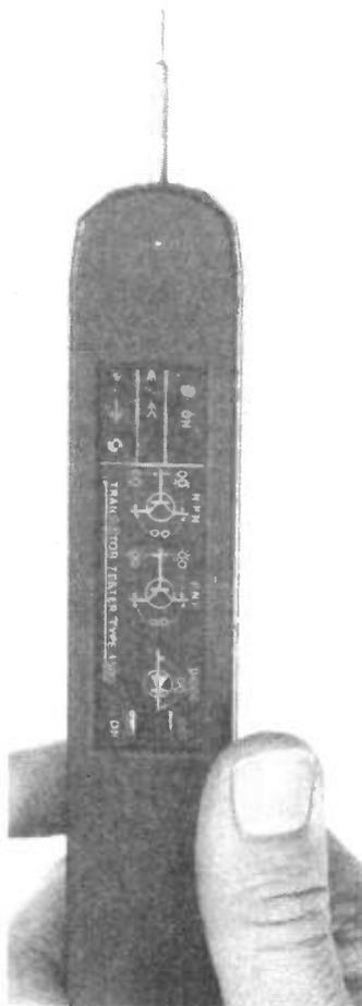
model 4500 transistor tester. Completely self contained, the unit simplifies and speeds the task of checking the PN junctions of discrete semi-conductors whether in or out of circuit.
