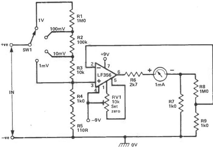
Fig 13 4-range dc millivoltmeter
