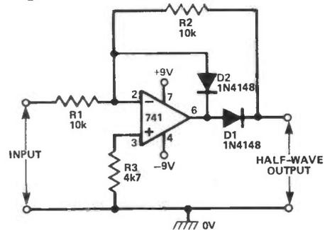
Fig 3 Precision half-wave rectifier
