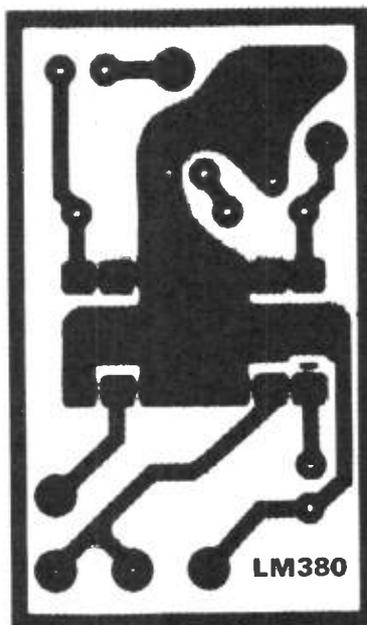
Fig 2 PCB foil pattern corresponding to Figure 1
