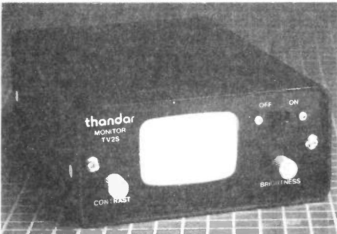
monitor. TV2S operates from a standard 1-volt composite video signal via a 75-ohm BNC connector.
