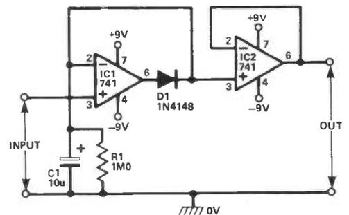
Fig 2 Peak detector with buffered output
