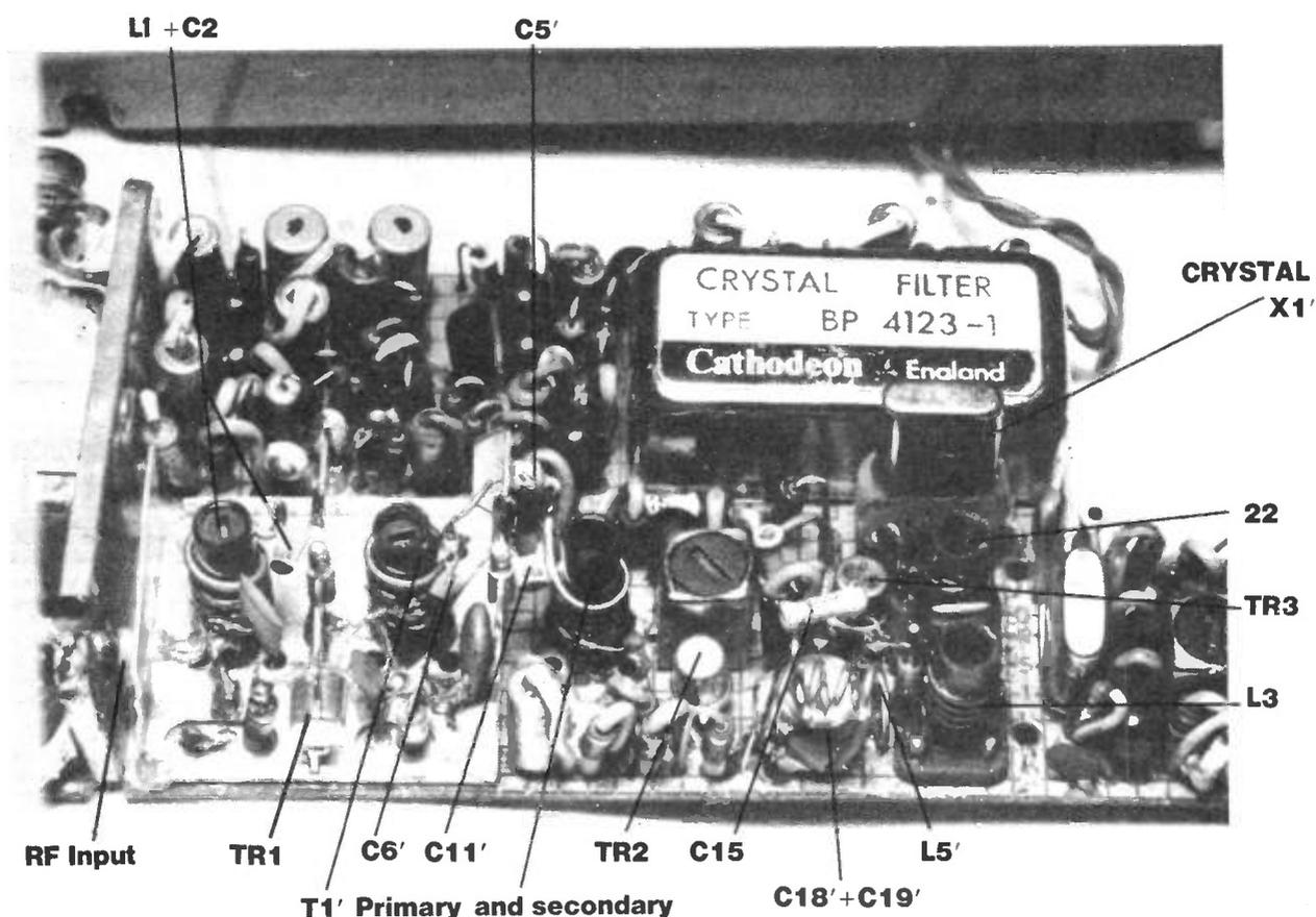
Fig 1 The receiver after modification
