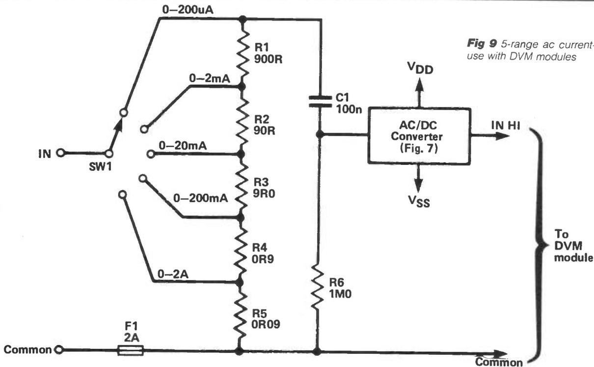
**Fig 9** 5-range ac current-meter converter for use with DVM modules
