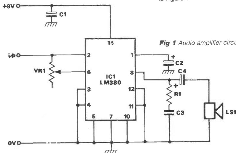
Fig 1 Audio amplifier circuit
