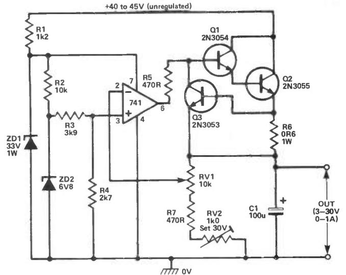
**Fig 22** 3V to 30V stabilised psu with overload protection
