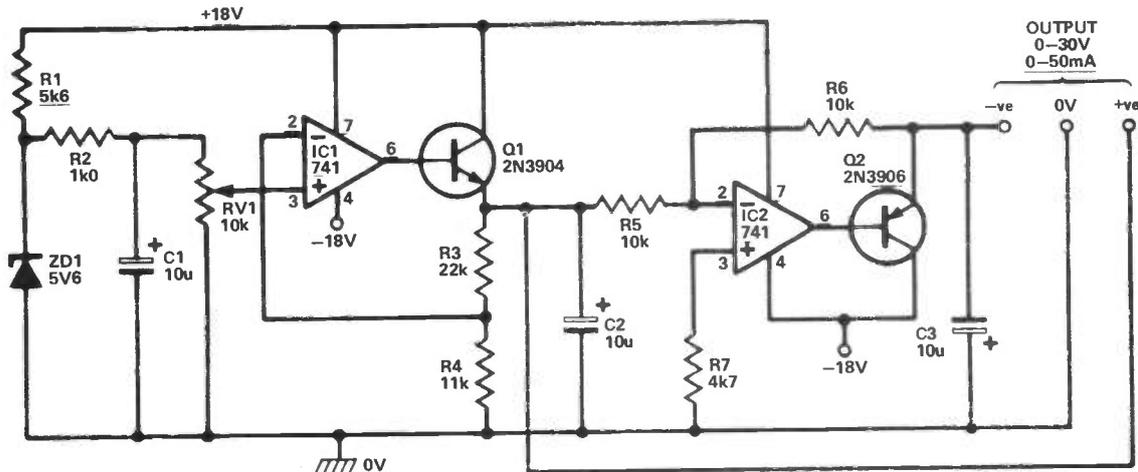
**Fig 23** Simple centre-tapped 0-30V psu
