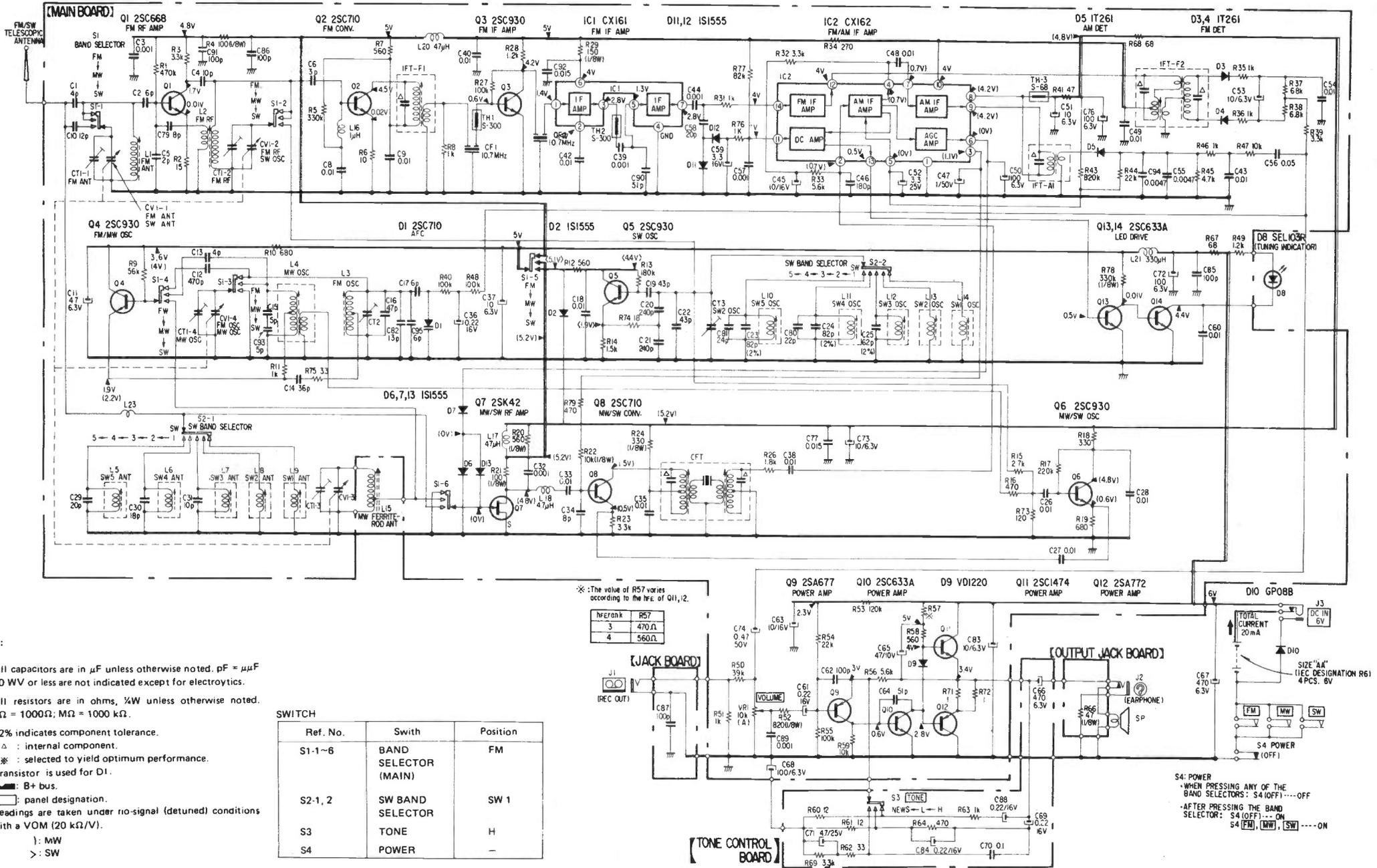
Fig 2 ICF 7600 Receiver - circuit
