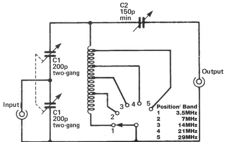
Fig 1 Circuit diagram of the 200W PEP transmatch
