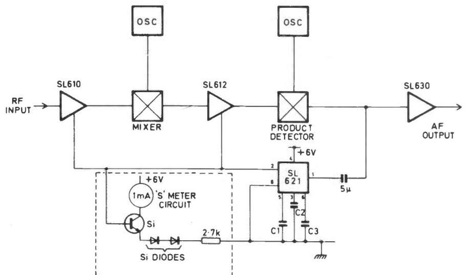
Fig 2 SL621C used to control SSB receiver
