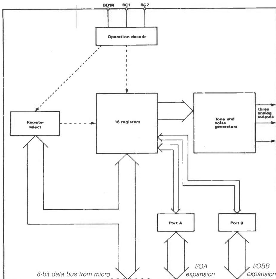
Fig 1 (a) PSG block diagram
