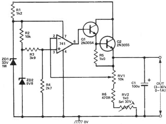
**Fig 21** 3V to 30V, 0-1 amp stabilised psu
