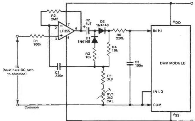
**Fig 7** Ac/dc converter for use with DVM module
