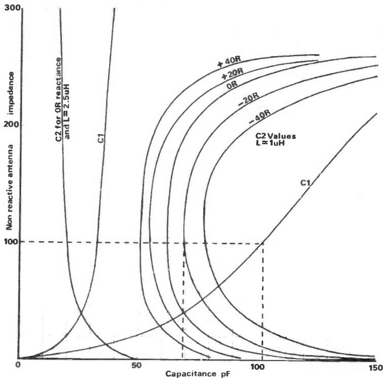
Fig 3 (a) The effect of degree of antenna reactance on the value of C2
