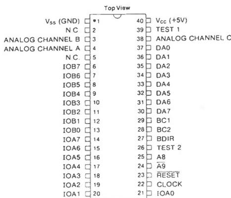
Fig 1 (b) AY-3-8910 pin assignments
