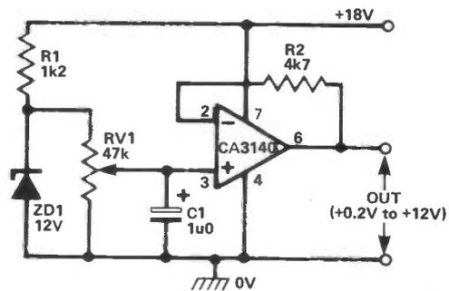
**Fig 17** Variable positive voltage reference
