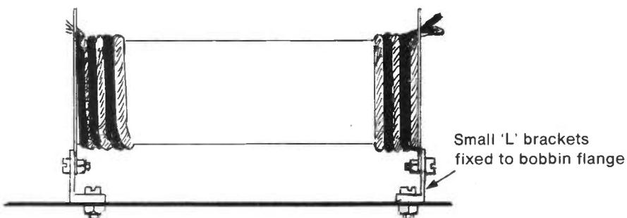
Fig 6 Construction of coil
