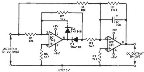
**Fig 4** Precision full-wave rectifier
