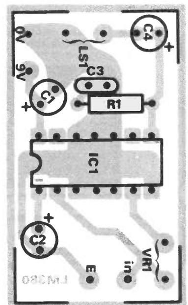
Fig 3 Component overlay
