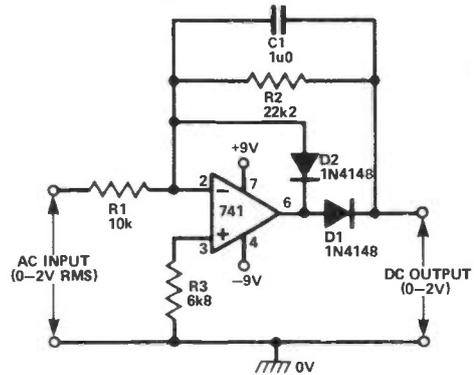
**Fig 5** Precision half-wave ac/dc converter
