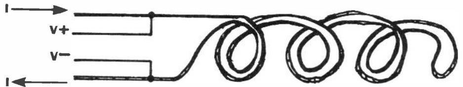
Figure 1 Voltage tapping points
