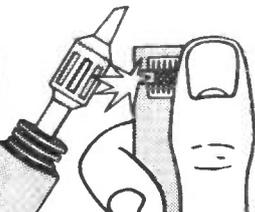
Flint ignition system built into the cap.
