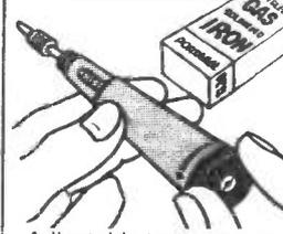
Adjustable temperature equivalent to electric soldering irons 10 to 60 Watt.
