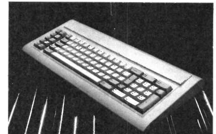
keyboard assembly uses a full-travel membrane key-switch action with a choice of linear or tactile switching action. Reliability is very high, with typical life cycles in excess of 50 million operations, and the membrane technique provides environmental protection for the switching elements.
