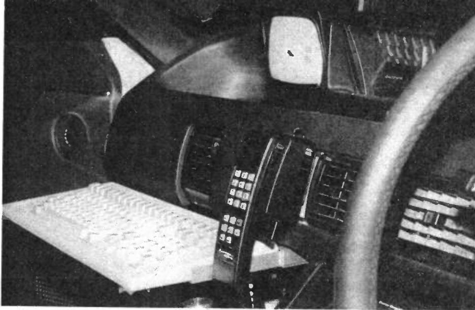
The Cellnet field strength measuring vehicle, which contains signal strength measurement and position fixing equipment. The field strength contours can be measured on the move
