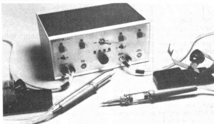
A self-contained unit for reworking assembled printed circuit boards is now being offered by Oryx. The rework station, HSR-1, is especially efficient for the removal of components from through-hole plated boards.
