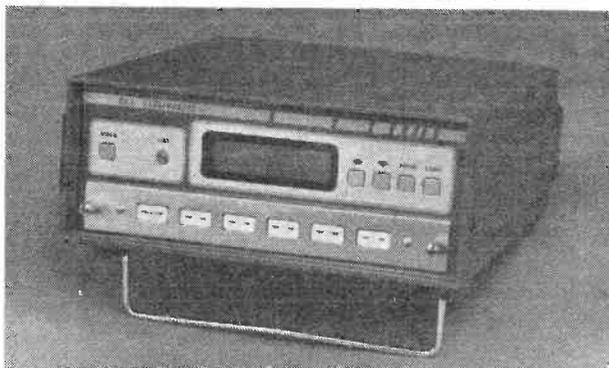
The module installed in the illustrated JAY is the 6 channel thermocouple temperature monitor. The microprocessor program is stored in PROM within the module. Each module therefore has a different program to perform its particular task.
