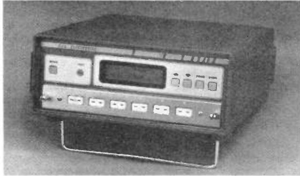
The module installed in the illustrated JAY is the 6 channel thermocouple temperature monitor. The microprocessor program is stored in PROM within the module. Each module therefore has a different program to perform its particular task.
