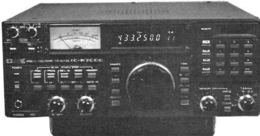
The top switch in the middle of the two rotary controls is the 'write' switch. When this is pressed the frequency and information shown on the display is automatically transferred to a vacant memory channel.
