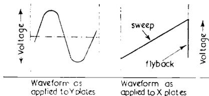
If this 50 cycle mains waveform is applied to the Y-plates, a vertical deflection will be all that is seen on the screen, corresponding to the peak-to-peak voltage
