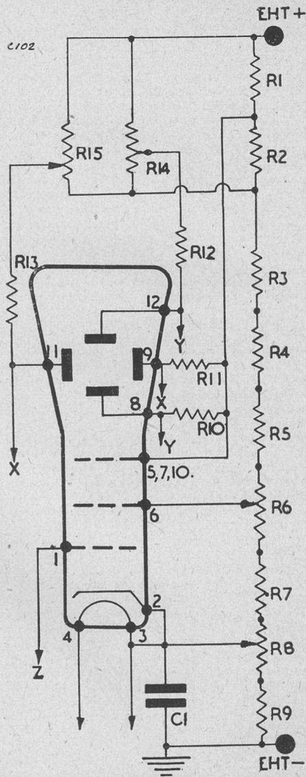
Fig. 1. Connections to tube bases as seen when looking at back of base. The numbering of the contacts for the VCR97 conforms with the numbering given in the tube network diagram.
