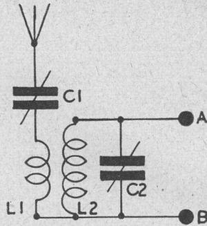
Fig. 2. L2 and L1 are standard SW coils to cover 6—9 Mcs. C1 is 100  $\mu$ F and C2 is 160  $\mu$ F. Points A and B are connected to RF pin on receiver and chassis respectively.
