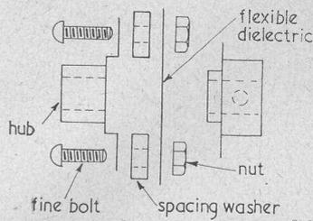
Fig. 4. Method of lengthening coupler.
