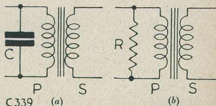
Fig. 13. Showing the addition of a capacitor or resistor to clear "threshold howl". The capacitor should be around 0.002μF and the resistor 50,000 Ω.
