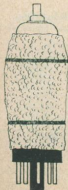
Fig. 14. Where expense is a prime consideration, a microphonic valve may be fitted with a sound-proof jacket as shown. The valve is covered with cotton wool, held in place by rubber bands.
