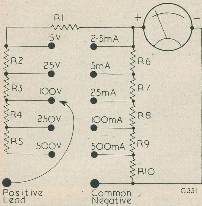
Fig. 2. Circuit of multi-range meter. Values are:—
