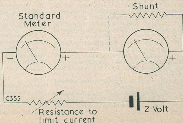
by the meter on the voltage ranges. However, with the shunt resistance values shown on the diagram this current is only 2.5 mA.
