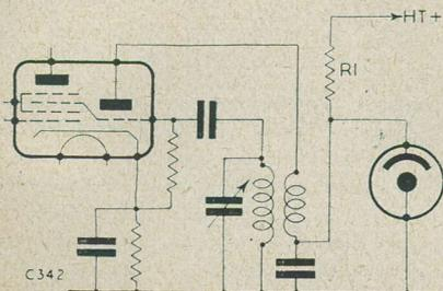
Fig. 1. Neon tube used for voltage stabilisation to prevent frequency drift.  $R1$  acts as a series resistor for both the oscillator anode and the neon. Suitable tubes are the VR150/30, VR105/30 and the Mullard 7475.
