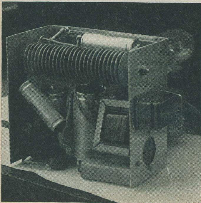
*Under-chassis view of the amplifier. The rectifier can be seen connected across the sub-chassis. The five-pin holder beneath the fuse box is the speaker socket. In the photo heading this article the valves are, reading left to right, V1, 2 and 3 along the front and V4, 5 and 6 at the rear.*
