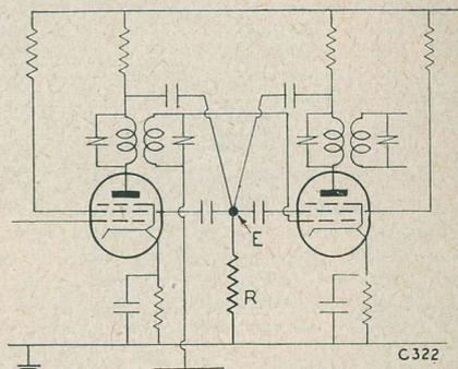
Fig. 10(a). Indicating how a badly connected earthing return, if for several circuits, may actually assist feed-back. The feedback voltages, at different stages of amplification, are built up across the resistance "R," which represents the resistance of the joint. (E is the earth tag with high resistance joint.)
