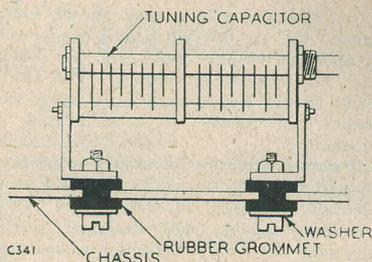
Fig. 15. A vibration-proof mounting for a tuning capacitor.
