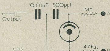
Fig. 2. A simple AF oscillator giving a 1,000 cps. note. Point A is connected to  $L1$  positive and B to chassis. A Bulgin NL1 or Osplin  $\frac{1}{4}$ -watt neon may be used.
