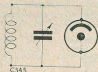
Fig. 4. Absorption wavemeter using the neon tube.
