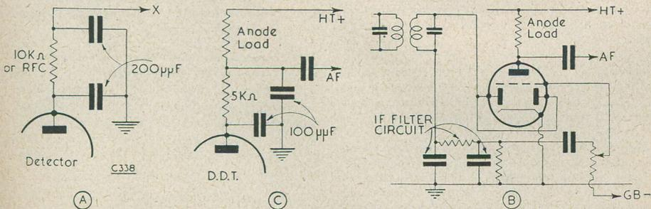
Fig. 12 (a). Additional RF filtering that may be added to the anode circuit of a leaky-grid or anode-bend detector. "X" is the connection originally taken to the anode of the detector.
