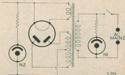
Fig. 5. Neons may be installed as voltage indicators in the power pack. Series resistors may be from 1.5 MΩ dependant on the current taken and consequent voltage drop.
