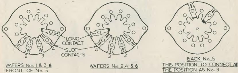
ALL SWITCH CENTRES IDENTICAL EXCEPT 5 WHICH HAS A WIPER ON THE BACK
