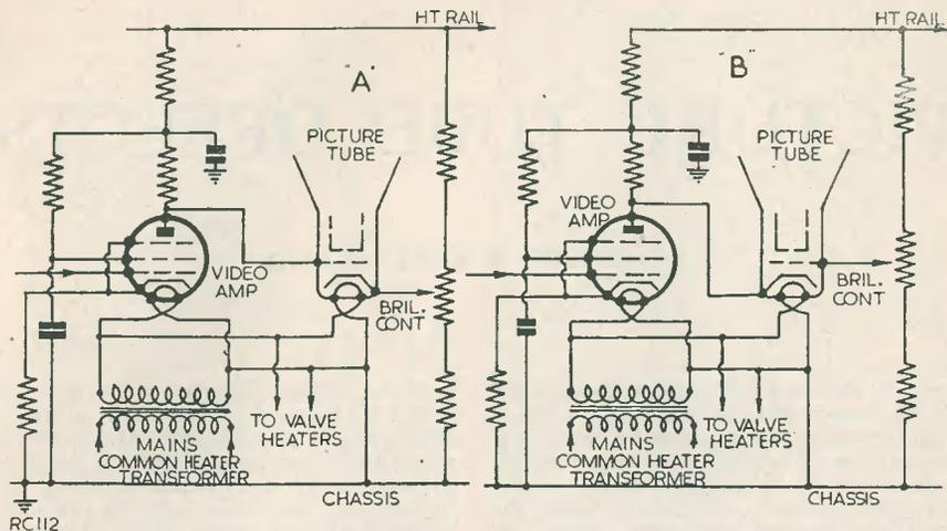
Fig. 1. Methods of modulating a picture tube:
