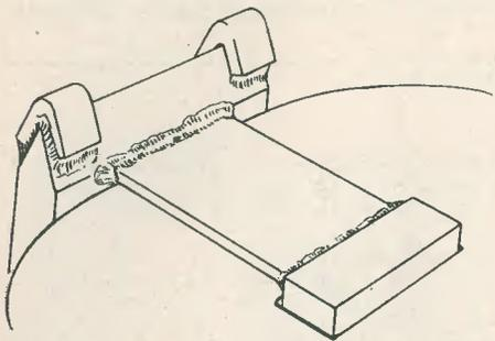
Fig. 2. Pole pieces of sensitive relay
