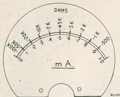
Fig. 3. Scale, showing "Ohms" range
