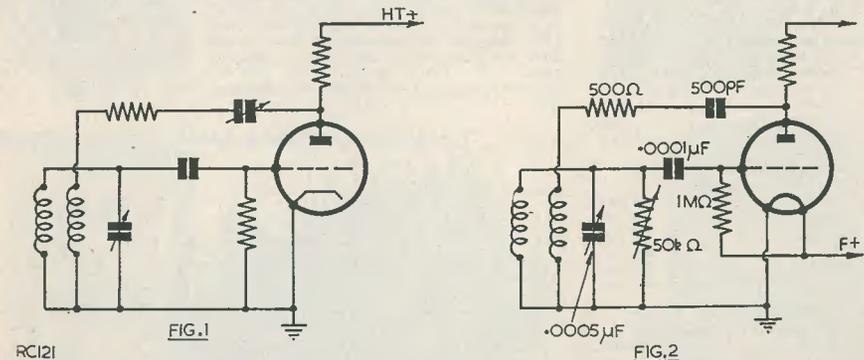
Fig. 1 shows a useful modification to the reaction circuit, which just consists of a resistor joined between the reaction condenser and the reaction coil. The effect is to alter the phase angle instead of the amplitude of the feedback. The result is very much the same, but is very much smoother. The value of the resistor can be almost anything between 100 and 5,000  $\Omega$ ; if it is too high the reaction
