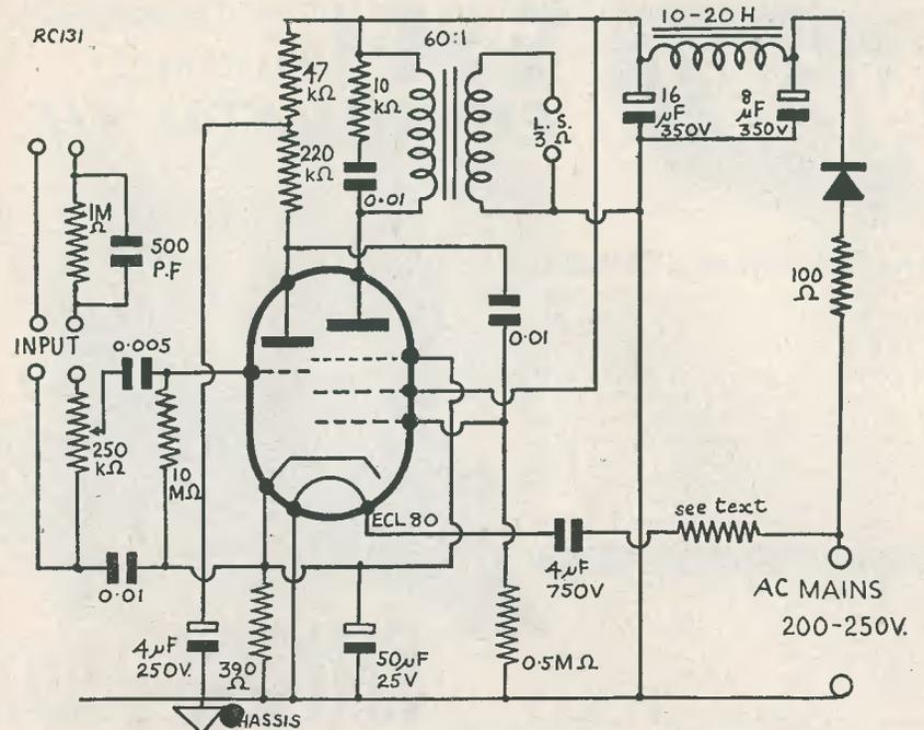
FIG. 1 CIRCUIT OF SIMPLE VALVE AMPLIFIER
