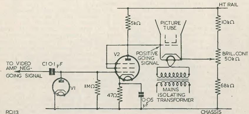
Fig. 2. Circuit changed to grid modulation enabling a faulty tube to be used
