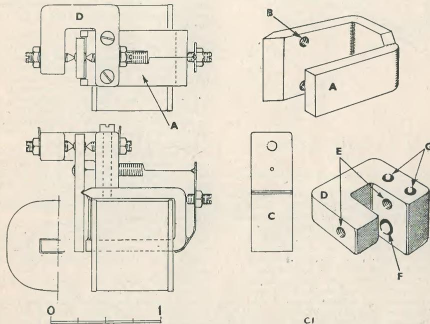
Fig. 1. Details of sensitive relay. Scale in inches
