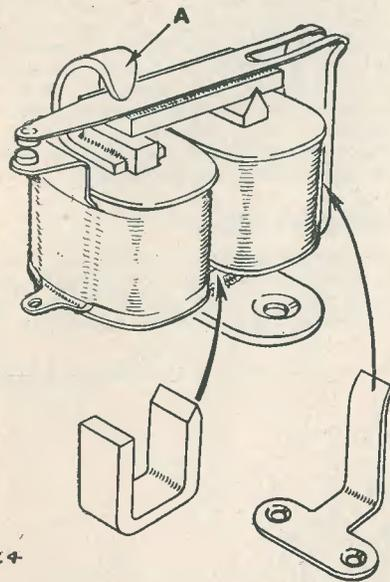
Fig. 4. Secondary relay
