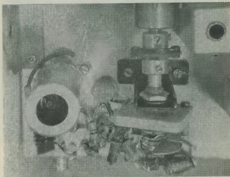
Top view of the chassis around the r.f. amplifier and mixer. The lead from L_5 which connects to pin 1 of V_3 passes round the left hand side of V_3 screening can. The chassis hole through which it passes is drilled as close as possible to pin 1 of V_3
