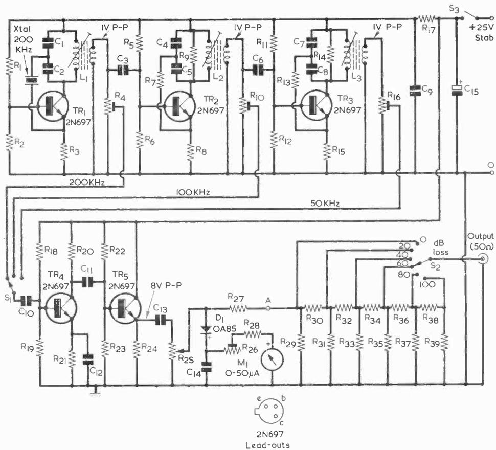
The complete circuit of the frequency divider signal generator
