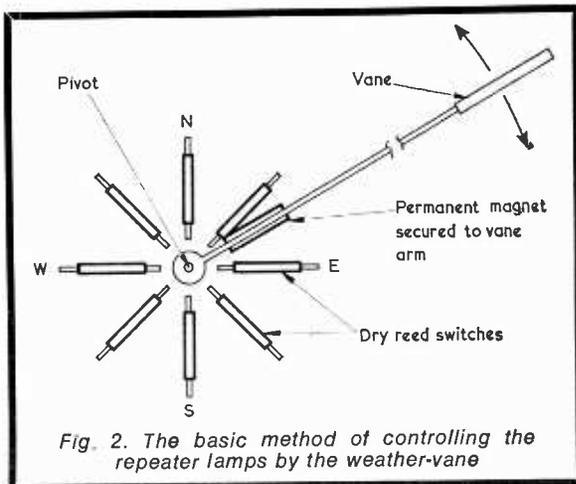
Fig. 2. The basic method of controlling the repeater lamps by the weather-vane
