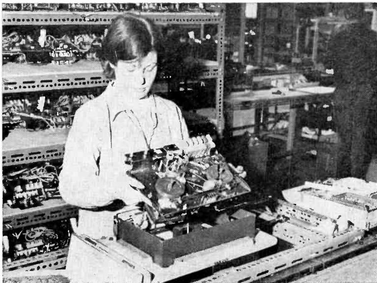
A final step in the manufacture of a British Radio Corporation tape recorder. The machine, mechanically and electrically completed, is fitted into its cabinet
