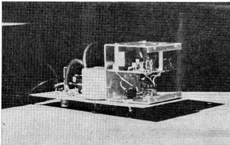
*View illustrating construction inside the main screening cover. Components, including the preset potentiometers, are mounted on a printed circuit board*
