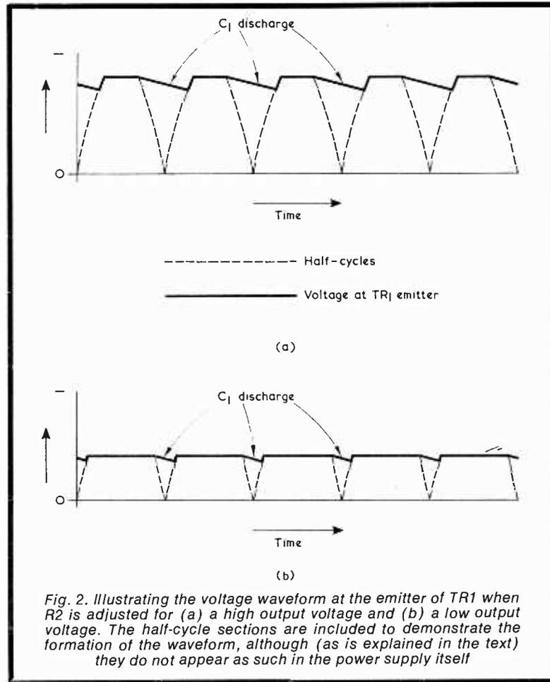
Fig. 2(a), because in Fig. 2(b) C1 receives a charge for a greater part of the cycle. This point is, in fact, borne out in practice, and regulation becomes poorer as output voltage increases.
