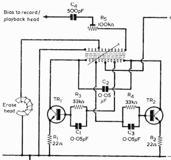
Fig. 4. A push-pull erase oscillator circuit
