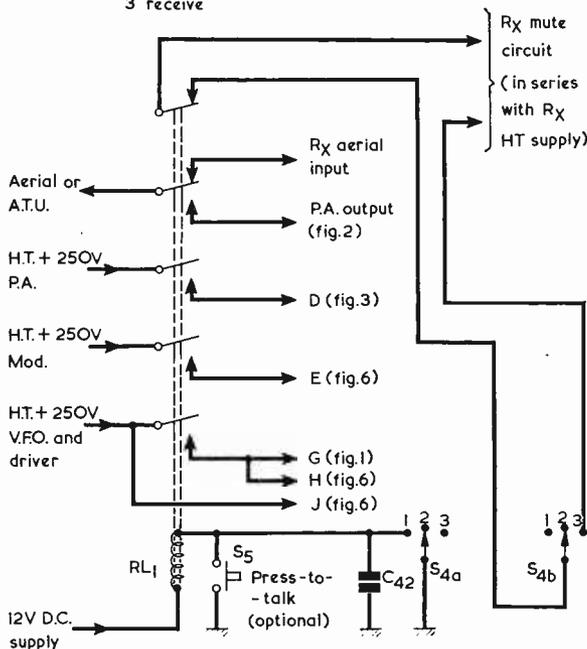
Fig. 5. The main switch and transmit/receive relay
