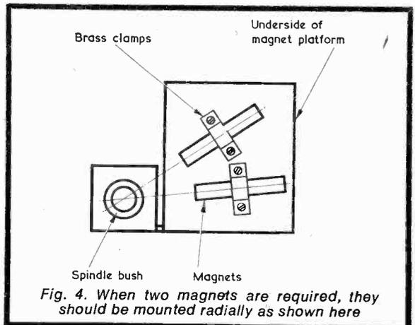
Fig. 4. When two magnets are required, they should be mounted radially as shown here
