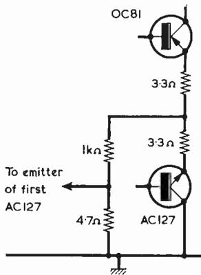
Fig. 4. At audio frequencies, negative feedback to the emitter of the first AC127 is effectively applied in the manner shown here
