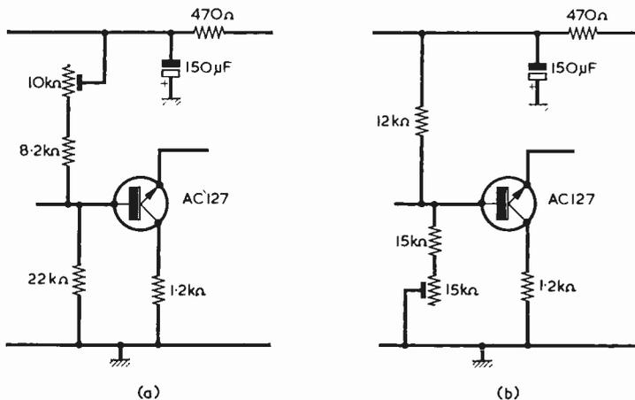
Fig. 5. If the circuit of Fig. 1 were used for a home-constructor project, it would be advisable to have the base bias for the first AC127 adjustable, using either the method of (a) or that of (b). All fixed resistors may be 10% tolerance
