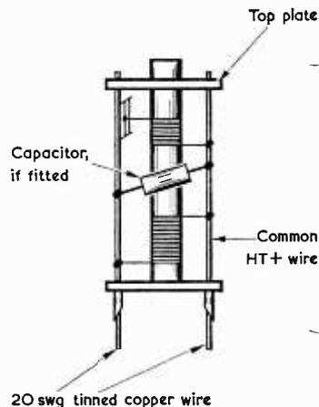
Fig. 8. Coils L6 to L11 are wound in the manner shown here, in which two coils are fitted on a single former
