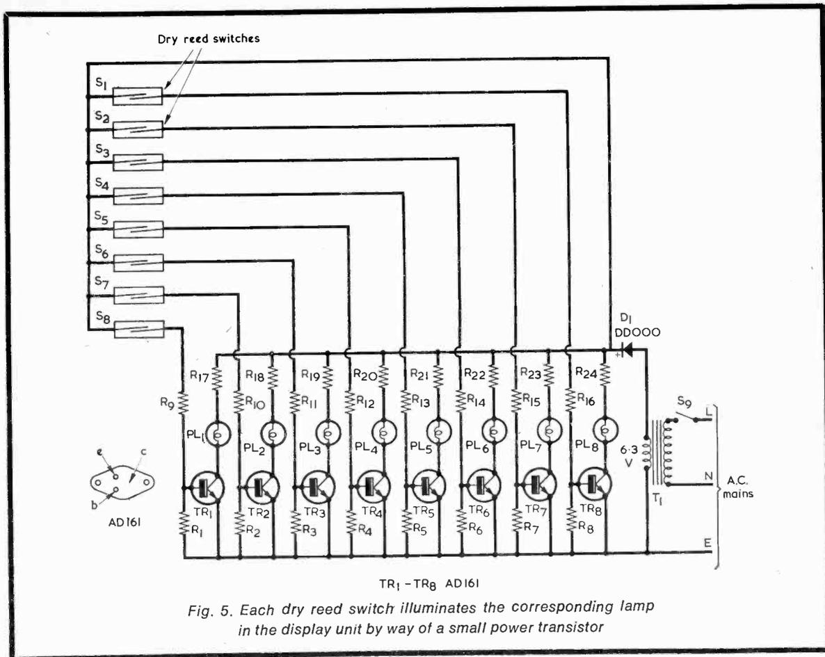
Fig. 5. Each dry reed switch illuminates the corresponding lamp in the display unit by way of a small power transistor
