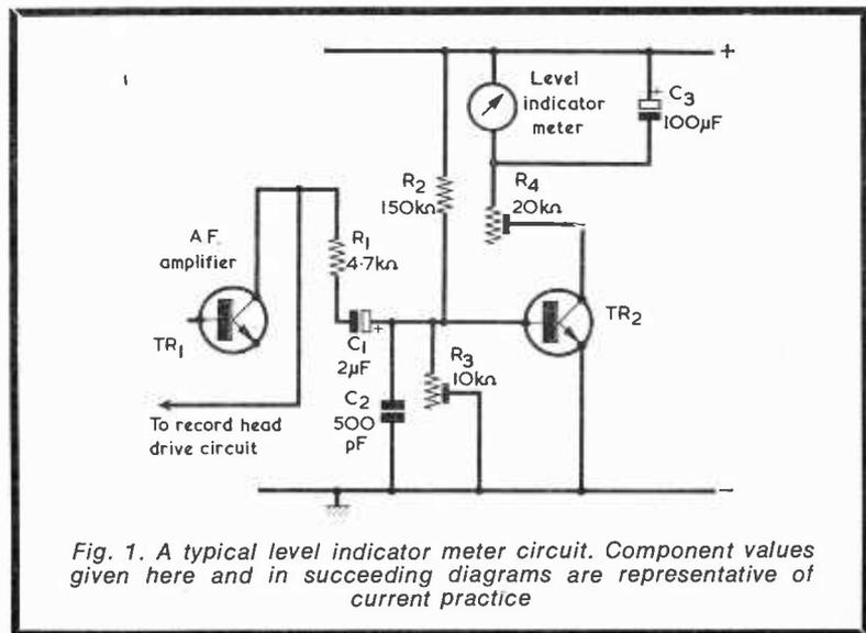
*Fig. 1. A typical level indicator meter circuit. Component values given here and in succeeding diagrams are representative of current practice*
