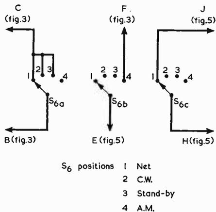
Fig. 6. Connections to the function switch
