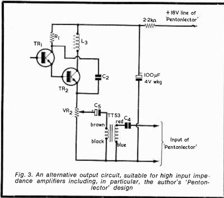
Fig. 3. An alternative output circuit, suitable for high input impedance amplifiers including, in particular, the author's 'Pentonlector' design
