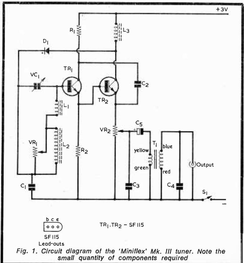
which used a potentiometer between TR1 and TR2. T1 gives an impedance step-up of 1:20 so that the load across the large winding is about 1kΩ. T1 also provides a step-up of voltage of 4½ times.
