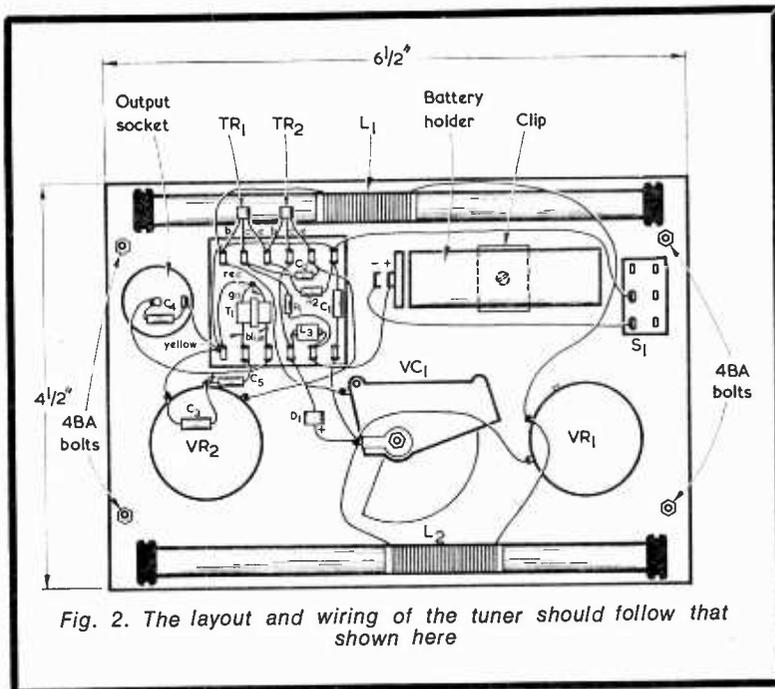
Fig. 2. The layout and wiring of the tuner should follow that shown here
