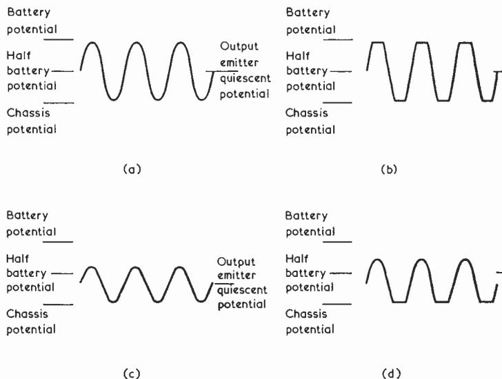
Fig. 2(a). The a.f. voltage output of a correctly set up complementary output stage
