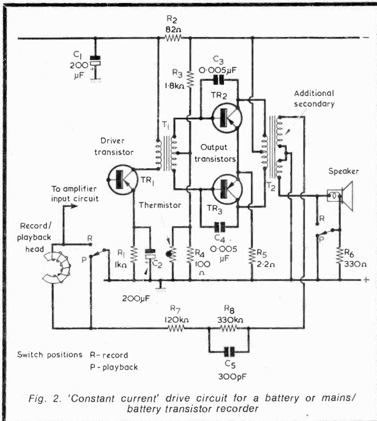
Fig. 2. 'Constant current' drive circuit for a battery or mains/battery transistor recorder
