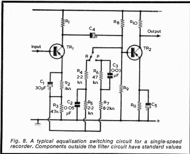
Fig. 8. A typical equalisation switching circuit for a single-speed recorder. Components outside the filter circuit have standard values
