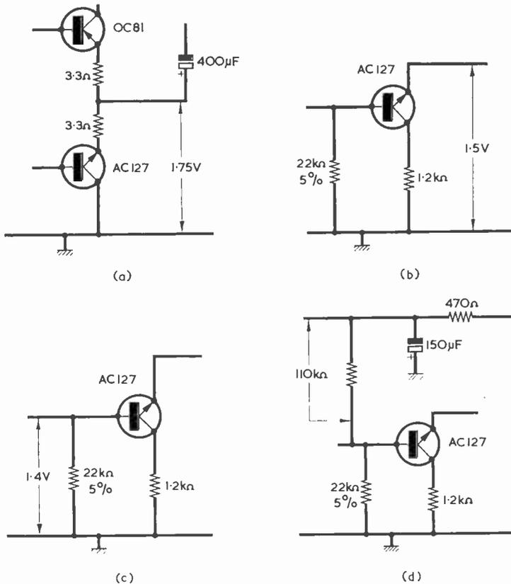
Fig. 3. Testmeter readings obtained with the circuit of Fig. 1. Output emitter voltage is shown at (a), and emitter and base voltages for the first AC127 in (b) and (c). The resistance reading in (d) located the faulty component
