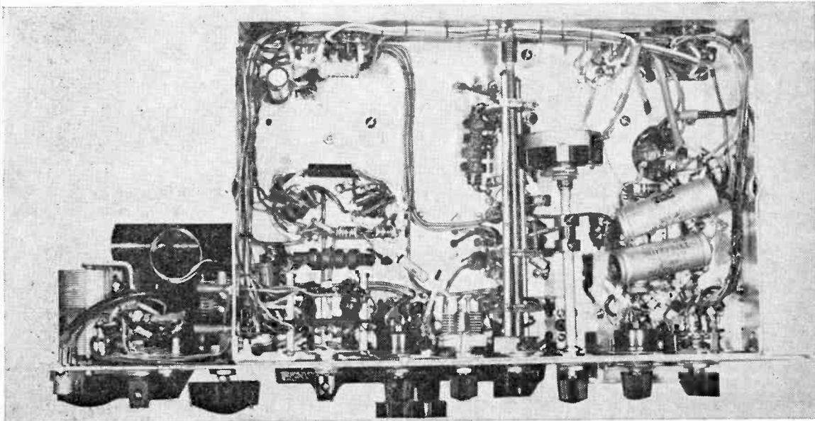
Underneath the chassis. Note the 3-section band switch and the drive control potentiometer alongside
