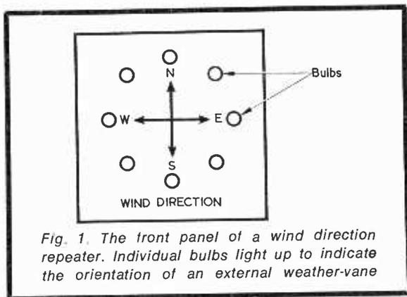
Fig. 1. The front panel of a wind direction repeater. Individual bulbs light up to indicate the orientation of an external weather-vane
