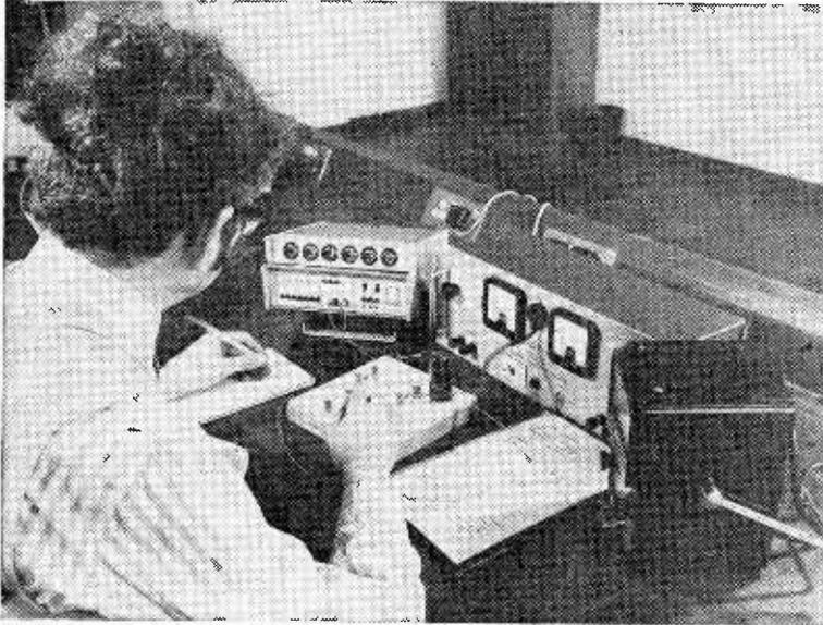
Using a six-digit Dawe Digital Frequency Meter, Counter and Timer Type 3001A in the electronics laboratory at South Birmingham Technical College to examine the performance of a multivibrator
