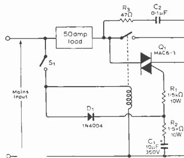
A triac circuit, developed by Motorola Semiconductors, which is capable of increasing the a.c. switching capacity of a relay by up to ten times
