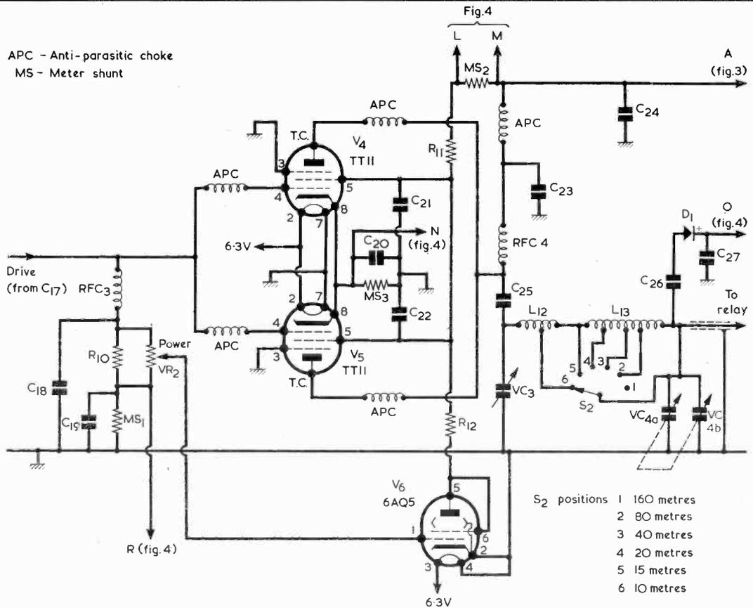
Fig. 2. The p.a. stage and output circuit. V6 is a clammer valve and reduces p.a. current in the absence of drive
