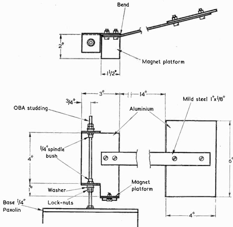
Fig. 3. Top and side views of the prototype weather-vane assembly constructed by the author
