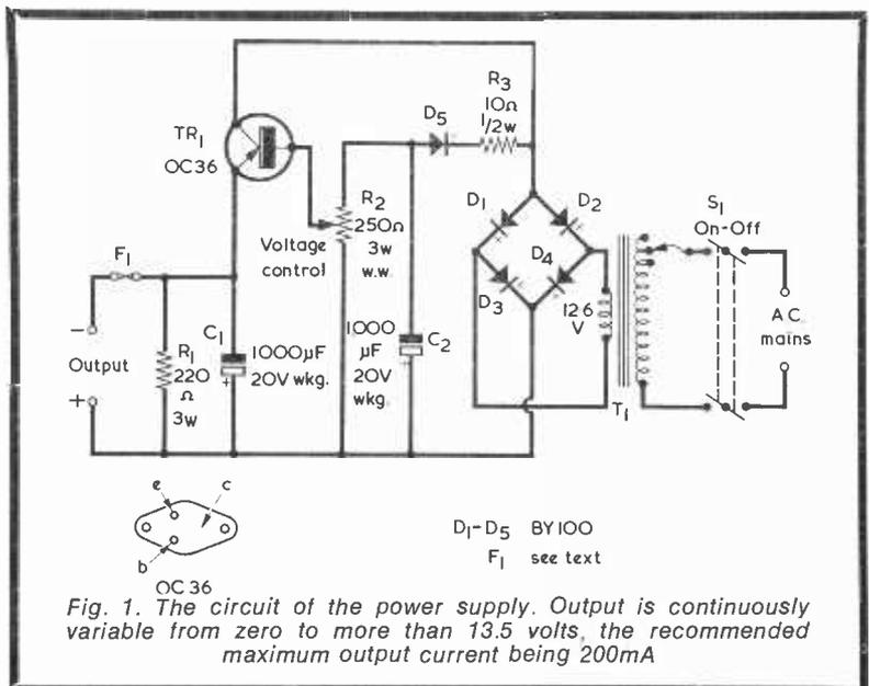
BY100 is widely available at low cost and the alternatives would provide no significant improvement in performance.
