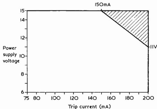
Fig. 2. The shaded area indicates the power supply voltages and trip currents which may require the fitting of an extra limiter resistor, as described in the text
