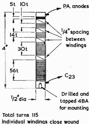
Fig. 7. Winding details for RFC4. The prototype used a solid former. If a tubular former is employed an alternative means of mounting it vertically to the chassis must be provided
