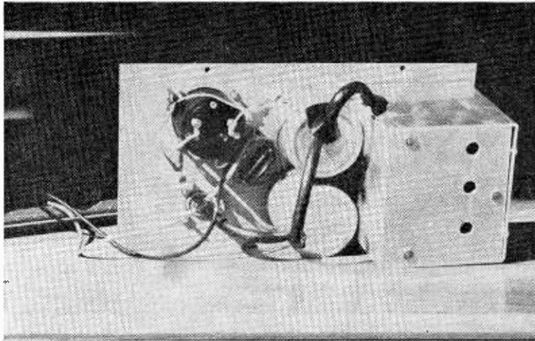
*The rear of the front panel. The large screening cover encloses the transistor circuitry*
