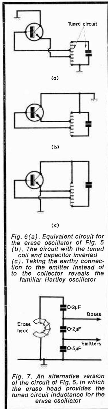
Fig. 6(a). Equivalent circuit for the erase oscillator of Fig. 5 (b). The circuit with the tuned coil and capacitor inverted (c). Taking the earthy connection to the emitter instead of to the collector reveals the familiar Hartley oscillator
