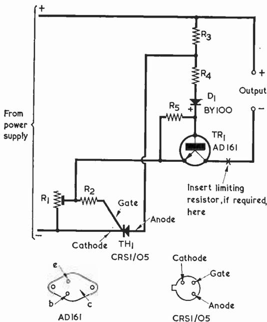
Fig. 1. The circuit of the overload trip
