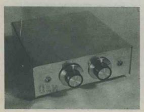
An inexpensive general purpose a.f. amplifier which will be particularly useful for experimental, testing and servicing work
