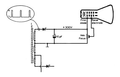
Fig. 6. Flyback rectification is used to feed the tube first anode and the focus potentiometer
