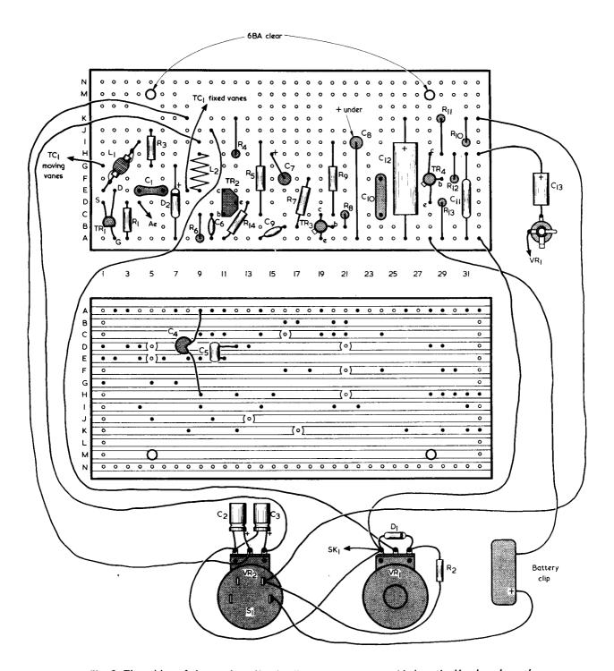
Fig. 2. The wiring of the receiver. Nearly all the parts are assembled on the Veroboard panel
