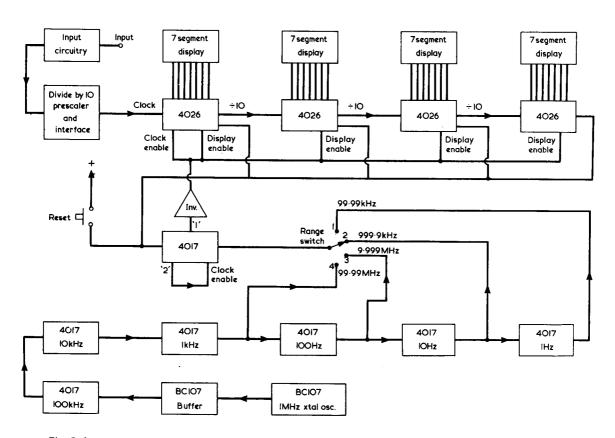
Fig. 2. In practice the frequency meter is more complicated than is evident from Fig. 1. However, the use of integrated circuits simplifies construction to a considerable extent
