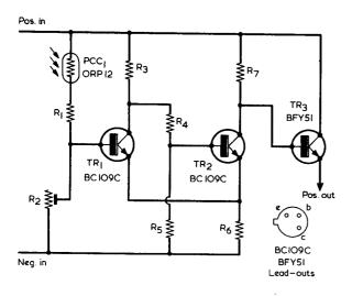
Fig. 2. The auto-dimmer circuit. TR1 and TR2 form a Schmitt trigger which is actuated by the voltage on TR1 base. TR3 is an emitter follower feeding the clock circuit
