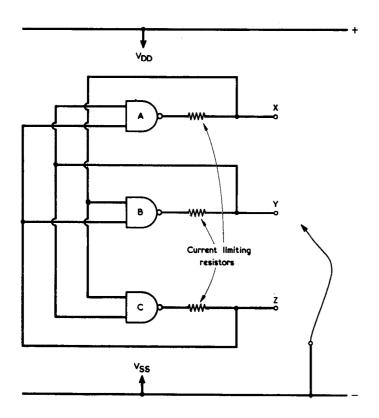
Fig. 2. Adding output current limiting resistors enables the circuit to be changed from one state to enother
