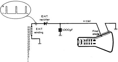
Fig. 4. The e.h.t. section of the line output stage. In most receivers the e.h.t. reservoir capacitor is given by the capacitance between the inside and outside graphite coatings of the picture tube. In this receiver a 1,000pF capacitor is added in parallel
