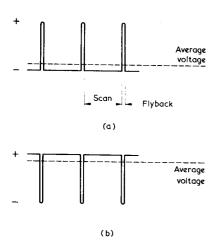
Fig. 5. According to the way connections are made to it. e winding on a line output transformer may produce flyback pulses which are positive-going with respect to chassis, as in (a), or scan pulses which are positivegoing, as in (b)
