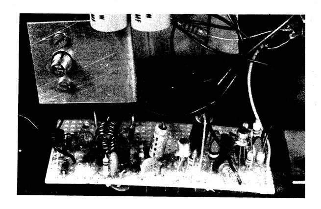
Detail illustrating the Veroboard assembly more closely. The board was not bolted to the case when this shot was taken
