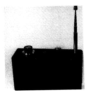
Another view of the receiver. The telescopic aerial is slightly more than one metre in length when it is fully extended
