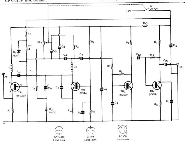
Fig. 1. The circuit of the single tuned circuit f.m. receiver. Tuning is carried out by VR1 and varicap diode D2
