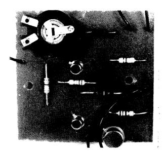
The auto-dimmer components assembled on their printed board
