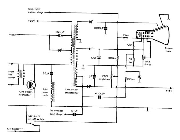
Fig. 2. Line output stage of a monochrome mains/battery television receiver. (This is a slightly simplified version of the circuit employed in the Thorn 1590-1591 Series of television receivers.)
