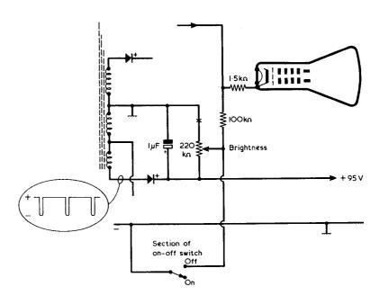
Fig. 7. The higher current 95 volt supply for the video output stage is provided by scan rectification. The cross indicates the position of the open-circuit in the faulty brightness control potentiometer
