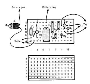
Fig. 3. Most of the components are wired up on a small Veroboard panel, employing the layout shown here
