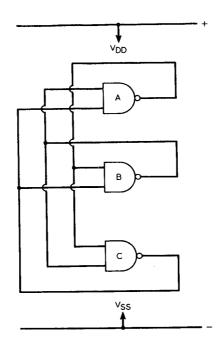
Fig. 1. Theoretical circuit incorporating three CMOS NAND gates. The circuit has three stable states
