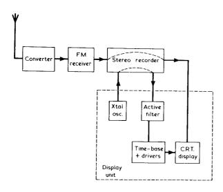
Block diagram of Satellite Receiving set up
