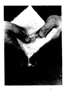
Araldite from a 200 gram sachet being poured to form a small potted assembly. The resin and hardener are in separate halves of the sachet, being brought together just before use by removing a clip
