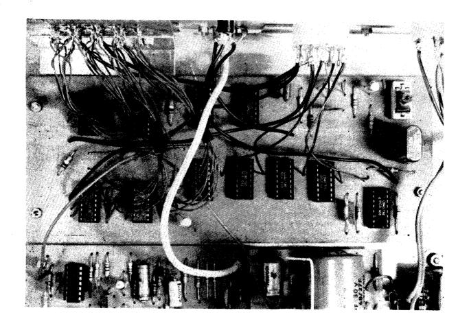
The main board with the divider and counter i.c.'s. The leads from this travel to the pins of the l.e.d. displays
