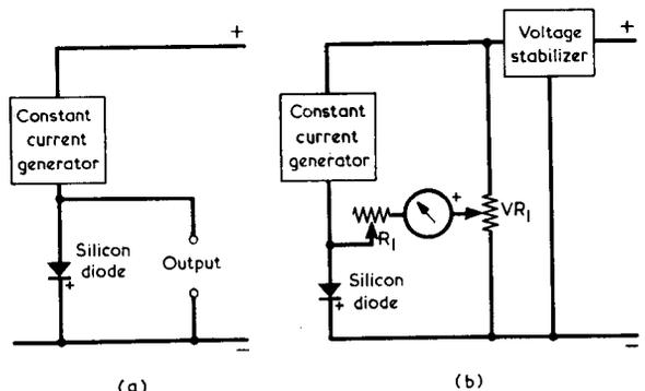
Fig. 1(a). In this circuit the voltage across the silicon diode varies in linear fashion with the diode temperature
