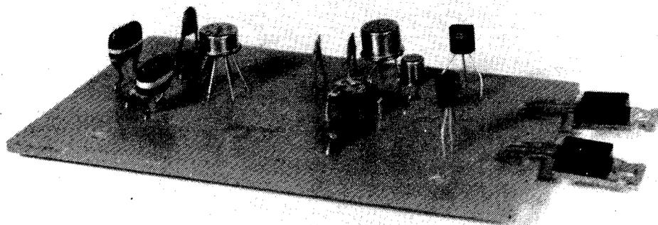
*The d.c. coupled amplifier module. The two output transistors appear at the extreme right*
