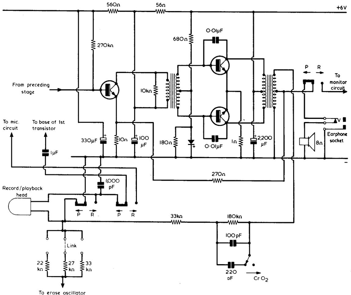
Fig. 4. The a.f. driver and output stages of the cassette recorder. The monitor circuit consists of a switch and several attenuating resistors which permit the earphone or speaker to monitor the output signal during recording. The three sections of the record-playback switch are shown in the "Playback" position. This, and Fig. 2, are slightly simplified versions of the corresponding sections in the Ferguson 3276 cassette recorder.
