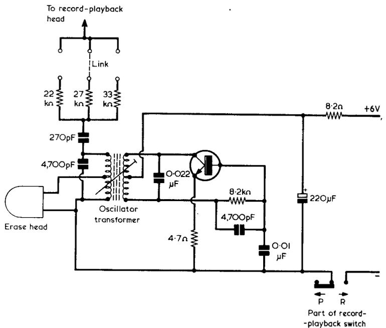
Fig. 2. The erase oscillator circuit in the cassette recorder serviced by Dick
