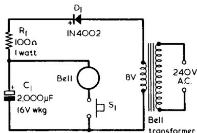
Fig. 2. Running costs are reduced to a negligible level if the single ping circuit is powered by a bell transformer.
