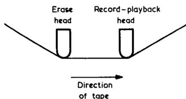
Fig. 1. The tape in the cassette recorder passes the erase head and then the record-playback head. During recording the erase head is actuated and erases any signal which is present on the tape before it reaches the record-playback head
