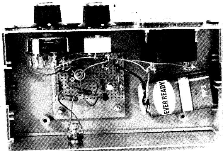
on for long periods but will only be turned on when a reading is to be taken, a small 9 volt battery such as a PP3 is a perfectly suitable power source for the unit.
