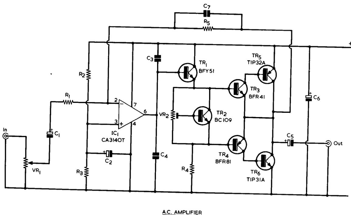
*Fig. 4. The a.c. version of the amplifier requires only a single supply rail. There are d.c. blocking capacitors at the input to the integrated circuit and at the output to the speaker*
