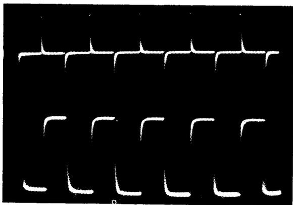
Waveforms with a high level 1kHz square wave input. Only super-sonic harmonics are fed to the inverting input and the output shows little evidence of high frequency attenuation
