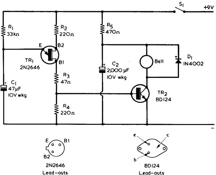
Fig. 3. A circuit which causes a series of pings to be sounded at approximately 3 second intervals
