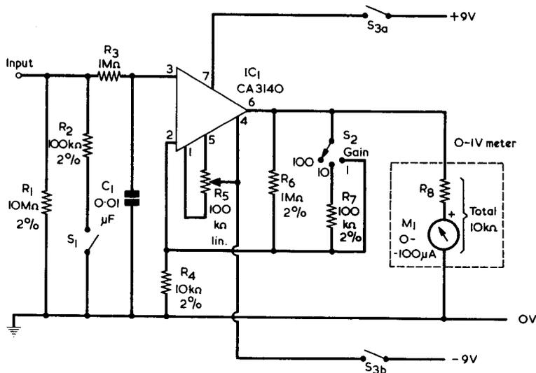
consist of employing a centre-zero 100-0-100 $\mu$ A meter movement; the circuit could then measure input voltages and currents of either polarity.
