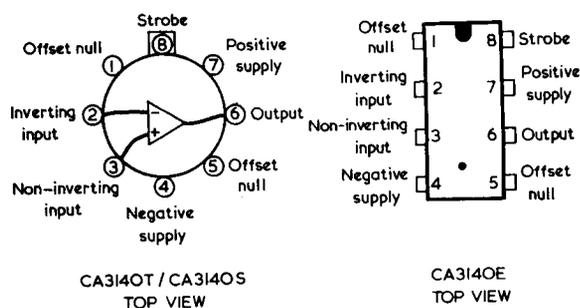
Fig. 1. Pin connections for three versions of the CA3140
