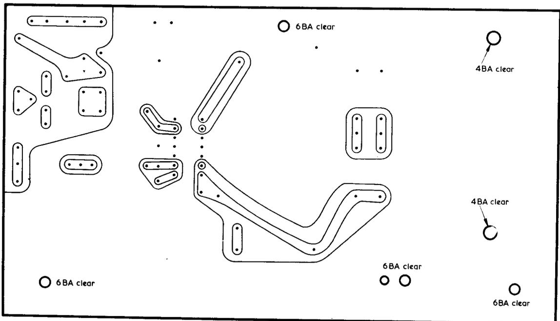
Fig. 3. Details of the printed circuit board, which is reproduced full size. The large copper area at chassis potential provides heatsinking for IC1
