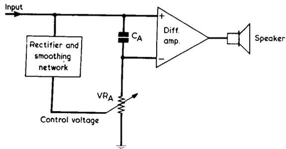
**Fig. 1. The basic manner in which the noise reduction amplifier functions. The resistance of VRA reduces with increasing input signal voltage, causing less high frequency content to be present at the inverting input of the amplifier**
