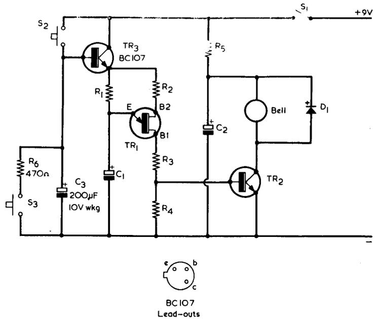
Fig. 4. The circuit of Fig. 3 adapted as a door bell. The pings continue to sound for about 1½ minutes after S2 is pressed
