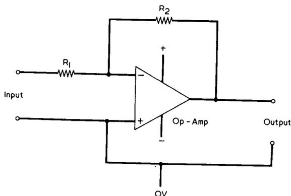
**Fig. 2. The basic d.c. coupled inverting input operational amplifier configuration**
