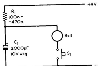
Fig. 1. A simple battery operated circuit. The bell gives a single ping when the push-button is pressed
