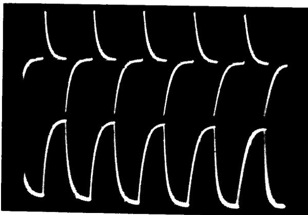
Waveforms at the inverting input (upper) and the output (lower) given with a low level 1kHz square wave input
