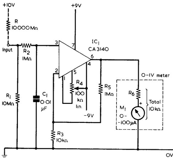
Fig. 2. Simple operational amplifier circuit capable of low current and voltage measurements
