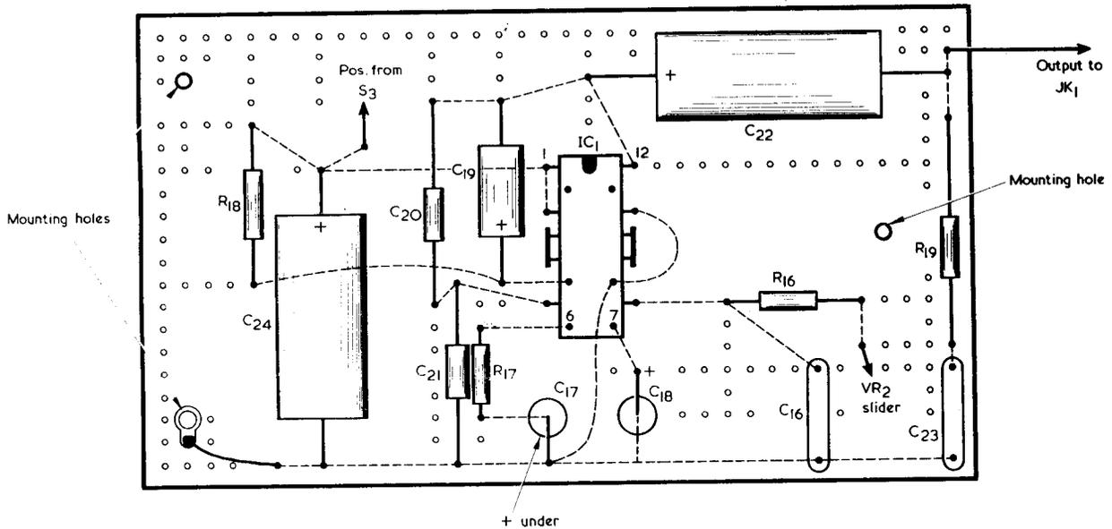
Fig. 8. The audio amplifier board is wired as shown here. Wiring under the board is reproduced in broken line
