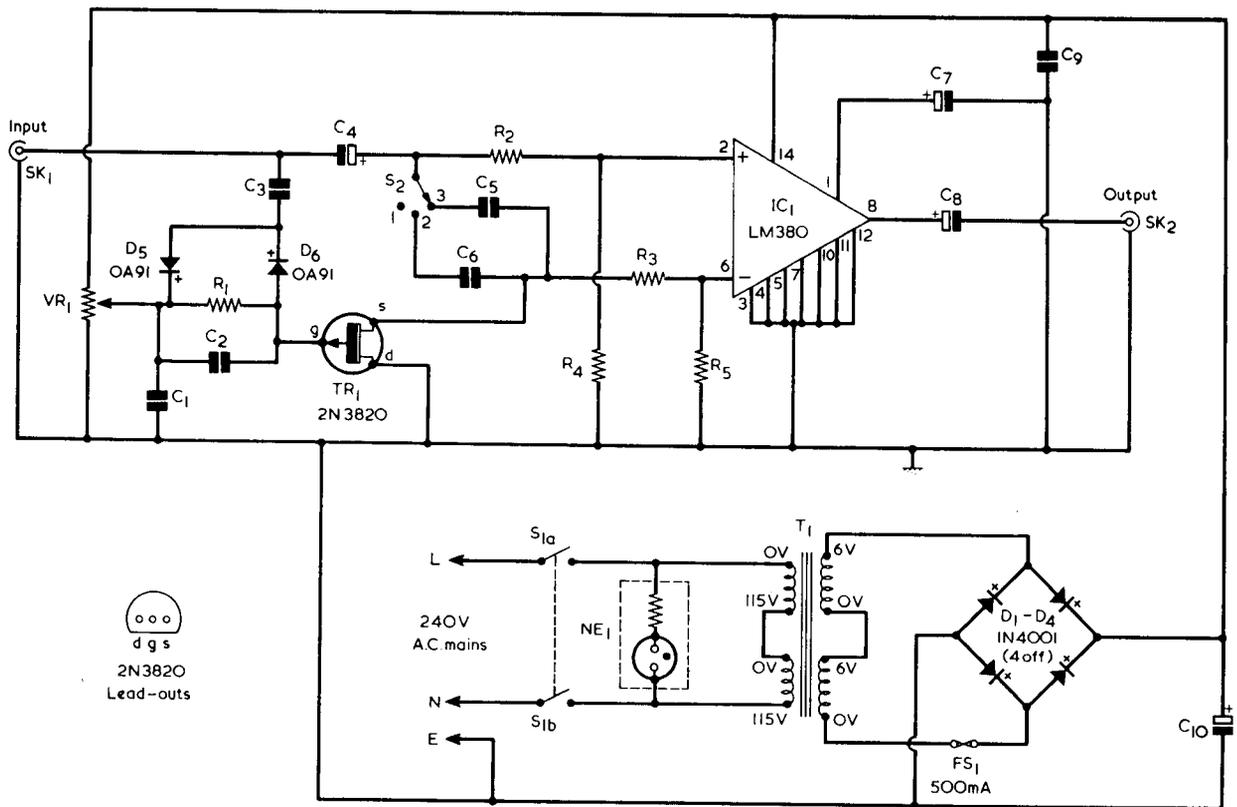
Fig. 2. The complete circuit of the noise reduction amplifier. The use of an integrated circuit audio amplifier considerably reduces complexity
