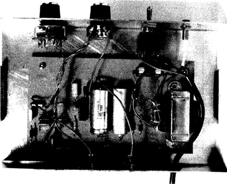
*Looking inside the amplifier case. Wires from the printed board to the front panel components may, for neatness, be lightly twisted together as shown here*
