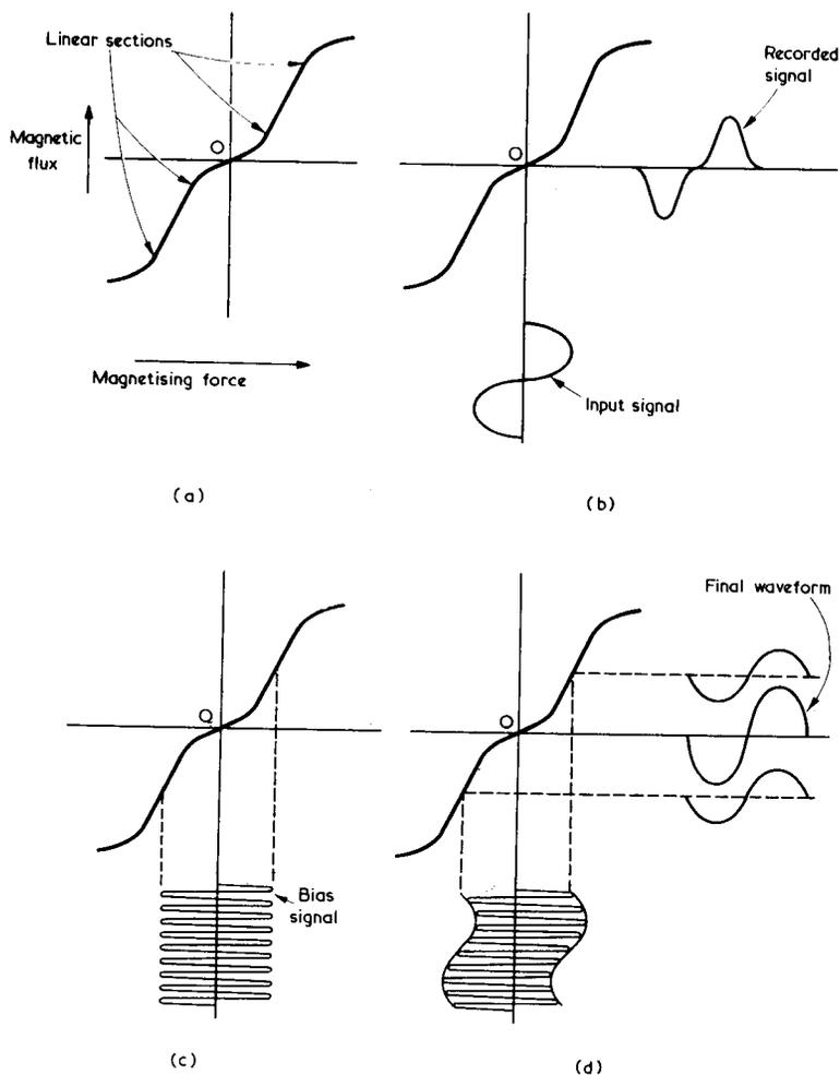
Fig. 3(a). Characteristic curve illustrating magnetising force, provided by the record head, and the consequent magnetic flux in the tape
