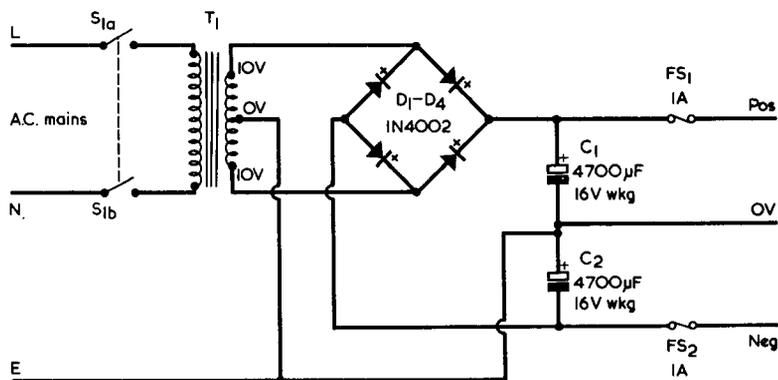
As shown, the power supply of Fig. 6 offers the positive and negative rails for the d.c. version of the amplifier. With the exception of the centre rail, the
