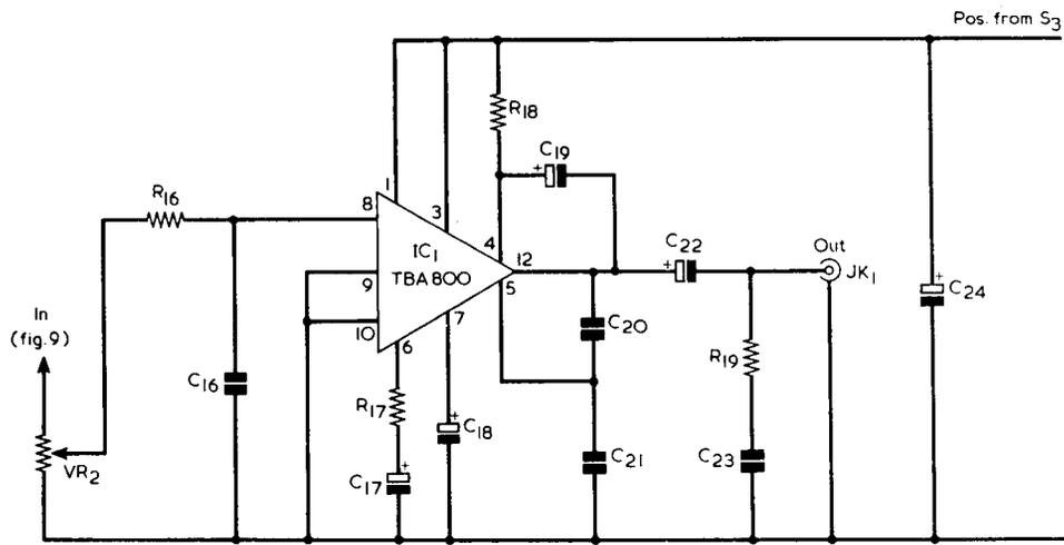
**Fig. 7. The circuit of the a.f. amplifier section**
