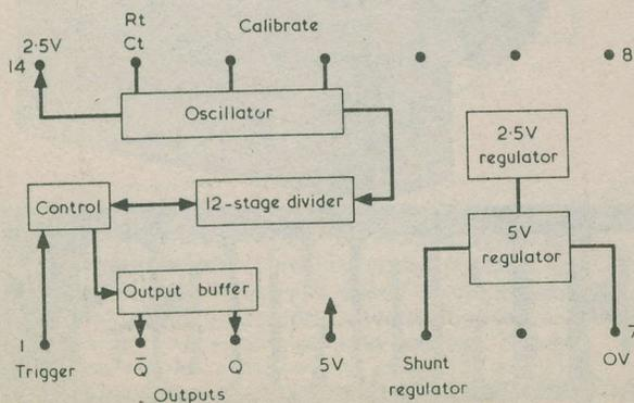
Fig. 1. The main internal functions of the ZN1034
