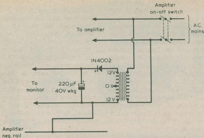
**Fig. 4.** The monitor can be powered by an inexpensive supply incorporating a low-cost mains transformer. The same supply can also be used for the second monitor in a stereo system
