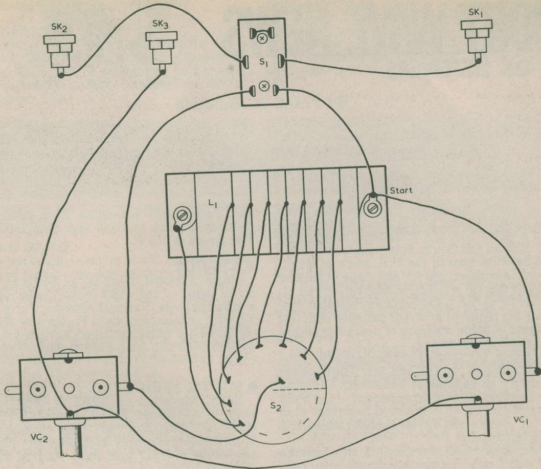
**Fig. 3. Wiring up the aerial tuning unit. The wires should be kept reasonably short and direct**
