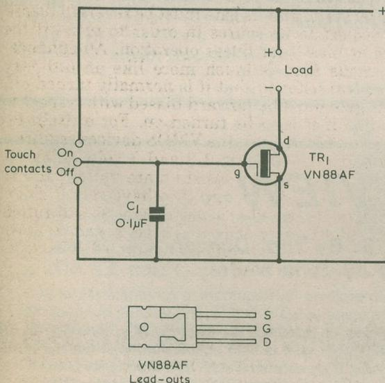
Fig. 2. A very simple touch switch incorporating a VMOS transistor. If leakage resistances are kept very high the circuit remains almost indefinitely in the on or the off state
