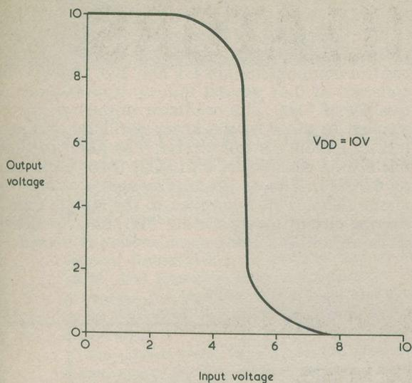
Fig. 3. Typical transfer characteristic for a CMOS inverter
