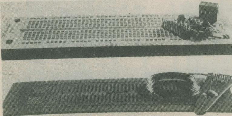
*The continental Specialties Corporation Experimentor system of solderless bradboard and, underneath, the matchboard pre-drilled*
