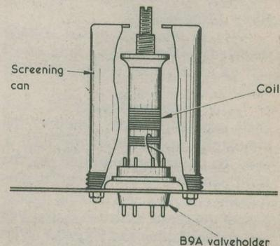
Fig. 1. Denco plug-in coils are supplied in an aluminium container with a screw-on lid. If the lid is secured under the valveholder into which the coil is plugged, the container may then be screwed into it to form a screening can
