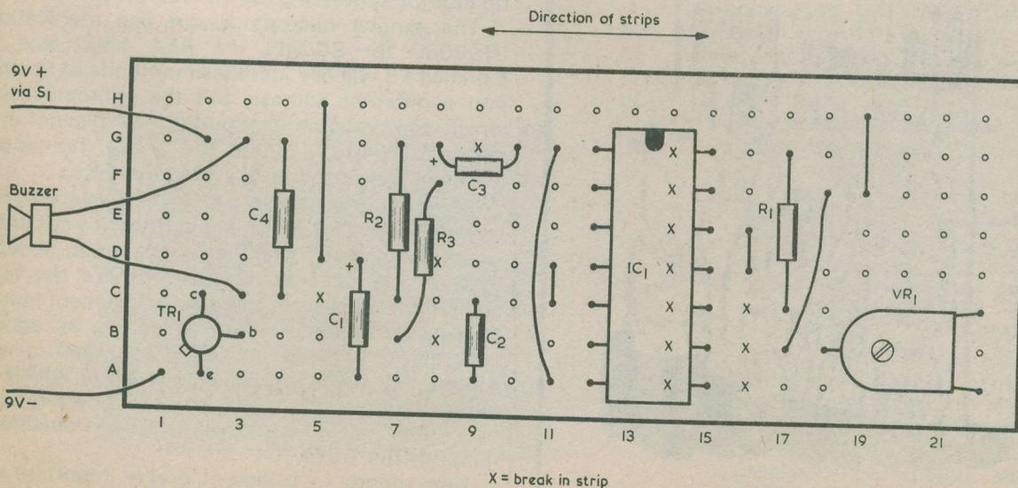
Fig. 3. The component side of the Veroboard assembly employed in the prototype
