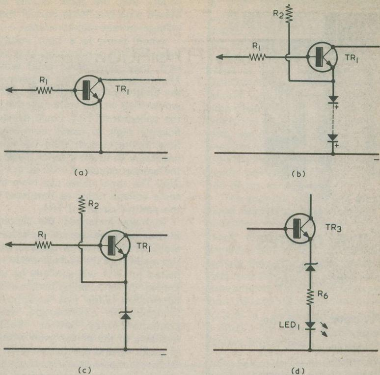
**Fig. 2(a)** If D1 and R2 are omitted, and the emitter of TR1 is connected direct to the negative rail, the voltage delay at TR1 base is 0.6 volt only
