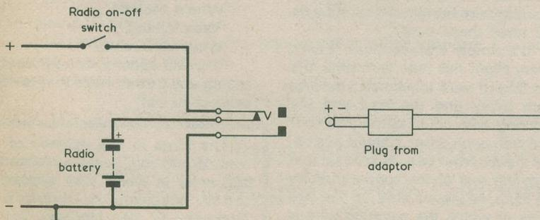
Fig. 9. Using a low-cost pocket calculator mains adaptor to power a small radio. It is necessary to find the polarity and voltage available at the adaptor output plug before using it with the receiver. Not all calculator adaptors may be suitable for this application
