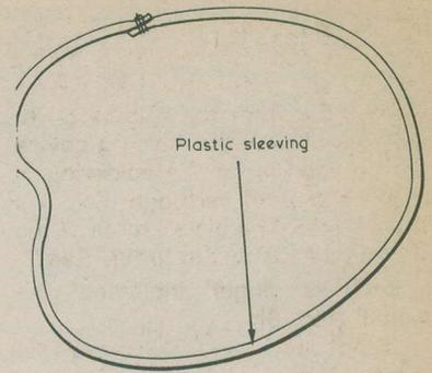
Fig. 7. A driving belt made up from tough plastic sleeving. The belt will be found a suitable replacement in many reel-to-reel tape recorders
