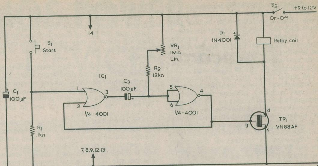
Fig. 3. A timing circuit in which the output of a CMOS gate couples directly to the gate of the VMOS transistor. The loading placed on the CMOS output is negligibly low
