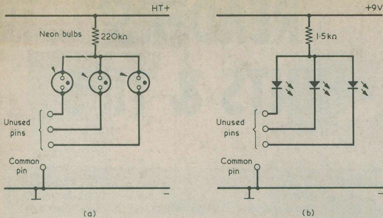
**Fig. 2(a).** The three neon bulbs are wired to the B9A valveholder so that each lights up when one of three separate coils is plugged in. The series resistor has a value suitable for h.t. voltage of around 150 to 200 volts
