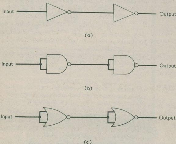
Fig. 1(a). Two CMOS inverters connected in tandem. The output is in phase with the input (b). NAND gates may be employed to act as inverters (c). The inverters may also consist of NOR gates
