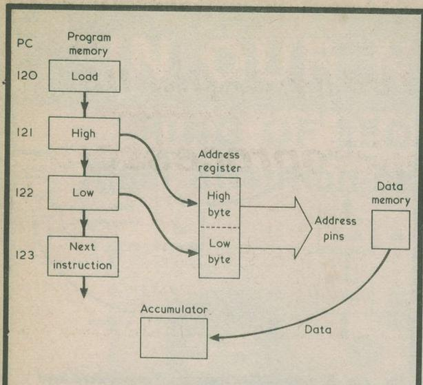
*Fig. 2. Direct addressing. The instruction code is followed by two bytes which are assembled into a 16-bit number in an address register. This is then gated to the address pins, causing data to be released from the memory with that address. The data on the data lines is gated into the accumulator, completing the instruction*
