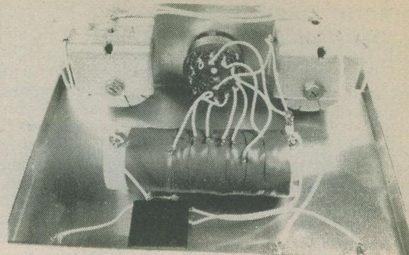
with about the same dimensions can be employed. An alternative is a length of 1in. diameter timber, such as a piece cut from a broom handle. Provided that it is dry this will have more than adequate insulation resistance for the present purpose.
