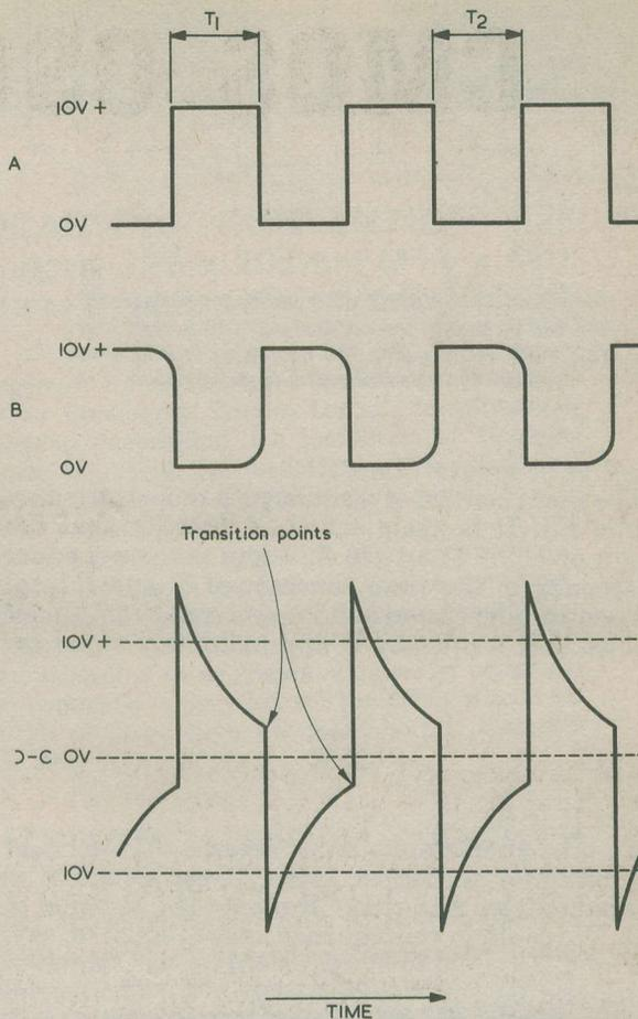
Fig. 5. Waveforms appearing in the oscillator circuit of Fig. 2. The bottom waveform shows the voltage at point D with respect to point C
