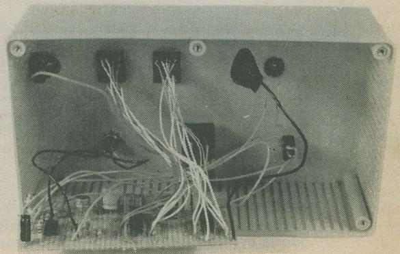
*Here, the Veroboard panel is secured in place. After the battery has been fitted, the rear panel is mounted in position on the case*
