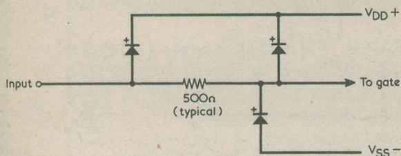
Fig. 4. CMOS logic gates have diode input protection circuits
