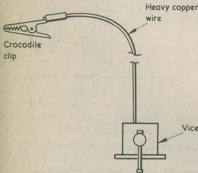
Fig. 8. A "third hand" for holding components during soldering. The copper wire can be bent to place the crocodile clip in any desired position
