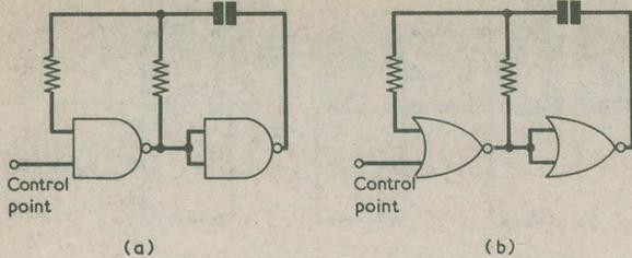
Fig. 6(a). This NAND gate oscillator may be inhibited by taking the control point to a logic low
