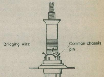
**Fig. 3.** The bridging wire is soldered to the appropriate coil pins in the manner shown here
