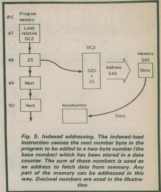
**Fig. 5. Indexed addressing.** The indexed-load instruction causes the next number byte in the program to be added to a two-byte number (the base number) which has been stored in a data counter. The sum of these numbers is used as an address to fetch data from memory. Any part of the memory can be addressed in this way. Decimal numbers are used in the illustration
