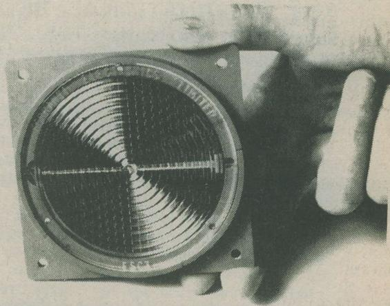
*The Ferranti ESC3 Solar Cell which will produce 0.9A at 0.5V under good sunlight conditions. Ferranti Electronics Limited have developed the cell specifically for educational use, although there are obvious DIY applications*
