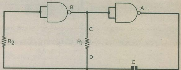
Fig. 2. Recommended CMOS oscillator circuit. NAND gates are shown here, but the circuit will function equally well with inverters or NOR gates
