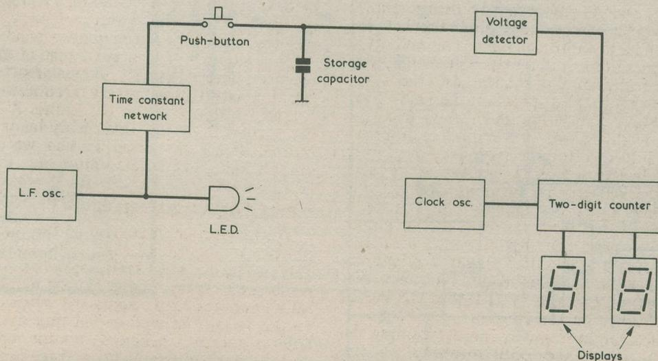
*Fig.1. Basic line-up of the "Tantaliser" game. The low frequency oscillator produces a square wave which lights the l.e.d. when the output voltage is low. The purpose of the game is to manipulate the push-button such that the storage capacitor becomes charged sufficiently to trigger the voltage detector. The latter then stops the two-digit counter*
