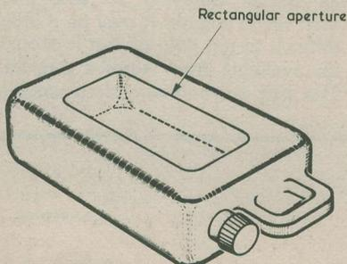
Fig. 5. A home-made bath for printed circuit etching is made from a supermarket lemon squash container
