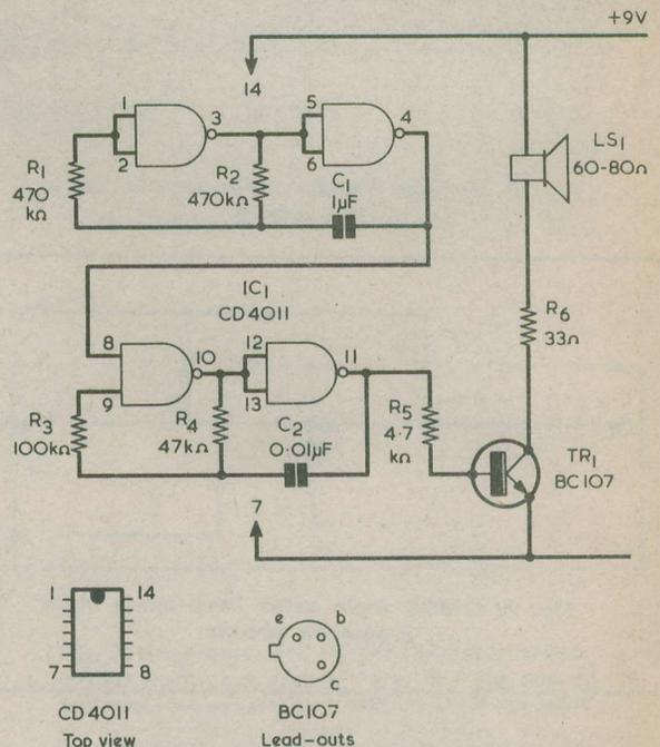
Fig. 7. A 1-second bleeper circuit incorporating a CD4011. All the resistors may be 1/2 watt 5%. The function of R6 is merely to limit collector current in TR1
