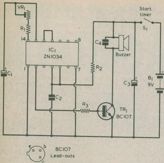
Fig. 2. The circuit of the parking meter reminder timer. This causes the buzzer to sound after 50 minutes
