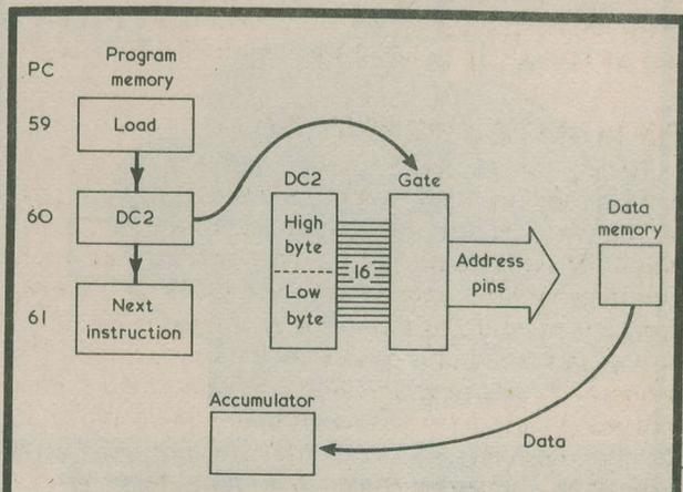
*Fig. 3. Implied addressing. A two-byte address is stored in a data counter, DC2 in this example. The instruction to load, implied, followed by the code address of the data counter causes the number stored in DC2 to be gated to the address pins so that it fetches data from that memory address into the accumulator*
