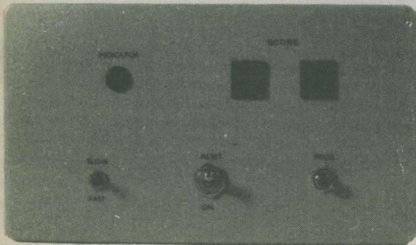
*In the prototype the flashing l.e.d. is situated upper left on the front panel. To its right are the two 7-segment displays. Below, S3 is mounted centrally with S1 to its left and S2 to its right*
