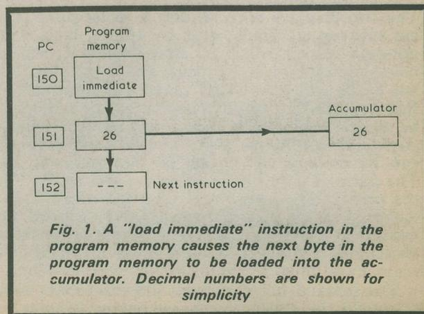
*Fig. 1. A "load immediate" instruction in the program memory causes the next byte in the program memory to be loaded into the accumulator. Decimal numbers are shown for simplicity*
