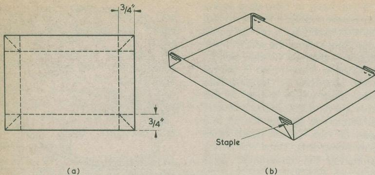
Fig. 4(a). A rectangle of plastic cut from a plastic container is marked up as illustrated
