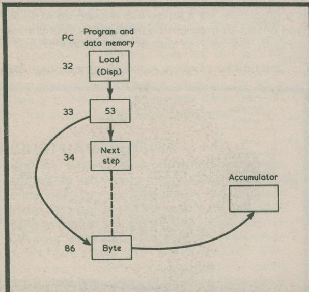
**Fig. 4. Program-relative addressing.** When the program-relative load instruction is used, the next byte in memory is added to the number which is in the program counter register, and the sum is used as a memory address. The address number must be fairly close (128 steps or less) to the step in program where this instruction is used
