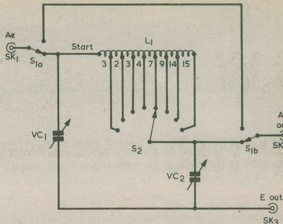
Fig. 2. The practical a.t.u. circuit requires variable inductance in addition to variable capacitance, and this is provided by tapings in the coil which are selected by S2. The numbers indicate the number of turns in each section of the coil
