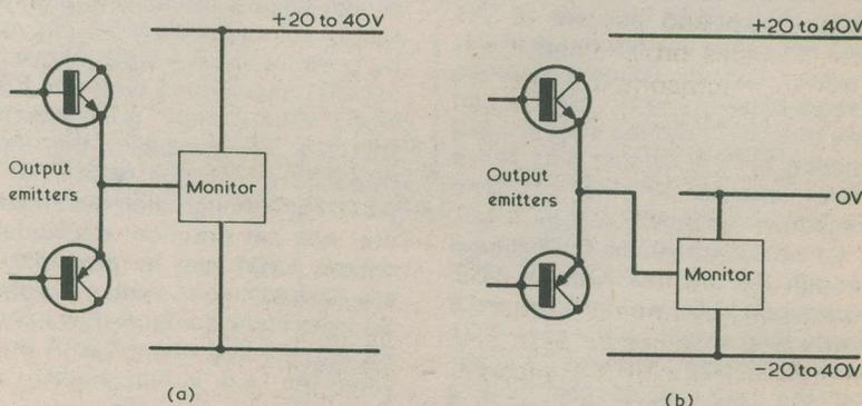
Fig. 3(a). With amplifiers having two supply rails the monitor is connected as shown here
