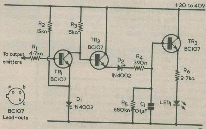
Fig. 1. The basic circuit of the clipping monitor. The single silicon diode in the emitter circuit of TR1 causes the l.e.d. to light up when the output emitters have a voltage which is less than 1.2 volts positive of the negative rail
