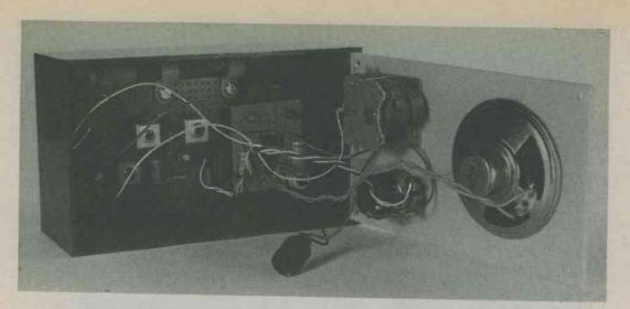
The tuning capacitor, volume control/on-off switch and speaker are mounted on the front panel. The main component board is bolted to the rear panel of the case.
