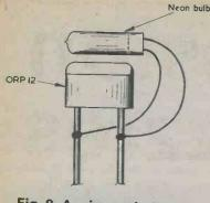
Fig. 8. A wire-ended neon bulb soldered to the leads of a photoconductive cell. (This arrangement was originally described by G. A. French in the May 1970 issue.)
