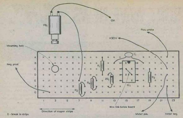
Fig. 3. The booster Veroboard layout. The bush of PB1 passes through the mounting hole and secures the board to the lid of the plastic case in which the booster is housed.
