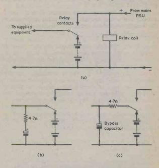
Fig. 1(a). Relay circuit which gives automatic transfer to battery operation when the mains supply fails. The relay moving contact is shown in the de-energised position.
