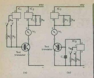
Fig. 2(a). The test circuit which is set up when an n.p.n. transistor is connected to the meter.
