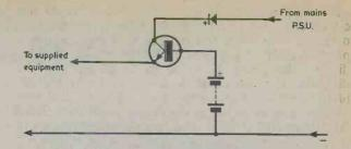
Fig. 3. Another solid-state circuit which gives automatic changeover.
