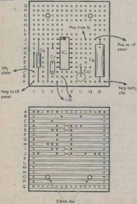
Fig.3. The a.f. amplifier board. This is bolted to the main component board.
