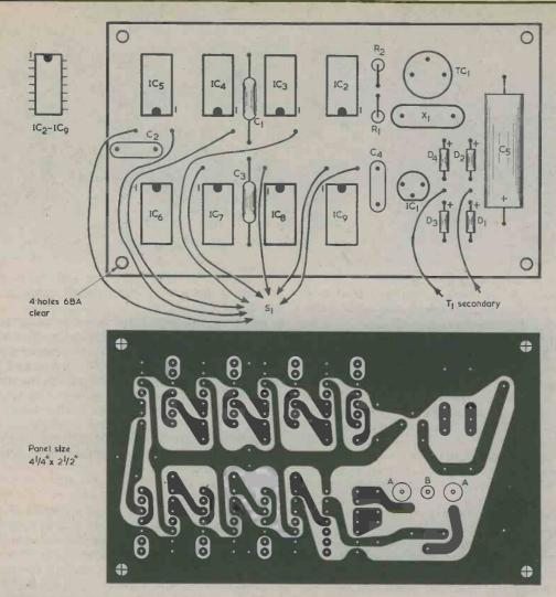
Fig. 2. The component and copper sides of the printed circuit board. This is reproduced full size.
