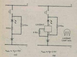
Fig. 4(a). If the l.e.d. in this circuit fails to light when the push-button is pressed the supply voltage is below the Vmin level.
