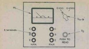
Fig. 4. A recommended front panel layout for the hFE meter. Connections to test transistors are made by way of short flexible leads terminated in small crocodile clips.
