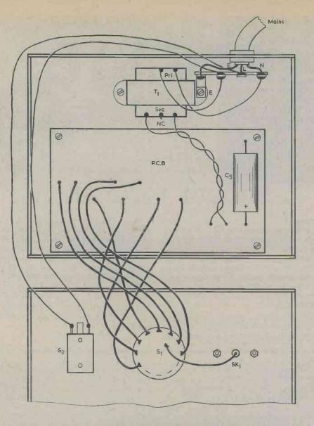
Fig. 3. The mains input wiring and the external connections to the printed circuit board.
