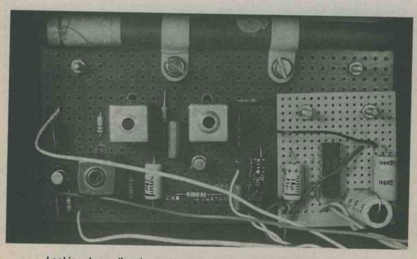
Looking down directly on the main component board and the smaller a.f. board. The ferrite aerial is secured to the main board.
