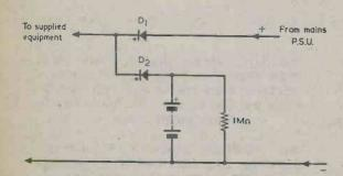
Fig. 2 Automatic changeover to battery operation is given by the two steering diodes. The mains supply voltage is higher than the battery voltage.
