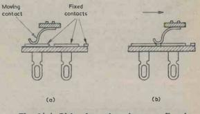
Fig. 2(a). Side view showing two fixed contacts in a typical make-before-break rotary switch.
