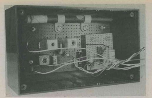
The main component board is of 0.15in. matrix, which is reasonably compatible with the pins and mounting lugs of the i.f. transformer's and oscillator coil. A small sub-assembly board, of 0.1in. matrix, carries the a.f. amplifier i.c. and its immediate components.
