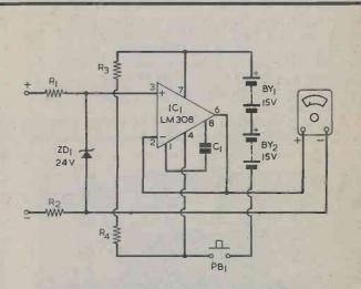
Fig. 2. The circuit of the voltmeter sensitivity booster. This employs an LM308 as a voltage follower, with protection against excessive input voltages being provided by ZD1. The multimeter should, preferably, have a sensitivity of  $10,000\Omega$  per volt, or better.
