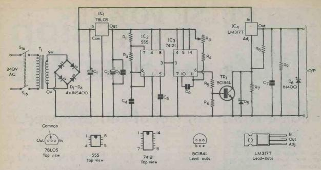
Fig. 3. The full circuit of the pulse power supply. IC2 triggers IC3 into producing a series of positive pulses whose width is controlled by R3.
