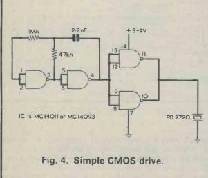
Fig.4: is also a continuous tone circuit but built this time from a single CMOS quad Nand gate.
