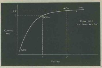
Fig. 3. Positive Temperature Coefficient. Although the resistance is different at each point of the graph, the volts, amps and ohms still obey Ohm's Law.
