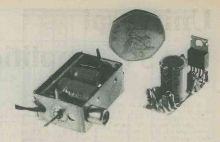
Photo of Universal Amplifier PCB, and when mounted in screening can.
