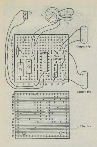
Figure 2. The component and copper sides of the Veroboard panel, on which most of the components are assembled. The output clip connects to the battery clip of the radio, hence its apparent reversed polarity.
