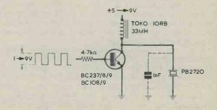
Fig. 6. An inductive voltage multiplier for increased output.
