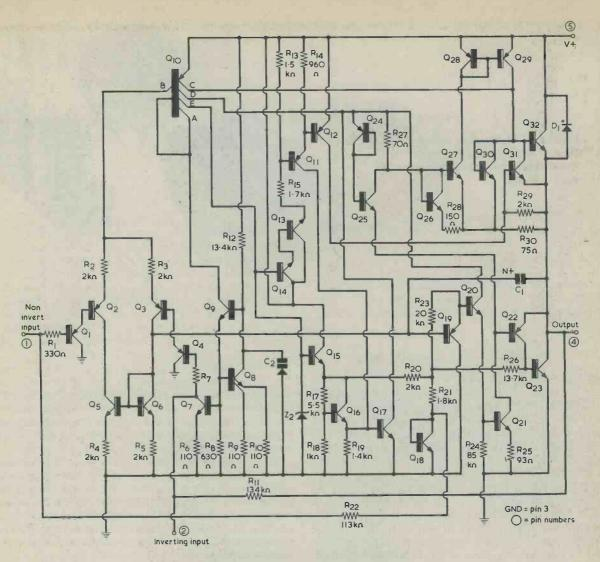
Fig. 3. TDA 2002 internal circuit diagram.
