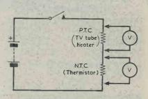
5. When switched on the heater and thermistor are cold. The heater is therefore low resistance, but the thermistor is high resistance and prevents any damaging current surge.
