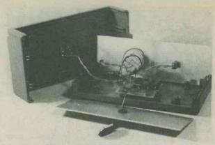
The prototype timer unit with the case disassembled. The Veroboard panel is mounted on the case bottom.
