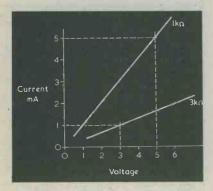
Fig.2. Smithy shows the straight line or 'linear' between relationship voltage and current for fixed values of resistance.
