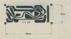
Fig. 4. PCB layout. Scale 4:1.
