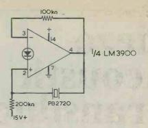
Fig. 5. Using a spare 'Op-amp' section.
