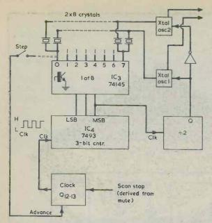
Fig. 2. The automatic scanning logic. Sixteen channels can be scanned in two separate bands of eight. The frequency coverage of each band is determined by the choice of crystals and coils, explained in paragraph "The RF/IF/AF sections".
