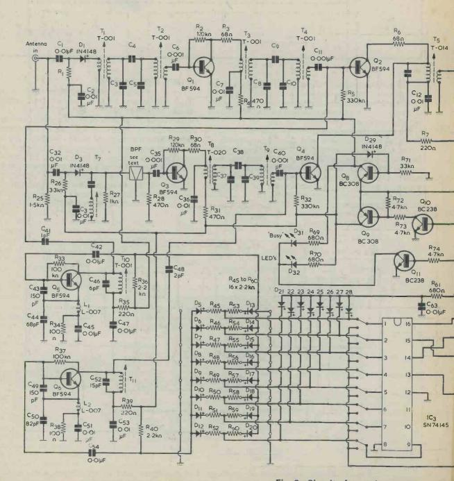
Fig. 3. Circuit of complete receiver. Deta
