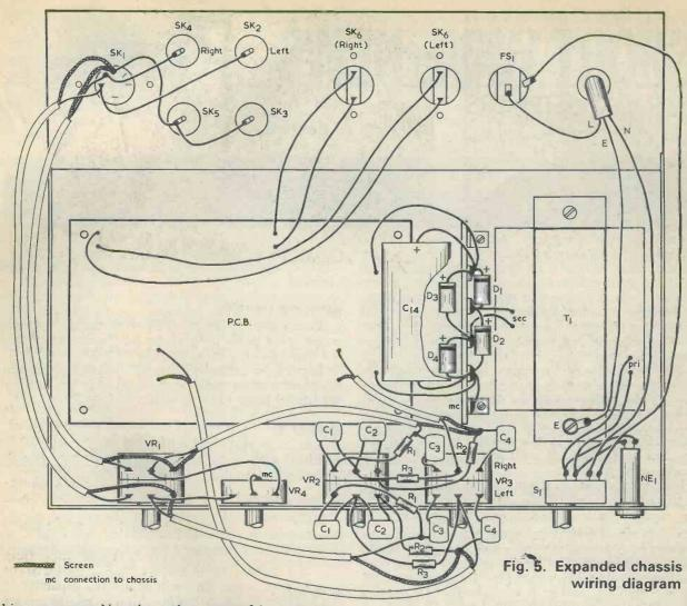
this component. Note that only one tag of the tag strip is earthed and has wiring going to it. For safety reasons the exposed tags of the fuseholder, neon and mains switch should be insulated with tape. Also ensure that the centre tag of the fuseholder cannot touch the case of the transformer.
