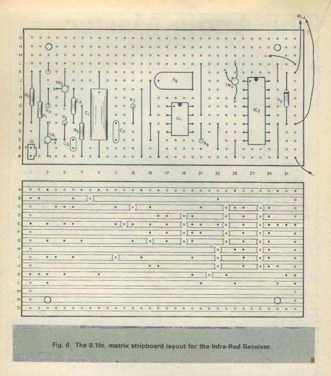
be facing the hole, and this is opposite the face with writing on. If D1 is mounted direct on the component panel its leads must be bent through 180 degrees in order to face the sensitive surface away from the panel. The unit should not be positioned where it will pick up strong mains hum that could cause spurious operation.
