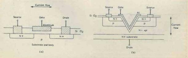
Fig. 1. (a) Cross section of Conventional Mosfet (b) Cross section of Vmos device
