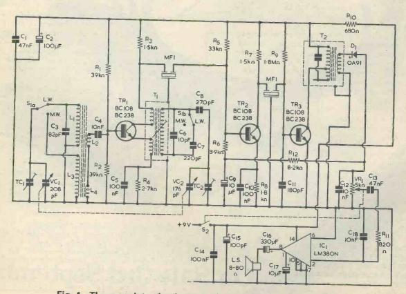
Fig. 1. The complete circuit diagram of MW/LW superhet radio.
