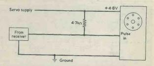
Fig. 6. Using a 'pull-up' resistor at the servo input in cases of marginal operation.
