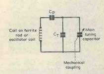
Fig.3. Smithy sketched a simple tuned circuit and added two extra preset capacitors ... Cp is the 'padder' which can effectively reduce the maximum value of the main tuning capacitor. Ct is the 'trimmer' which can effectively increase the minimum value of the main tuning capacitor. By adjusting Cp set the trimmer, again for maxand Ct the overall tuning range can be imum signal. Repeat once altered.
