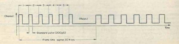
Fig. 1. The control waveform at the encoder output and decoder input.
