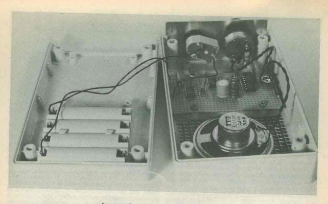
Layout showing built-in battery box.
