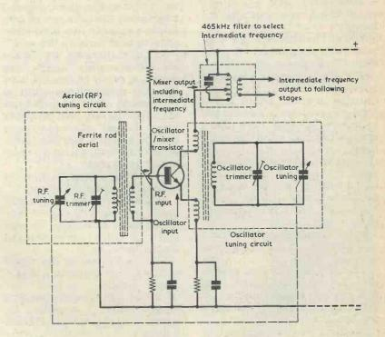
Fig.1. Smithy's sketch of a simple Oscillator/Mixer stage shows the first important sections of Dick's 'tranny' superhet radio. The variable capacitors are 'ganged' together and each has an additional trimmer capacitor to help with the 'tracking'.
