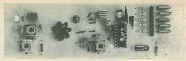
The completed transmitter board. (Actual size)
