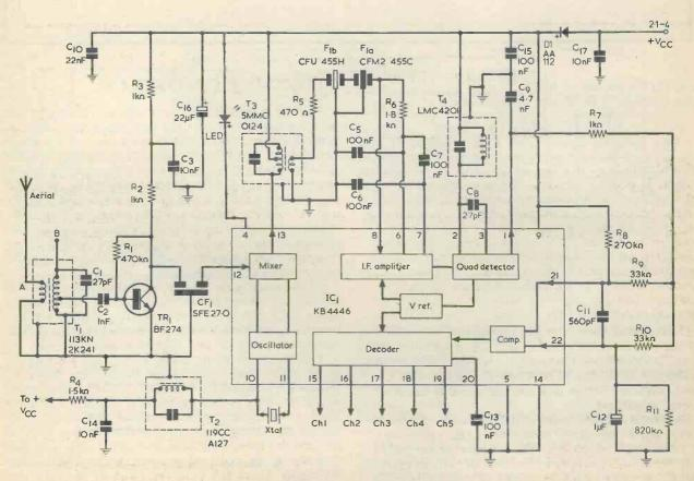
Fig. 5. The receiver circuit.
