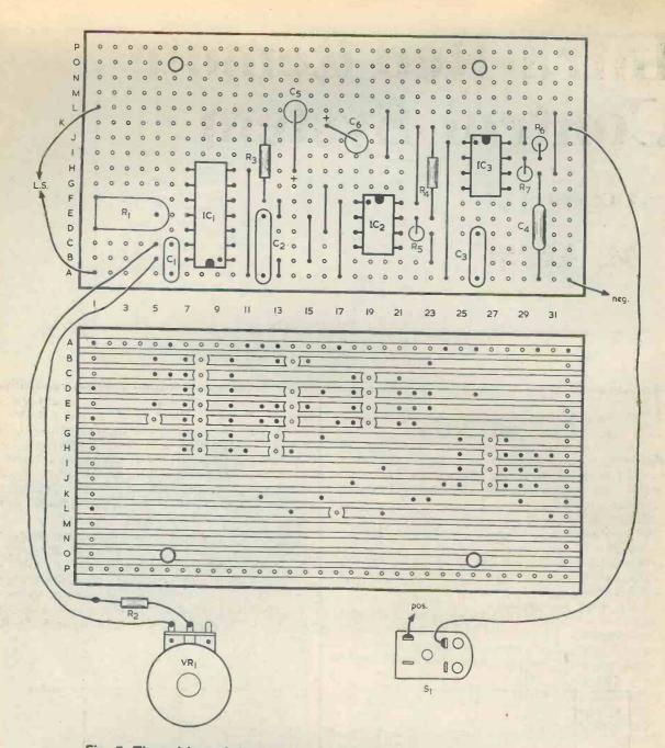
Fig. 5. The wiring of the Timer and details of the component panel.
