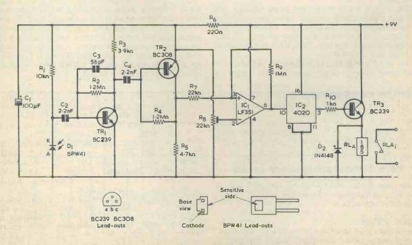
Fig. 4. The circuit diagram of the Infra-Red Receiver.
