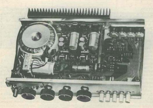
The unit assembled in the chassis.
