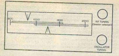
Fig.2. Smithy's idea of the tuning arrangements for a hard-to-tune superhet which nevertheless could achieve perfect tracking. The top pointer is set to select the station. The bottom pointer is then set to be 465kHz higher.
