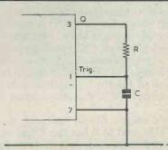
Fig. 3. By coupling the Q output to the trigger terminal, the circuit will continuously retrigger itself.
