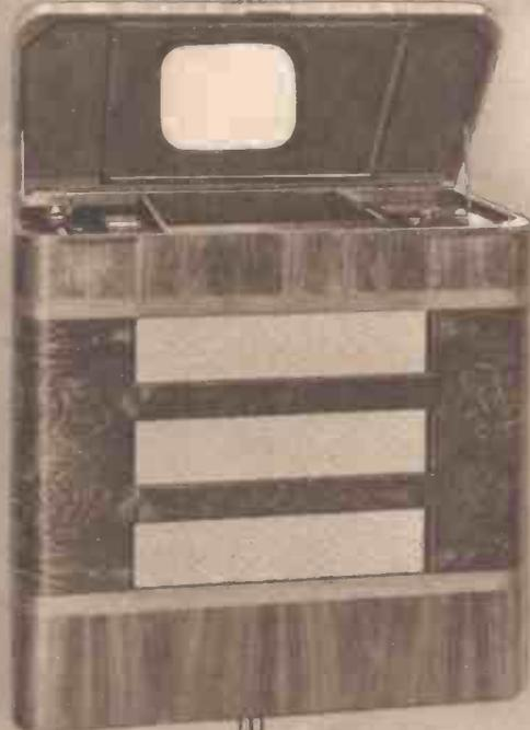
All major controls are mounted on instrument panels on either side of the vertically mounted tube. In this G.E.C. instrument the picture is viewed from a mirror mounted in the lid
