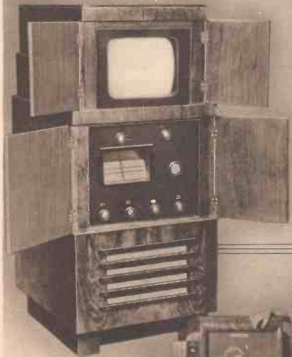
One of the most popular receivers is the Cosmor 137T which has most of the controls preset at the back of the cabinet. An all-wave radio receiver is also included
