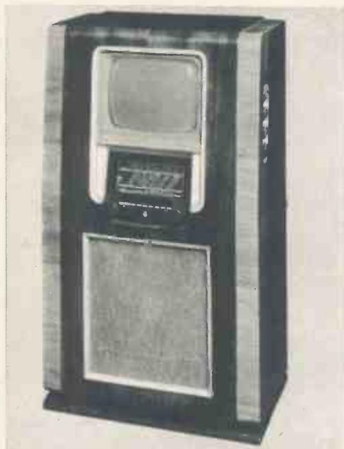
Philips Television 1939/40 Type 2415 de luxe model of the new range gives a big picture measuring 10 ins. by 8 ins. Incorporating a 5-valve all-wave receiver, it has the Philips Automatic Tuning and many other refinements
