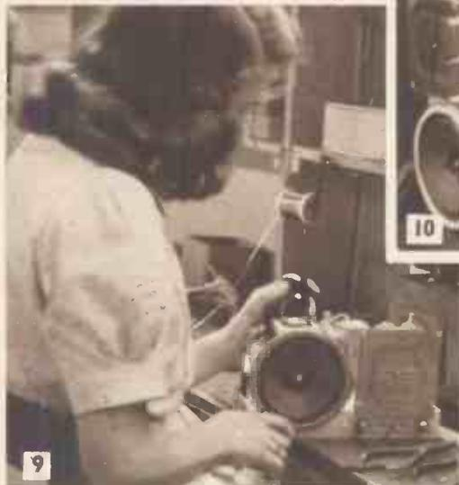
9. The valves are fitted for the first time and the scale is added to the scale plate by four press studs. With the addition of the pointer and dial indicator the chassis is ready for a series of severe tests
