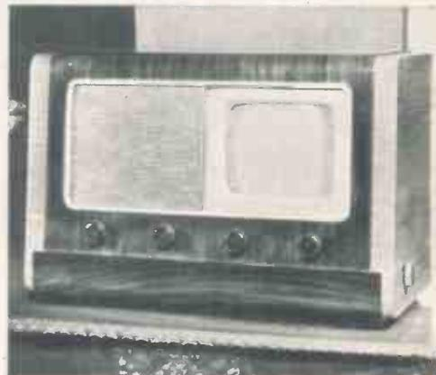
The Philips horizontal Television Unit is built for television and accompanying sound only. It is one of the smallest table vision receivers available, and is not to be confused with an add-on unit
