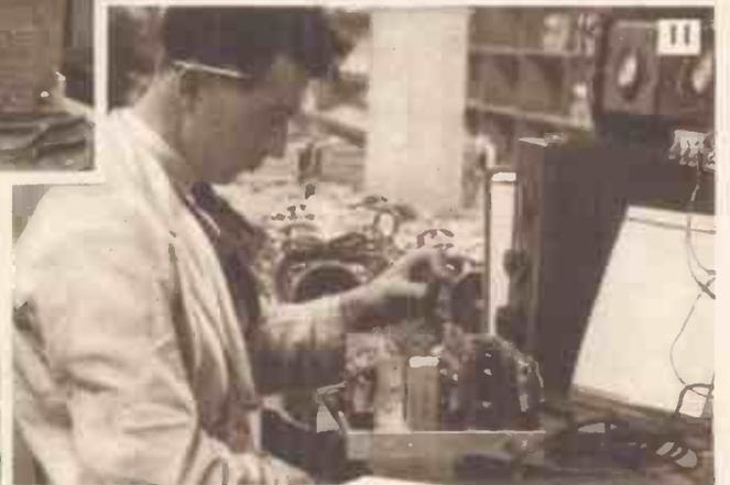
11. On the Intermediate Frequency test the I.F. transformers are tuned to a crystal control oscillator, thus ensuring accuracy of the final calibration
