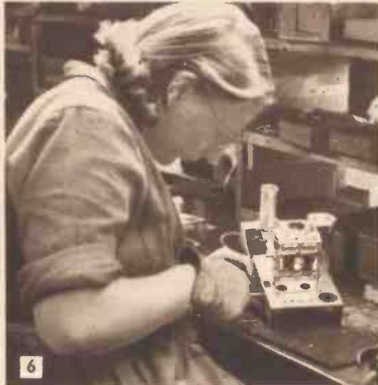
6. The next operator adds the gang condenser and the intermediate frequency transformer, soldering a small number of additional components and wires, all furthering the circuit to completion
