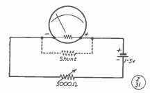
Fig. 5. Set-up for adjusting current-range
