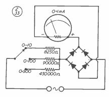
Fig. 7. The basic AC voltmeter.
