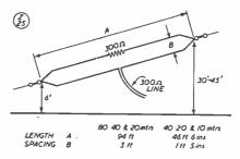
Fig. 7. A recently developed amateur aerial design, suitable for both transmission and reception. It is a multi-band system, and therefore is becoming popular, particularly as space requirements are reasonable. This system is known as the "T2FD."
