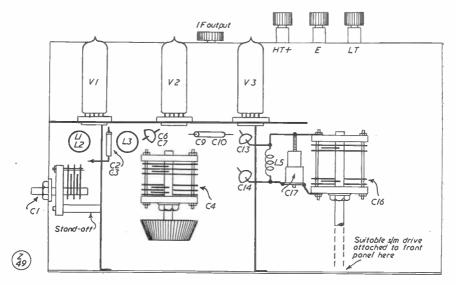
Fig. 2. Physical layout for the G2IQ two-metre converter; the oscillator stage is to the right, the mixer in the centre, and the RF stage at left. Some valuable practical advice on construction is given in the article.
