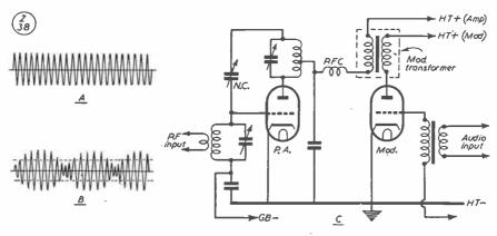
This sketch illustrates the answer to Question 1, sections A, B, C, being Figs. 1, 2 and 3 respectively. "A" is the unmodulated carrier, "B" a carrier wave with modulation on it, and "C" a suitable modulating circuit.
