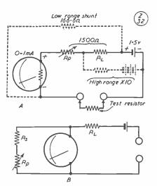
Fig. 6. (A) Basic ohmmeter, showing in dotted outline methods used to read higher and lower resistances than those provided for within the basic range of the instrument. (B) The shunt-type zero adjuster, which gives more accurate setting, as explained in the text.
