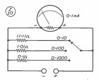
Fig. 3. Basic multi-range DC milliammeter.
