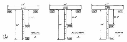
Fig. 2. A 67-foot wire, commonly used because it is one of the useful resonant lengths and within the space available at many amateur locations, with various modes of operation, as explained and discussed in the text.
