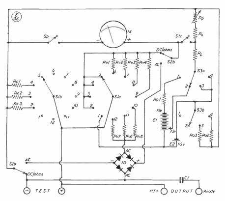
Fig. 10. Circuit covering all the possibilities discussed in the text, resulting in a very versatile instrument giving both AC and DC readings over a wide range, as well as resistance values.
