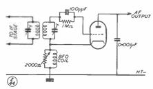
Fig. 2. A triode valve connected to operate as a detector and beat frequency oscillator stage. The variable resistor controls the oscillation.
