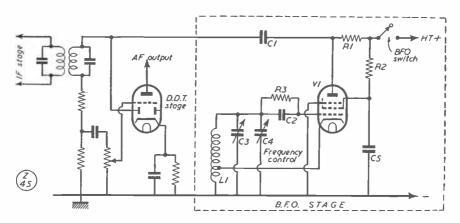
Fig. 3. Using a separate Beat Frequency Oscillator, as described in the text. To the left is the existing receiver output stage, showing the point of connection for the BFO injection. Values are: C1, 2-5  $\mu\mu F$ ; C2, 100  $\mu\mu F$ ; C3, 100-500  $\mu\mu F$  variable, as required; C4, 25  $\mu\mu F$ , variable; C5, 0.1  $\mu F$ ; R1, 27,000 ohms; R2, 220,000 ohms; R3, 47,000 ohms;
