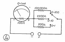
Fig. 1. Basic multi-range DC voltmeter.
