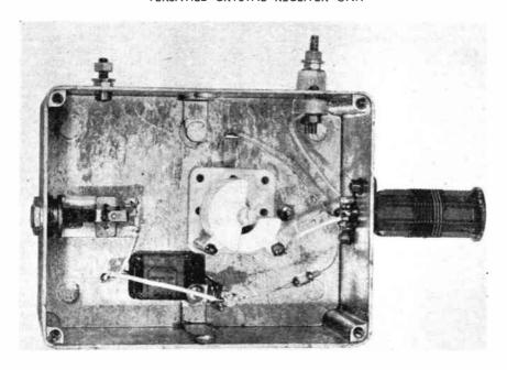
Interior construction of the Crystal Unit, showing layout and wiring -- what could be simpler!
