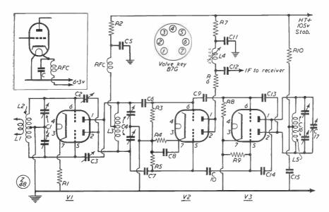
Fig. 1. Circuit of the two-metre converter using 6J6's, as described in detail in the article. The symmetry of the electrical layout should be noted — this should be translated into practice in the actual construction, of which one possible form appears at Fig. 2.
