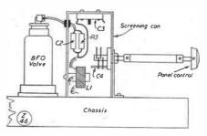
Fig. 4. In Fig. 3 is shown the circuitry for a useful BFO unit, external to the receiver, but for which space could usually be found on the average chassis. This sketch shows a suitable constructional layout.
