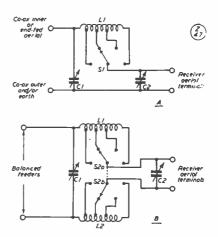
Circuits for the front-end tuner discussed in the text. An aerial coupler of this sort will nearly always give much improved results and is very desirable for serious DX work on the S/W bands.
