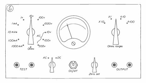
Fig. 11. Suitable panel layout for the instrument for which the full circuit is given at Fig. 10.
