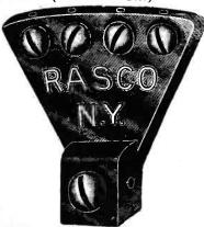
Illustration by Courtesy of Radio Specialty Co., Inc. Fan Connector—The leads from each wire of a multi-wire aerial go to the wide portion and are held by the set screws: the lead to the set goes to the small end.
