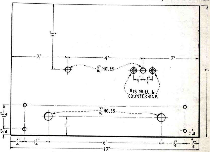
Front panel layout of the amplifier with dimensions of the holes to be drilled.
