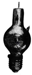
Fig. 12. A typical rectifier tube. The screw-base allows it to be inserted in a standard lamp socket from which current is obtained for the filament. Connection is made to the graphite disc by means of a Fahnestock con-nector which clips on to the wire post project-ing from the other end of the tube.
