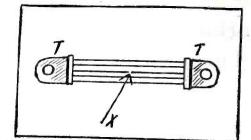
Fig. 2. This illustrates why Litzendraht must be well soldered.
