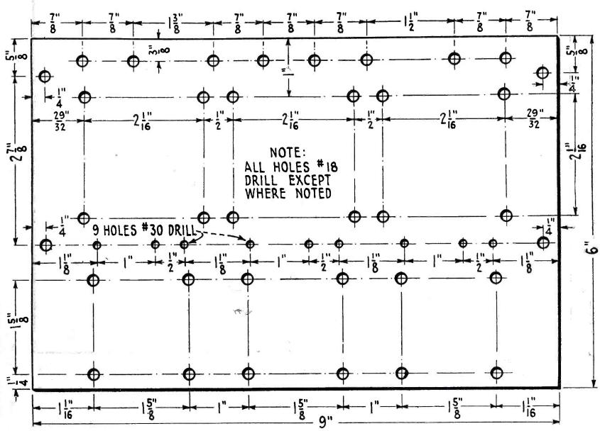
Details for drilling the bakelite or hard rubber sub-panel on which the three choke coils, sockets and hinding posts are mounted. Note how the sockets are mounted in the accompanying photo. All connections are made beneath this sub-panel.
