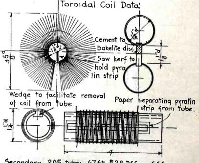
Secondary 205 turns 67ft #28D5C or 5CC Primary 20ft. #28D5C or 5CC to extend over entire length of secondary. Primary + secondary are cemented to pyralin strip with collodion.
