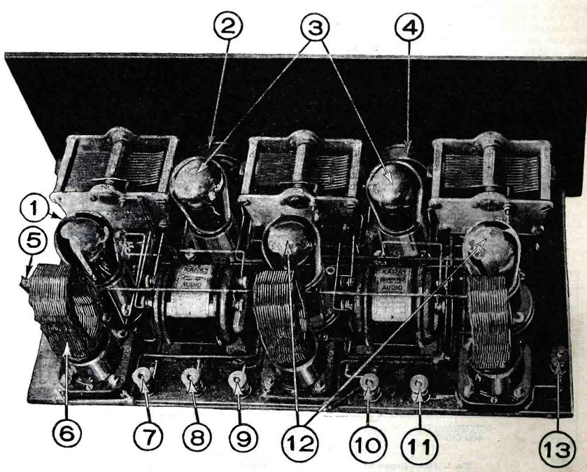
Rear view of the three-range receiver. 1 is the detector tube; 2, a potentiometer; 3, radio frequency amplifier tubes; 4, a rheostat; 5, the gridleak; 6, removable coil for different wave-lengths; 7, +45 volts; 8, +"A" and -"B"; 9, -"A"; 10, +90 volts; 11, antenna binding post; 12, audio frequency amplifier tubes; 13, the ground binding post.
