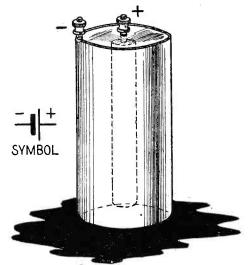
Dry cell showing positive and negative electrodes.
