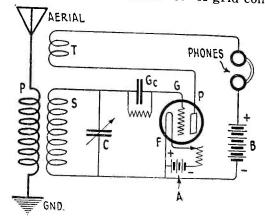
Regenerative circuit in which the coil "T" returns, or "feeds back" to the grid circuit a portion of the radio frequency current in the plate circuit, resulting in increased amplification.
