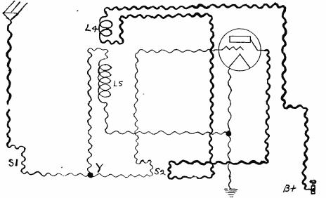
Fig. 4. By switching to wireless range, the vibrations divide at Y, and are tuned through L5.
