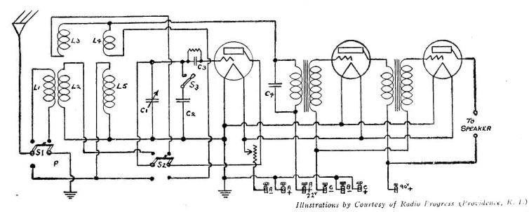
Fig. 1. This hook-up uses a four-pole double throw switch, shown here divided into S1, S2. The entire range of broadcast and code may be heard.
