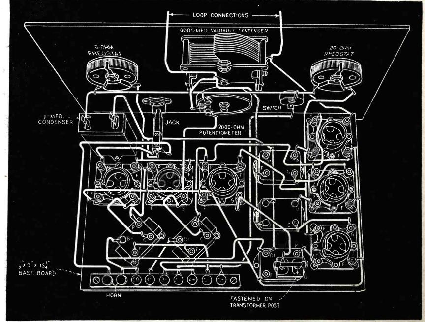
The above shows the complete assembly and wiring of the six-tube self-contained loop set. The binding posts on the insulating strip are connected as follows: Reading from the left—First two, loud speaker; third, 90 volts +"B" battery; fourth, 45 volts +"B" battery; fifth, "B" battery —; sixth, "A" battery — 4½ volts; seventh, "A" battery +; eighth, "C" battery — 4½ volts; and ninth, "C" battery +.
