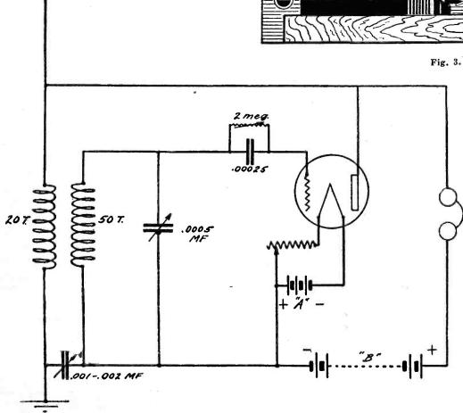
Fig. 4. Circuit diagram of the set.
