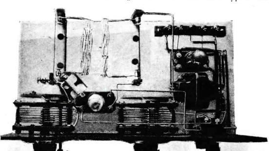
that both capacity and resistance losses are reduced to a negligible amount. The position of the coils is such, relative to the other apparatus, that neither dielectric materials nor metal parts are situated closely in the fields of the coils. yet, all connecting leads in the radio frequency portions of the circuit are short and direct.
