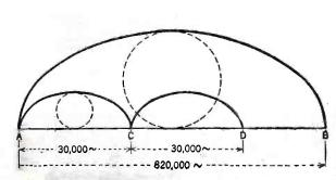
Fig. 1. The broadcasting band of frequencies is 820,000 cycles wide and is represented here by taking a point on the circumference of a wheel and marking out its path as it rolls along the frequency line. At the end of one complete revolution the point has traversed 820,000 cycles. The smaller wheel representing the oscillator dial traces a similar path but in one revolution it traverses only 30,000 cycles. There are two points 60,000 cycles apart that a given station may be heard.
