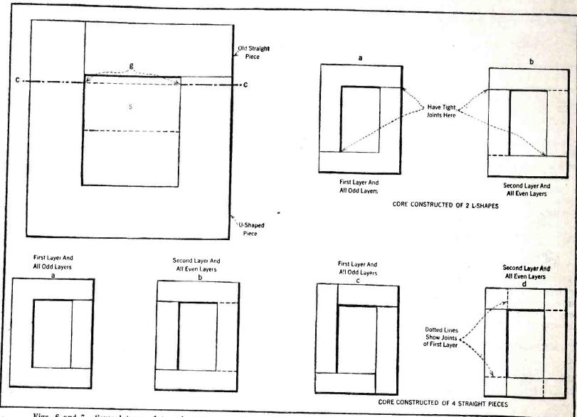
Figs. 6 and 7. Several types of transformer cores which may be employed in this construction. The sketches are self-explanatory.
