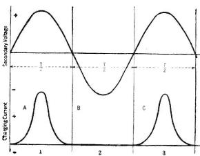
Fig. 1. A graphic representation of how a charger functions. The curve labeled "secondary voltage" shows the sine wave-form of the 60-cycle lighting circuit. That curve labeled "charging current" shows the portion of the alternating wave which is rejected in the rectifier allowing only the periodic pulsations of that portion of the curve where the current is "direct current" to enter the battery.
