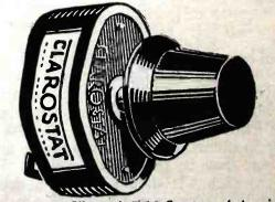
"Illustrations by Courtesy of American Mechanical Laboratories, Inc., Brooklyn, N. Y. Q. 14 (Fig. 3). Type of variable resistance which was used to aid control of regeneration.
