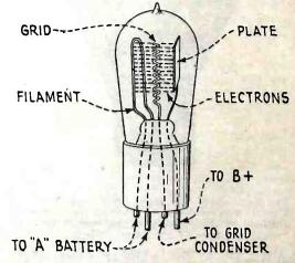
When an "A" battery is connected to the filament terminals, heating the filament, electrons are thrown off and fill the space between filament, grid and plate.
