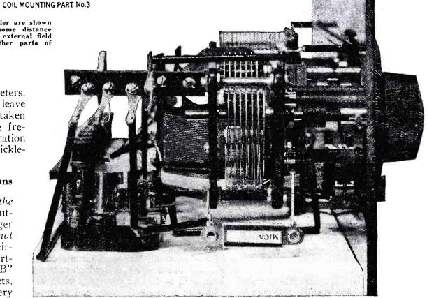
Fig. 11. End view showing the method of placing the condenser some distance behind the panel to lessen body capacity effects. The separation of the coupling coils is clearly shown here.
