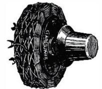
Illustrations by Courtesy of American Mechanical Laboratories, Inc., Brooklyn, N. Y. Q. 22 (Fig. 2). Antenna coil on left, and detector tuner on right, which were used in the "Neutralized Baby Super" as described by Mr. Holtz.
