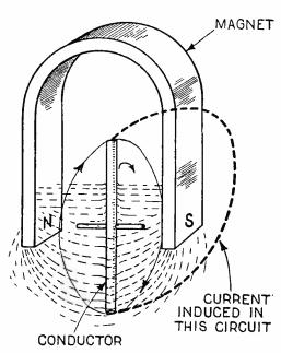
Simple method of producing electric currents by causing changes in the magnetic field.
