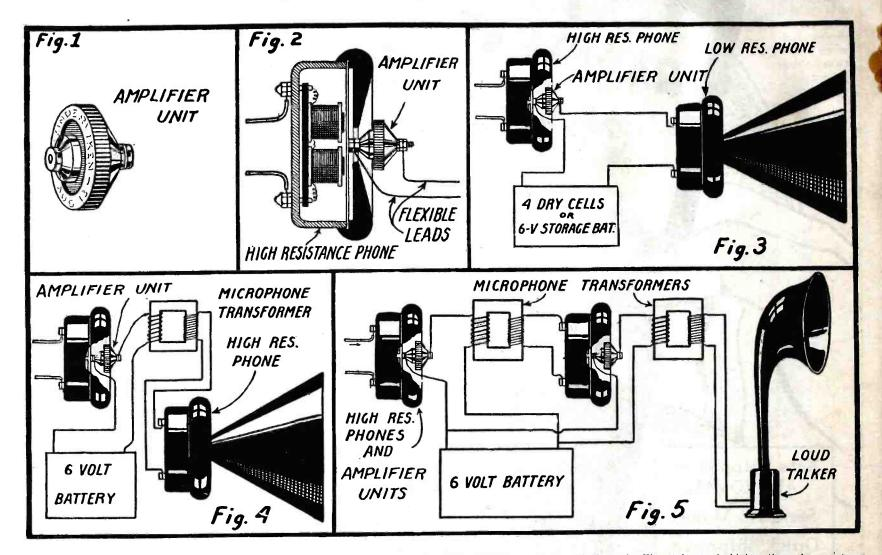
FIG. I shows the amplifier unit, actual size.
