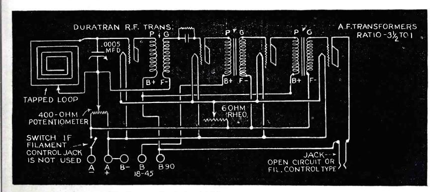
Schematic diagram of the set. Note the tapped loop employed. This loop is of the Lincoln or Nazeley type.
