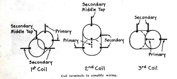
silk or paper between the two windings. The coils are placed in the set at right angles as shown in diagram.
