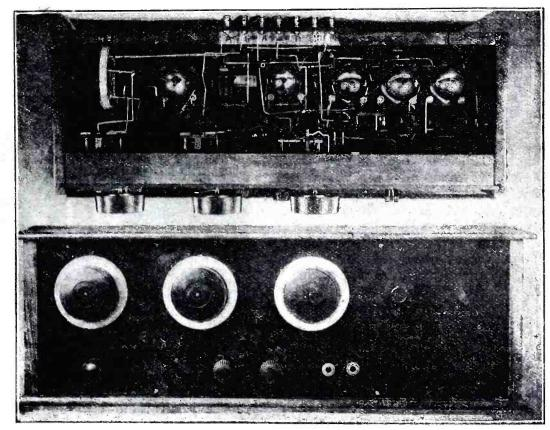
Fig. 6 (top), rear view of a set built by C. V. Curthoys, of Lenox, Mass. Fig. 7 shows the front view of panel and cabinet. It is a 6-tube set, built for a deaf man. There are one stage of tuned RF, regenerative detector, one stage of transformer audio and three stages of resistance audio.
