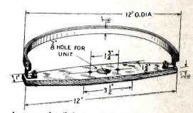
A more detailed drawing of the hoop and baseboard system of the paper disc loud speaker. For the sake of clearness, half of the hoop has been removed.
