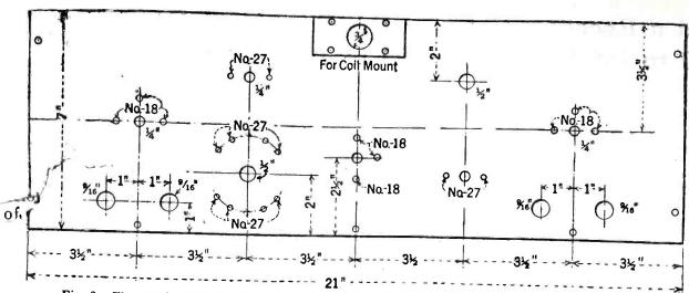
Fig. 3. The panel layout for the universal receiver. The numerals near the designated holes indicate the size drills to be used in drilling them.
