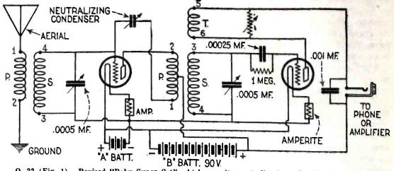
Q. 22 (Fig. 1). Revised "Baby Super Set" which permits neutralization. In this circuit using 201A tubes up to 90 volts may be used for detector "B" battery, but the correct amount must be determined by experiment.
