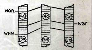
How a three dial set can be logged. Three calibrated strips are numbered to correspond to the divisions of the dials. Thus, the dial settings for each station can be logged as shown.
