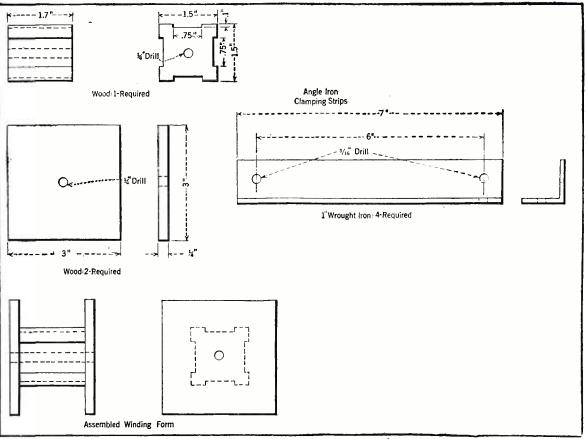
Figs 8 and 9. Details of construction for the coil winding form and angle pieces. Note that some of the dimensions are indicated in decimals and it is suggested that constructors adhere to these specifications.
