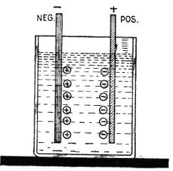
Illustration showing the action of ions in a primary cell.
