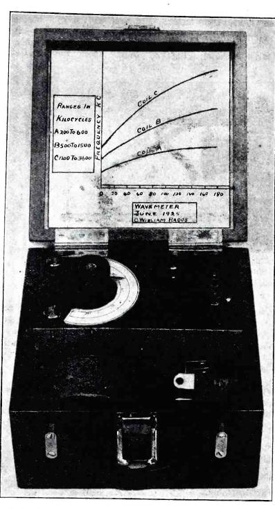
Fig. 2. Here is a view of complete meter. Extra coils are in front. The curves on cover read direct
