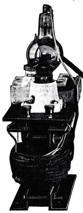
Fig. 11. Another view of the completed charger. This is an end-view picture and shows how the angle pieces are employed not only to hold the core together but as fect and supports for the bakelite shelf.
