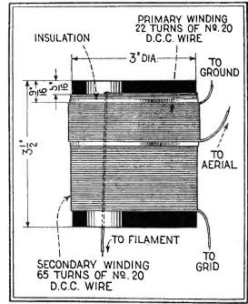
Q. 14 (Fig. 1). Radio frequency tuner for "Baby Super Set."
