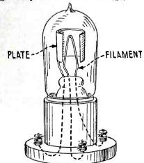
Fig. 1. The Fleming valve, which contained but two elements; i. e., filament and plate. It was the forerunner of the modern vacuum tube.
