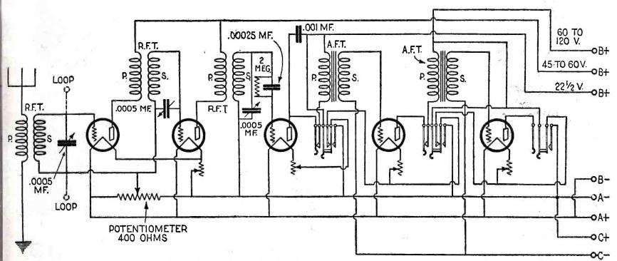
Fig. 1. Circuit diagram for receiver that has a wave-length range from 40 to 555 meters.
