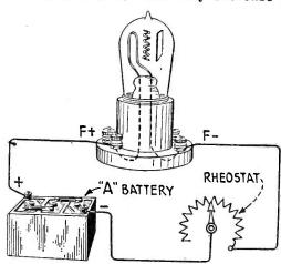
Fig. 2. Showing method of connecting a rheostat in "A" battery circuit of a vacuum tube.
