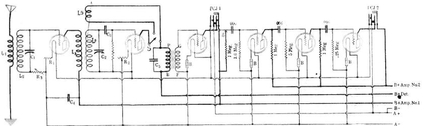
Fig. 5. The circuit diagram of the wiring of the set built by C. V. Curthoys. Photos of the set are shown in Figs. 6 and 7.
