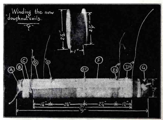
Fig. 1. Showing (on top) the spool which constitutes the mount or form on which the coil is placed after being wound, and (lower view) the original form on which the wire is placed prior to removal. The text explains the designations.
