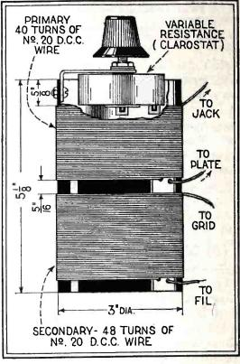
Q. 14 (Fig. 2). Tuner, tickler and variable resistance used in Mr. Feeney's experiments with the "Baby Super."
