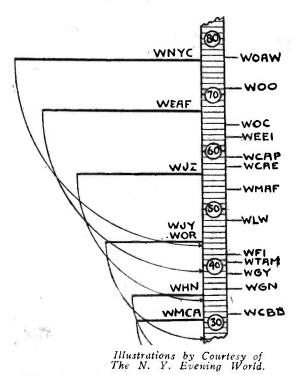
Calibration scale of oscillator dial of a superheterodyne receiver. In making logs for super-heterodyne sets it is advisable to allow an ample margin on the left of the chart in order to record harmonics as shown in the log above.
