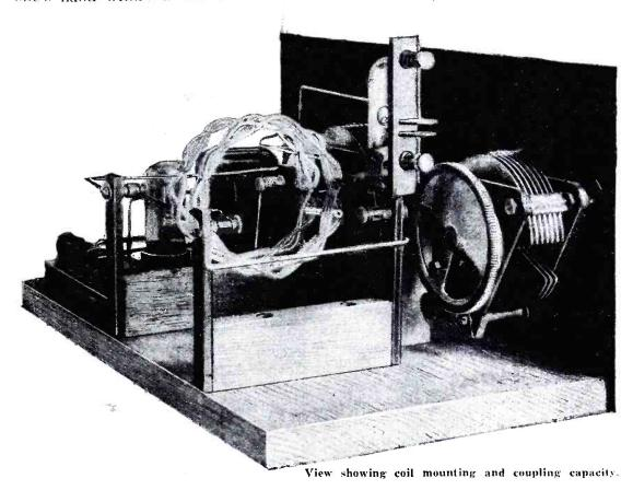
high potential point such as the autenna condenser or the grid coil will introduce enough capacity into the circuits to completely detune them and tune out a signal.
