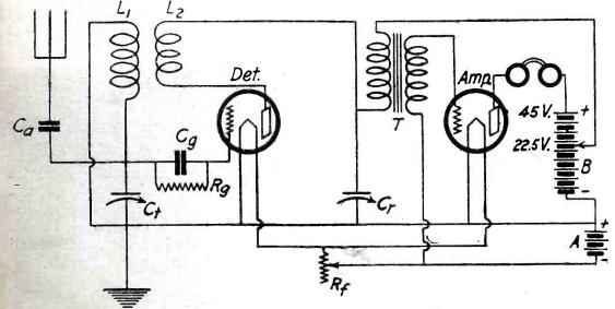
Schematic diagram of the 9XH-9EK short wave set No. III. See nomenclature at the right for parts.
