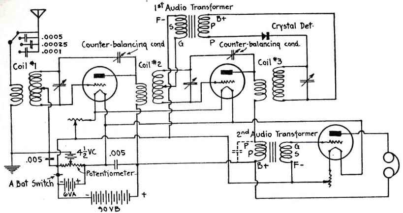
Circuit diagram for three-tube reflex receiver.
