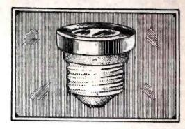
Fig. 1. A common type of fuse used in lighting, heating and power circuits.
