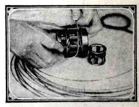
Winding the bare copper wire and the heavy cord side by side on the secondary section of the stator form.
