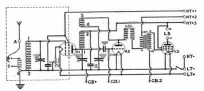
A BOVE is a circuit diagram of the Mullard S.G.P. Master Three. One of the main points in the design is the fact that selectivity may be adjusted for every individual case. This is effected by the suitable use of the alternative aerial taps, and in extreme cases, by a suitable modification of the aerial turn numbers.
