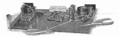
SHOWING the baseboard components placed into position and partly wired-up. Here the dual mounting of the specified valve-holder is to be seen. That for the screened-grid is vertical. It is mounted flat for the Mullard Pentone. The illustration below shows a closer view of the panel.
