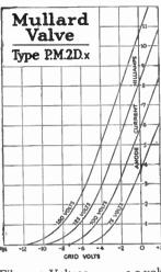
Max. Filament Voltage 2.0 volts. ... Filament Current ... 0.25 amp. ... Max. Anode Voltage 150 volts. ... ... 10,700 ohms. \*Anode Impedance... \*Amplification Factor 13.5 . . . 1.25 mA/Volt \*Mutual Conductance . . .
