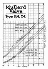
Max. Filament Voltage 4.0 volts. ... Filament Current ... 0.15 amp. ... Max. Anode Voltage 150 volts. . . . Auxiliary Grid Voltage As H.T. + . . . \*Anode Impedance... 28,600 ohms. . . . \*Amplification Factor 62 . . . \*Mutual Conductance 2.3 mA/Volts • • • \*At Anode Volts 100, Grid Volts Zero, Auxiliary Grid Volts 100.
