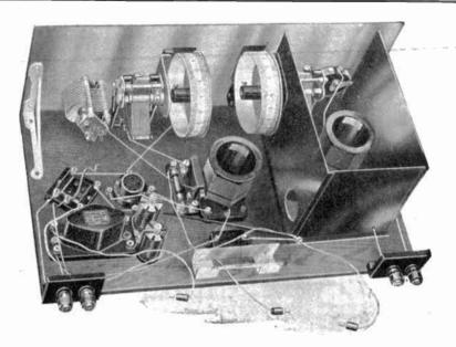
$A\,S$  was the case with the previous Mullard Master Three Receivers, all battery leads are taken direct from the terminals of the components. Needless to suggest the method eliminates a number of rigid wires.
