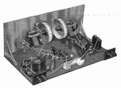
A NOTHER view of the receiver which provides a number of useful points to note during the construction. Connecting Links were actually used for the wiring-up of original receiver.
