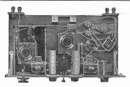
A N illustration of the combined-wave model, which, in conjunction with the "Wiring Step by Step," makes the assembly of the receiver an easy undertaking, even for those without any technical experience whatever. The disposition of the coils is clearly shown. They should be fixed to the hasehoard in the manner described in the text.
