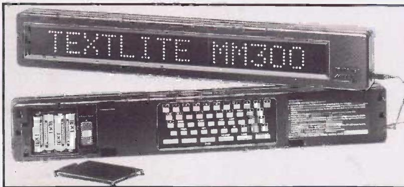
MOVING MESSAGES speak louder than words is the campaign slogan from Textlite UK. The Washington, Tyne & Wear company manufactures an electronic visual display unit which can carry horizontal and vertical messages – up to 200 words memorised at any one time.
