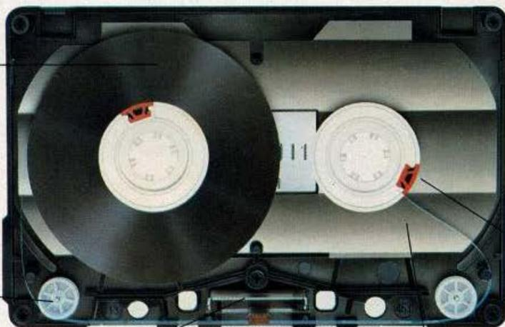
New exact pressure pad: thicker, with a strong spring, and twice as accurate as in conventional cassettes. It keeps the tape precisely perpendicular to the tape head.
