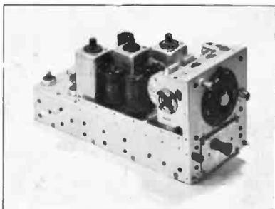
BC-453. THE Q5'er. 190/550 kc/s. These sets are now well known for their use with communication receivers to give improved selectivity, attenuating unwanted signals by at least 30 db., making single signal reception easily obtainable, and improving even the H.R.O.
