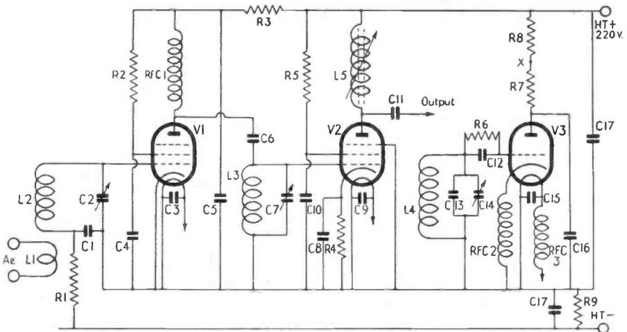
**Fig. 1. Circuit of the G2XC Converter complete.** There is no direct connection between oscillator (V3) and mixer (V2) it being found that sufficient stray coupling exists for the required oscillator injection. The working details and the design of the unit are fully discussed in the text. (Suppressor V1 should be earthed in this diagram).
