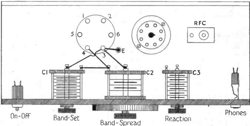
Fig. 2. Suitable parts layout, in plan view.
