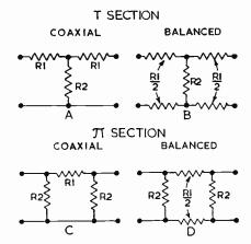
Fig. 2. Four basic types of attenuator networks as used for television purposes. These are fully discussed in the text. In examples A and C the outer conductor is taken to the lower leg of the network.
