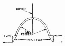
Fig. 5. Illustrating how the input pad of Fig. 4 can be used to terminate the feeders where two receivers are using the same dipole aerial.
