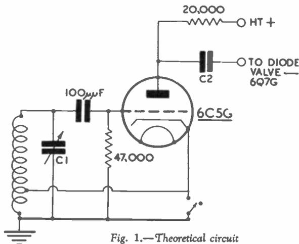
Fig. 1.—Theoretical circuit
