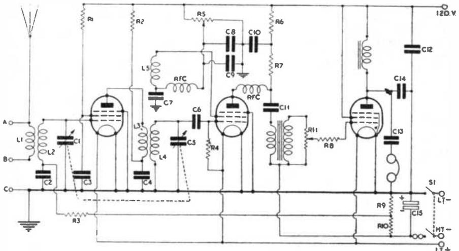
Fig. 1. Theoretical Circuit
