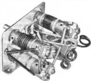
We manufacture permeability tuned iron cored coils for use in a small one-valve set to a large superhet, which have a greater "Q" than air-spaced coils, and will therefore give you a higher gain and also increased selectivity. Other advantages of small permeability tuned iron-cored coils, are a decided saving in space and at the same time allowance for a reasonable latitude in changing the inductance of the coil.
