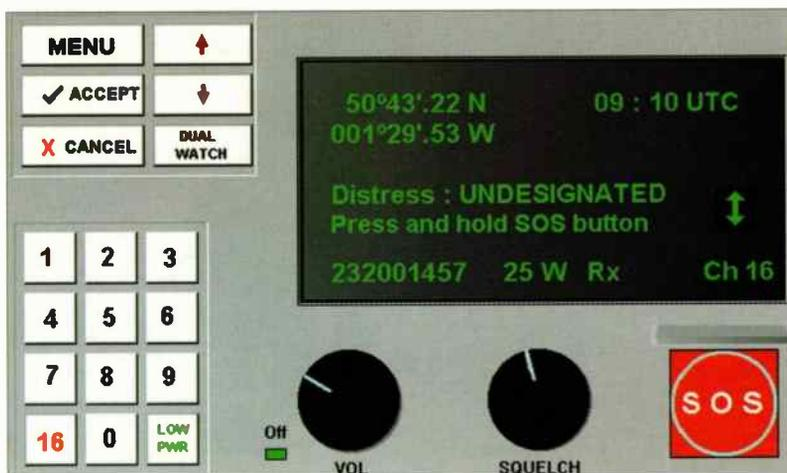
Fig. 2: DSC controller sending distress message.
